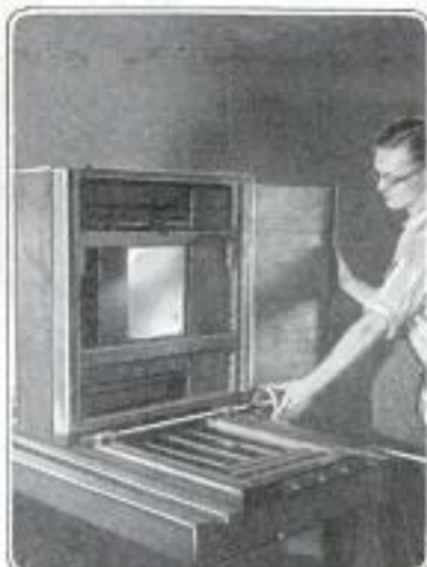
Sensitized Plate in Position in Camera behind Half-Tone Screen to Make the Dots
