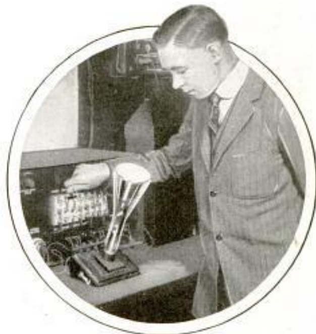
Tube Devised So That the Alternations of High-Frequency Currents May Be Followed
