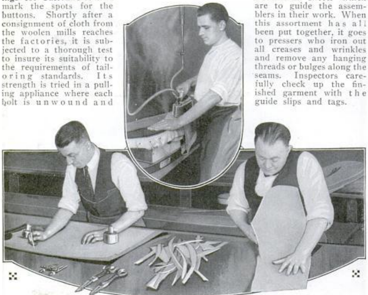
Marking and Cutting Pasteboard Patterns Which Are to Guide Cutters in the Shaping of Suit Pieces; Above, Presser Removing Creases and Wrinkles from Finished Garment
