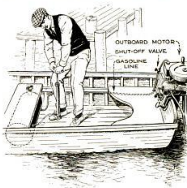
Auto Gasoline Tank in Boat Holds Large Quantity of Fuel for Small Outboard Motor
