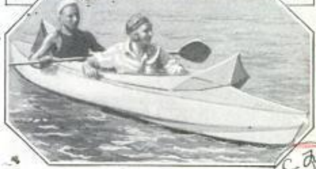
Collapsible Canoe Carried on Fender on Auto Trips, Which Can Be Assembled in Ten Minutes
