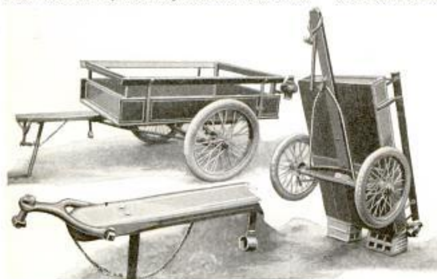
Light and Sturdy Trailer Can Be Built by Anyone from Old Automobile Parts to Carry Tools and Other Equipment
