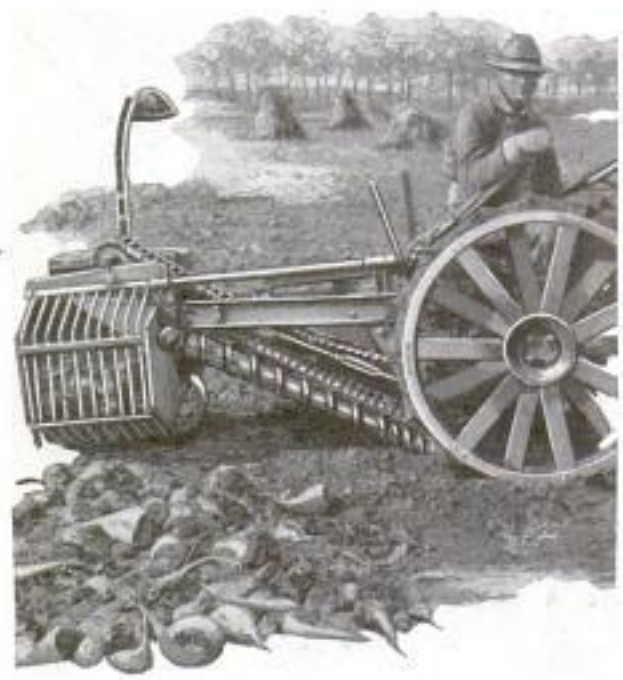
Beet Harvester in Operation behind Tractor Showing One of the Revolving Augers and the Hopper
