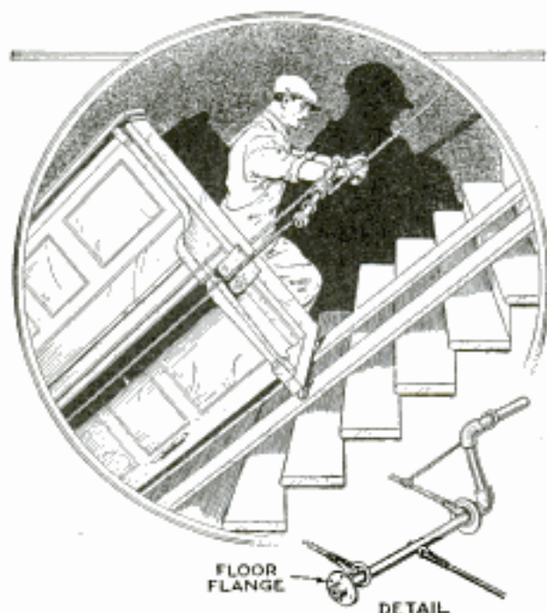
Simple Winch for Moving Pianos and Other Heavy Furniture up Steep Stairways
