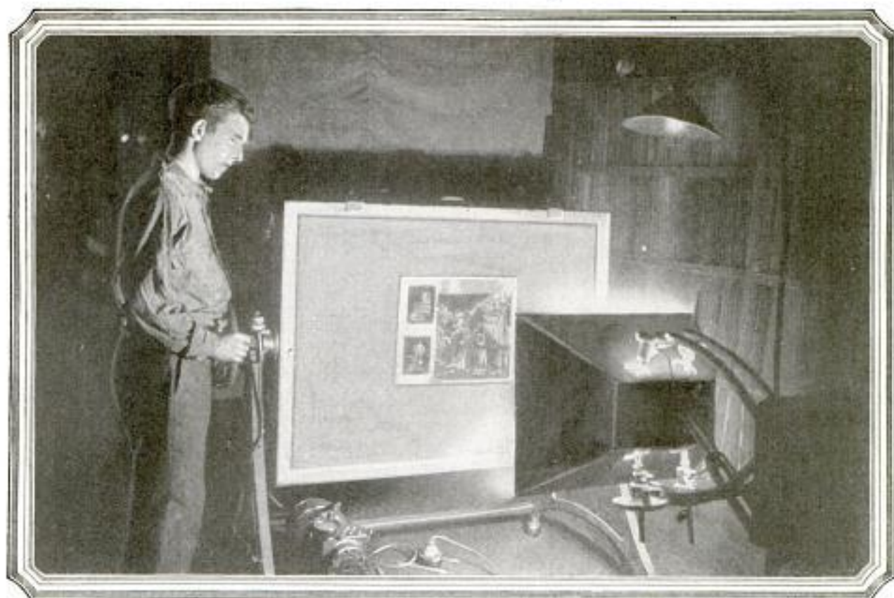
Printing the Photographic Impression upon Sensitized Copper Plate through the Negative Superimposed upon It and Exposed to Rays of Powerful Battery of Electric Lights
