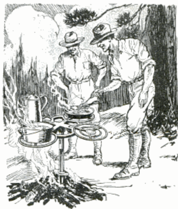
Sketch of Camp-Fire Cooker; Pots Are within Easy Reach on Grid Frame That Revolves
