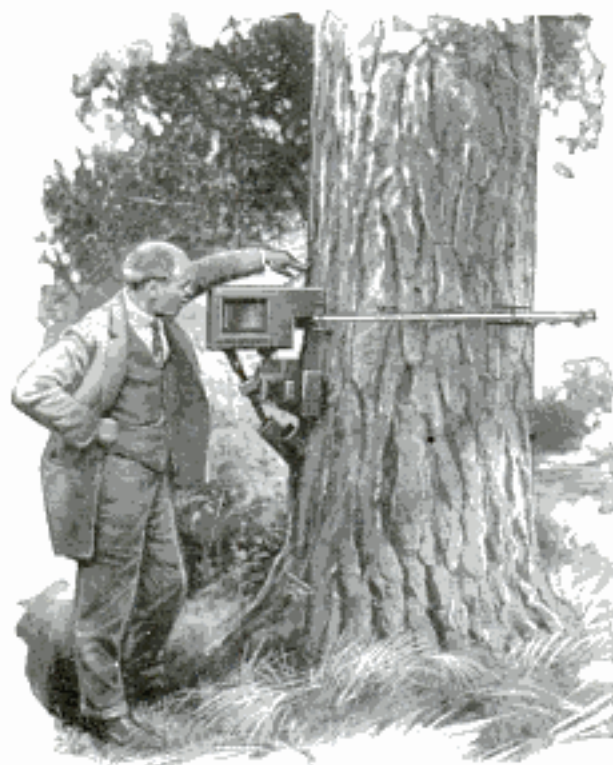
Instrument Attached to Pine Tree in California to Measure Its Rate of Growth
