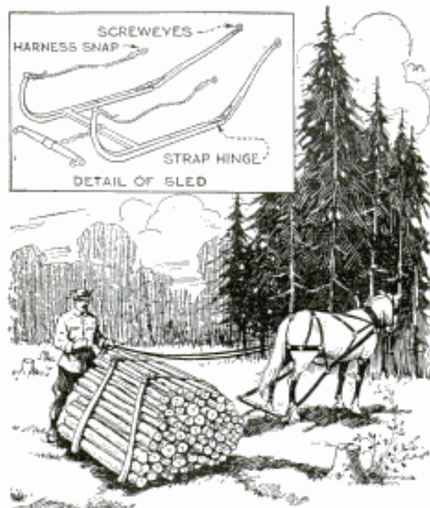
A Novel and Effective Sled for Transporting Cordwood
