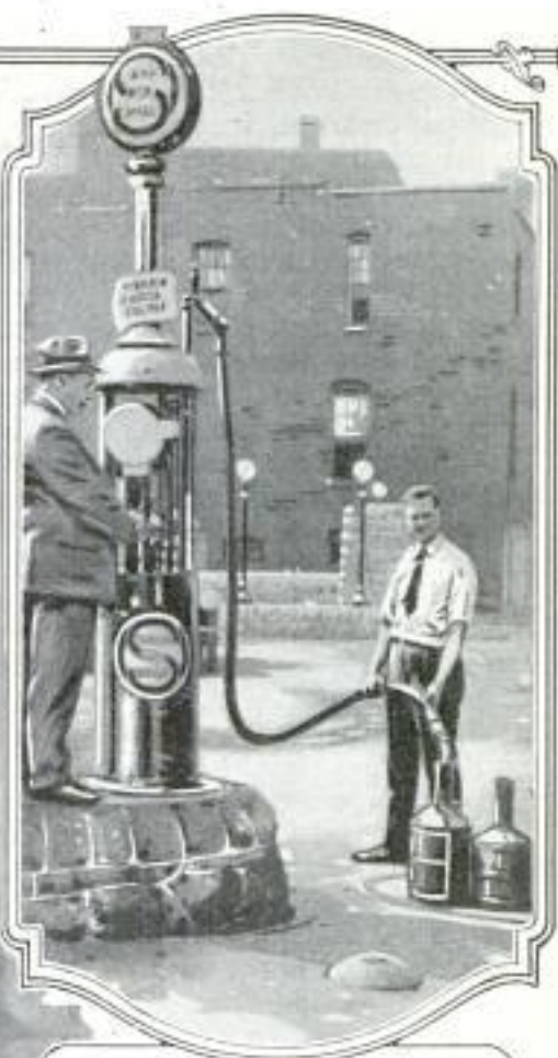
Inspecting an Automatic Pump at a Gasoline Filling Station to Insure Automobile Owners Full Gallons in Their Fuel Purchases
