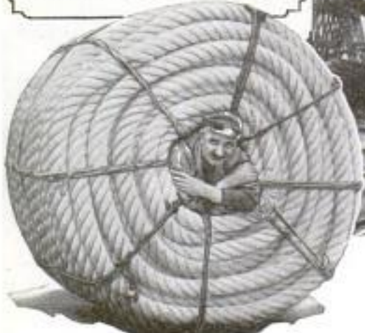
Cleaning the Barnacle and Rust-Covered Bottom of a Destroyer in Dock in Preparation for Protective Coats of Paint; Left, a Champion Rope Maker Framed in a Coil of Ten-Inch Rope That Weighs a Ton and a Half and Can Hold a Load of 75,000 Pounds
