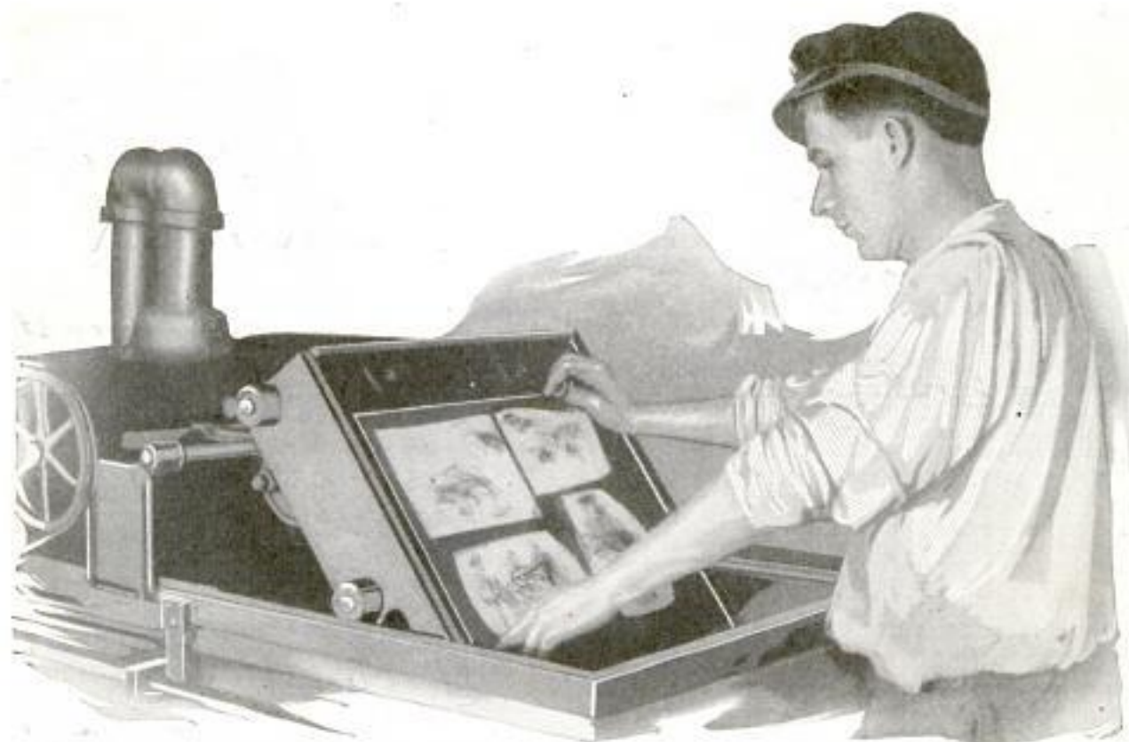
After Copper Plate Is Printed, It Is Etched in Machine Where It Is Sprayed with Acid Bath to Produce the Relief Surface Necessary for Impression on Paper
