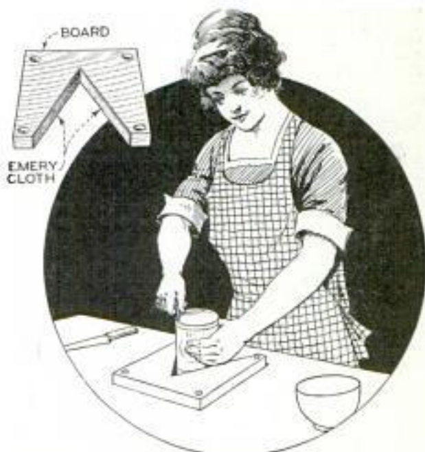
Opening Cans Is Made Easy for the Housewife by the Use of This Simple Holder
