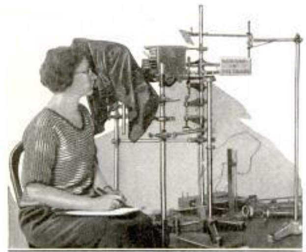
Radium Expert in Bureau of Standards Measuring Value of Metal with Gold-Leaf Electroscope
