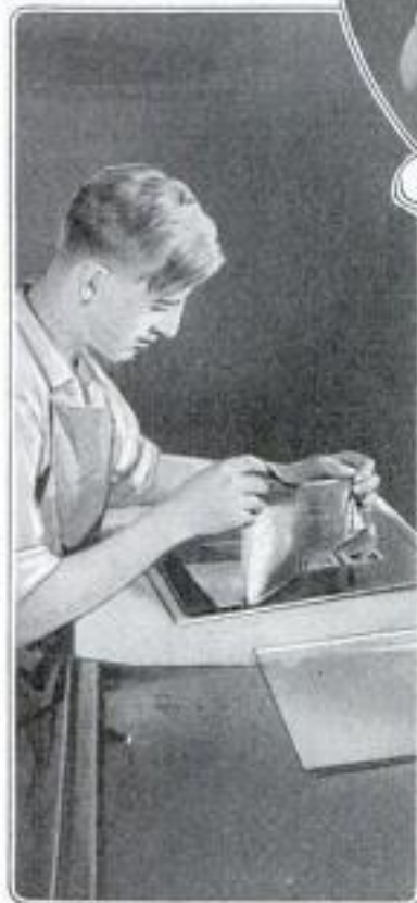
Lifting Film from Negative Glass after Soaking It in Bath of Acetic Acid
