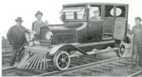
Automobile "Train," Adapted to Inspection and Emergency Service, Which Is Capable of High Speed
