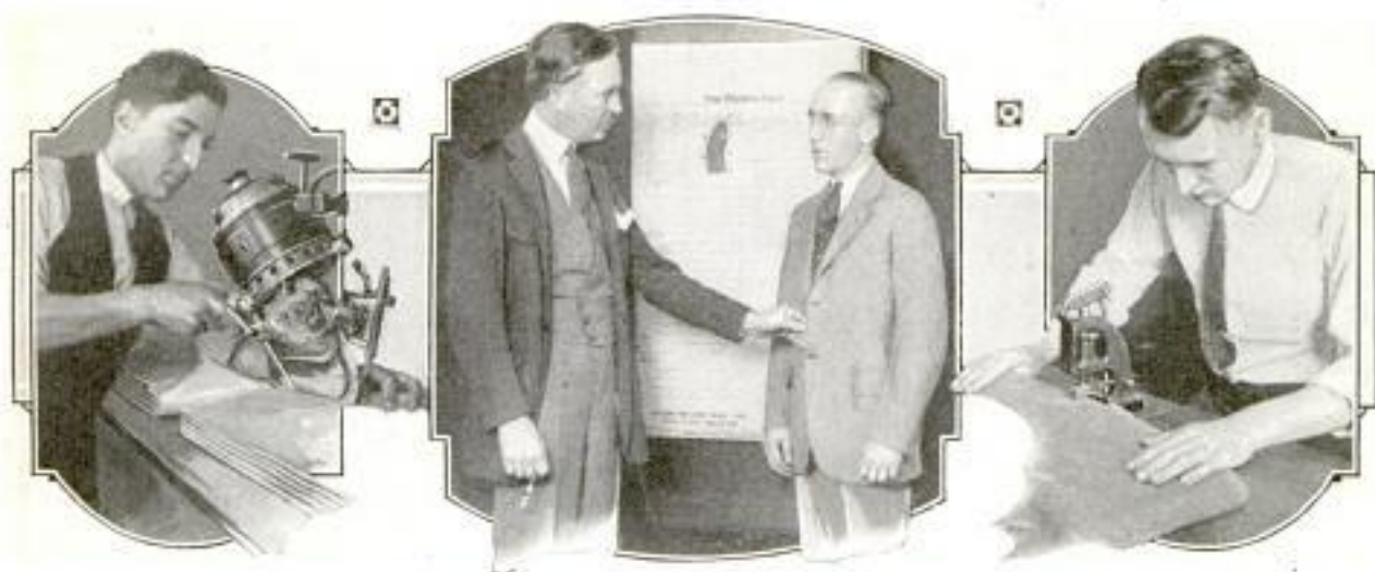
Motor-Driven Knife That Cleaves Its Way through Several Layers of Cloth; Designer Inspecting a Sample Suit Model and Cutter Notching Cloth to Guide Sewers in Assembling Pieces
