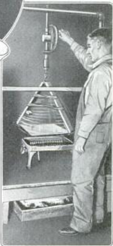
Drying Coated Copper Plate by Whirling It over Gas Flame in Dark-Room Cabinet
