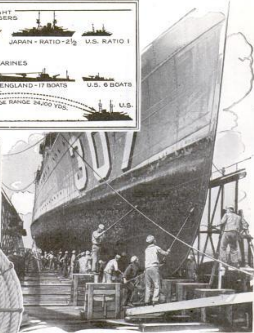
Cleaning the Barnacle and Rust-Covered Bottom of a Destroyer in Dock in Preparation for Protective Coats of Paint; Left, a Champion Rope Maker Framed in a Coil of Ten-Inch Rope That Weighs a Ton and a Half and Can Hold a Load of 75,000 Pounds
