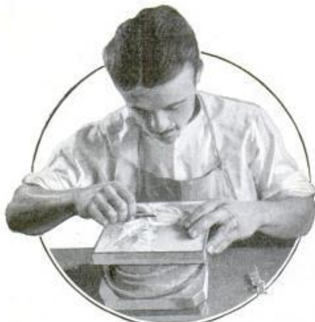
Tooling and Finishing Plate by Hand Removes Rough Edges and Secures Contrasting High Lights
