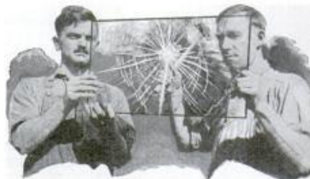
Testing Resistance of Pane of Bullet-Proof Glass with Blows of Heavy Hammer
