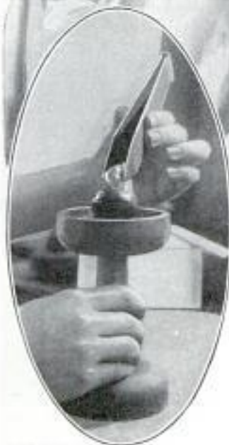
Setting the Mounts Containing Raw Gems in Holding Frame of Polishing Machine; Left and Right, Shaping the Soft Mold for the Diamond, and Placing the Stone in the Tip of the Cone
