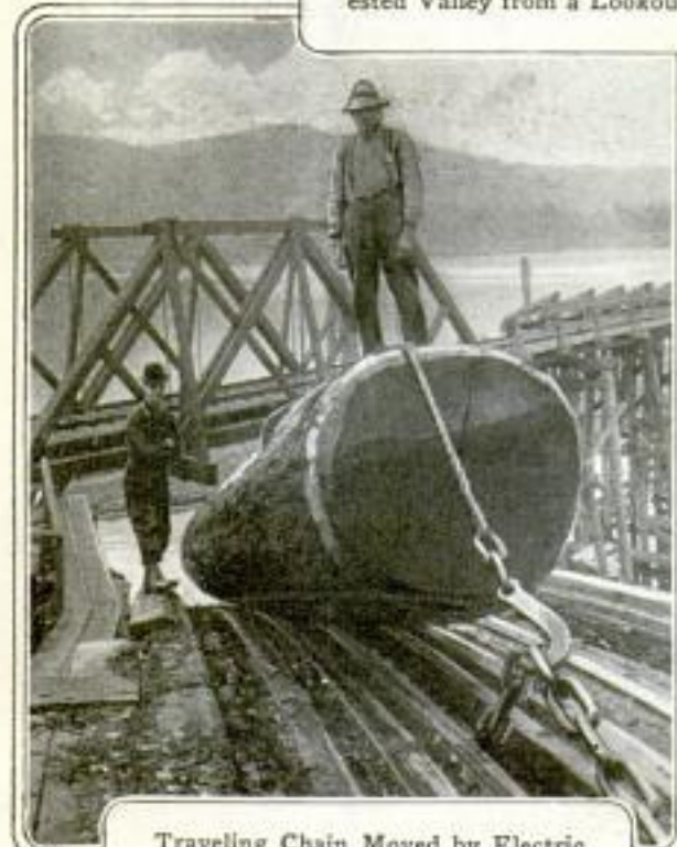
Traveling Chain Moved by Electric Power Which Transports Logs along Steel Skidway
