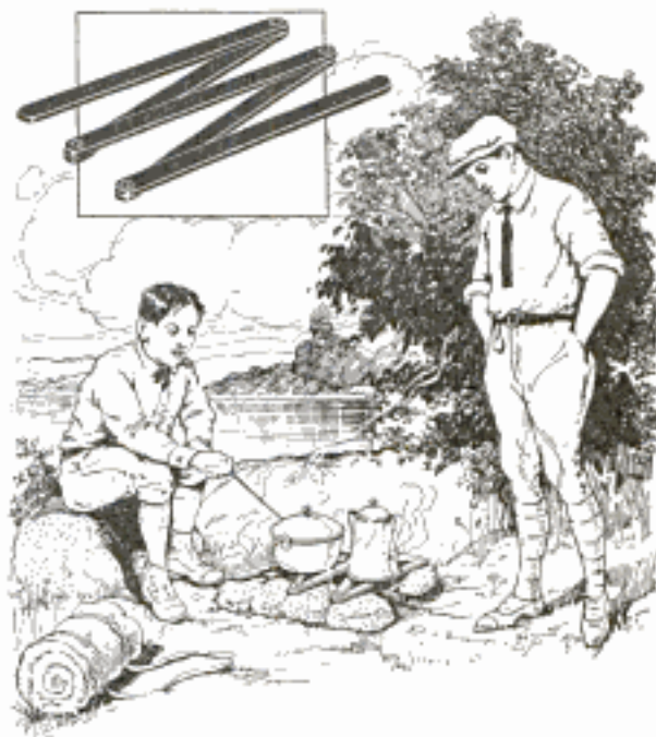
Campers' Fire Grate, Which Can Be Folded Up Compactly When Not in Use
