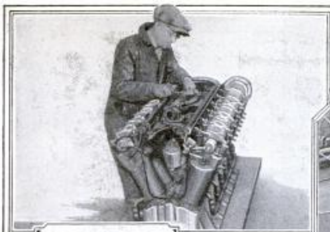
After a Hundred Hours' Running Time, the Big Liberty Motors Are Removed and Given an Overhauling
