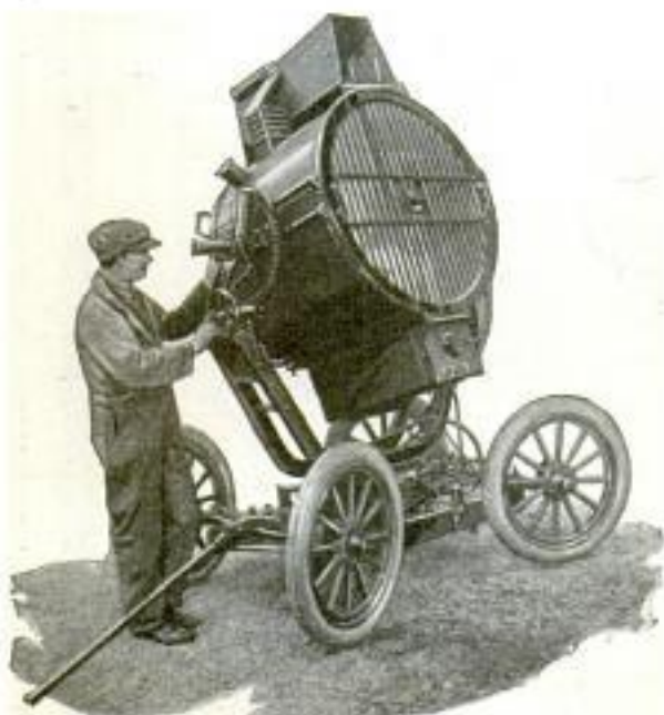
Looking Directly into the "Tunnel" Produced by Rays of 460,000,000-Candlepower Beacon; Below, Adjusting Angle of Portable Light
