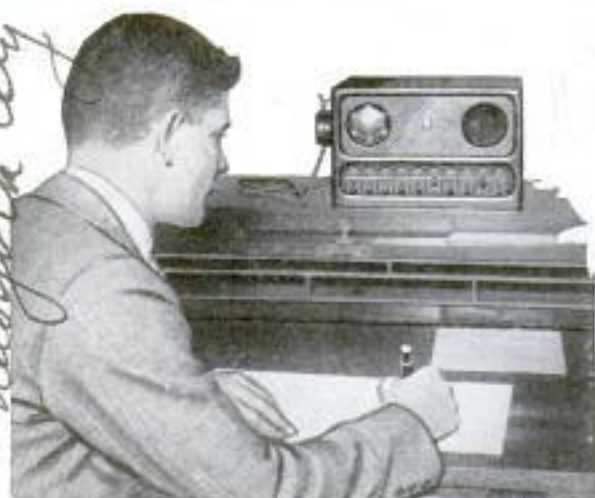
Party Telephone Instrument in Use; Keys Below Connect Offices in Any Combination Desired
