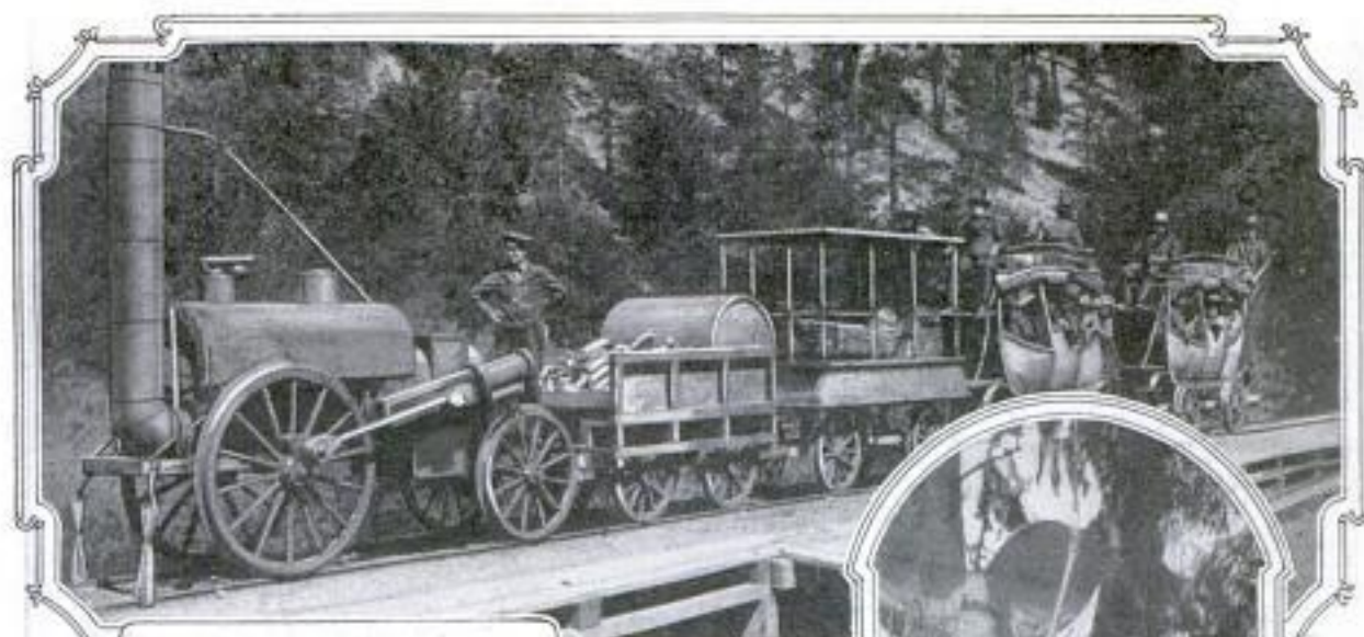
Modeled from a Picture of the Original, This Old-Time Railway Train Is Run by a Hidden "Gas" Engine
