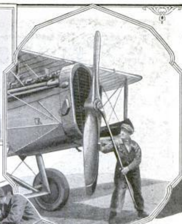
With a Twist or Two of His Wrench, Mechanic Removes a Propeller That Needs Repairing
