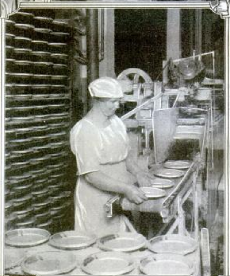
Pastry-Molding Machine That Makes "Open" Pies and Crusts for the Custard Varieties
