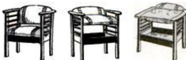
Convertible Chair with Seat Raised to Form Stool, and Placed as Table Top
