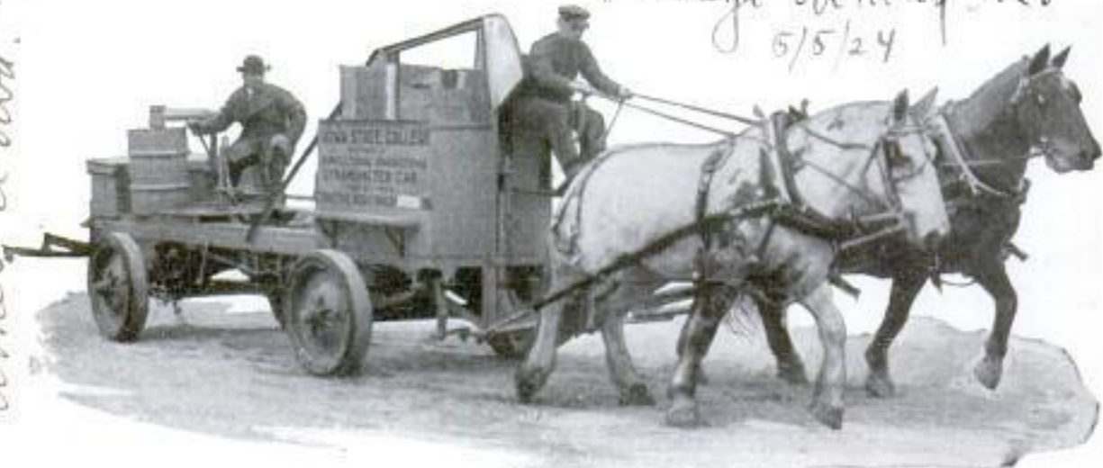
Pull-Measuring Wagon in Operation; When Team Is Started, Weights in Front Are Raised on Hydraulic Platform While Operator in Rear Controls and Observes Their Action
