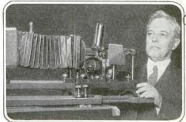
Inventor and His Camera with Transmitting Apparatus which Registers Waves Produced by Sound
