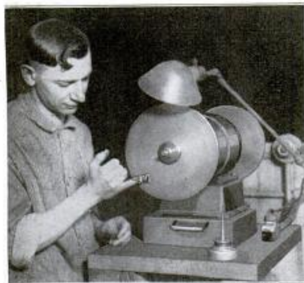
Copyright, Underwood & Underwood Operating One of the Gold-Polishing Buffers in a Large Jewelry Store
