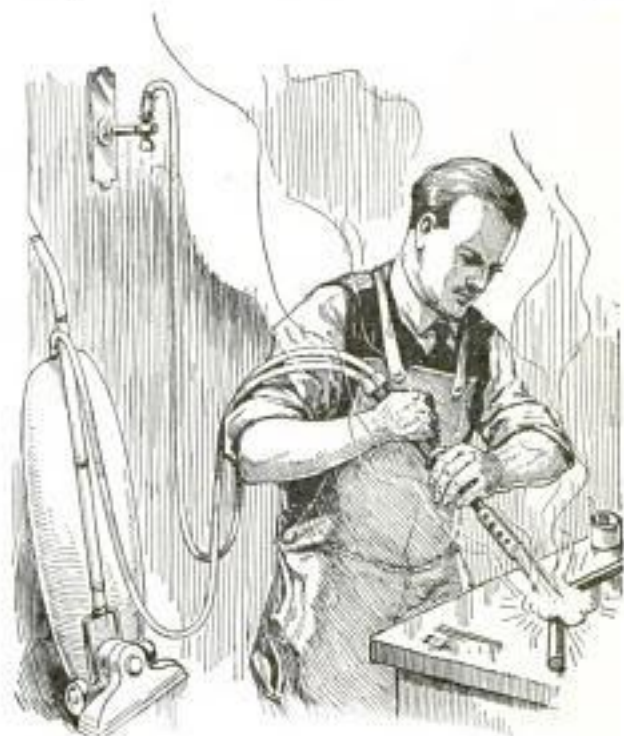
Hot Brazing Flame Produced by Using Ordinary Gas and Compressed Air from Vacuum Cleaner
