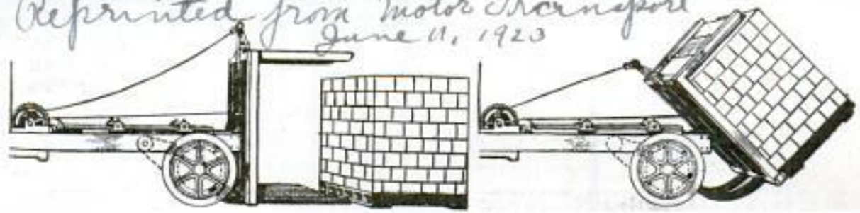
Loading Log Truck by Pulling Filled Platform over Rear; Diagrams Below Illustrate Working Principle of Winch Run by Motor and Winding Cable Attached to Sliding Body
