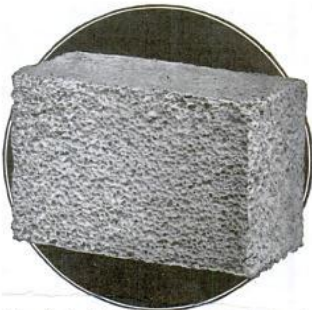
Cross Section of a Puffed Gypsum Block Showing the Large Number of Confined Air Cells
