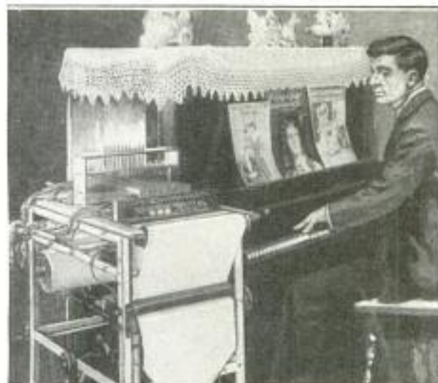
Inventor Playing Directly upon the Roll through the Record Punch Connected with Piano
