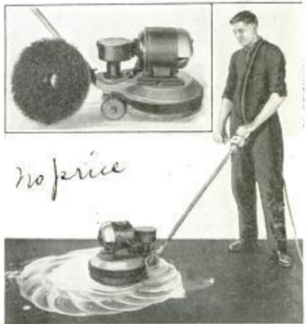
Cleaning Floor with Electric Scrubber; Above, "Close-Up" of Apparatus and Brush Attachment
