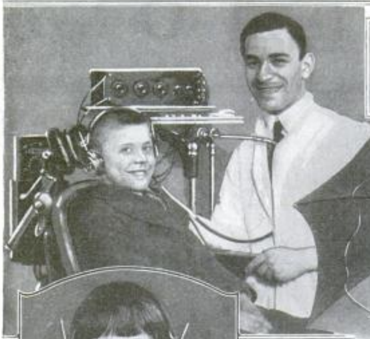
A Real Radio Fan: the Set Is Tuned by Opening and Closing the Leaf Coils
