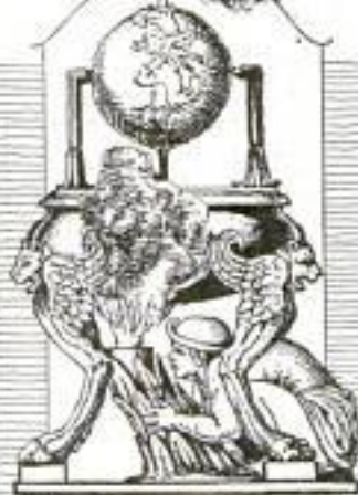
About 120 B.C. this Ancient Turbine Was Invented by Hero, a Scholar of Greece
