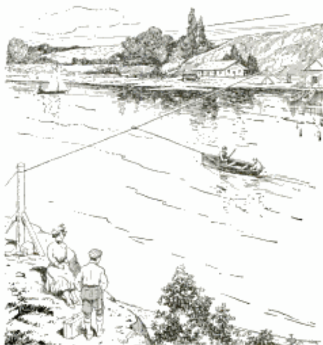
A Novel Method of Using a Rowboat to Ferry Across a Stream
