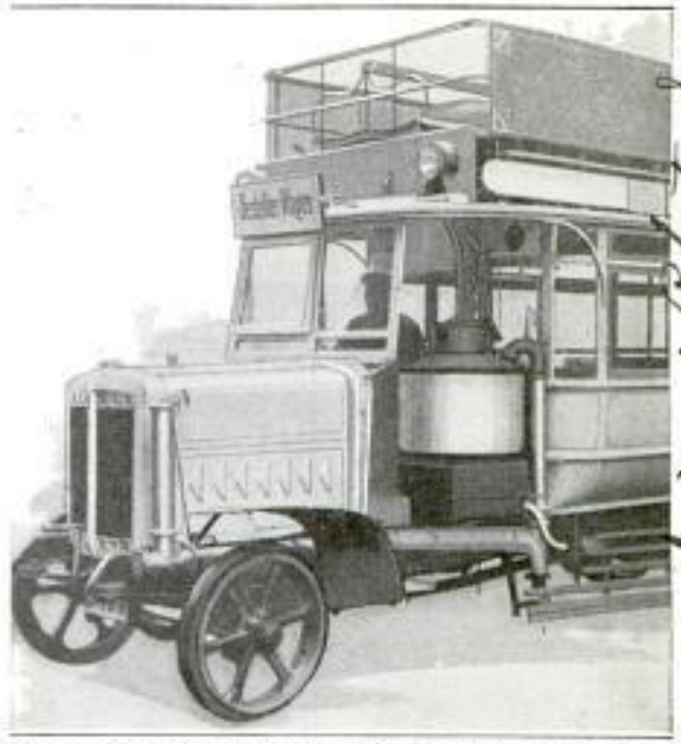
Charcoal Gas Generator that Supplies Power, Is Placed Where Driver Can Tend It
