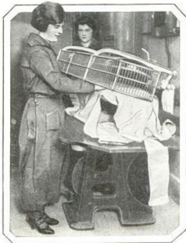
Wire Guard on Pressing Machine that Stops It if Accidentally Touched by the Hand
