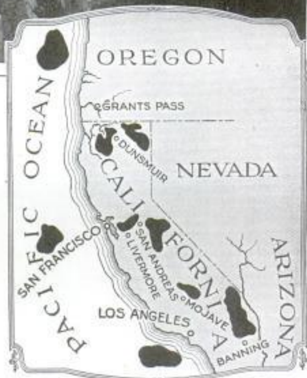
Map Showing Approximate Positions of California's "Dead" Gaps through which Radio Will Not Pass
