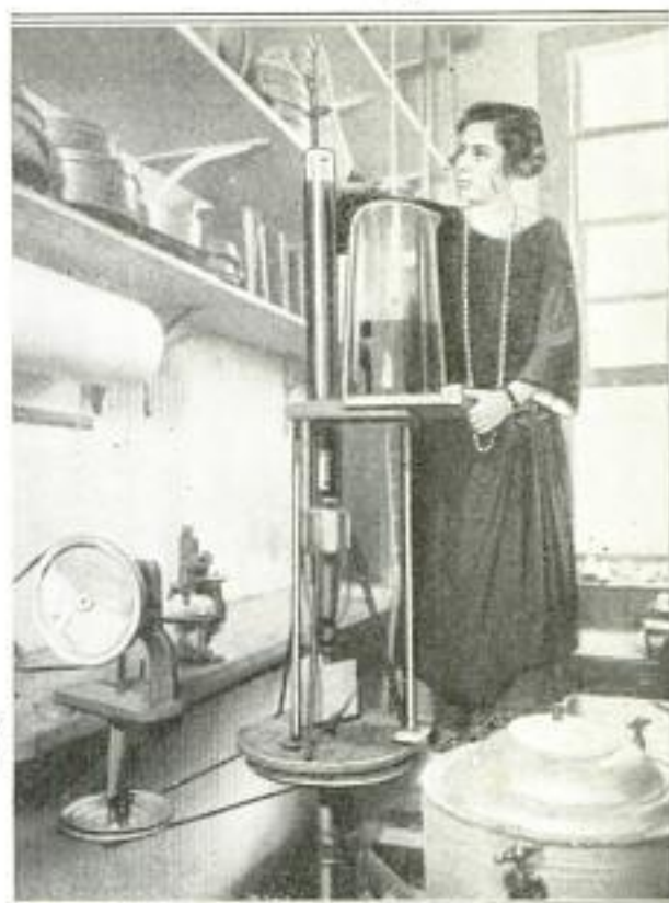
Testing Soil with Machine that "Floats" Bugs and Worms for Study and Numbering
