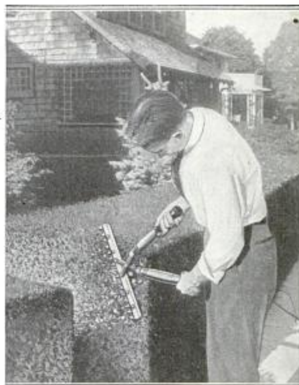
Using Hand Hedge Trimmer that Works Like Toothed Blades of a Mowing Machine
