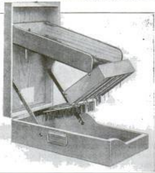
Hopper Sorter Open and Tipped to Working Position; Nails Falling into Wire Slots
