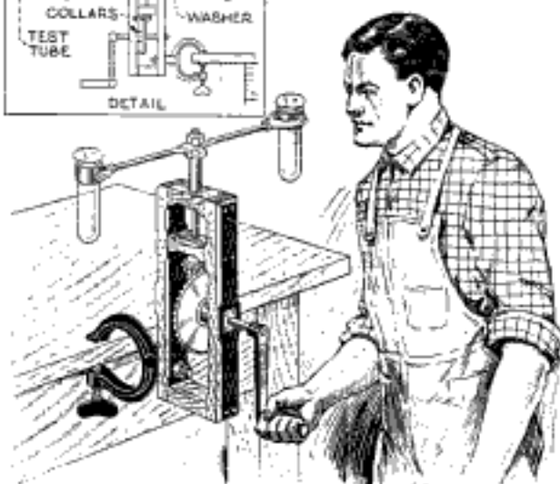
Inexpensive Homemade Centrifuge Made by a Farmer to Determine the Fat Content of Milk
