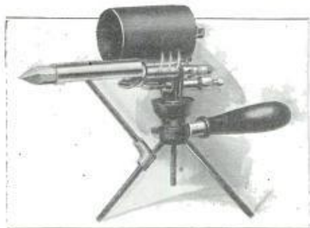
Blowtorch without Pump or Wick that Has a Removable Iron for Soldering
