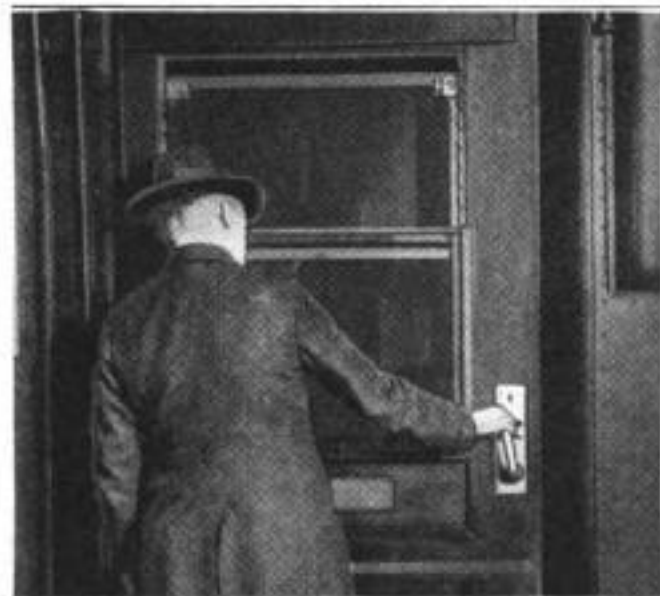
Releasing Door Brakes by Turning Handle to One Side to Permit Easy Entrance
