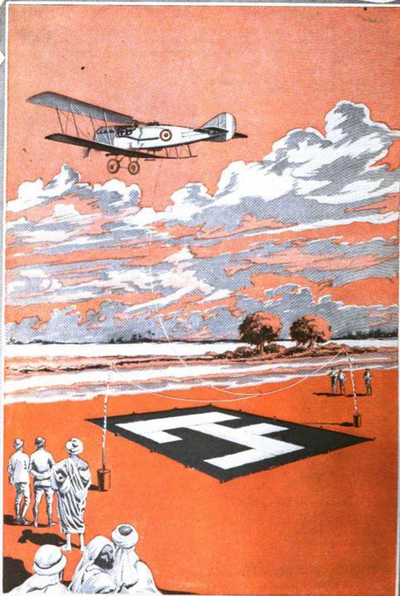
Picking Up Mails During Flight; a British Airplane in Mesopotamia Catching by Means of a Hook a Message Attached to a Line Suspended from Two Poles
