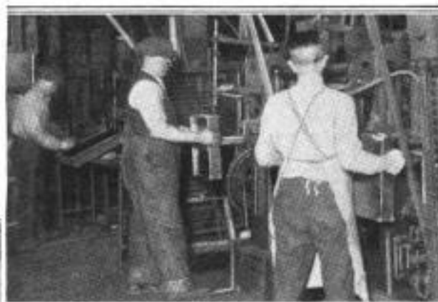
Glimpses Inside a Busy Metal-Furniture Factory Where Power Apparatus of Special Design Has Been Installed to Speed Production; Above: Welding the Projecting Lips of the Corners of Dresser Drawers by Electricity; Left: Power Presses; Right: Adjusting Mirror Posts to a Steel Dresser
