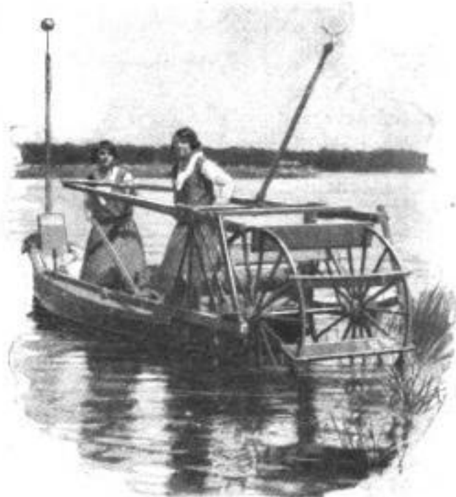
Stern-Wheel Boat that Is Operated by Hand-Car Principle and Is Steered with Feet
