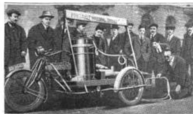
Rapid-Transit Welding Outfit on Motorcycle that Speeds to Relief of Stranded Motorists
