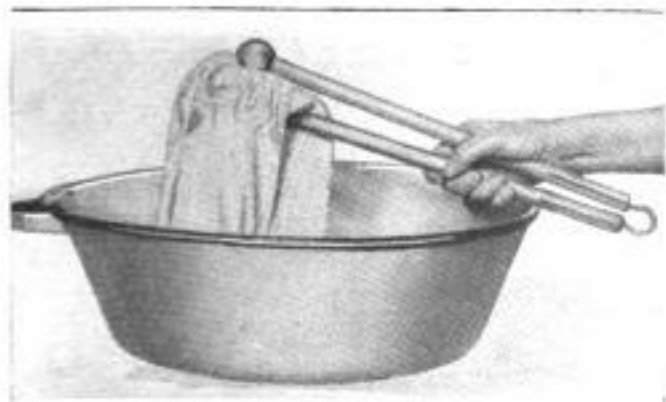
Wooden Tongs for Feeding Clothes into a Wringer without Danger of Injury to Fingers
