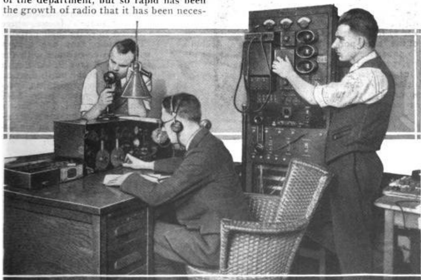
Adjusting Transmitting Amplifier in Station WMAQ under the Direction of Federal Radio Supervisor, Who Makes Four Inspection Calls Each Year at Every Broadcasting Station in His District
