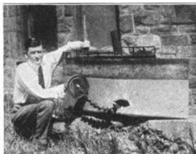
Model of Ship and Rubber Patch Designed to Prevent Sinking of Vessels after Collisions
