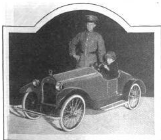
Miniature Automobile Driven by a Storage Battery and Built by Soldier During Spare Time
