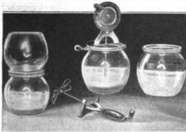
Egg Beater Clamped to Bowl and Extra Jar Tipped on Top as Mixer
