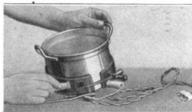
Converting a Sauce Pan into an Electric Cooker with Adjustable Heating Pad
