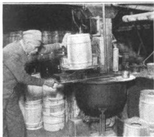
Paraffining Interior of Keg to Make Possible Its Repeated Use as a Food Container
