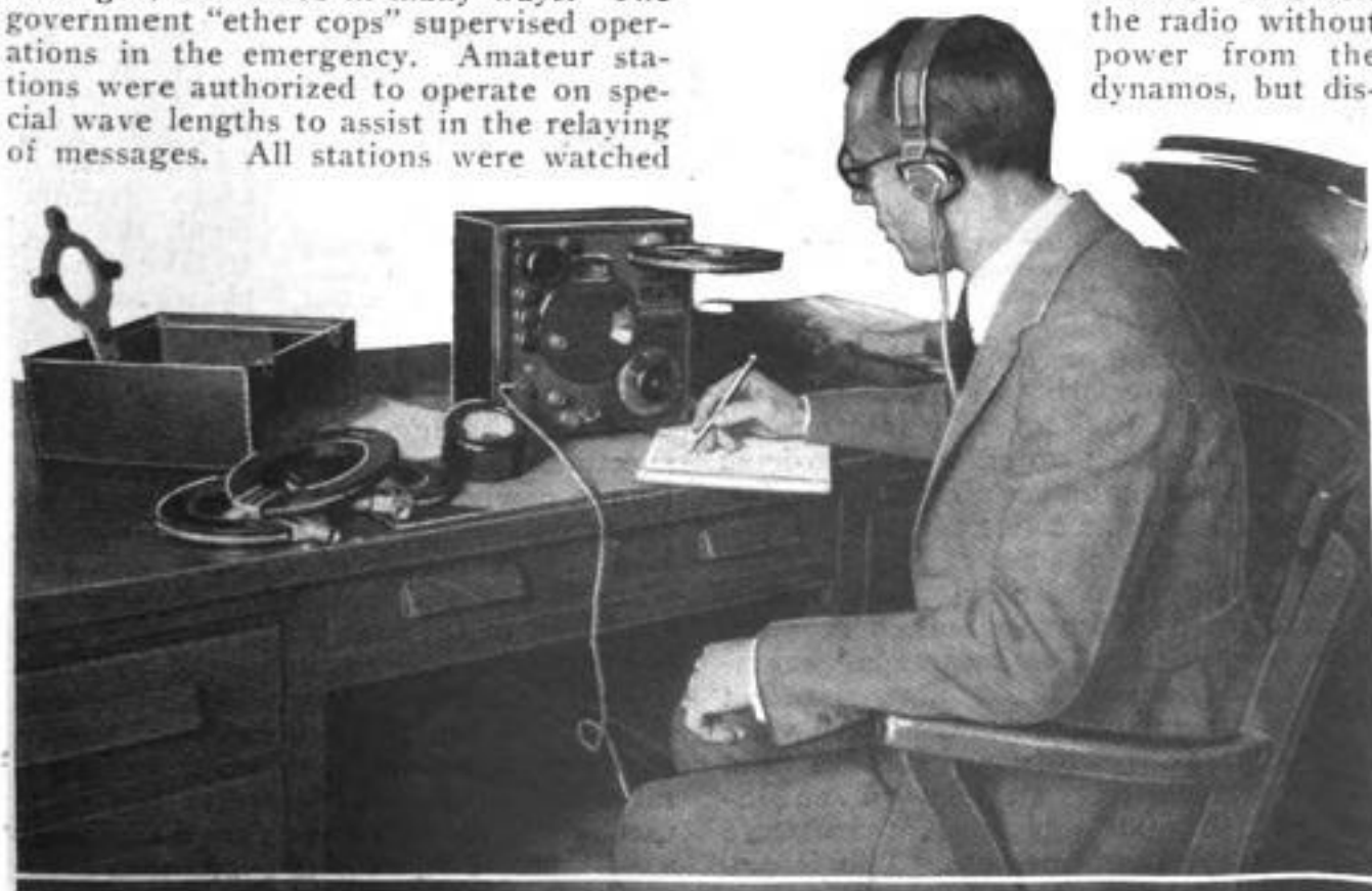
Close View of Decimeter Outside of Case with Exploring Coil Attached and with Others at Left. Connected with Head Phones, Instrument Can Be Used as Receiving Set
