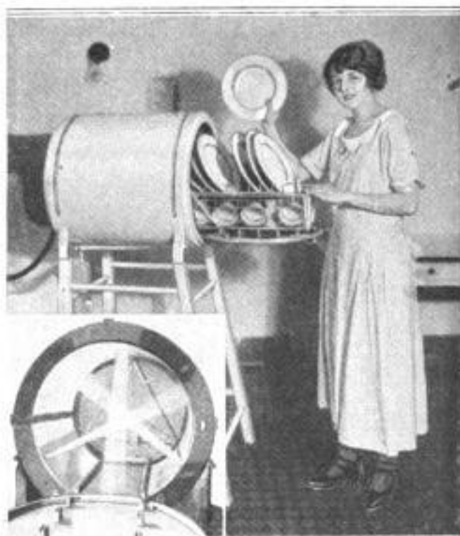
Tray of Dishes Thoroughly Washed in Machine: Inset Illustrates Action of the Water
