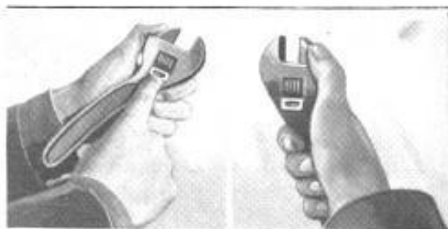
How Grip of Wrench Is Locked by Thumb and Released by Touch of Spring
