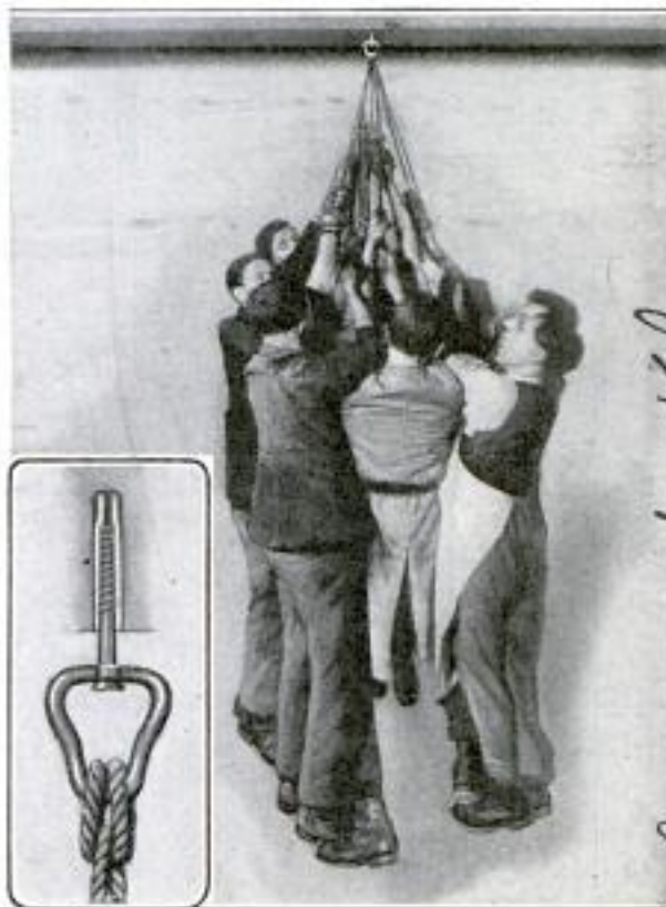
Fiber Plug to Hold Screws in Stone or Iron, and Illustration of Its Strength
