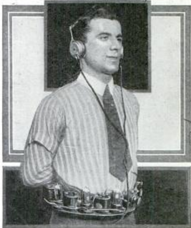
Complete Radio Set Attached to Canvas Belt, Strong Enough to Operate a Loud Speaker.
