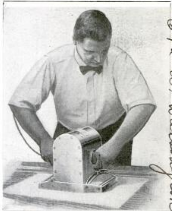
Portable Sander that Also May Be Used on Floors by Attaching It to an Extension Handle
