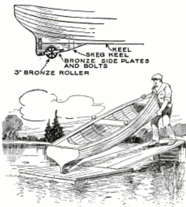
Small Bronze Roller Attached to Skag Keel on Rowboat Enables One Man to Launch It
