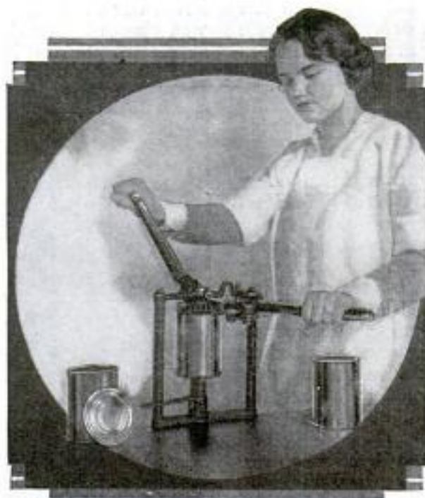
Sealing Cans of Fresh and Uncooked Fruit to Be Preserved by Keeping Them at Low Temperature
