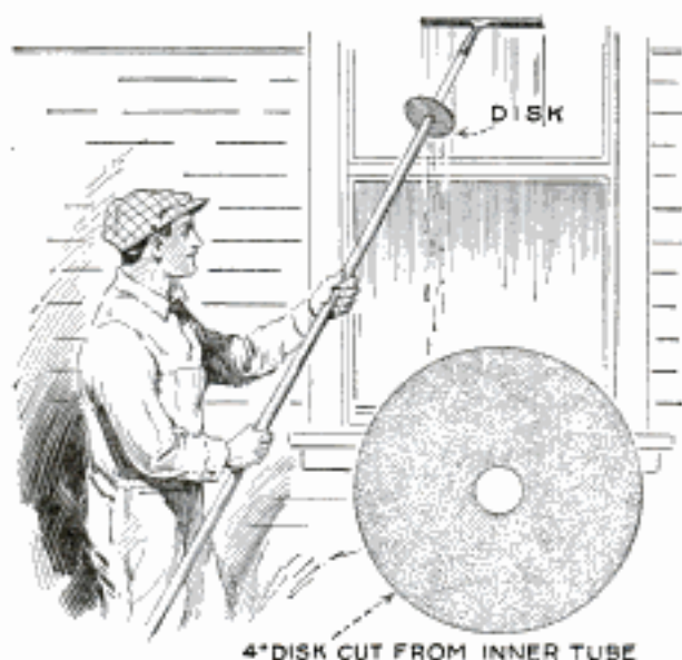
4" DISK CUT FROM INNER TUBE Disk on Handle of Window-Cleaning Squeegee Keeps Worker Dry
