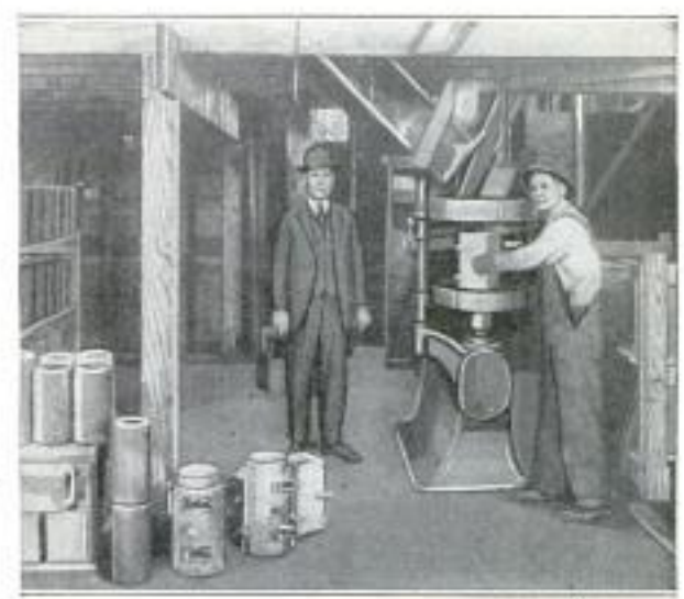
Molding Fireproof Brick and Tile from Sawdust that Has Been Soaked in Chemical Solutions
