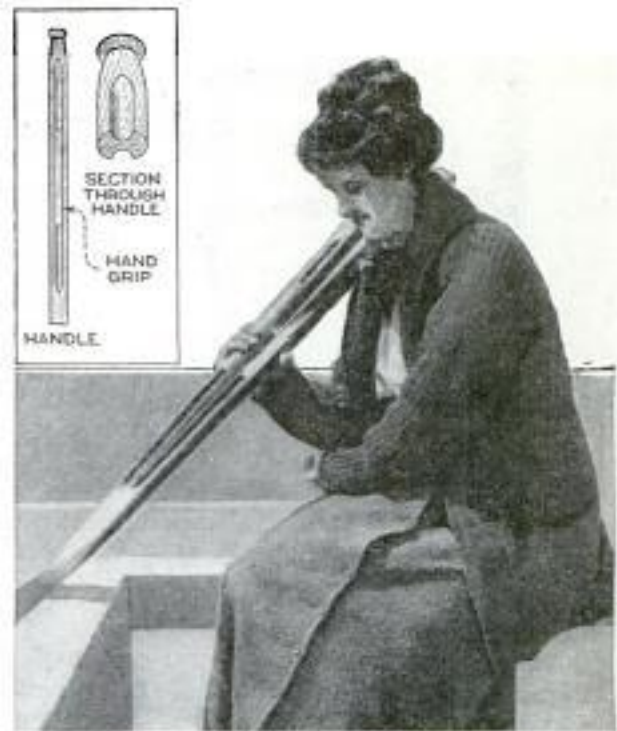
Grooving the Handles of Canoe Paddles Reduces Their Weight without Sacrificing Any Strength
