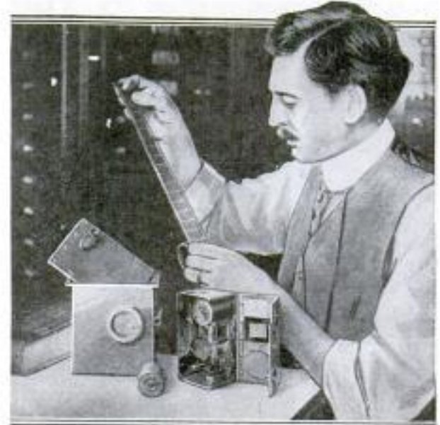
Examining a Length of Film: Camera Open and Shown without Its Water-Tight Submarine Case
