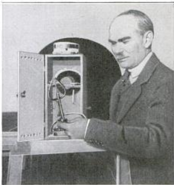
Microphone that Converts Electrical Impulses into Sound Waves without a Diaphragm
