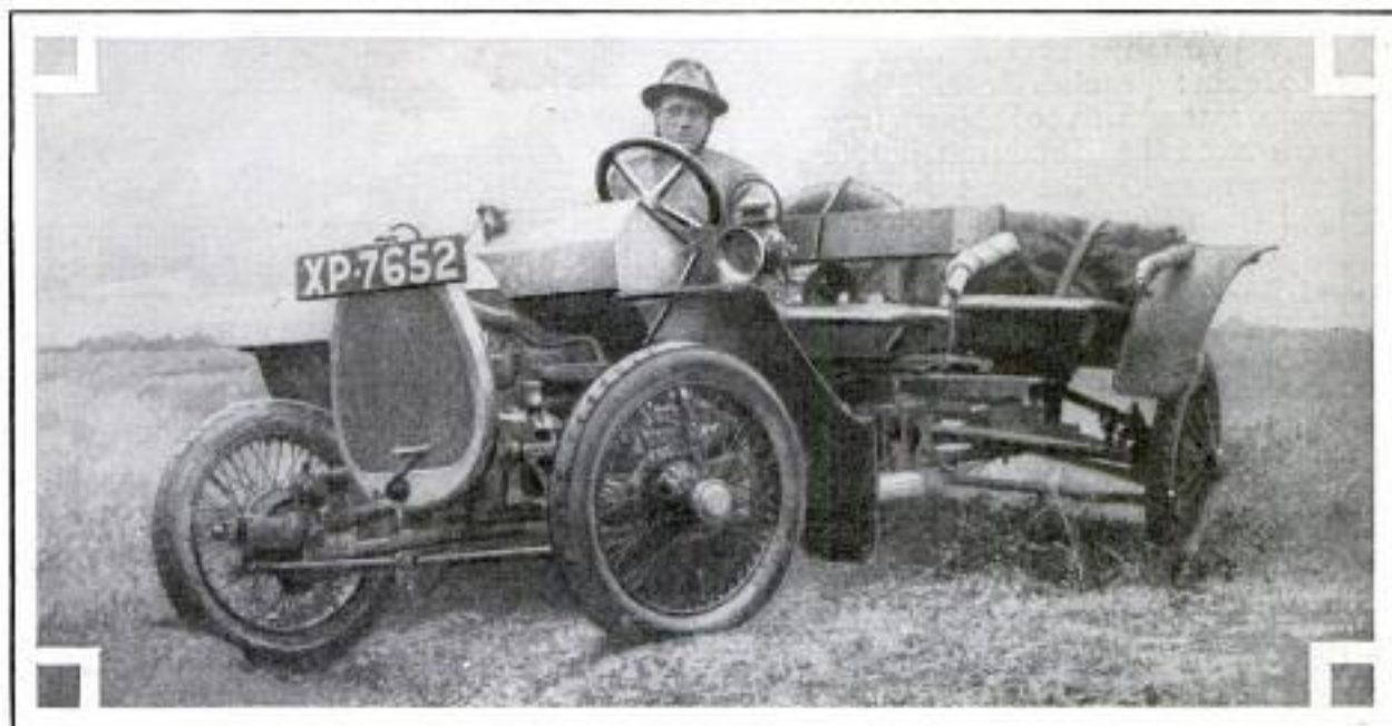
Copyright, Underwood & Underwood Automobile that Drives, Brakes and Steers from All Four Wheels and Is Able to Turn About in Its Own Length and Travel Sideways Like a Crab
