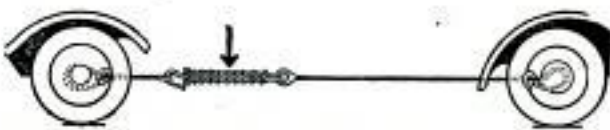
Tow Line with Spring Section that Acts as Shock Absorber When Attached to Cars
