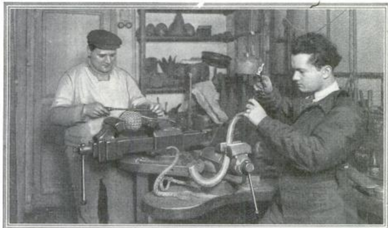
Filing and Chiseling the Finishing Touches on Ornamental Pieces for Hammered Bowls and Vases
