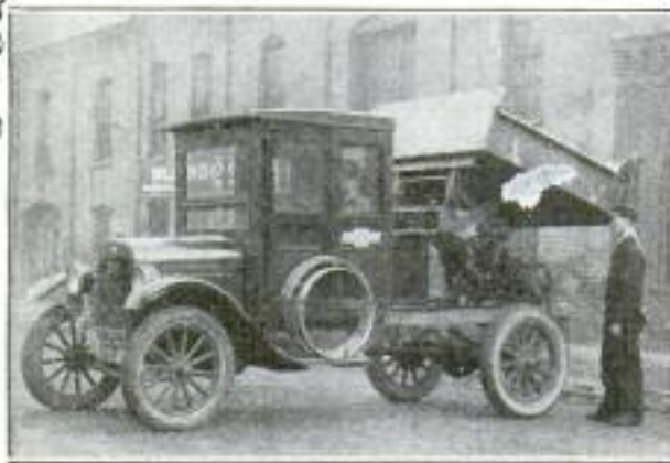
Hand-Elevated Dump Hopper for Automobile Trucks that Deposits Loads on Raised Platforms
