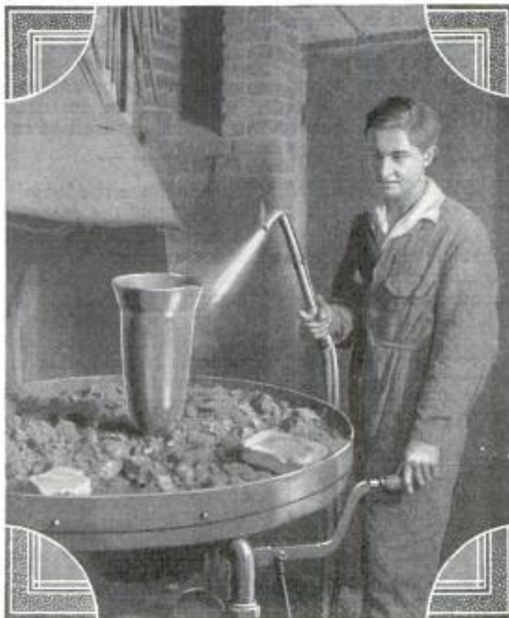
Heating the Metal with Torch Flame to Soften It
