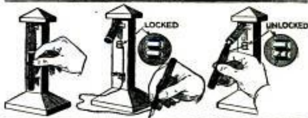
Fountain Pen and Attractive Holder to Replace Ink-wells in Public Writing Places
