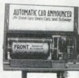
Street-Car Announcer that Shows Approaching Intersections and Principal Buildings by Pushing Button
