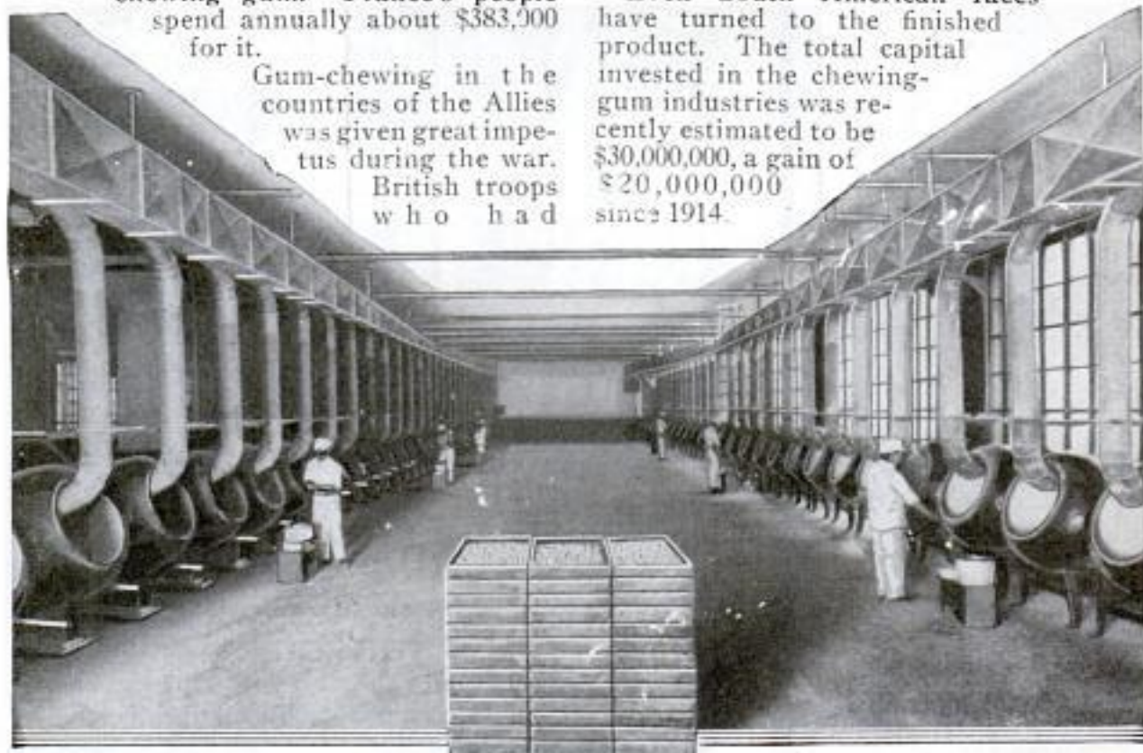
Battery of Immense, Revolving Coating Vats which Add a Sweet, Flavored Covering to Tiny Balls of Chicle. After Dipping, They Are Placed on Trays to Cool and Harden
