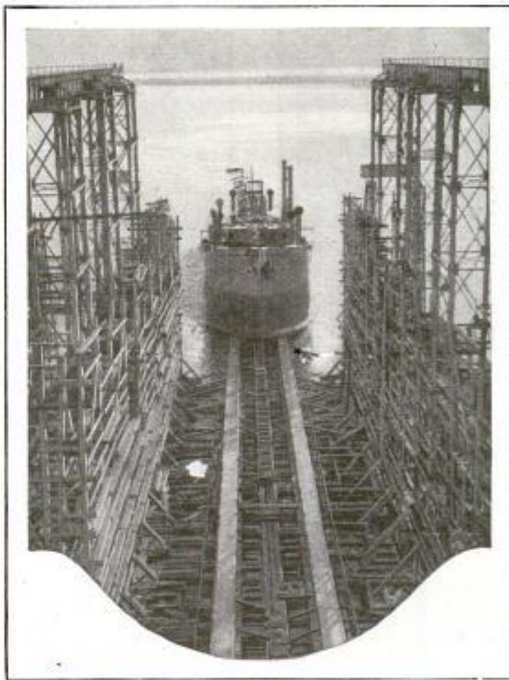
An Electrically Operated Ship, a Seagoing Dredge for Harbor Service Being Launched by United States Army
