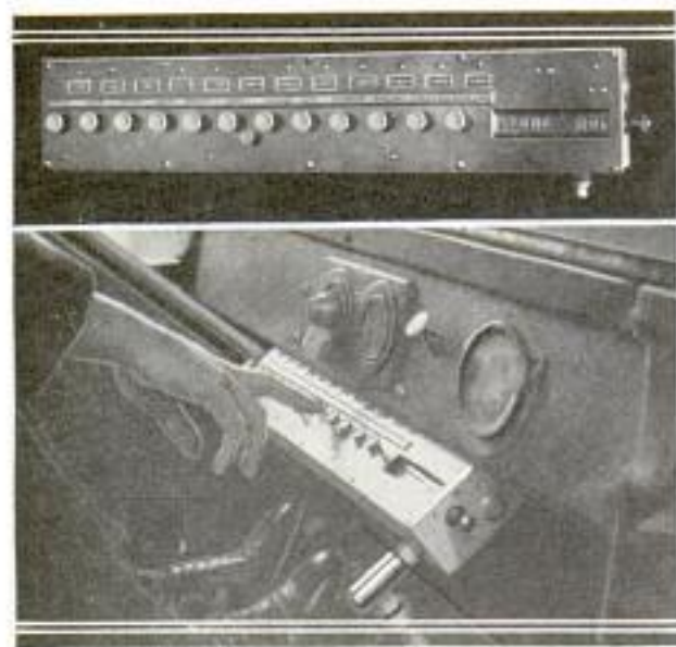
Meter for Dashboard of Automobile that Automatically Measures Fields Planted in Various Crops
