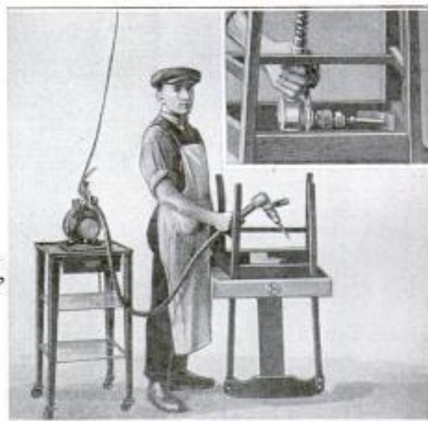
Motor-Operated Screwdriver and Nut Setter that Does Fast Work in Difficult Positions
