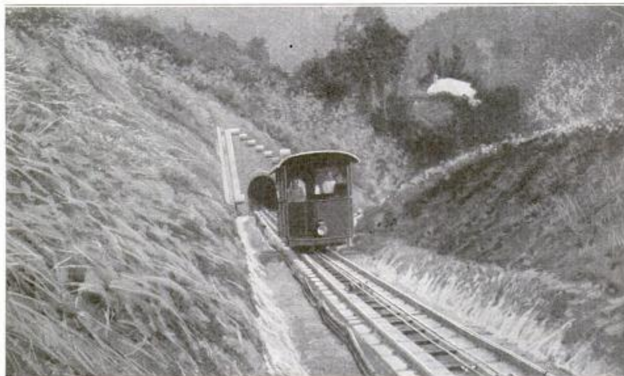
Climbing Out of a Steep Tunnel, this Step-Seated Car Ascends the Mountain Side Pulled by a Cable Winding on Drum at the Summit of the Grade
