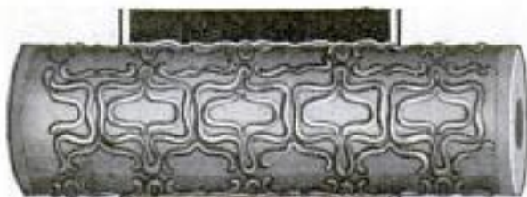
Wood Rolls upon which Patterns Are Outlined in Strips of Sheet Brass Hammered Firmly into Place by Skilled Craftsmen, the Spaces Being Filled with Prepared Felt
