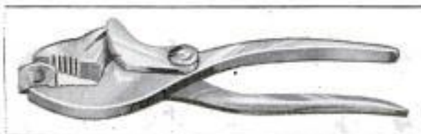
Ratchet Pliers that Automatically Lock Their Jaws after They Have Secured a Hold
