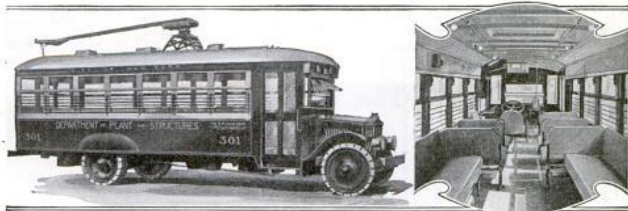
Left, Trackless Trolley Bus that Has a Leeway of 15 Feet on Each Side of the Feed Wire; Right, Interior of Coach Showing Driver's Cab
