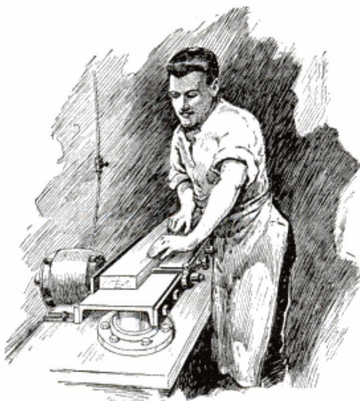
Simple and Easily Built Jointer for the Small Woodworking or Pattern Shop
