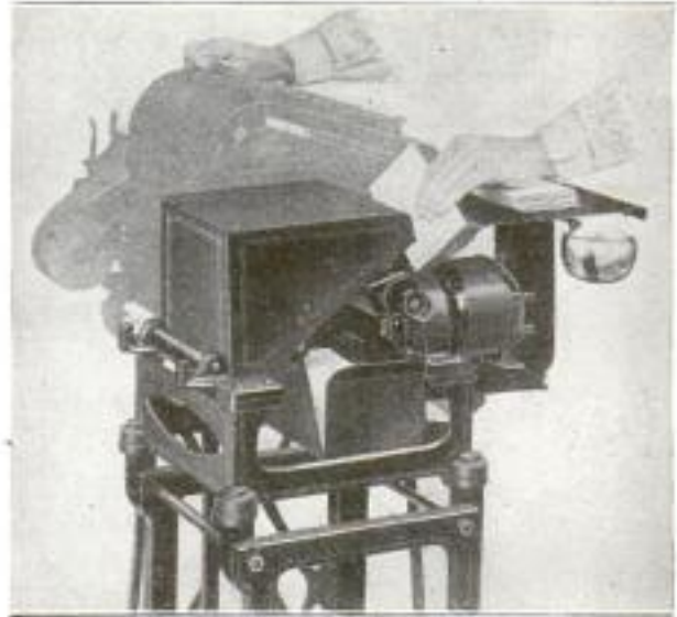
Endorsing Machine and Lister in Background Used as a Unit in Handling Checks
