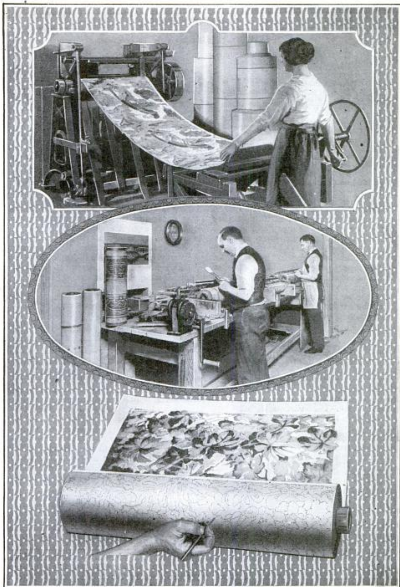
Wallpaper Coming through Embossing Rolls (at Top); Transferring Artist's Designs to Printing Rolls (Bottom), and Hammering Strips of Brass into Maple Cylinders (in Center)
