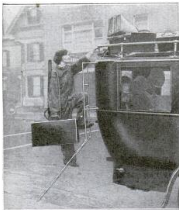
Folding Ladder on Auto Bus that Permits Easy Loading of Luggage on Roof of Car
