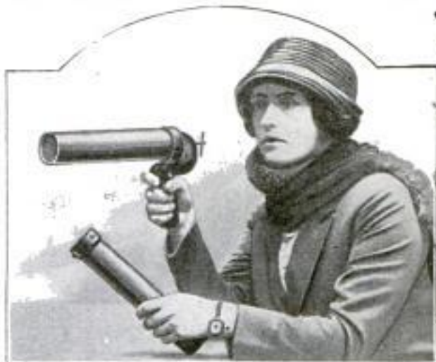
Effective Fire Extinguisher that Works like Pistol to Shoot Stream into Flames
