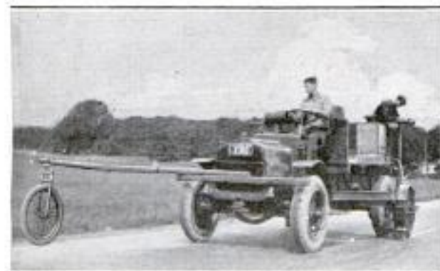
Traffic Marker, Made from Condemned War Materials, Used to Help Prevent Accidents in Minnesota
