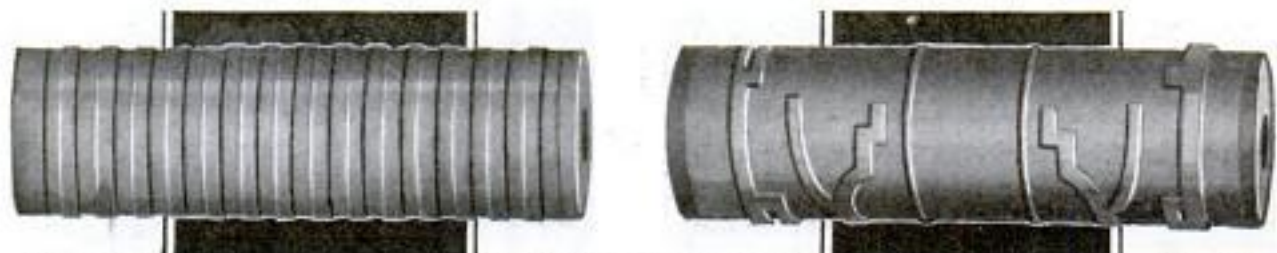
When Placed in the Printing Machine, the Maple Rolls, Similar to Those Shown Above, Are Supplied with Ink by Means of a Short Felt Band
