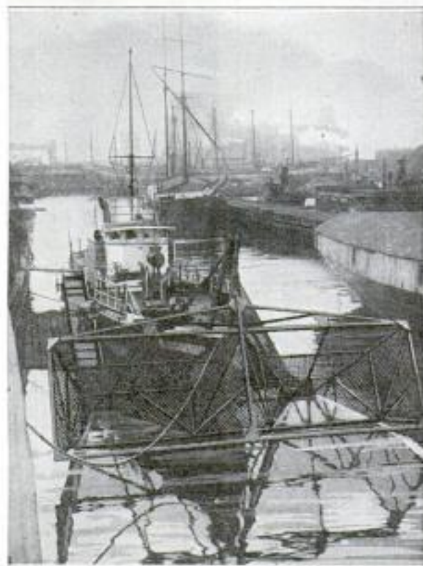
Copyright, Underwood & Underwood Scoop Net on Steel Frame and Belt Conveyors Attached to a Fishing Steamer
