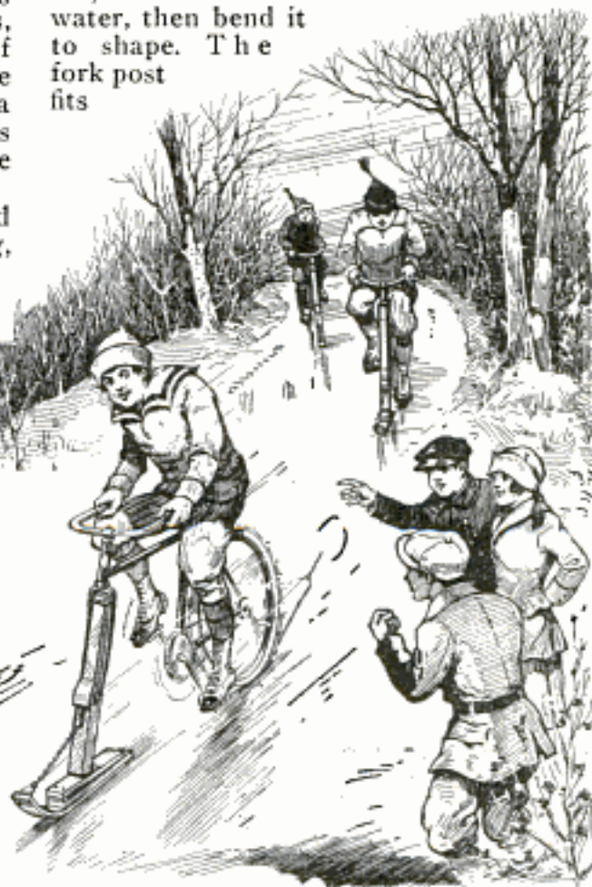
A Simple Tread and Steering Runner for the Bicycle that Will Enable It to Be Used in Winter as Safely as in Summer, and that Lessens the Hard Work of Pedaling in the Snow
