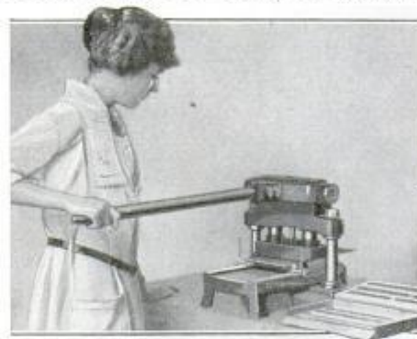
Hand Embossing Press that Prints Letters in Colored Paper and Needs no Expert Operator
