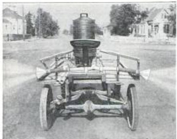
This Sprayer Dusts the Vines with Wet or Dry Sulphur to Prevent Mildew
