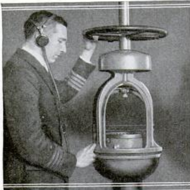
Radio Compass on "Leviathan" that Gives Position in Fogs and Diminishes Collision Risks
