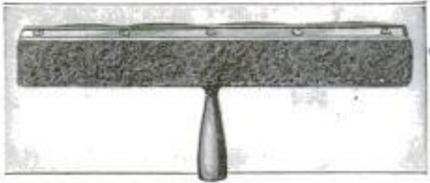
Squeegee with Absorbent Felt Pad Containing Chemical that Loosens Dirt on Window Panes
