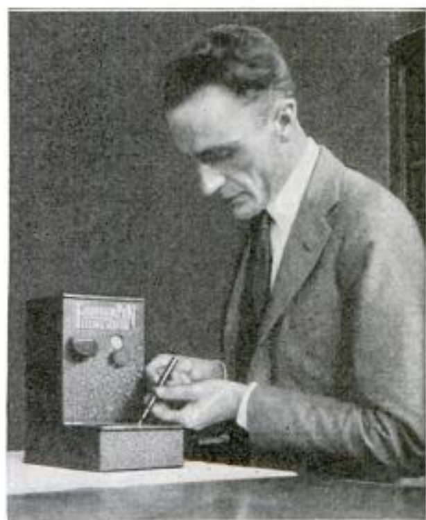
Loading a Fountain Pen with Ink from a Penny-in-the-Slot "Filling Station"
