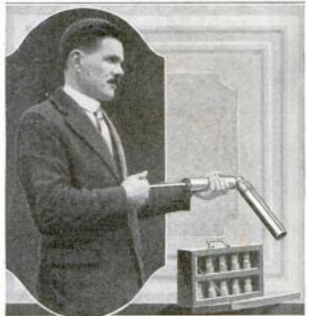
Instrument Used by the Government to Determine Number of Grains of Dust in the Air
