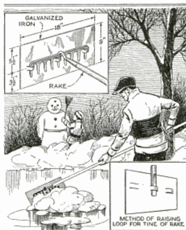
Serviceable Snow Scraper Made from a Piece of Galvanized Iron Attached to the Teeth of a Rake
