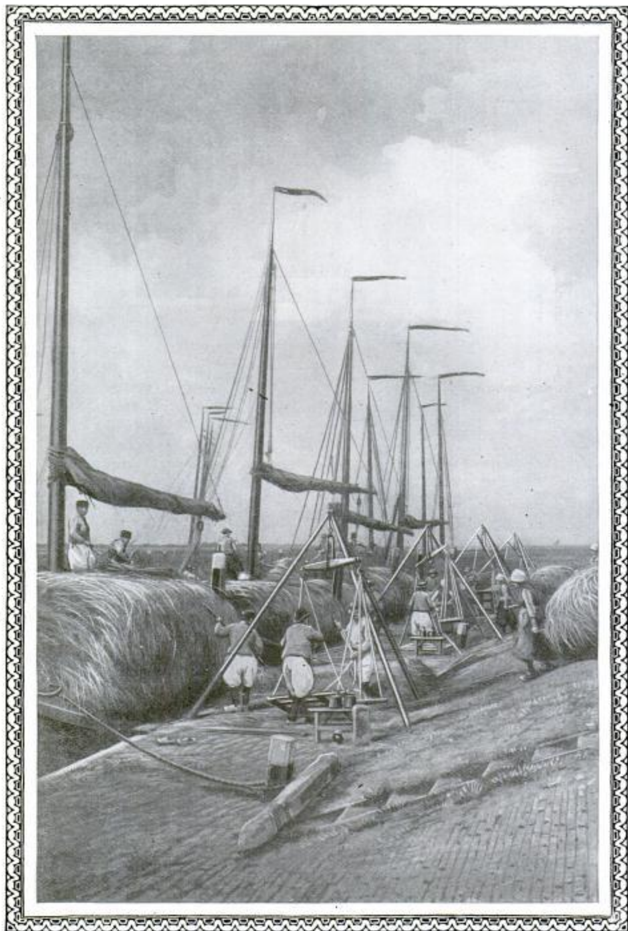
Copyright, Ewing Galloway Curious Scales, Set upon Long Tripods, that Are Used for Weighing Hay for Shipment by Boat Along One of the Many Canals that Lower Transportation Costs in Holland
