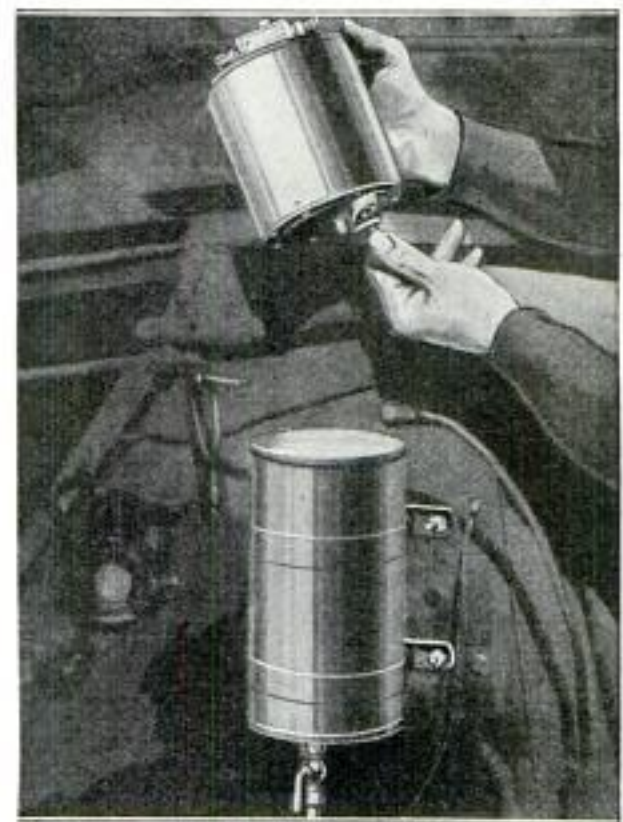
Vacuum Tank that Is Operated Directly from the Oil Pump Instead of the Intake Manifold
