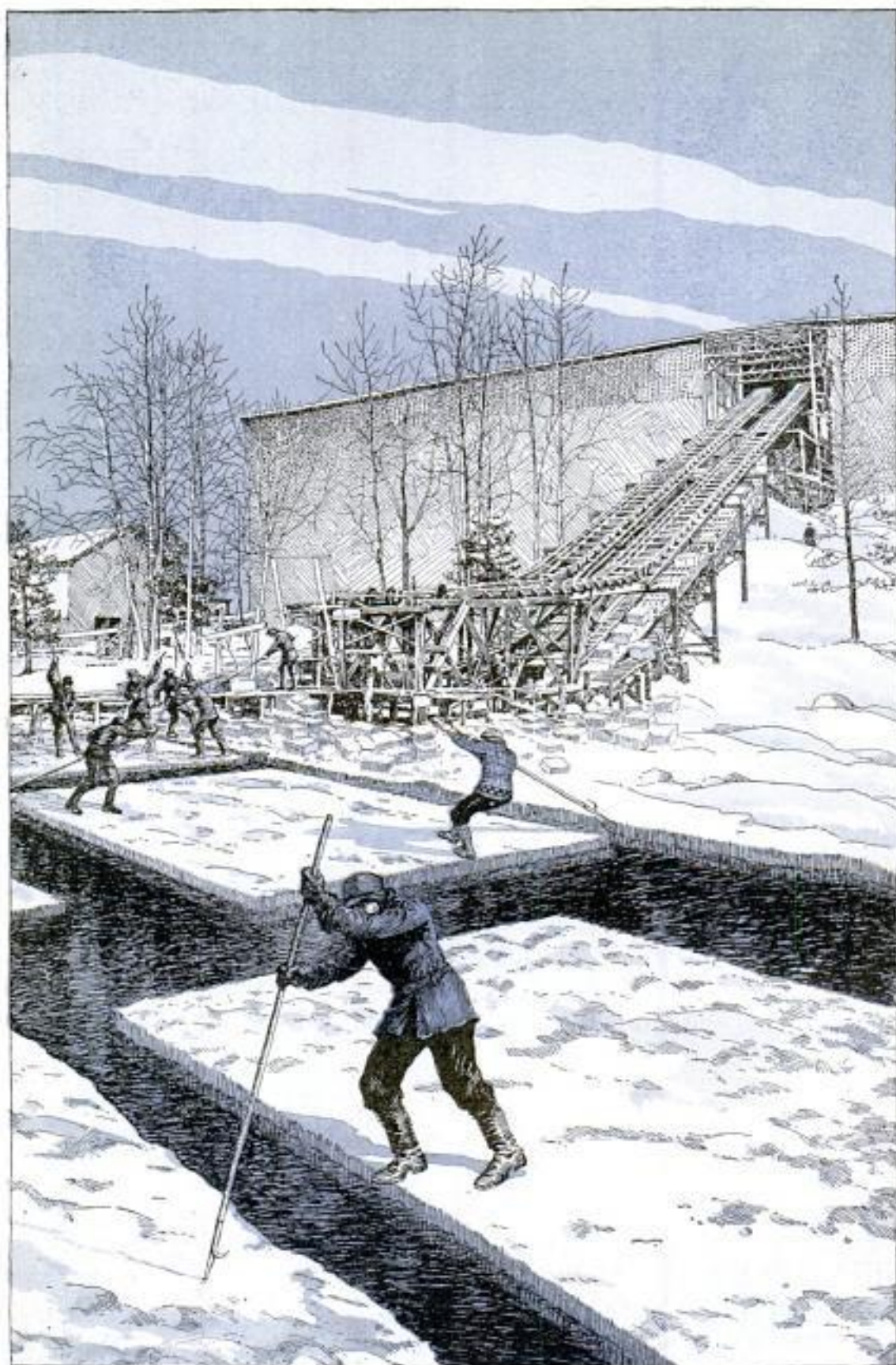
Armed with Sharp Pike Poles, Skilled Workers Guide the "Floats" Like Massive Logs to the Elevator Hoist where They Are Cut into Storage Blocks
