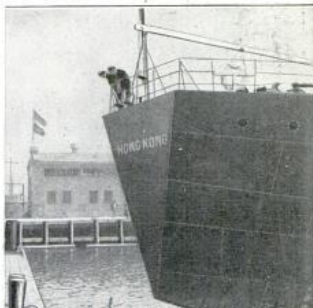
Triangular-Shaped Stern of Steamer that Is Favored by Superstitious Oriental Sailors
