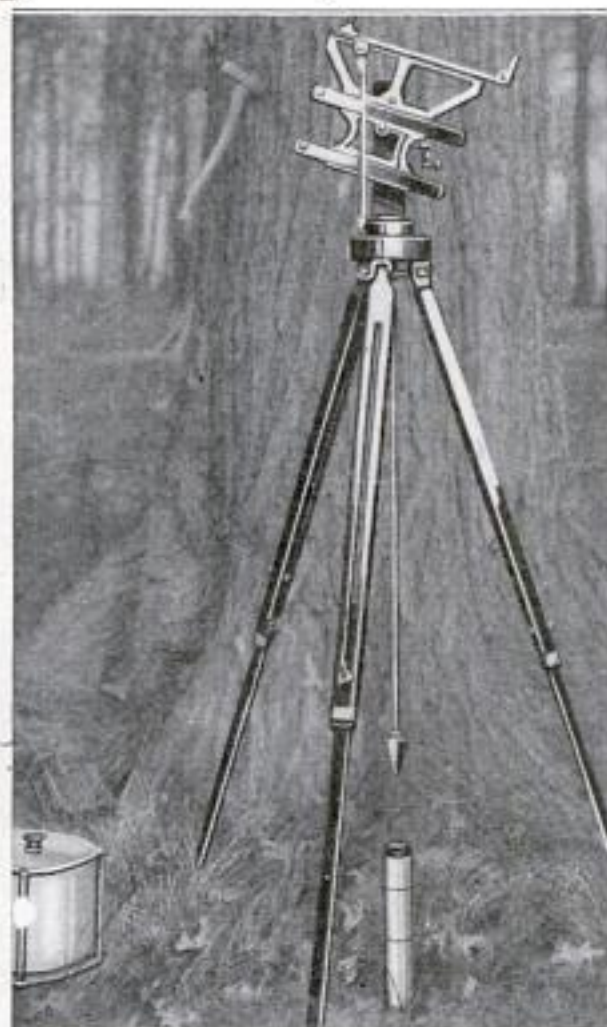
Accurate Tripod Scale for Measuring Board Feet of Lumber Before the Tree Is Felled
