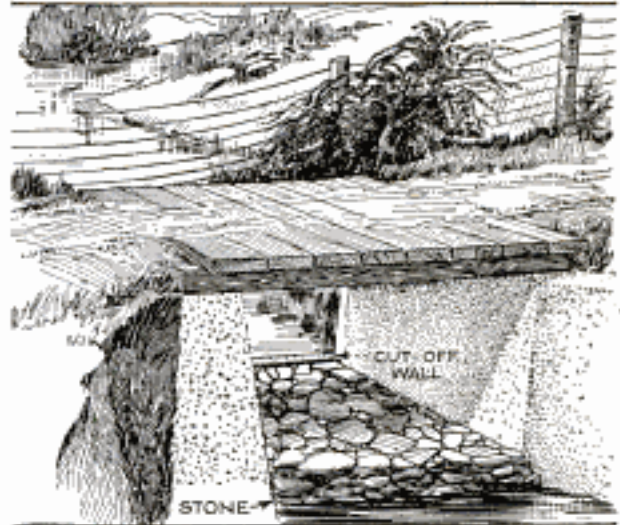
A Concrete-Covered Stone Floor on a Stream Bed to Prevent Scouring of Bridge Abutments
