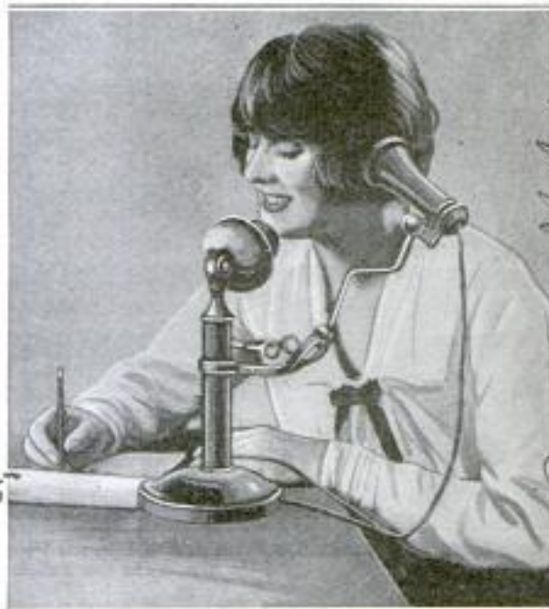
Holder for Telephone Receiver that Permits Free Use of Both Hands while Talking
