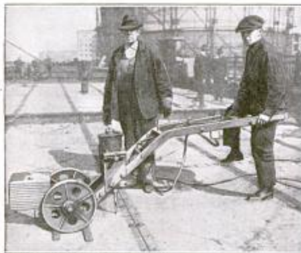
Copyright, Underwood & Underwood Electric Drill on Wheels that Is Easily Moved and which Two Men Can Operate
