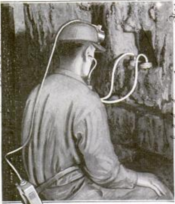
Listening with an Instrument that Can Locate Underground Sounds Half a Mile Away
