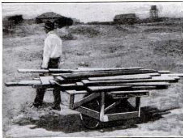
A Wheelbarrow Equipped with a Drum Instead of a Wheel Is Convenient to Handle on Soft Ground
