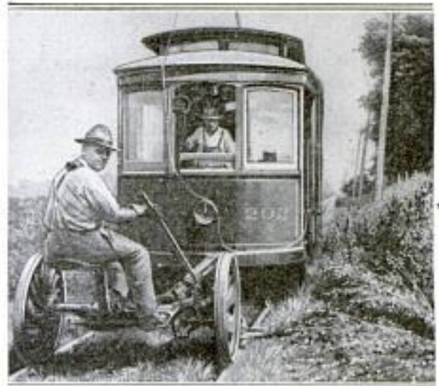
Mower, Pulled over Rails by Trolley Car, Cuts Weeds Growing along Right of Way
