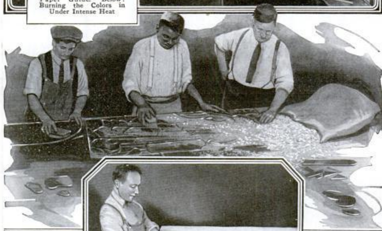
Above: Applying Cement Dressing for Waterproofing Window
