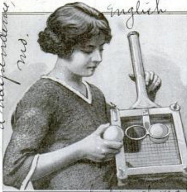
Spring Clip Attached to Racquet Press, Holding Tennis Balls Firmly without Cutting Them
