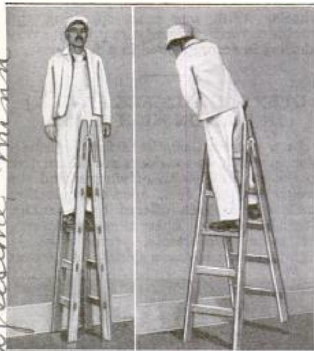
Stepladder So Designed as to Permit User to Move It About as Though on Stilts
