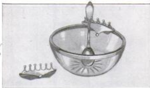
Metal Holder Placed on Edge of Serving Dish to Keep Spoons from Slipping into Food
