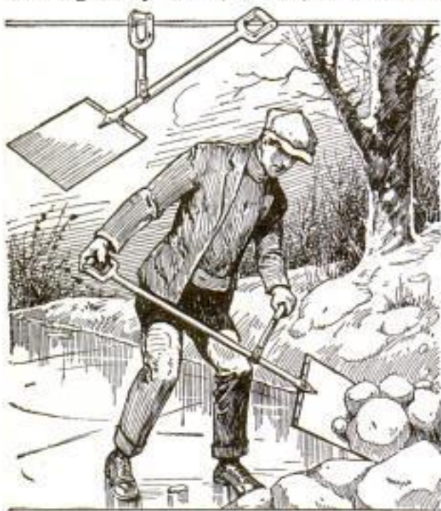
An Auxiliary Handle on a Shovel Used for Clearing Away Snow, Is of Considerable Assistance
