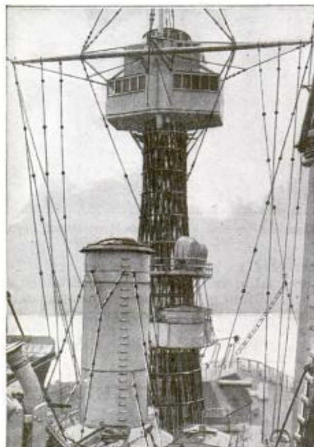
Ropes and Lines on Warship Studded with Insulator Knobs Resembling Strings of Beads
