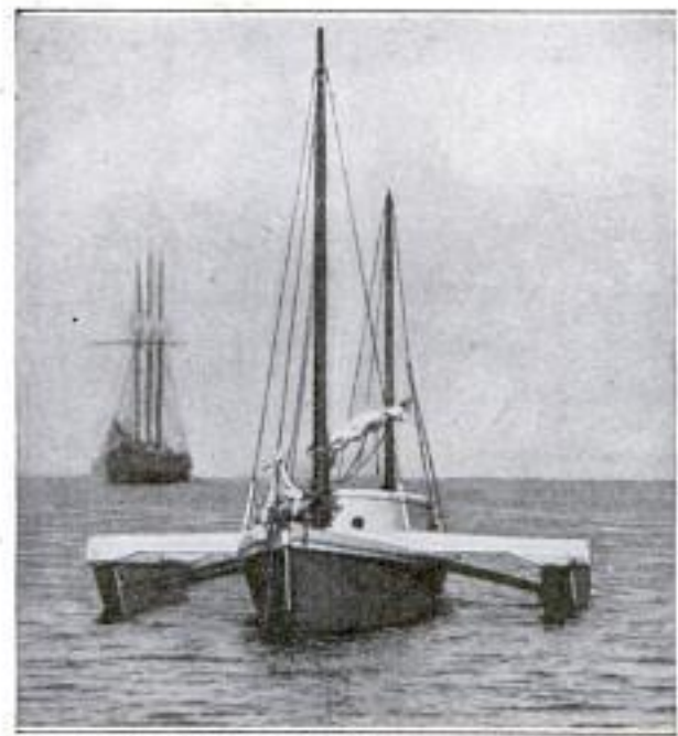
Pleasure Boat Fitted with Pontoons to Keep It from Rocking in Heavy Seas
