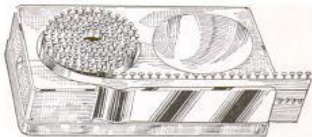
Holder that Keeps Pins in a Paper Roll from which They Can Be Easily Picked
