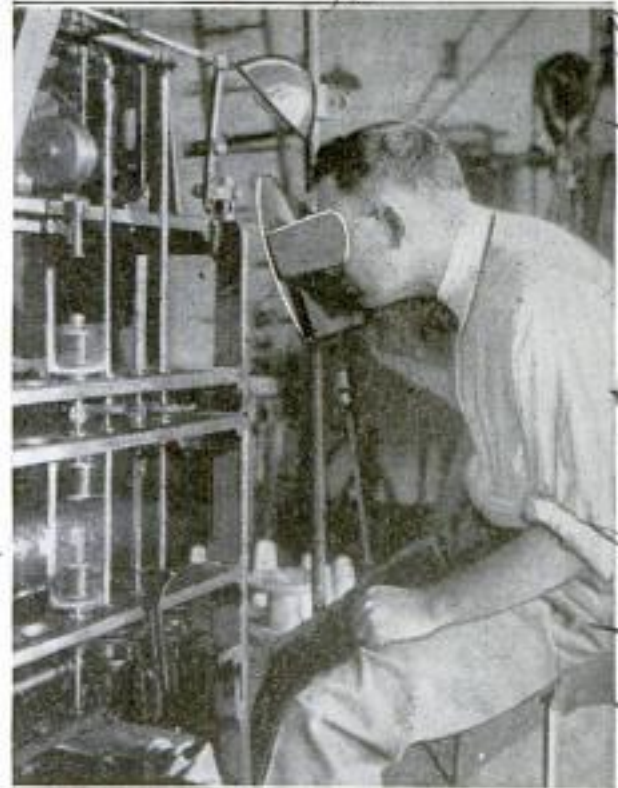
Observing Working Machinery through Instrument that Reduces High Speed to Slow Motion for Eye
