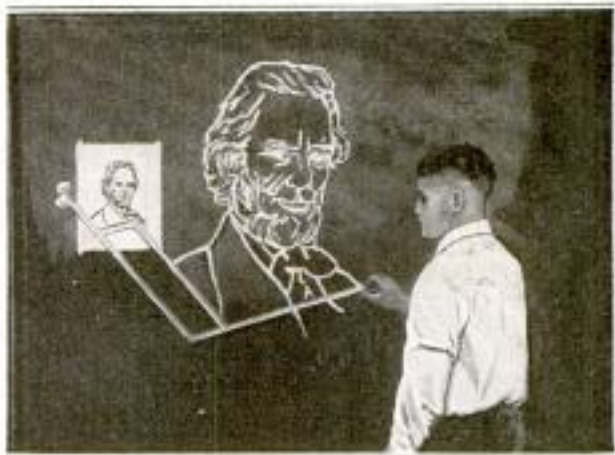
Form of Pantograph that Can Be Operated by Anyone for Enlarging Drawings on Walls
