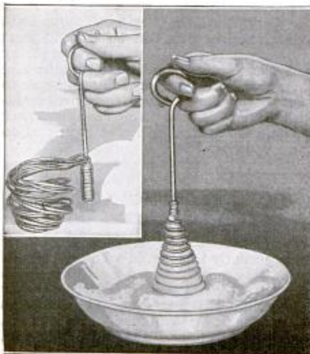
Coiled-Wire Egg Beater that Works by Strokes that Compress Spring Base
