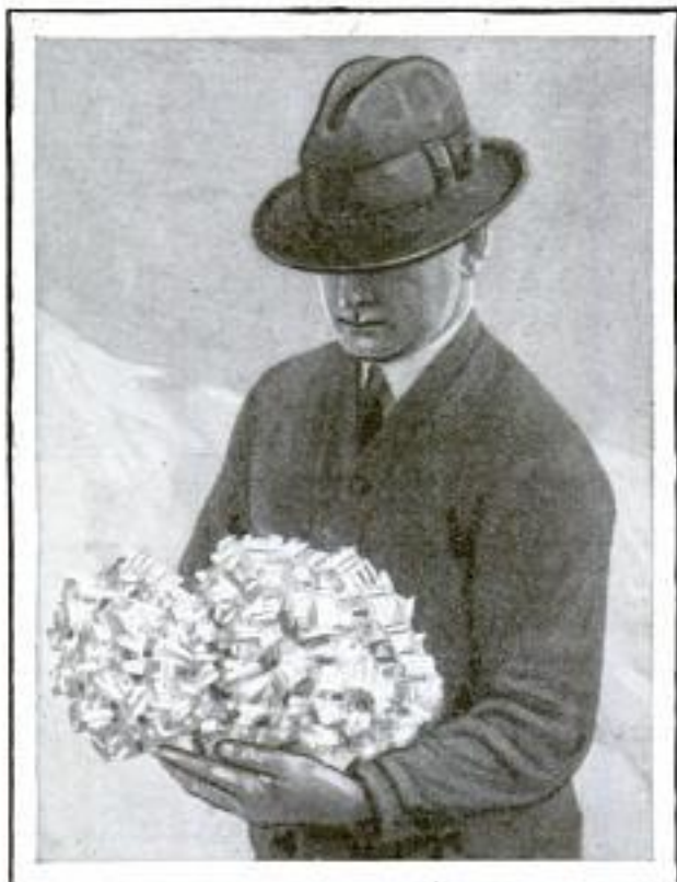
Lump of Rock-Salt Crystals Taken from Vats After Moisture Has Passed off
