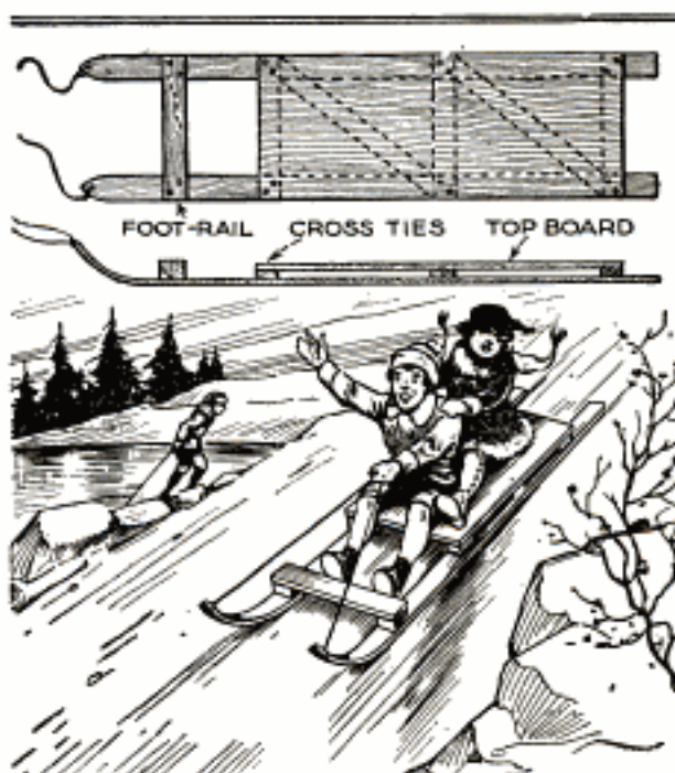
A Sled Made from a Pair of Skis Is Much Safer than the Ordinary Kind on Crusted Snow
