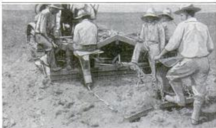
Rear View of Cane-Planting Machine, Showing Seed in Furrows, and Breaker Plow
