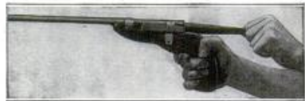
A Novel Pistol for Shooting Arrows That Will Shoot Nearly 1,000 Feet with Considerable Accuracy
