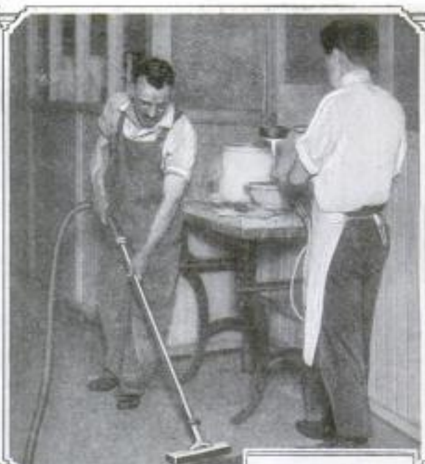
Floors of Factories Working in Valuable Metals Are Cleaned Daily by Powerful Vacuum Devices that Convey the Sweepings to Storage Tanks for Safe Keeping
