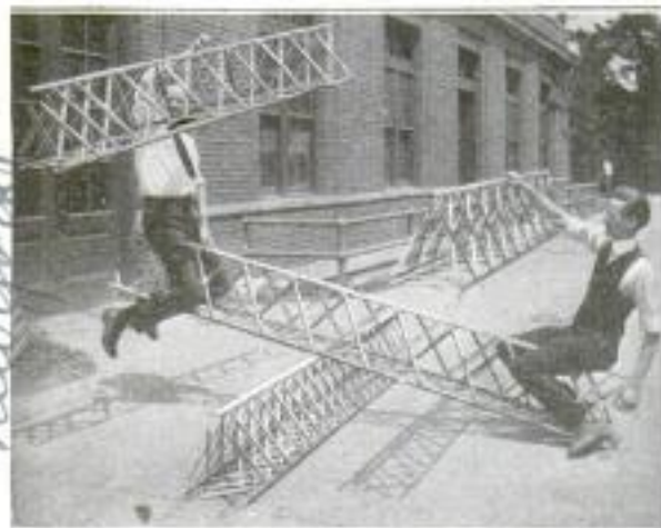
Test Showing Strength of Metal Used in Building Girders for Giant Airships
