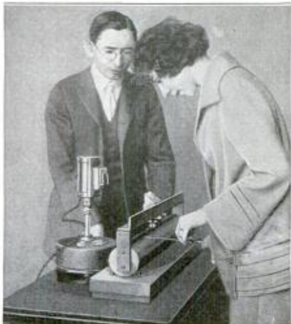
Copyright, Underwood & Underwood Proving that Weight of a Pencil Would Bend Steel Over Three Inches Thick
