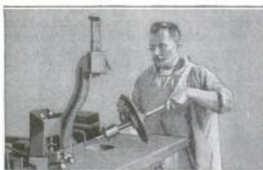
Placing Steel Cutting Disk in Machine
