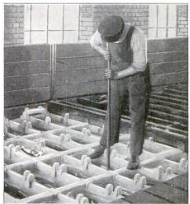
Breaking Cakes of Ice Loose from Containers Immersed in the Brine Pool
