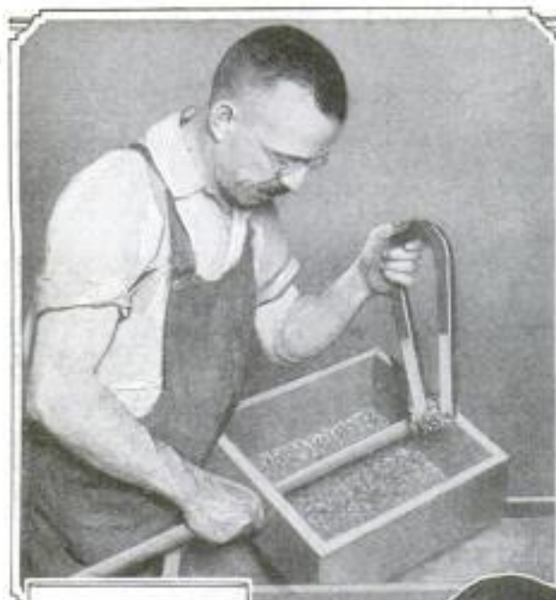
Magnets Have Proved Efficient for Removing Iron and Steel Filings that Become Mixed with the Fine Particles of Valuable Metals Gathered About Jewelry Plants
