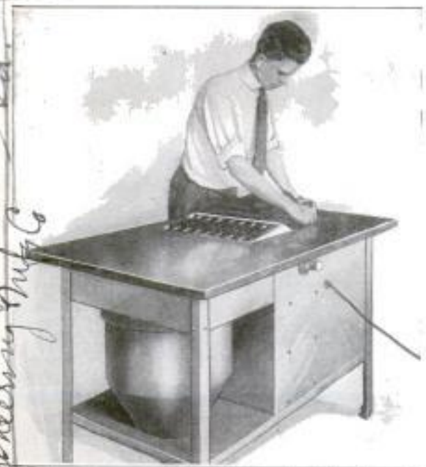
Clothing Renovator That Draws the Dirt from the Fabrics with Revolving Brushes and Vacuum
