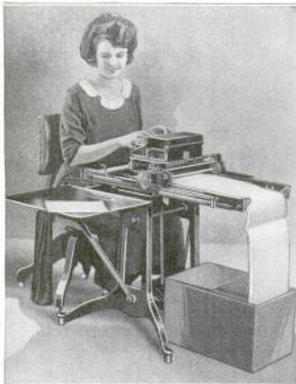
Machine on Which Person Can Write 1,000 Pages without Inserting a New Sheet
