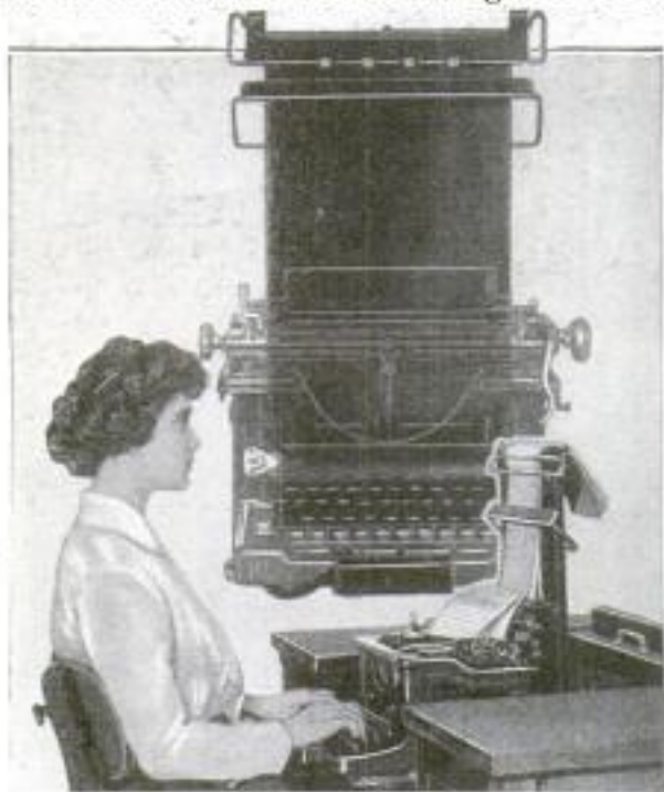
The Line Guide and Copyholder that is Operated by Electricity to Increase Typist's Speed
