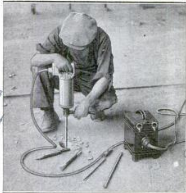
Electric Hammer with Single Movable Part That Takes Less Current than Flatiron
