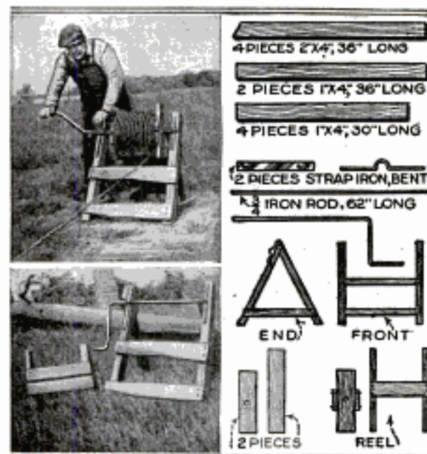
A Simple Homemade Barbed-Wire Winder Made from Material Available on Every Farm
