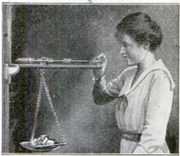
Folding Household Scales for Either Small or Large Packages Prevent Short Weights
