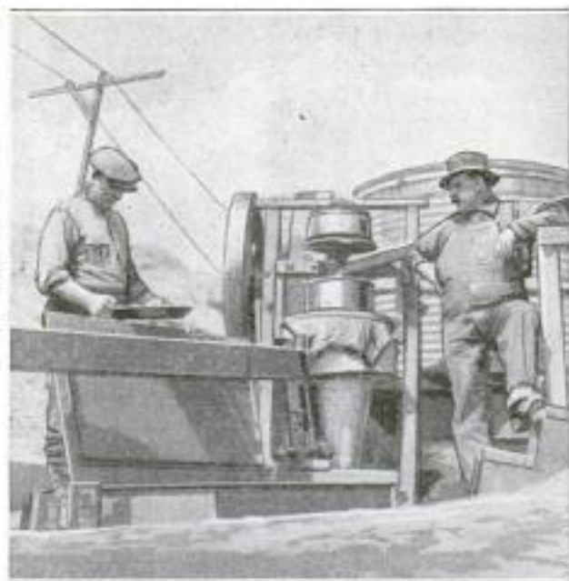
Rotary Washing Mill for Extracting Gold from Metal Bearing Rock without Requiring Outside Labor
