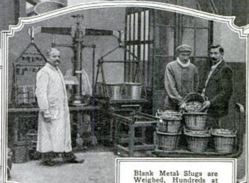
Accurate Glass - Inclosed Devices Equip the Rooms Where Coins are Weighed on Delicate, Automatic Scales as Rapidly as Men can Feed the Pieces into Electrically Operated Machines. When Rejected, They are Placed in Stacks Labeled "Lights" and "Heavies"
