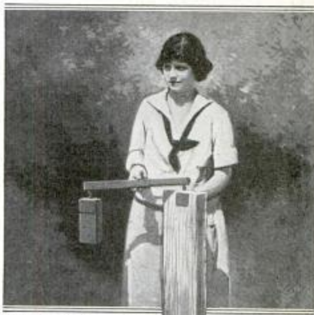
Balsa-Wood Log Balanced by a Piece of Other Timber One-Tenth Its Size
