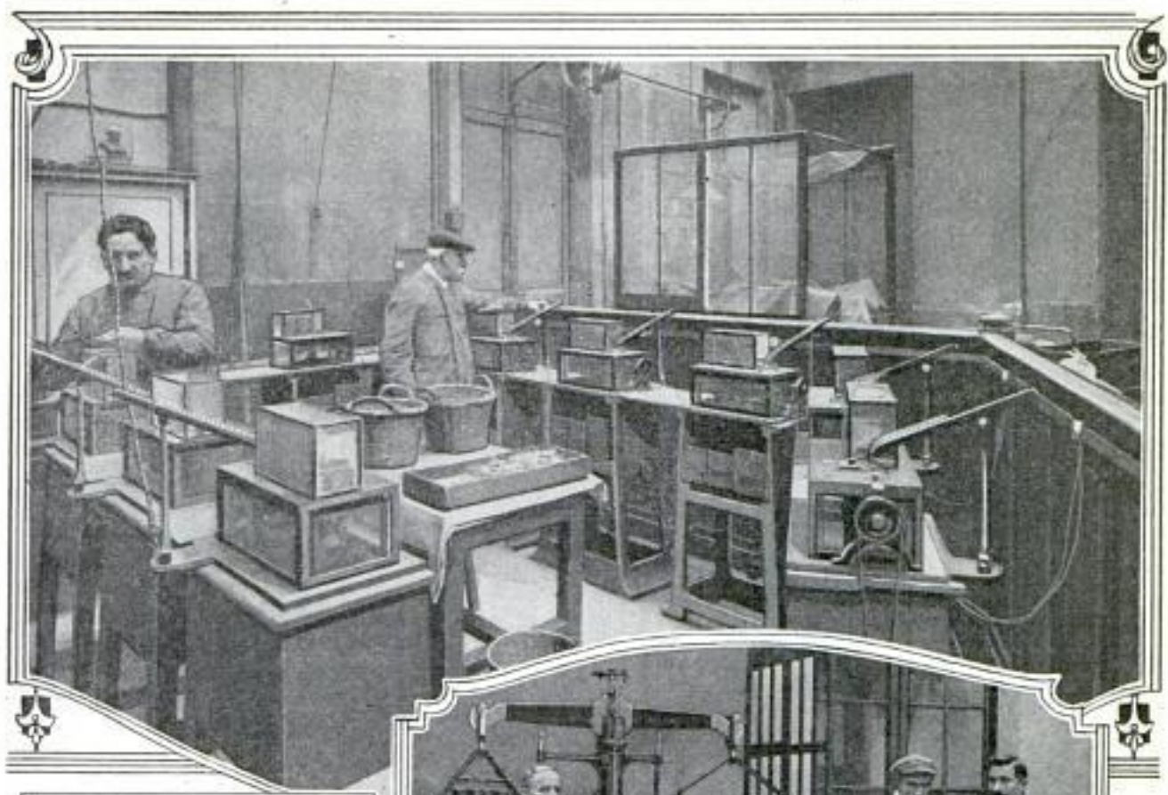
Accurate Glass - Inclosed Devices Equip the Rooms Where Coins are Weighed on Delicate, Automatic Scales as Rapidly as Men can Feed the Pieces into Electrically Operated Machines. When Rejected, They are Placed in Stacks Labeled "Lights" and "Heavies"
