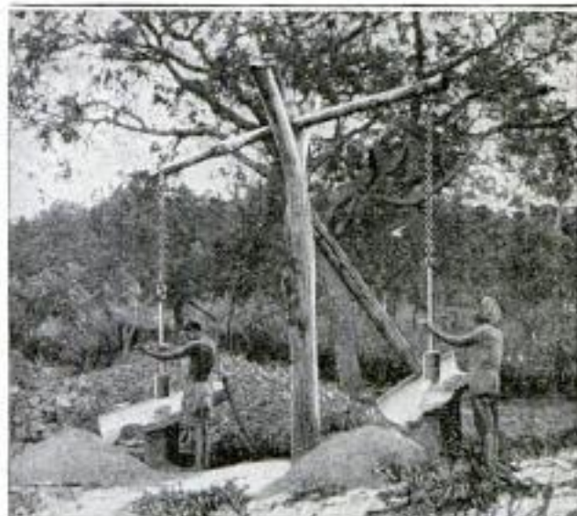
NEWMAN TRAVEL TALKS Natives in African Wilderness Stamp Ore with Weights Raised and Lowered by Hand
