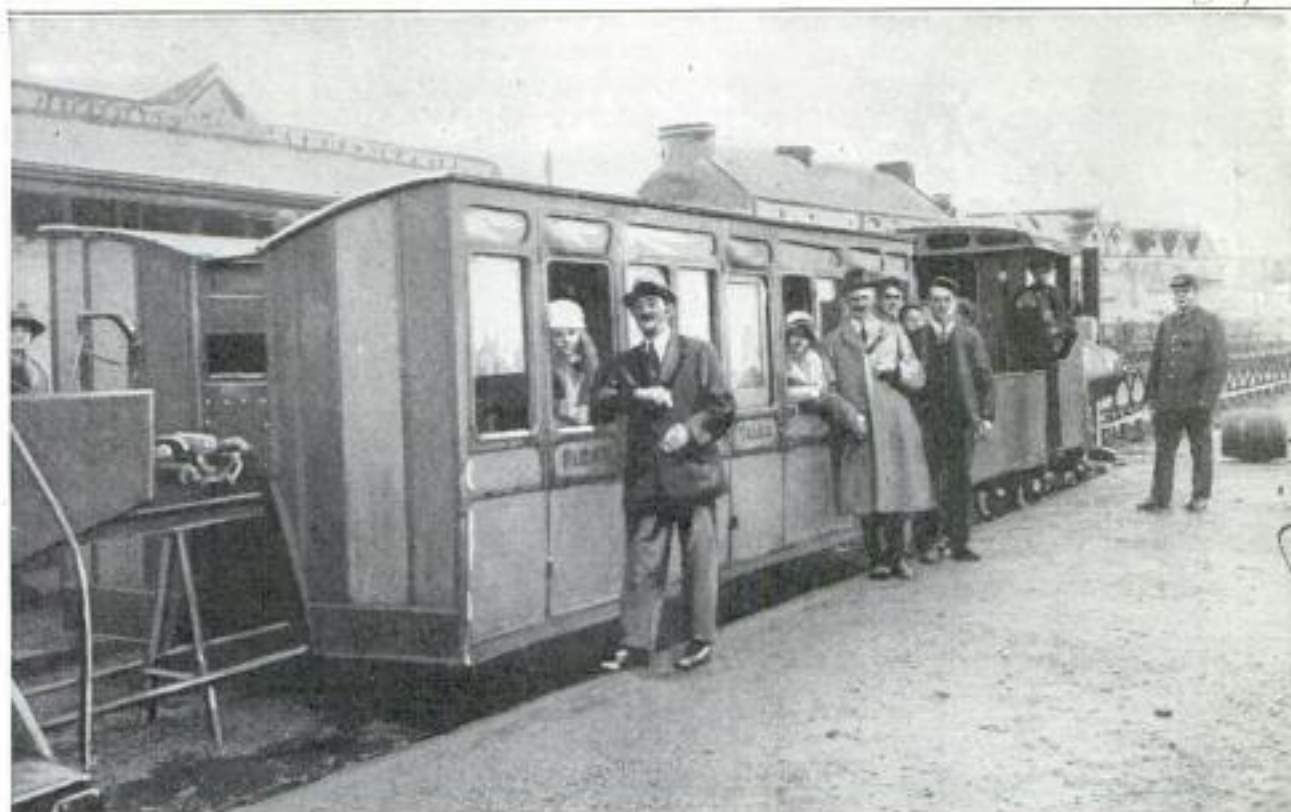
Passengers Enter the Coaches from Both Sides of This Monorail Train in Operation in Ireland. Several Classes of Accommodations Are Available as on the Standard Railroads
