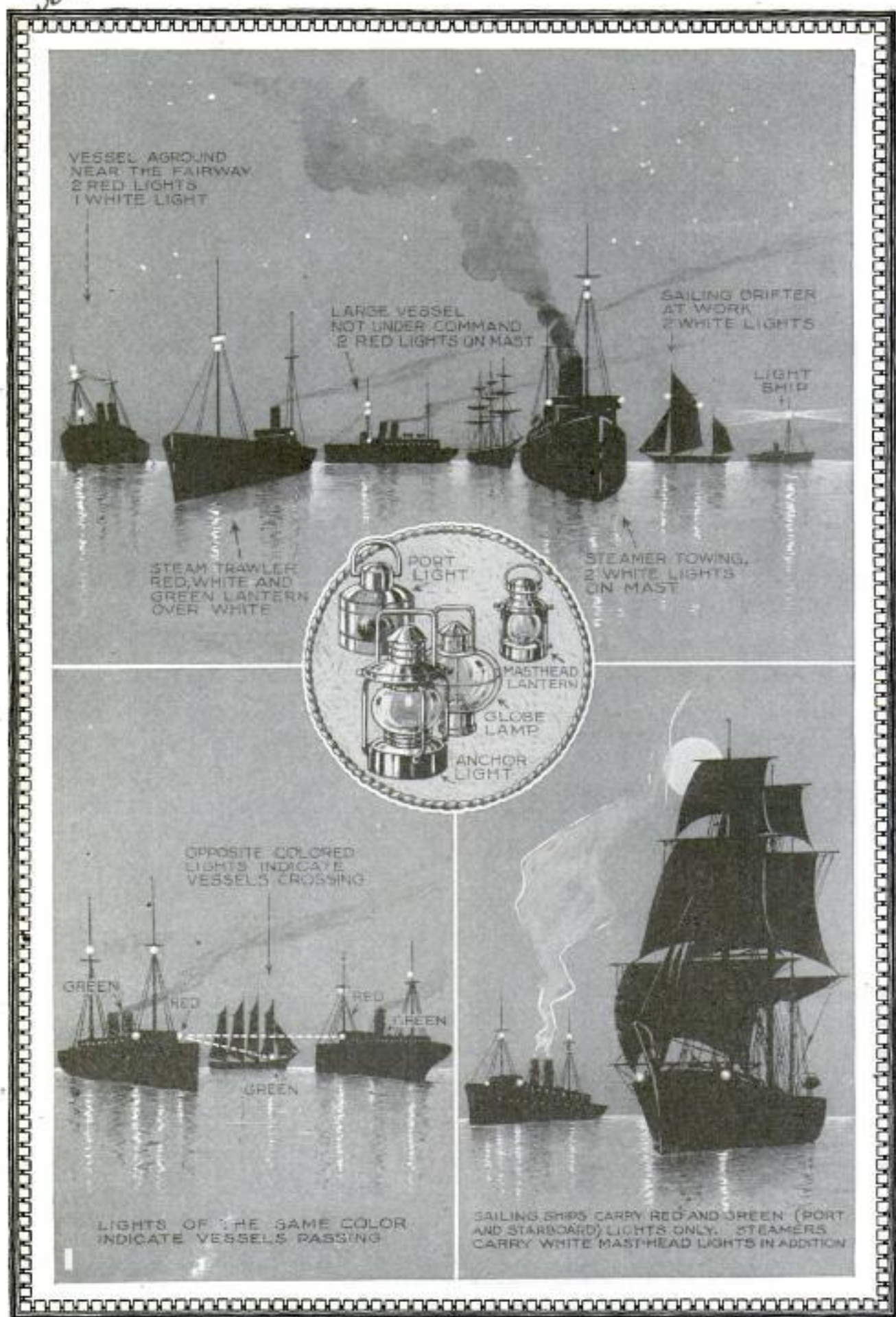
Ships of the Sea Employ a Universal Language of Lights to Inform Neighboring Craft of Their Size and Type, and Direction of Travel During Fog or Darkness
