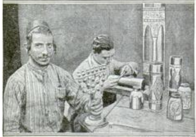
Skilled Brass Workers with Objects of Art Made by Engraving Discarded Cartridge Shells
