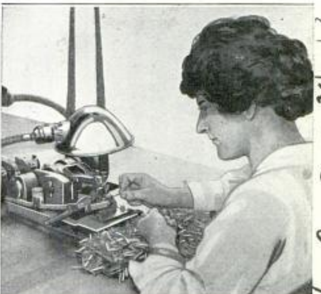
Operator Turning Out 180 Bamboo Phonograph Needles a Minute from Long Strips of the Material
