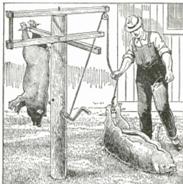
A Hog Hanger That can Easily be Operated by One Man without Any Assistance
