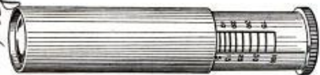
Small Range Finder That Is Aid to Amateur Photographers in Correctly Focusing Objects
