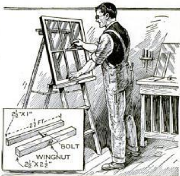
Handy Clamp on Stepladder for Holding Windows While Working on Them
