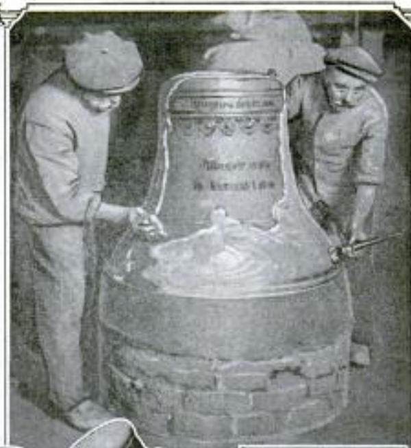
Grease is Applied to the Plaster Cast of the Bell, So That the Clay Molds can be Easily Removed When Hardened
