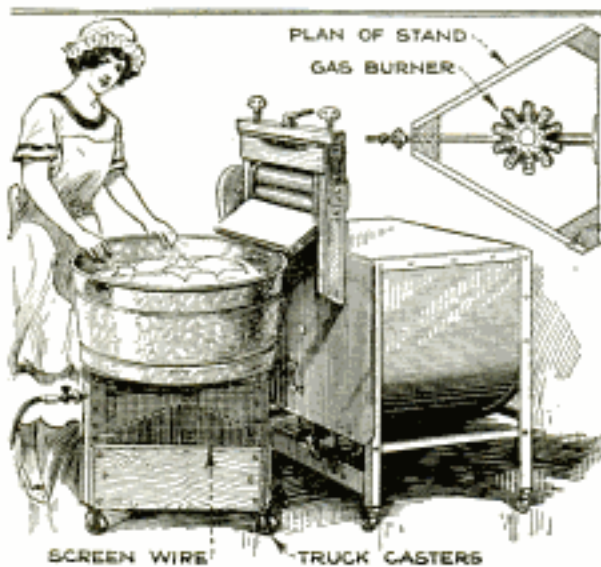
Movable Tub Stand and Burner Combined That Saves Much Lifting on Wash Days
