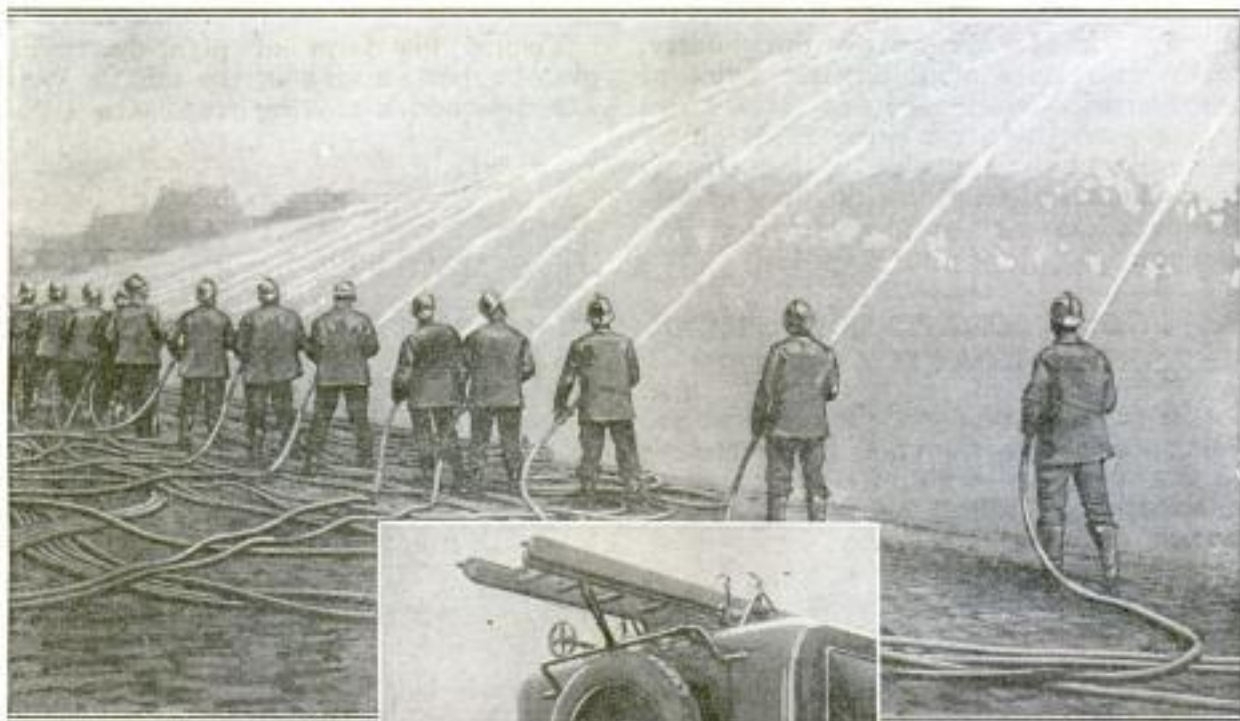
Right, Fire Engine That Feeds Twenty-four Lines of Hose
