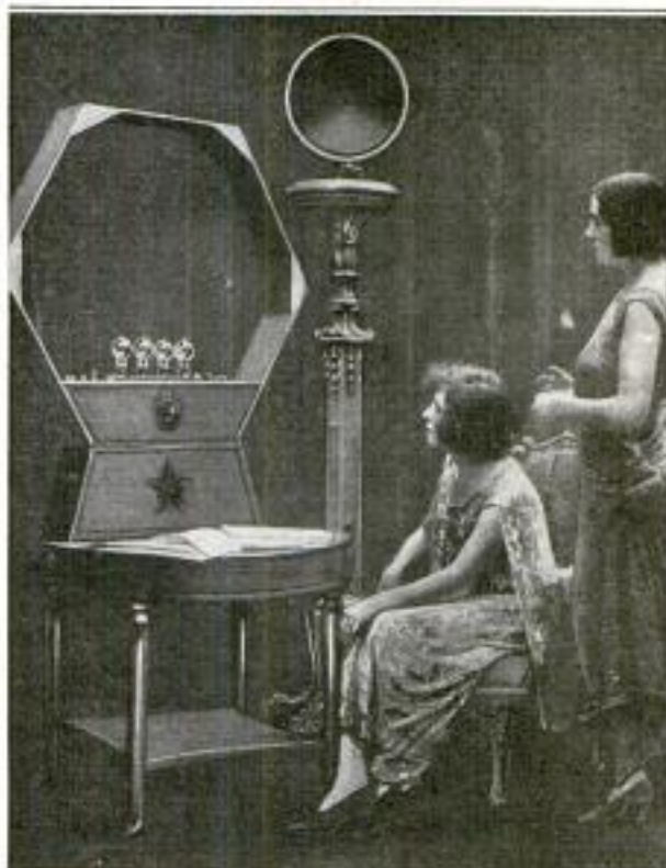
Listening to Message from French Radio, the Sound Intensified by Plate on Pedestal at Right
