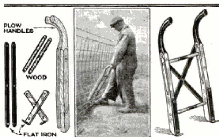
Left, Parts for the Wire-Fence Straightener; Center, Tool in Use; Right, Assembled Fence Straightener
