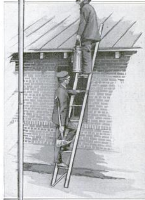
Fighting Fire from Folding Ladder that Can Be Opened in a Few Seconds: Left, Ladder Collapsed into Pole
