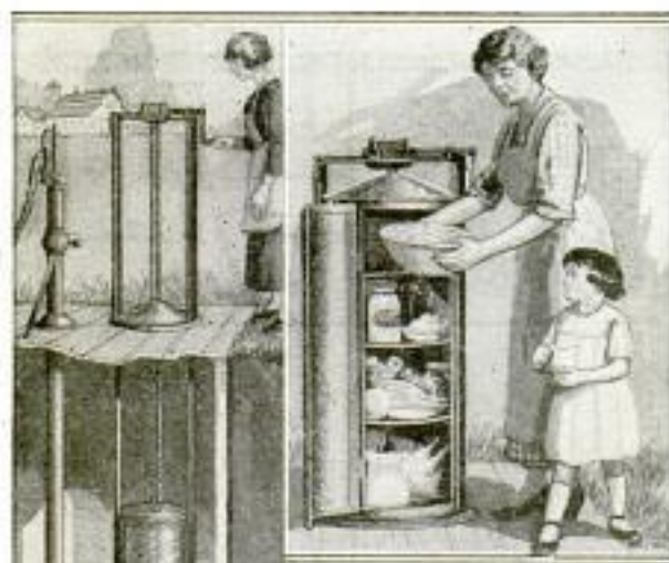
Iceless Cooler Installed in Deep Well to Keep Food Fresh at Little Cost
