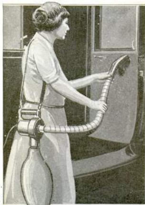
Renovating Upholstering of an Automobile with Vacuum Cleaner That Straps to Shoulder
