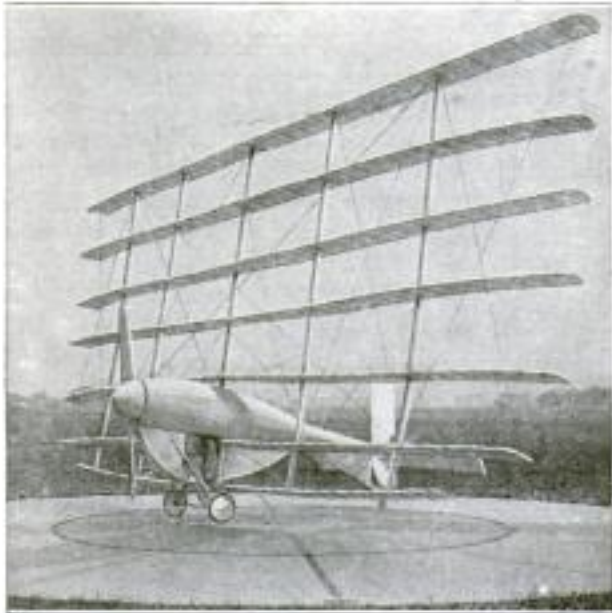
Seven-Winged Airplane That Made Seven-Yard Flight Propelled Only by Foot Power
