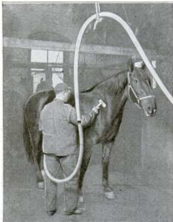
Cleaning and Dressing the Hair of a Horse With Currycomb Attached to Vacuum Cleaner
