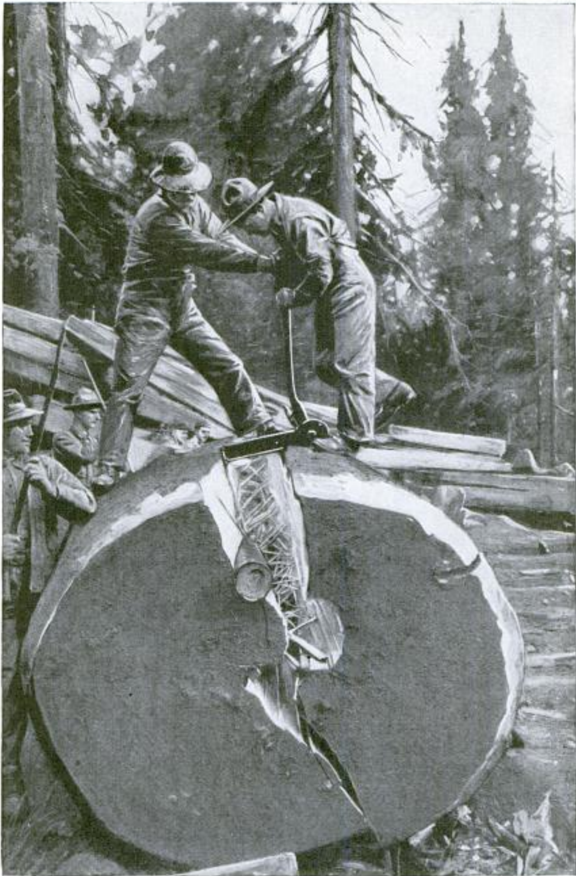
After It Is Down, the Hemlock Giant is Divided by the Spreader and Cut into Smaller Logs That Are Easier to Transport to the Railroad Siding for Shipping
