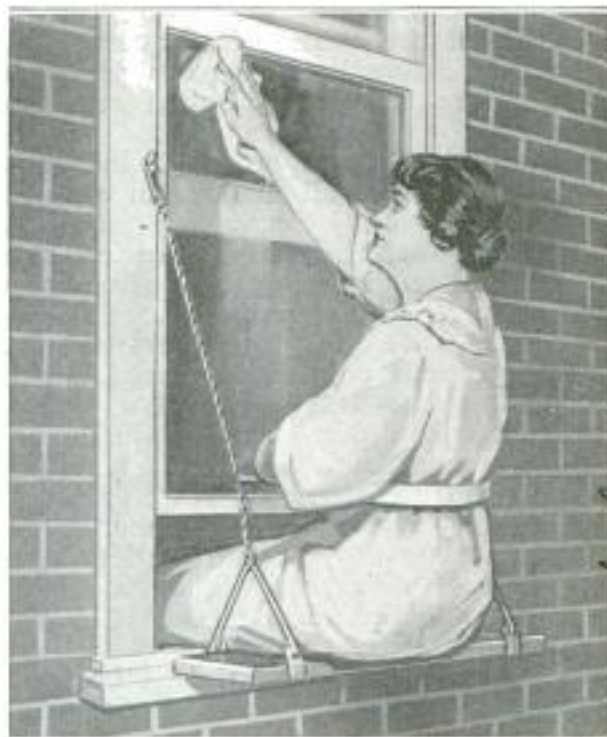
Seat Swing for Preventing Accidents to Those Washing Outside Surfaces of Windows
