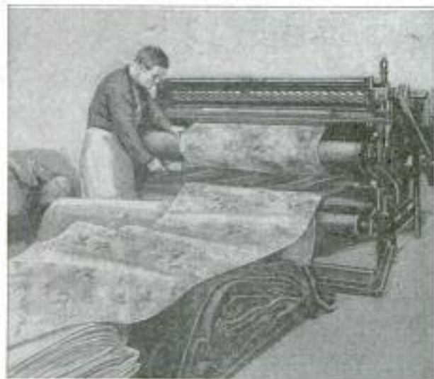
Revolving Knives Trim the Pile of Machine-Made Carpets to a Velvet Finish
