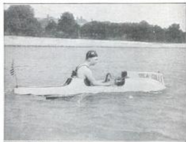
Copyright, International Newsreel Corp. Rider Operating Bathing Boat by Pumping Bicycle Pedals That are Connected by Chain with Propeller
