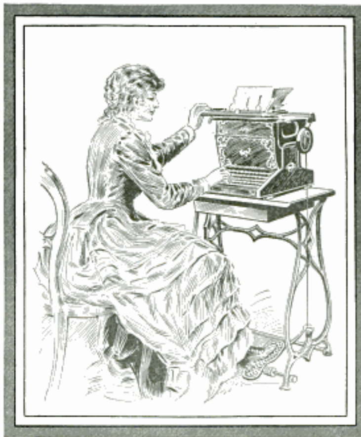
First Typewriter Put on the Market in 1873 with Curious Foot Treadle to Return Carriage
