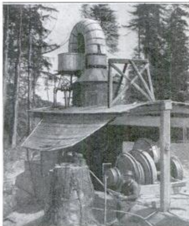
Fire Protector being Used on a Logging Engine in a Big Lumber Camp
