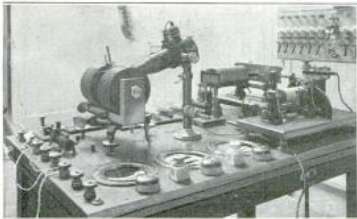
Transmitting Autographic Messages by Wire. Using Photographic Process of Recording the Movements of a Beam of Light Directed against Chemically Treated Paper
