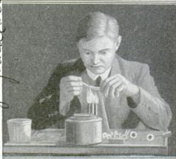
Hollow Crystallike Stems are Attached to Melted Glass for Inflating the Bubble
