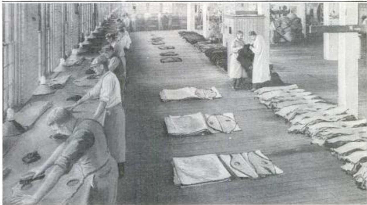
Dyeing Sealskins by Brushing on the Color with Ordinary Scrub Brushes: Note How Skins are Folded; They are Not Allowed to Rest Otherwise
