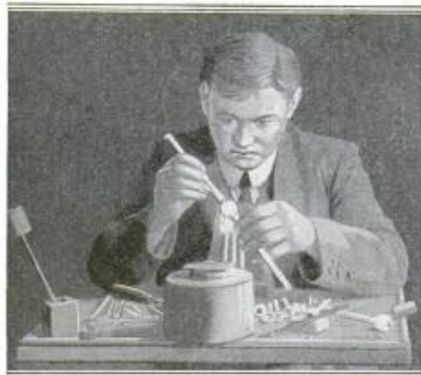
Ground Shades for the Iris are Traced from Sticks of Brightly Colored Glass
