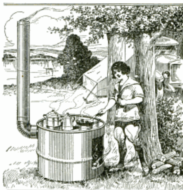
A Serviceable Camp Stove, Made from a Steel Oil Drum, and Equipped with a Chimney
