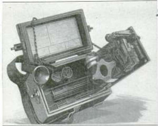
Batteries and Wiring Inside of the New Army "Buzzerphone" Devised to Defeat Spies
