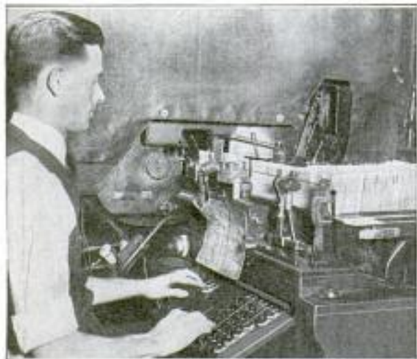
Machine That Does Work of Several Clerks in Sorting Letters into Bags by Cities and States
