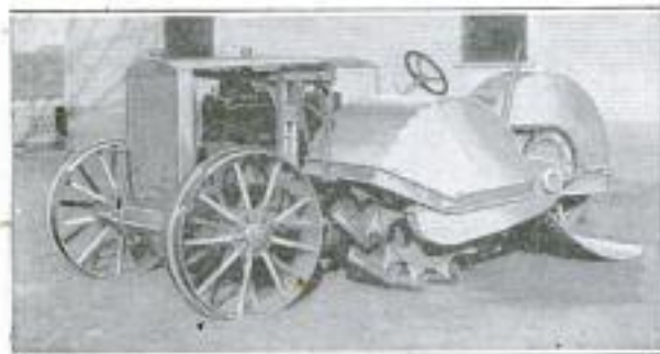
Drum Studded with Shears Which Make It Possible to Plow within Five Feet of the Corner Posts
