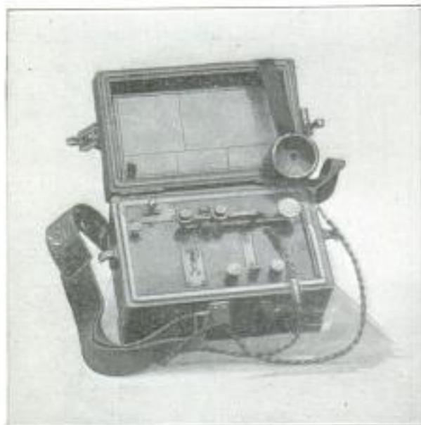
Telegraph and Telephone Set Built by Army Engineers to Send Messages without Detection
