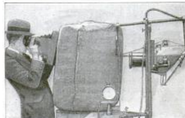
X-Ray Machine being Used to Look into Bale Suspected of Containing Contraband
