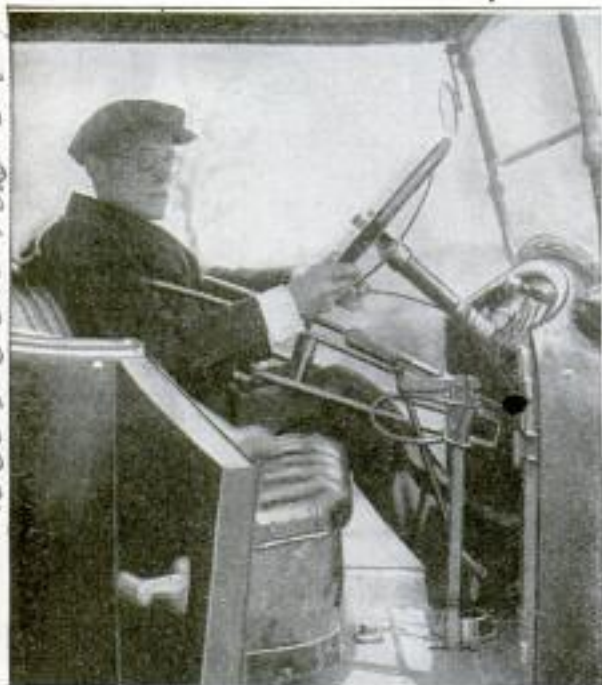
Auto Equipped with Special Devices to Enable It to be Easily Handled by Man Who cannot Use His Feet
