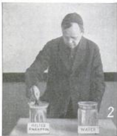
Dipping the Glove: The Cold Water Inside the Glove is Causing the Paraffin to Harden
