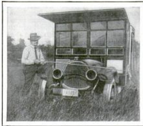
Front View, Showing the Clear-Vision Windshield That Allows Each Passenger an Unobstructed View
