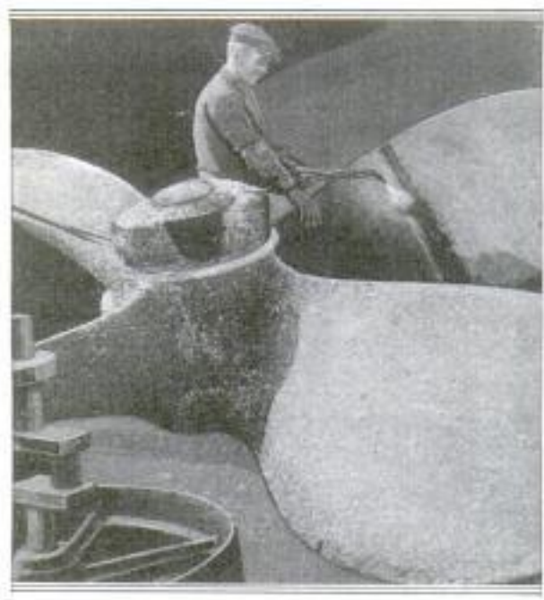
"Sawing" Up an Old Propeller with the Acetylene Torch, to Make Automobile Parts
