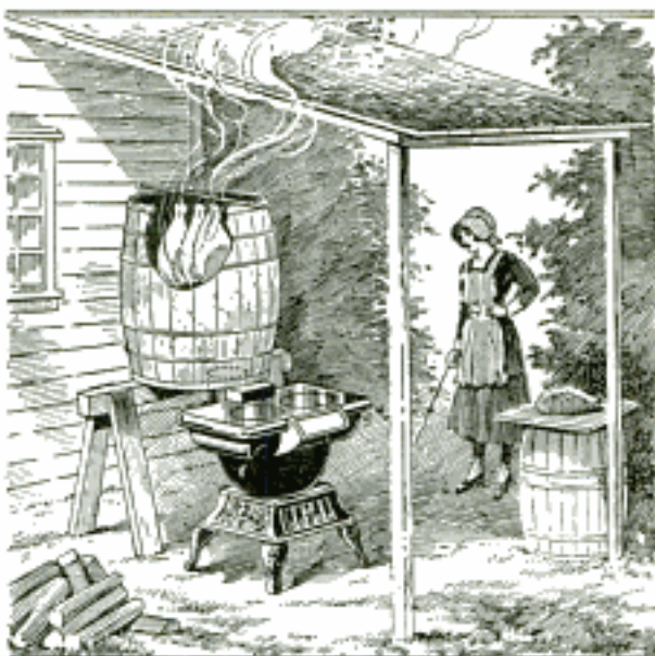
An Improvised Smokehouse, Consisting of a Laundry Stove, a Barrel, and a Support Such as a Sawhorse or Wooden Box
