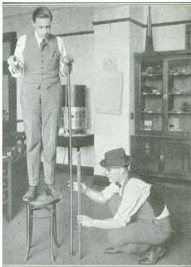
Baseballs Dropped from Different Heights and Rebounds Measured to Test Liveliness
