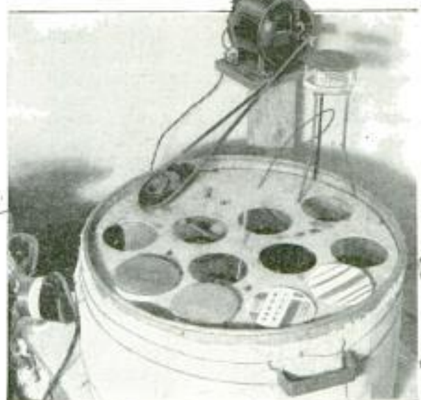
The Apparatus Shown Above is Used to Test the Moisture-Absorbing Properties of Blankets
