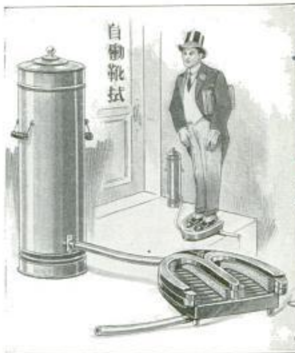
Close-Up of Japanese Boot Washer, and, in the Background, Its Installation and Use at an Office Entrance
