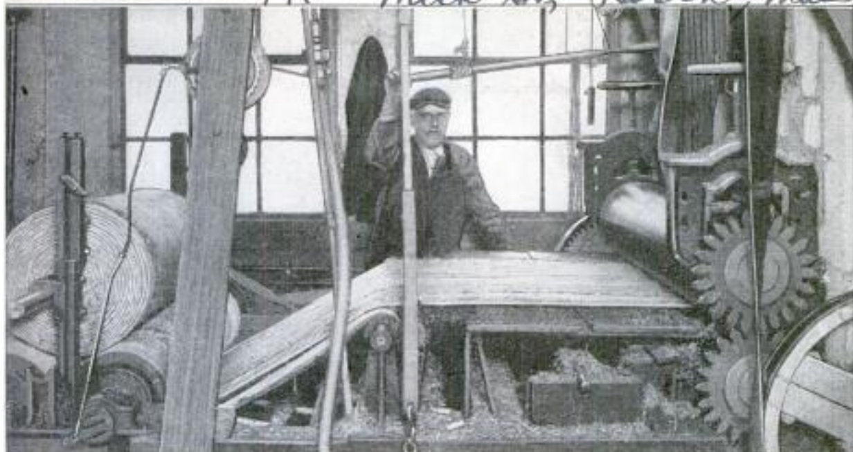
"Quilts" of Eelgrass Coming through the Rollers: They are Stitched, and the Stitching is Glued in Place to Prevent Ripping. Heavy, Hot Rollers Then Compress the Quilts, Which Pass On to be Crimped
