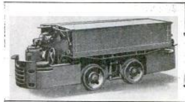
Electric Storage-Battery Locomotive Which is Made Flame-Proof for Use in Gaseous Mines
