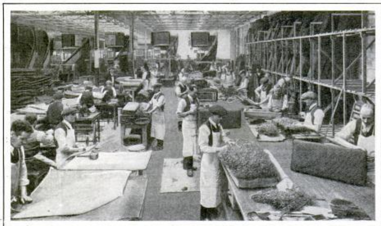
Interior View of the Upholstery-Trimming Shop: In This Department the Cushions are Completely Renovated, New Material being Used Where the Old is No Longer Serviceable
