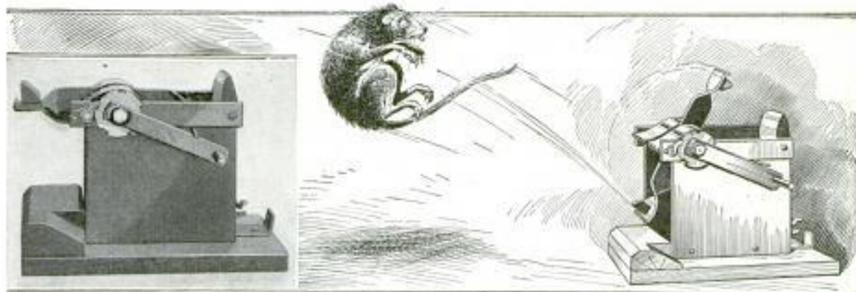
This Rat Killer Knocks Its Victim on the Head, Then Flings It Promptly Away from the Machine. On the Left is a Close-Up of the Device When Set
