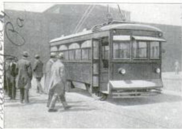
The Trackless Trolley in Perspective: It can Travel a Maximum of 16 Feet Each Side of the Overhead Wire
