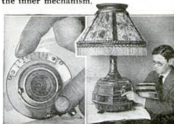
Right: Combined Lamp, Radio Set, and Phonograph, Said to Be the First of Its Kind Invented. Left: Magnetized Diaphragm for Varying the Sound
