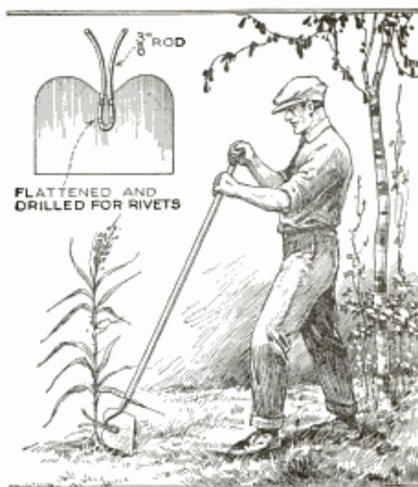
Simple Fork Attachment for a Garden Hoe, That Enables Weeds to be Uprooted without the Danger of Cutting Near-By Plants
