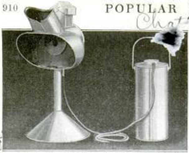
An Acetylene Egg-Candling Machine, Claimed to Furnish a More Satisfactory Means of Grading Eggs than the Electrical Candler
