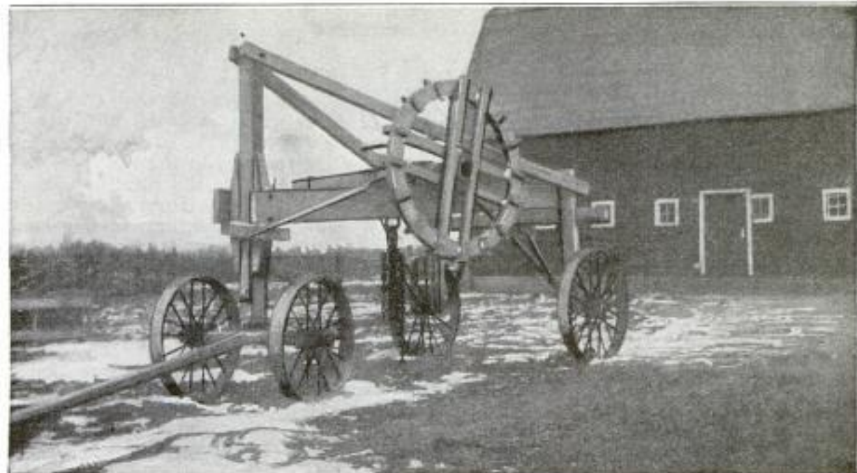
Simple Rig Devised by an Enterprising Farmer for Getting Heavy Stones Out of His Fields: One Pair of Horses, Pulling on a Rope around the Large Wooden Wheel, will Raise a Six to Eight-Ton Rock Out of the Ground
