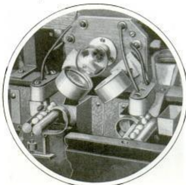
Close-Up of Two Units of the Bean-Sorting Machine: Note the Bad Bean Picked Out by the Unit at the Left.
