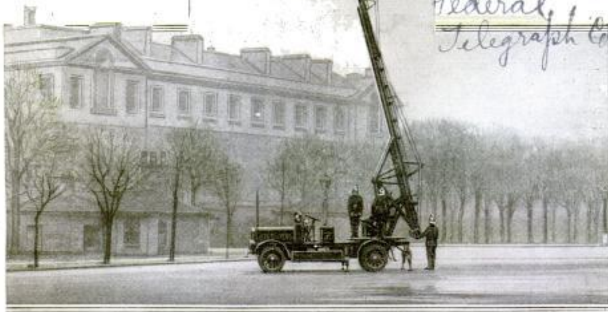
Motor Turntable Fire Ladder When Fully Extended to a Height of 90 Feet: With the Truck Stationary, the Ladder can be Turned Around at Right Angles to the Chassis. Indicators Give the Extension and Working Angle Found Safe
