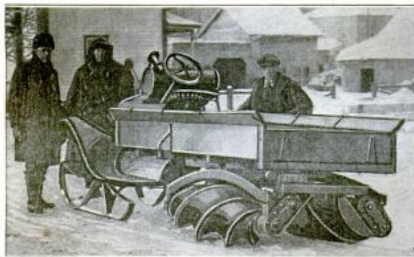
Motor-Driven Sleigh Equipped with Specially Designed Wheels, Which Increases Its Traction with the Load upon It: Each Wheel is Separately Driven through Gears at the Rear
