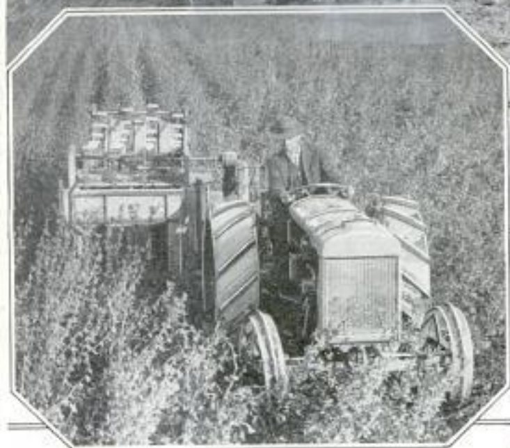
Above: Rear View of Combined Soy-Bean Harvester and Thresher, Showing Removal of Beans after Trip across Field. Left: Machine Operating in Field; Note That Machine is Offset from Tractor Which Travels over Harvested Ground
