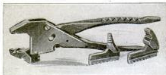
The Three Interchangeable Jaws of This Tool Convert It into a Wrench for Several Purposes
