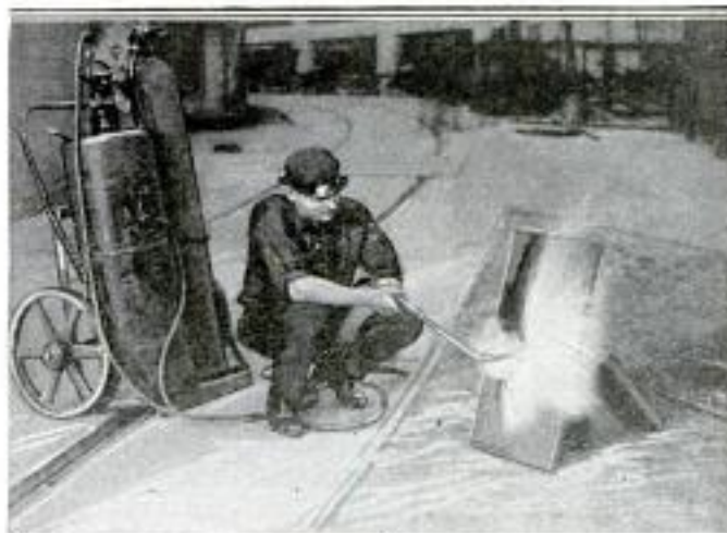
Upper Left: Showing the Unusually Severe Test to Which a Sheet of Fiber Flooring was Subjected to Determine Its Fire-Resisting Qualities. The Intense Heat of an Oxyacetylene Flame was Applied for Several Minutes. Upper Right: After the Test; Only a Few Scorch Marks Resulted, Not Even Burning through the Sheet. Lower Right: How the Sheets are Laid Down. The Joints between Them are Later Filled with a Special Compound
