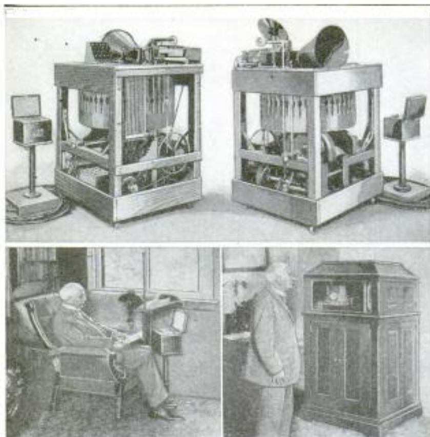
Above: Two Views, Showing Mechanism of Phonograph That Picks Out Its Own Records. Lower Left: Portable Keyboard Mounted on Pedestal. Lower Right: Listening to the Music
