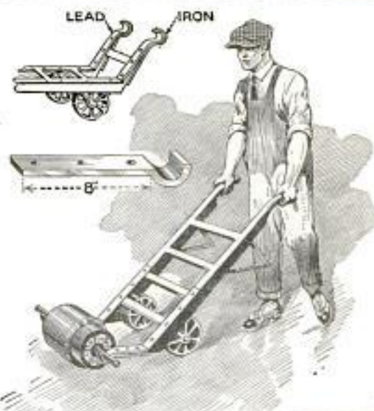
Attachment for Hand Truck That Facilitates the Handling of Armatures: With It One Man can Handle an Armature That Ordinarily would Require Two Men
