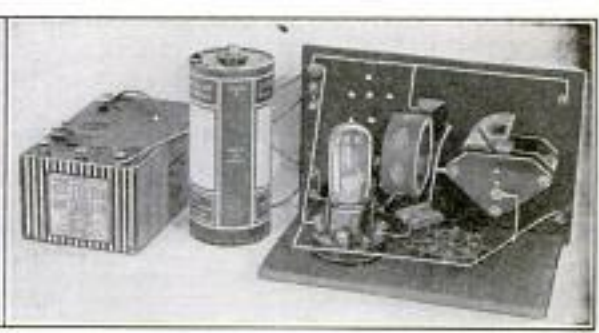
Figure 1, Template for Laying Out Detector Panel; Figure 2, Dry-Cell Tube and Sockets; Figure 3, Rear View of Detector Panel, Showing Location of Instruments, Battery and Phone Connections, and Method of Wiring; Figures 4 and 5, Front and Rear Photos of Completed Detector, with Batteries, Ready for Operation as Soon as the Phones are Attached
