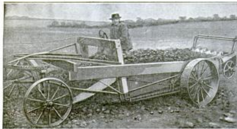
A New Type of Dumping Wagon Designed for Scooping Up and Moving Earth and Similar Materials on the Farm: The Hand-wheel Controls the Depth of the Scoop
