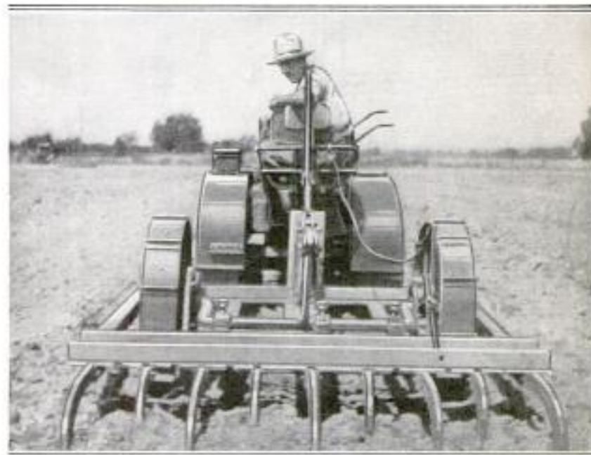
Heavy-Duty, Deep-Tillage Cultivator Operating at Depth of 12 Inches: The Large Teeth Tear the Hardest Soil
