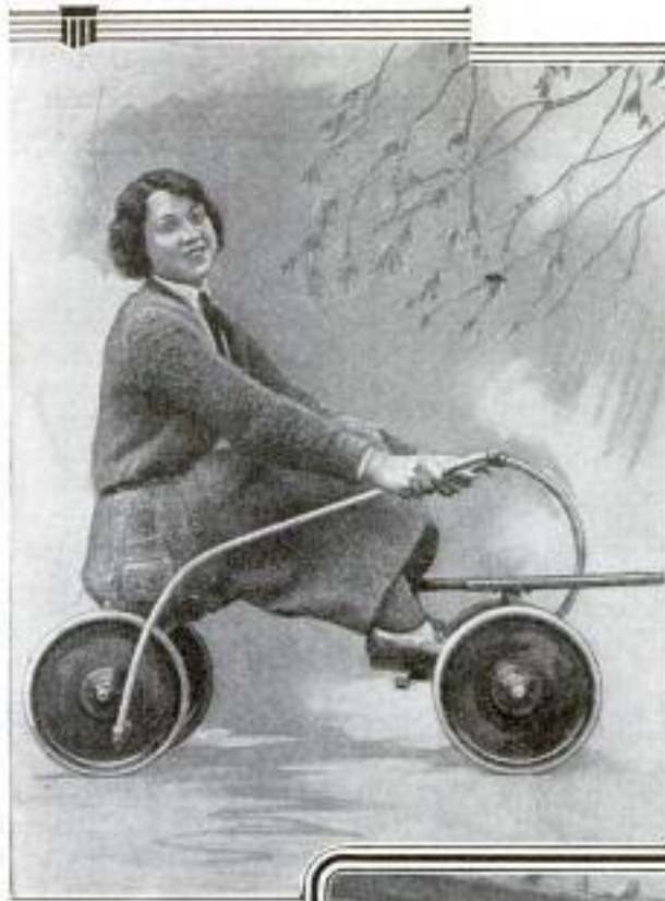
A New Vehicle for the Kiddies Which is Propelled with a Motion Similar to Rowing, and is Steered with the Feet: It is Also Seen as an Exerciser for Some of the Mothers
