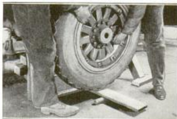
A Simple and Quick Method of Removing Heavy Truck Wheels: A Strong Board and Two Rollers Bear the Weight
