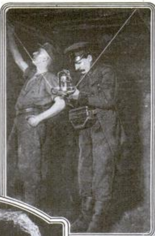
A Master Miner Establishing the Direction, by Means of a Surveyor's Compass, for a New Working in the Ruhr: In a Well-Organized Mine This Work is Done with Great Care, So as to Develop the Property Economically
