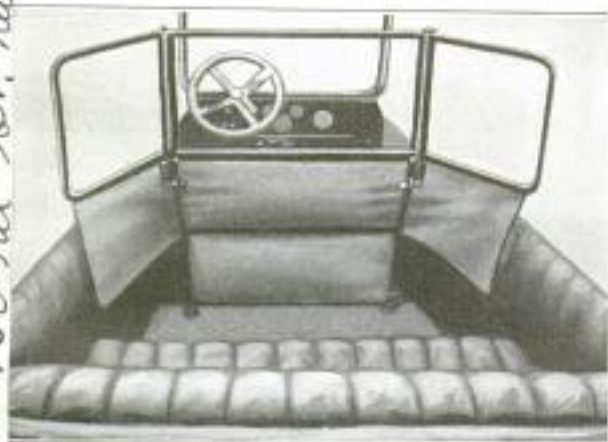
A Tonneau Shield with Adjustable Wings: The Attachment is Said to Be Rattle-Proof, and Easily Secured to the Back of the Front Seat
