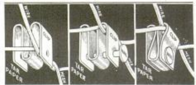
The New Furring Clip Showing, from Left to Right, How It is Applied to the Wire Mesh and Nailed to the Wall
