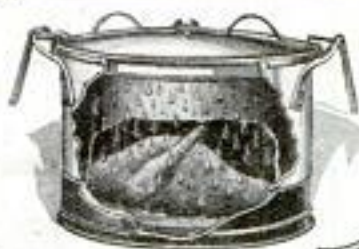
A Combination Cover Clamp and Lifter, Making It Easier to Keep the Lid Closed Air-Tight, or to Lift the Cooker When Hot
