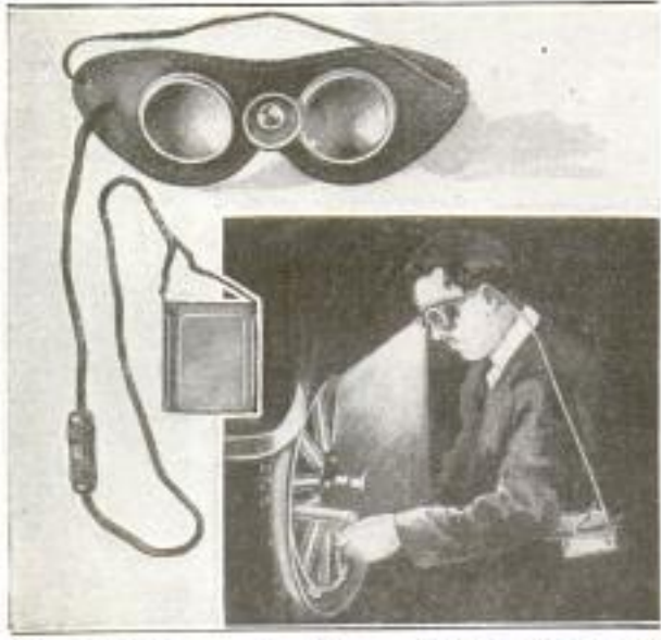
The Light between the Glasses of These Goggles is Arranged to Focus in the Direction of Vision. At the Right is Illustrated One of the Uses for Which the Lamp is Particularly Adapted
