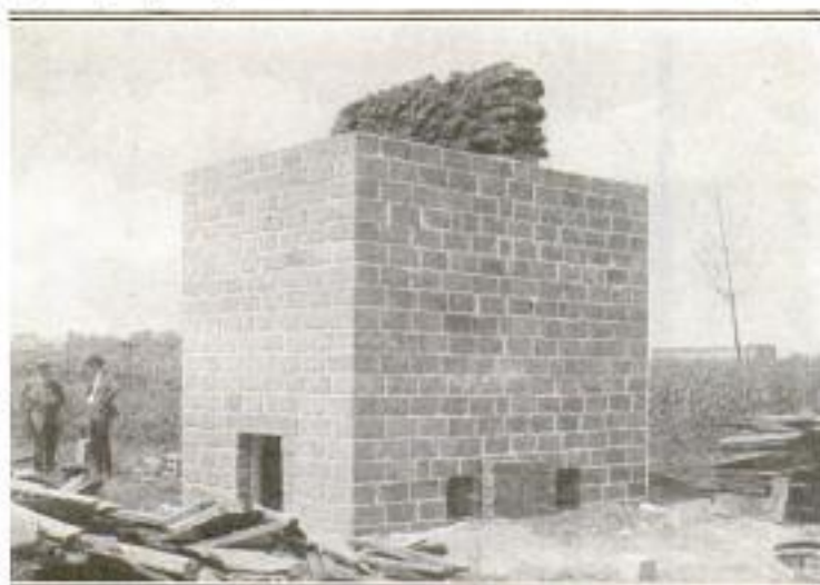
Test Block House, Loaded with 11 Tons of Pig Iron, in Which the Fire Raged for an Hour: The Blocks Withstood This as Well as More Severe Compression Tests Later
