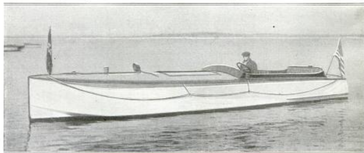
The "Isabell," Purchased by the University of Wisconsin, to be Used as a Lifeboat on Lake Mendota: The Craft Is 30 Feet Long, Has a Beam of 6.6 Feet, and Is Capable of Doing 28 Miles an Hour or More. Its Steering Wheel and Other Controls Resemble Those of an Automobile
