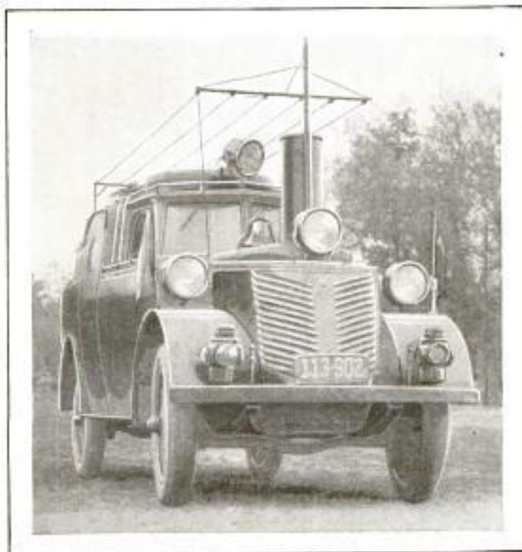
Front View of the Land-Going "Yacht," the Stack of Which Carries the Exhaust from the Engine: A Refrigerator and Steam Tables for Cooking are Included in Its Equipment
