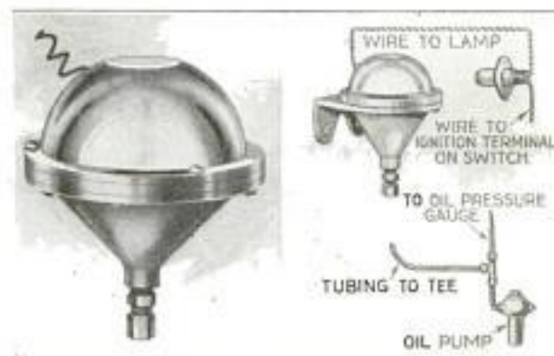
An Automatic Oil Signal for Automobiles: After Fitting to the Dash, a Connecting Wire is Run to the Lamp and Then to the Switch Ignition Terminal
