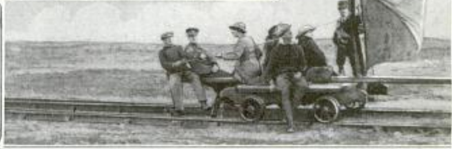
Sailing Cars on English Railroad Track. Above: Cars Sailing the Track with Wind on Their Beams. Right: Car before the Wind, Whose Force is Shown by the Tautness of the Sheet, or Rope Holding the Boom
