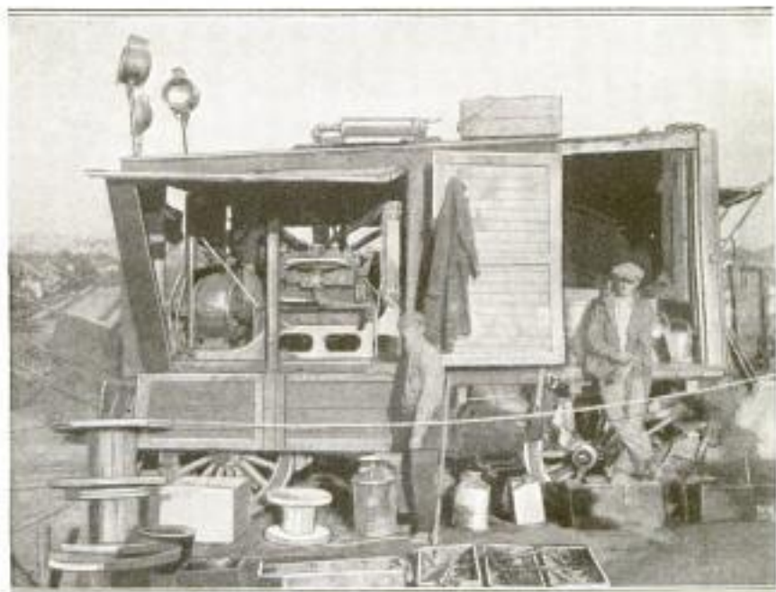
Electric-Lighting Plant Mounted on an Ordinary Horse-Drawn Circus Wagon, Which Supplies the Energy for Approximately 1,000 Medium-Sized Floodlights: It is Driven by a Gasoline Engine
