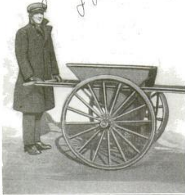
Machine Used to Sprinkle Sand on Icy Streets: A Chain Running on Sprocket Wheels Works an Agitator That Scatters the Sand from the Box
