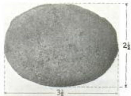
Fuel Briquettes. Like This, Made from Wood Waste, are Said to Equal Anthracite
