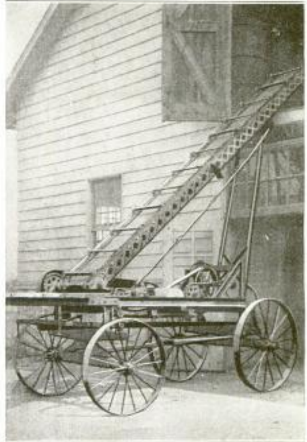
Portable Elevator for Raising Baled Hay and Mill Feed into Barn Loft
