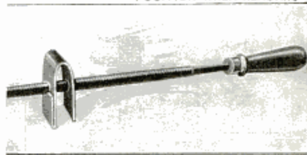
Above: Details of Spring Clip That Prevents the Workman's Fingers from being Pinched between Work and File. Below: Clip in Place on File
