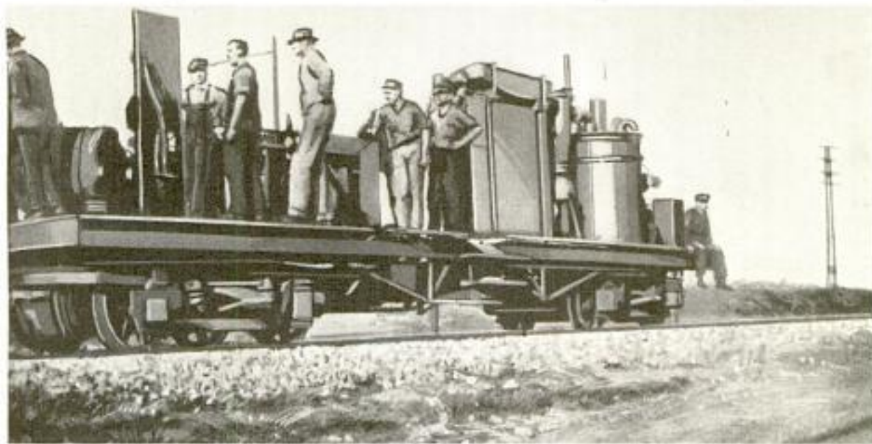
Self-Propelled Railway Car, Which Runs on Gas Generated from the Unburned Carbon in the Ashes Dumped from the Ordinary Type of Locomotive: It Carries Its Own Gas Producer, Internal-Combustion Engines, and Electric Generators That Supply Current for the Motors
