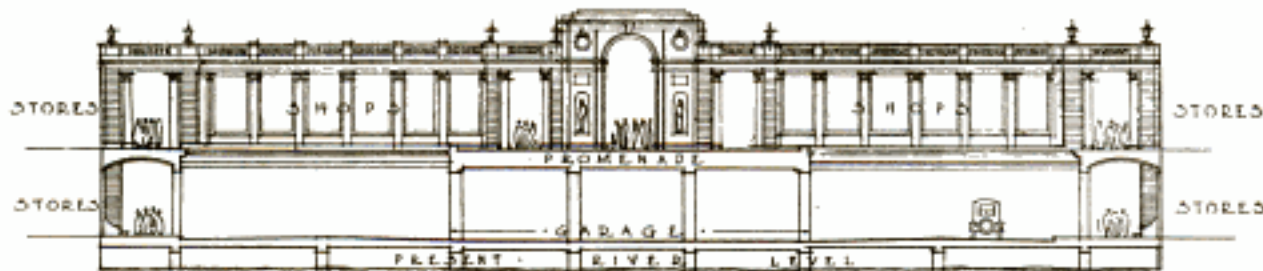
Cross Section at One of the Bridges: The Distance from the Water Level to the Street will Be 4 Feet, and from the Street to the Roof of the Bridge About 14 Feet. The Sidewalks will Be 15 Feet Wide, the Driveways 51 Feet, and the Garage Space between Them, 68 Feet. Each Section will Be Large Enough to Accommodate 250 Cars
