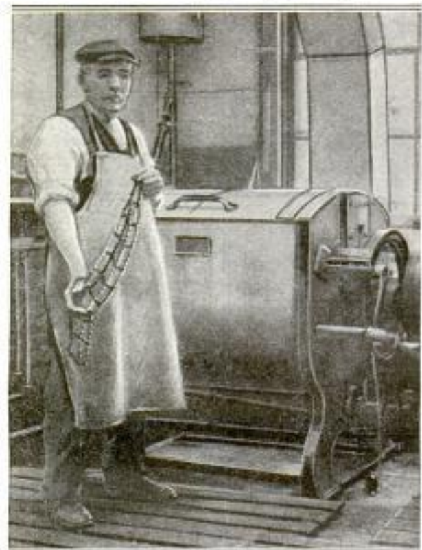
An Effective Device for Preventing Explosions in Dry-Cleaning Plants: The Chain Which the Workman is Holding Serves to Ground Static Charges of Electricity
