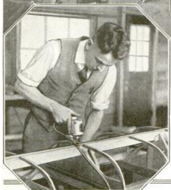
Above: One of the New Racing Shells of the University of Washington in the Course of Construction. The Framing is Made of Spruce and the Planking of Port Orford Cedar. In Order to Meet the Requirements of the Western Oarsmen, the Shell is Designed with a Decided Bow Lift. Left: Close-Up, Showing the Joining of the Keel and Ribs
