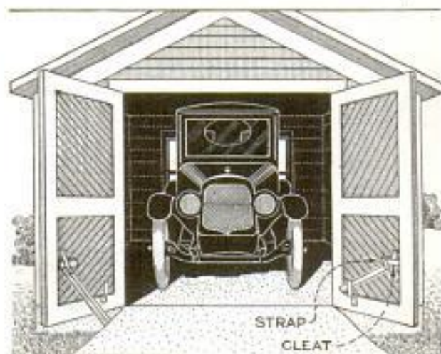
Method of Keeping Garage Doors from Closing, Which Proves of Considerable Assistance When Driving into the Garage Unaided
