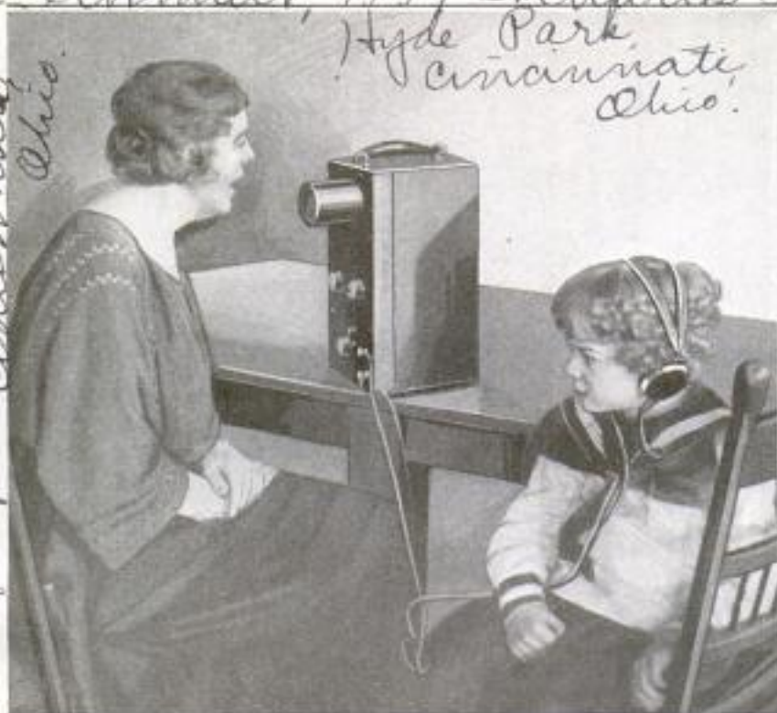
The Radiophone as Used in Teaching the Deaf to Hear: The Teacher Speaks Plainly and Slowly into the Transmitter, and the Pupil Listens through the Usual Head Receiver. The Method has Been Fairly Successful
