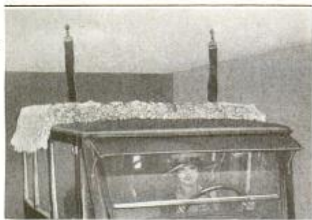
Auto-Top Duster, Hanging from Ceiling of Garage, Automatically Cleans Top of the Car as It Enters and Leaves
