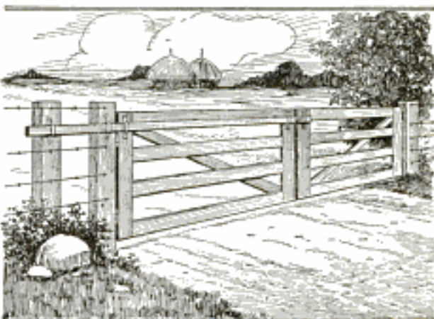
A Double Gate for the Farmyard, Constructed So as to Eliminate the Objectionable Center Post of the Usual Double Gates
