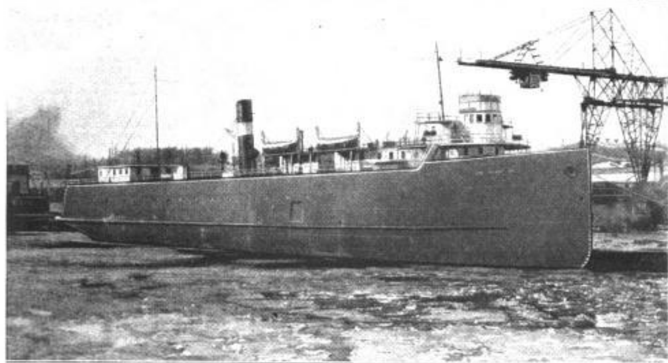
The "Ann Arbor No. 3," a Car Ferry of the Ann Arbor Railroad Which Recently Underwent an "Operation" by Which the Length of the Boat was Increased 48 Feet and the Carrying Capacity Made One-Third Larger: The Vessel Plies between Frankfort, Michigan, and Manitowoc, Wisconsin
