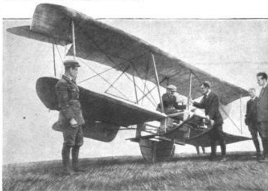
German Glider Student Learning to Operate a Motorless Plane Which Rests on a Double-Rocker Arrangement: The Pupil Thus Learns to Balance the Machine by Operating the Controls
