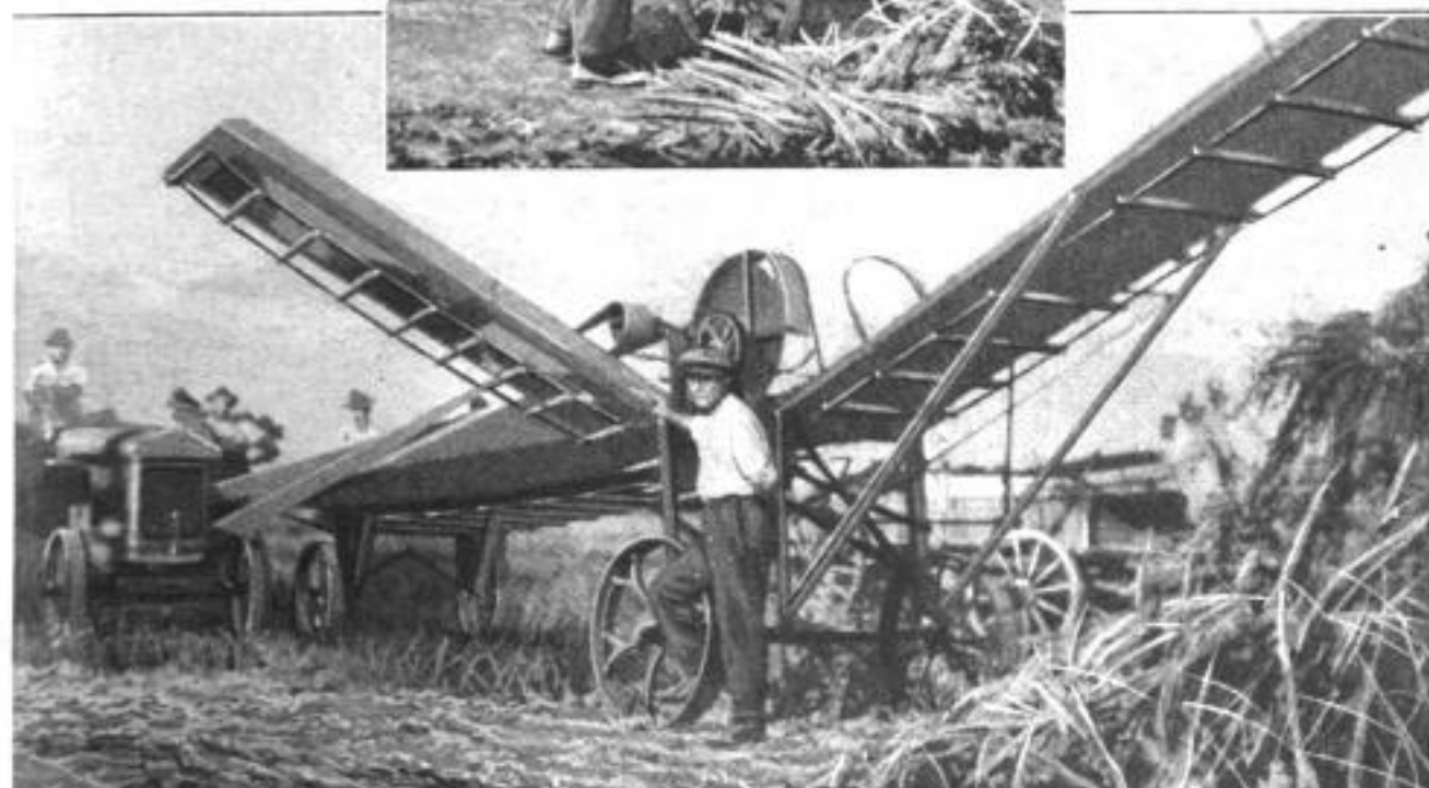
A Topping Machine for Cutting the Heads from Corn, Maize, and Other Grains: Above, the Loading End; Below, View of Both Conveyors, and the Belt-Driven Saw for Cutting the Stalks
