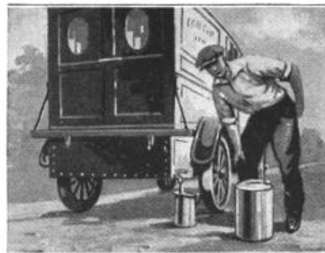
A Gasoline Tank from an Old Automobile Serves to Carry Kerosene on a Grocer's Truck, Thus Eliminating the Possibility of Spilling Groceries
