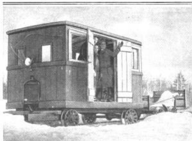
Above: The Combination Locomotive and Passenger Coach in Service, with Bulk-Freight Trailer. Note the Radiator and Auto Headlight on Front End. Right: The Manager of Maine's "One-Man" Railroad, in the Capacity of Engineer, at the Throttle of His Locomotive.
