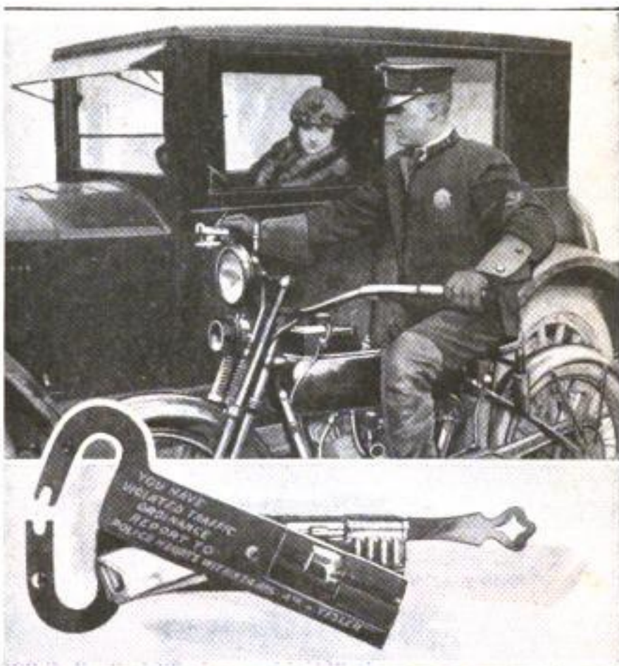
Police Officer Locking New Summons Device to Door of Car: Imprinted on the Lock, as Shown Below, Is a Notice to Report to Police Headquarters, While, within It, is Placed the Summons Proper
