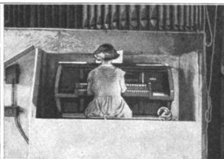
The Pipe Organ with the Removable Front Section of the Galvanized-Iron Protecting Case Pulled Up and Out of the Way
