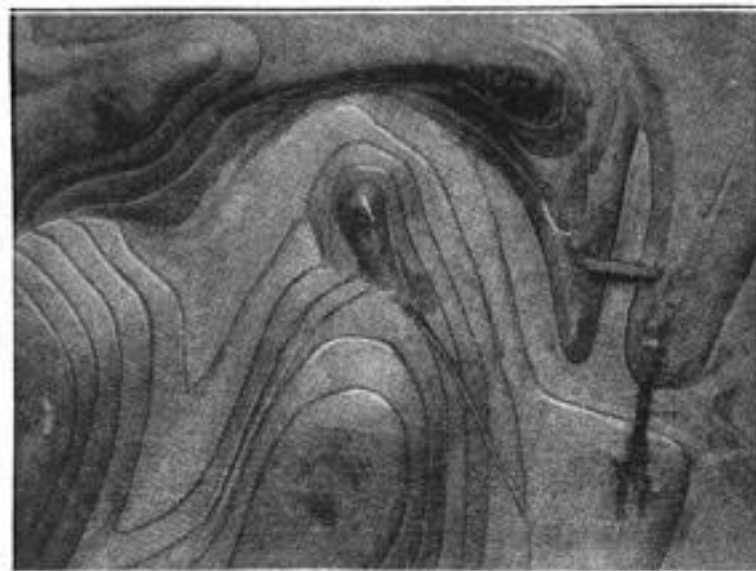
The Lines Like Knurls in a Knot Are in Reality Layers of Aluminum Used in a Military Contour Map
