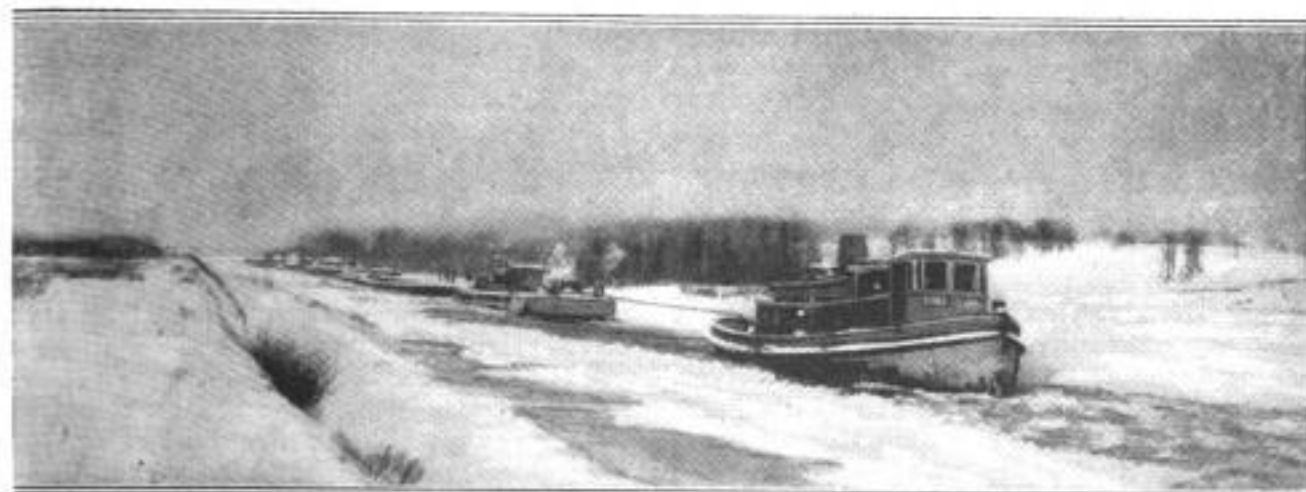
Powerful Steam Barge Assisting in Opening Up a Channel for the Ice-Bound Canal Boats: First Backing Twice Its Length, the Barge Then Dashed Forward, Plowing through the Ice Till It Stopped. The Assault was Repeated Until the Way was Cleared
