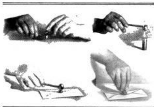
Successive Steps in Preparing the Sealing Wax: Dropping the Ball in the Ladle, Heating It, Pouring the Wax, and Impressing the Stamp
