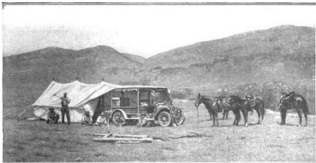
The Tent Carried by the Motor Truck is Erected So That, When Shut, It Incloses the Entire Body. In This Way the Floor of the Car can be Used for Sleeping Quarters, While in the Daytime the Truck and Tent, Respectively, Serve as Dining Room and Kitchen
