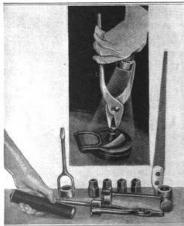
The Flashlight Handle: It is Quickly Attached to Any of the Tools Shown, and Serves as Handle for the Screwdriver, or as One of the Grips for the Pliers
