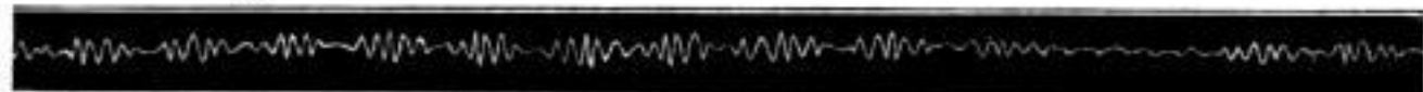
Records of Vibrations Caused by Two Dynamos Running at Different Speeds: Note the Repetition of the "Wave" Action Caused by the Periodical Rising and Falling of the Tremors
