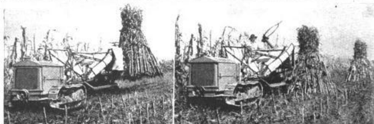
Left: A Harvester Which can be Drawn by Three Horses or a Light Tractor. A Full Sheaf of Corn can be Shocked Every Four Minutes. Right: When Shock Holder Is Full Enough to Make Desired Size of Shock, One Man Proceeds to Clamp the Circular Arms around the Shock at the Tying Point
