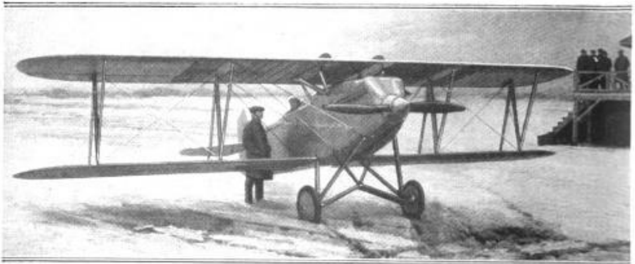
Army Pursuit Plane That Is a Modification of the Airplane with Which General Mitchell Established a Speed Record: In Addition to Speed, It Features a Wing Structure That Is Practically Invulnerable to Shrapnel Fire, and the Ability to Start Quickly in Cold Weather
