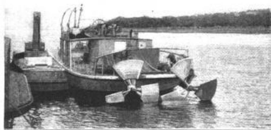
The 11-Foot Vane Wheels Temporarily Installed on a Vessel Designed for Twin Screws: Although Badly Handicapped by This Condition, the Wheels Proved Superior in Rigid Competitive Tests
