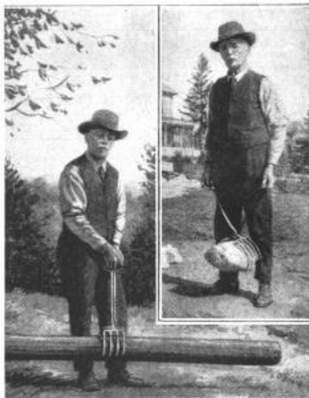
Quebec Farmer's Invention That Saves Stooping to Pick Up Light Loads in Farm Work: Left, Lifting a Log; Above, Raising a Stone
