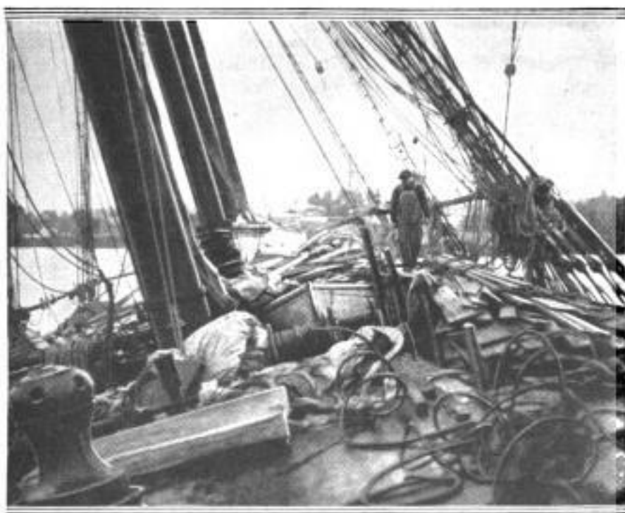
View of the Deck, Illustrating the Confusion Resulting from the Shifting of the Deck Cargo: One can Readily Imagine the Dangers and Difficulties of the Crew When the Seas Swept the Loose Lumber across the Deck or Overboard
