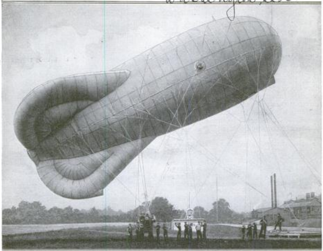
Captive Balloon Equipped for Protection against Lightning and Static Electricity: The Cone-Shaped Discharger on the Topmost Part Connects, through Flat Braided Copper-Wire Conductors around the Bag, to the Haul-Down Cables Which are Grounded to an Iron Pipe
