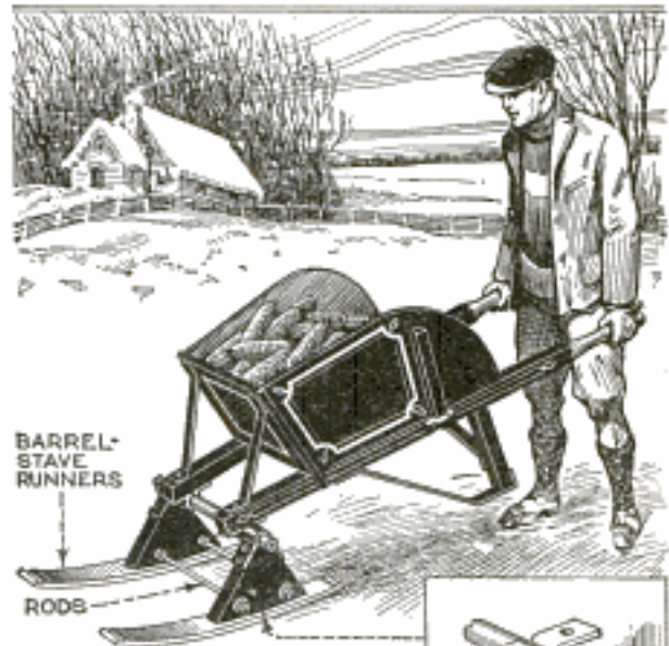
By Substituting a Pair of Runners for the Wheel of a Barrow, It Is Easier to Push a Load through Snow
