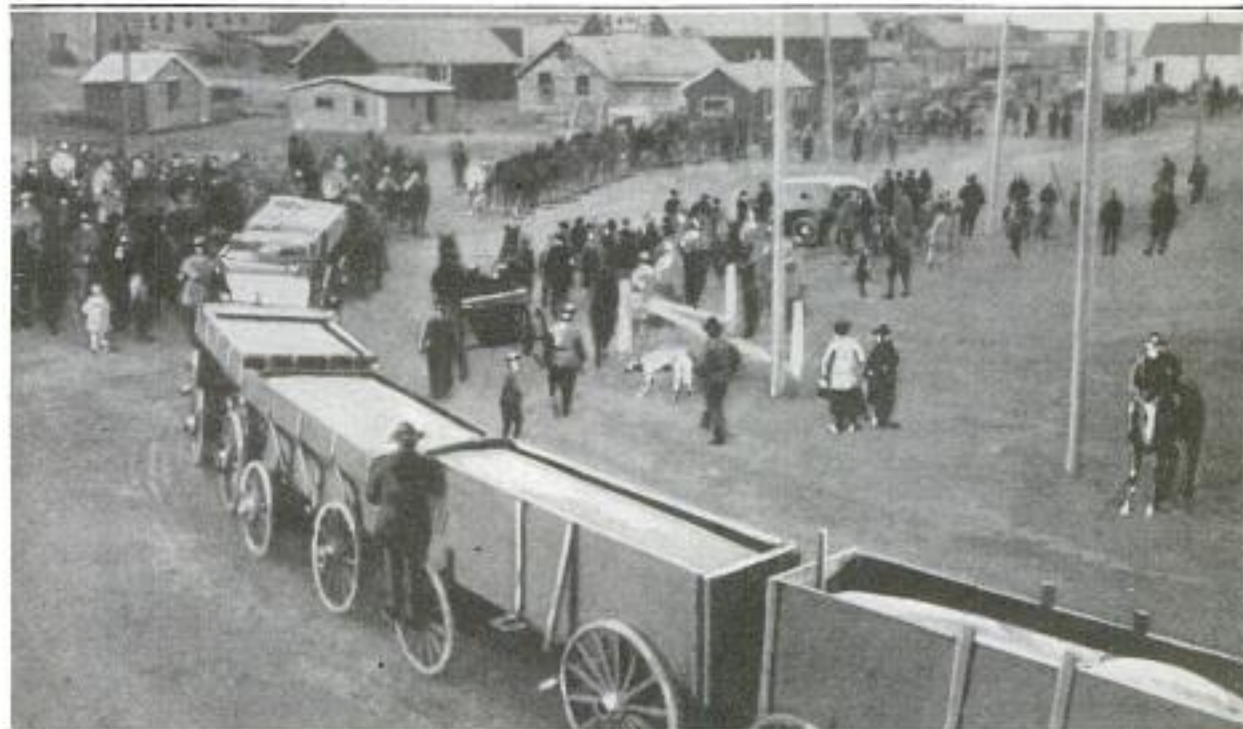
The Wagon Train Entering Vulcan: In Turning the Corners Encountered from This Point On, the Driver Swung the Hind Teams over the Hauling Cable, and Forced These Teams to Pull the Other Animals Until They, Too, were Headed in the Direction Desired
