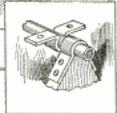
By Substituting a Pair of Runners for the Wheel of a Barrow, It Is Easier to Push a Load through Snow
