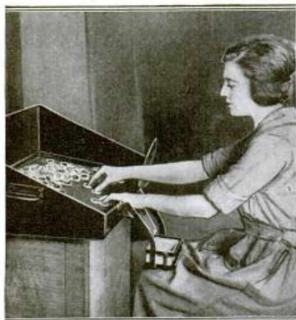
A Special Tray with Chute for Rapidly Counting Small Machine Parts and Filling Boxes with the Proper Number
