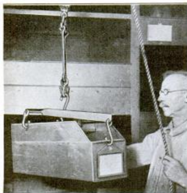
Heavy-Metal Shelf Box being Handled by Means of Block-and-Tackle Outfit, to Facilitate Lifting
