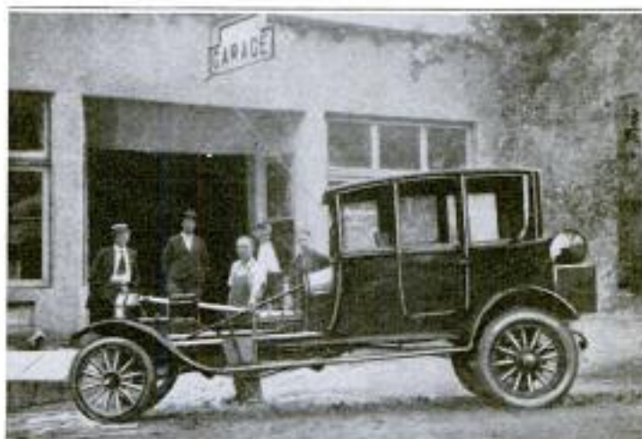
Standard Lightweight Automobile with Two Motors Instead of One: The Motors Are in Tandem upon an Extension of the Chassis That Increases the Wheel Base by About 38 Inches
