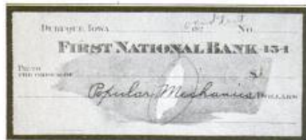
Result of Test in Which Ordinary Ink was Removed from a Check, While a Name Written with a New Ink was Not Affected
