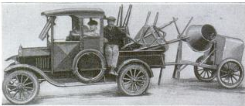
Concrete Mixer Mounted on a Rubber-Tired Two-Wheeled Truck, Which can be Hauled behind an Auto Truck at a 30-Mile Pace Instead of the Usual 10 Miles an Hour
