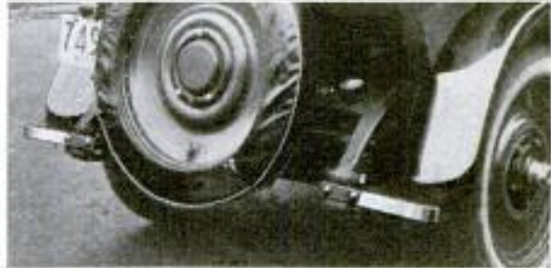
Only a Wrench is Needed to Install These Bumpers Which, though Light, Afford Adequate Protection for the Fenders
