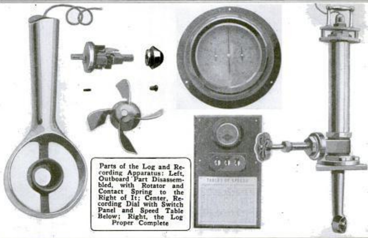
The Electric Log, Greatly Exaggerated in Size, as Installed in a Ship
