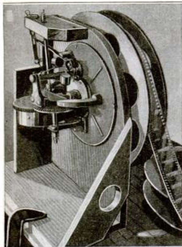
Left: Rear View of Film-Rewinding Machine, Showing How the Phonograph Motor is Attached. Right: Front View, Showing Reel in Place
