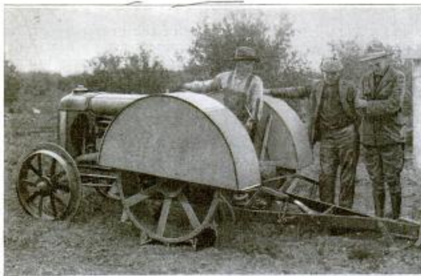
Subsoil-Plow Attachment Adapted for Use in Connection with Small Tractors, Which can be Adjusted to Pass over Obstructions and for Depth
