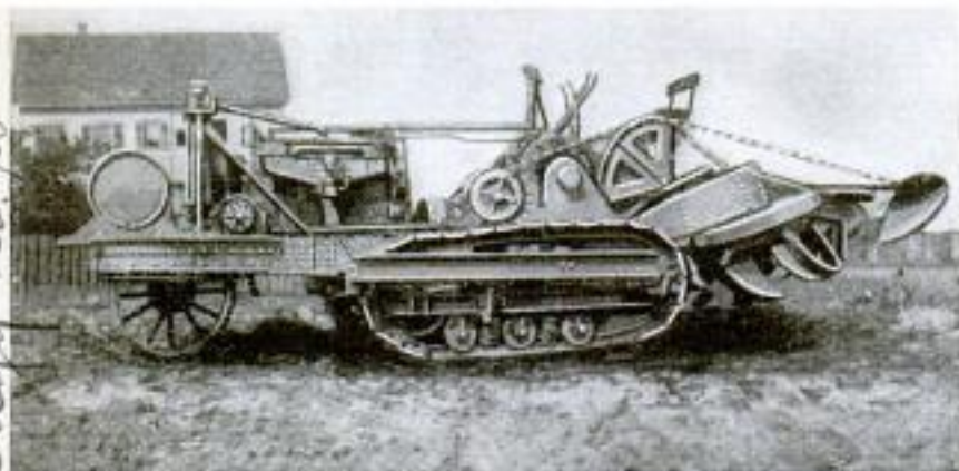
Side View of Powerful Machine Recently Built for Tillage of Sugar-Cane Soil in Porto Rico: Note Inclined Plow Frame
