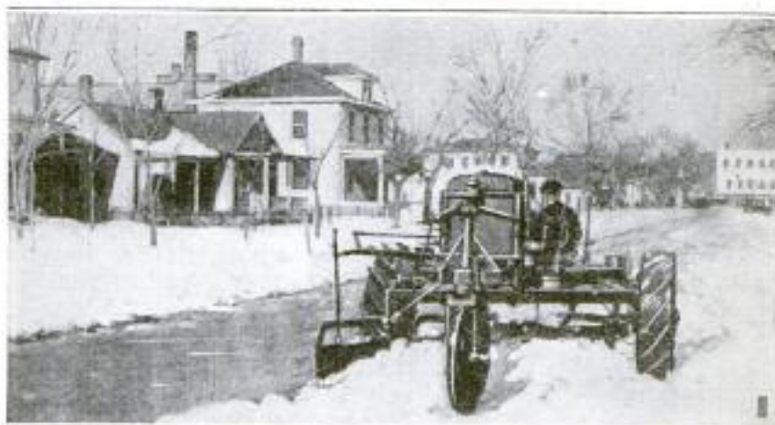
A Tractor Used to Clear the Snow from the Streets in a Kansas Town after a Heavy Snowstorm: The Work was Accomplished by One Man at the Rate of Three Miles per Hour
