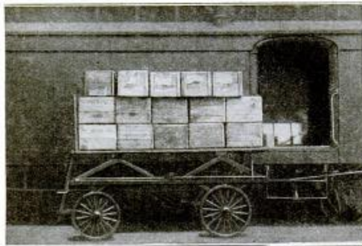
Above: New Station Truck Raised to Height of Floor in Baggage Car. Right: Man in the Act of Elevating the Truck Floor, Which can be Raised and Lowered through a Range of 18 Inches
