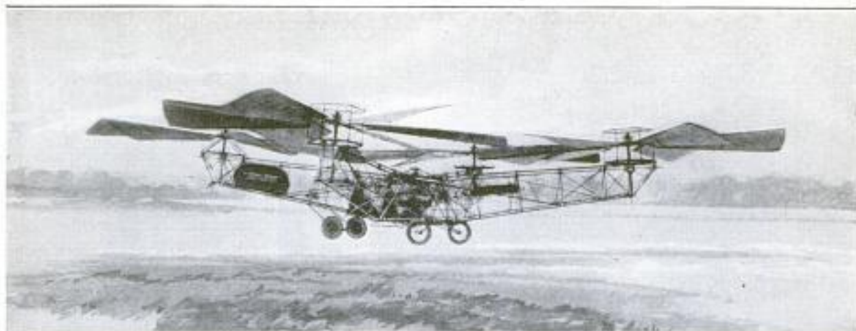
Latest Flying Machine of the Helicopter Type Just After It had Taken Off from the Ground in One of Its Recent Trial Flights: The Machine Has Four Six-Bladed Propellers, Each with a Lifting Capacity of About 1,000 Pounds
