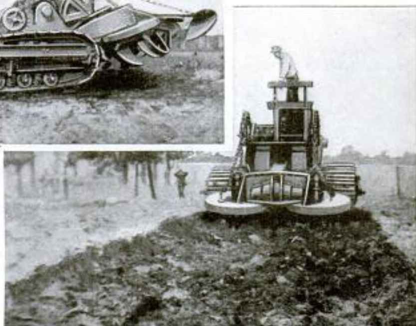
Rear View of Tillage Machine in Operation: It Plows More than the Width of the Machine and So does Not Travel over the Freshly Broken Ground
