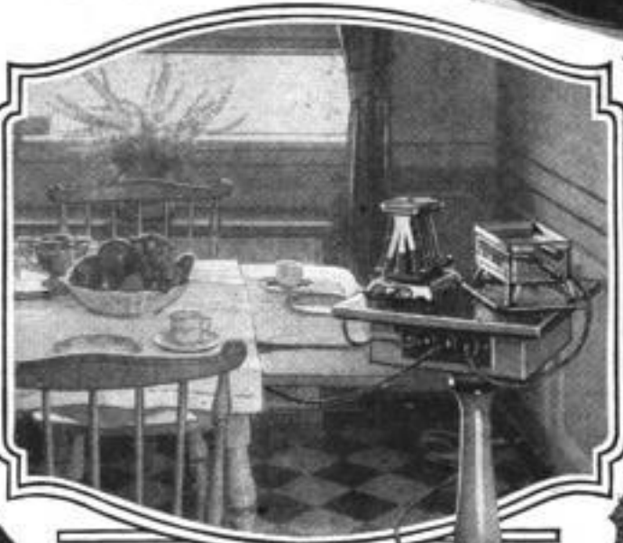
Portable Wired Stand That Has Three Electric Outlets for the Attaching of Various Electrical Appliances, and may be Easily Moved About
