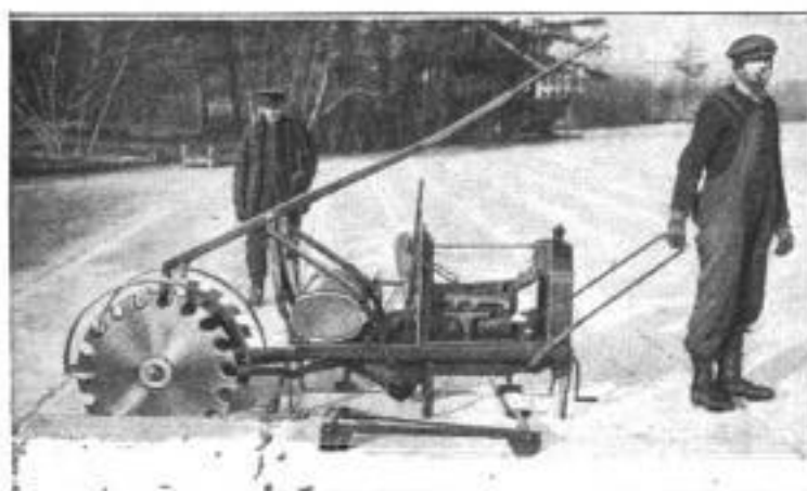
Ice is Cut and Grooved with This Rig, Driven by a Dismounted Auto Engine. The Large Lever is Used to Raise or Lower the Saws
