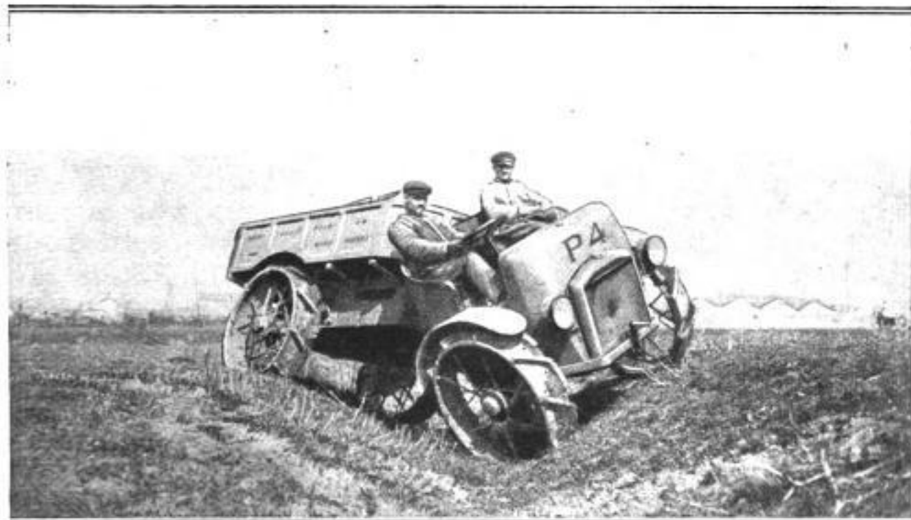
Italian War Tractors of This Type are being Converted into Truck Tractors for Agricultural Purposes. Note the Angle of the Front Axle as Compared with the Rear Axle, Made Possible by the Swiveled Action between the Two Frame Sections
