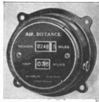
Recording Unit of the Air-Distance Measuring Apparatus for Airplanes
