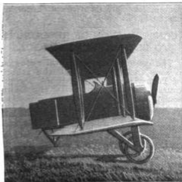
Tailless Airplane, in Which Longitudinal Stability is Automatically Obtained by Wings of Special Shape
