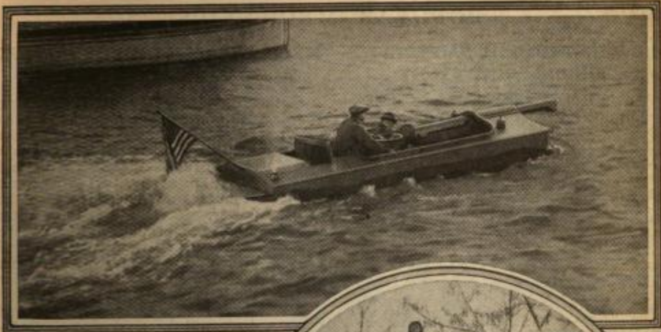
Above: The Armored Truck Seen Crossing the Hudson River at a Speed of about 20 Miles an Hour. Right: Front View of the Armored Truck as It Climbed to a Height of 100 Feet up the Palisades on the New Jersey Side of the River. For This Kind of Work the Continuous-Tread Is Necessary, and This can be Seen on the Wheels. Below: Armored War Truck without the Continuous-Tread Attachment. The Rear Set of Wheels does Not Touch the Ground When the Machine is Running as a Truck on Smooth Level Ground. The Gun Carried by the Car Is a 75-Millimeter Fieldpiece of the Type Made Famous by the Late War
