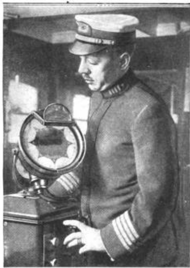
Gyroscope Compass, Which Automatically Makes Electrical Connections and Forms the Controlling Element of the Steering Gear for Ships
