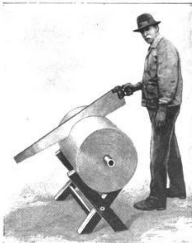
Four-Foot Handsaw Which was Specially Designed to Cut Rolls of Paper 24 Inches in Diameter
