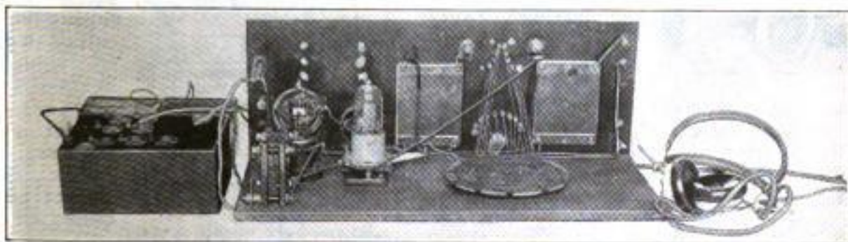
Above: Front View of Completed One-Step Receiver. Center: Details of Wiring, Assembly of Instruments, Method of Tapping Coil and Battery, Aerial and Ground Connections. Below: View of Rear of Completed Instrument; a Jack is Used for the Phones Instead of the Binding Posts Shown in the Drawings
