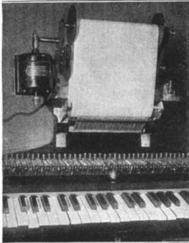
COPYRIGHT, KEYSTONE VIEW CO. Above the Movable Superimposed Keyboard Is the Musical-Typewriter Mechanism, Showing the Type Bars and the Motor-Driven Paper Roll
