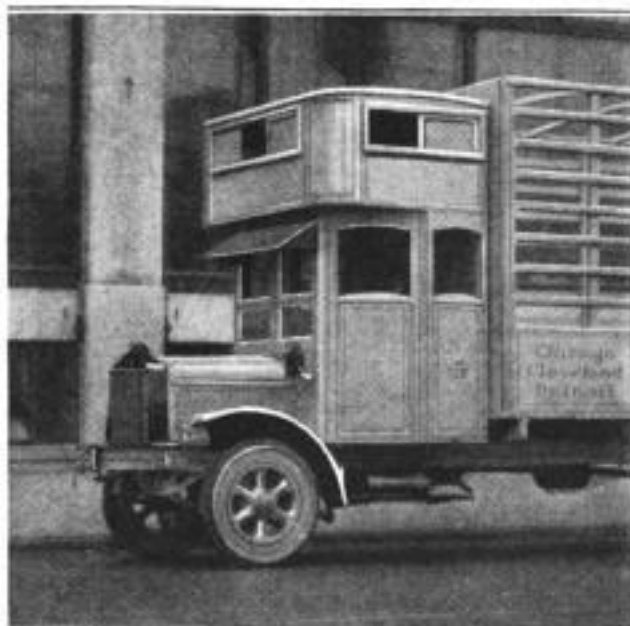
Truck Which Makes Long Hauls, Showing the Sleeping Compartment Built above the Driver's Seat for the Man off Duty
