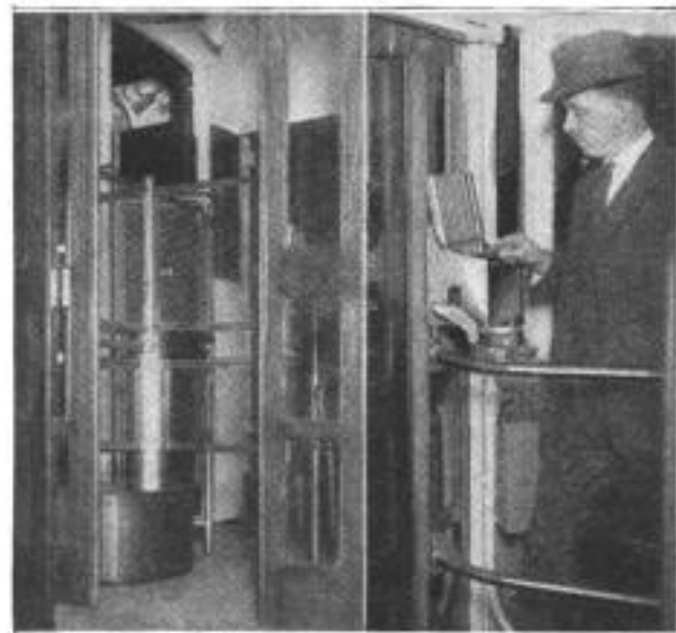
Equipment Used on New York "Pay-as-You-Leave" Car. Left: The Exit Turnstile Which Automatically Unlocks When a Nickel is Inserted. Right: A Near View of a Change Machine
