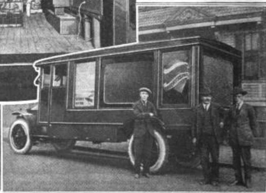
Above: Interior of the Large Motor Truck, Which Contains All the Apparatus Necessary for Giving Three Motion-Picture Shows at One Time. Besides the Triple Projector, There Is a Storage Battery and a Two-Kilowatt Generator That Charges the Battery in Two Hours. Right: Exterior View of the Truck, Showing the Rear Screen and One of the Side Screens
