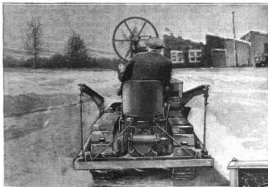
Above: Rear View of Endless-Tread Type of Tractor, Fitted with New Snowplow Rig, Intended for Use on Country Roads and City Streets Where Snowfall is Not Excessive. Right: Side View of Tractor Snowplow in Operation, Showing One of the Long Elevating Levers on the Side
