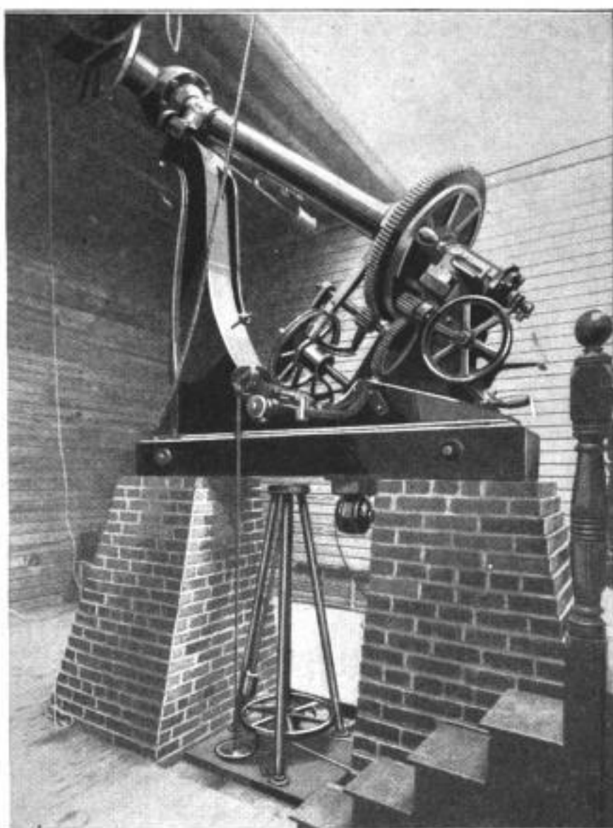
View Showing the Operating Mechanism of the 26-Inch Equatorial Telescope at the Naval Observatory, with the Old Friction-Drive Clock Mechanism Used for Photographic Purposes
