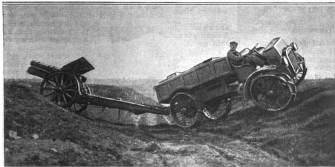
One of the Italian War Tractors of a Type That has been Lately Modified to Suit More Peaceful Pursuits, Shown Carrying Ammunition, and Hauling a Piece of Field Artillery over Rough Ground: All Four Wheels Respond to the Action of the Steering Gear
