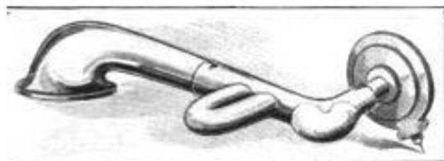
Two of the Interference Tubes Shown Fitted in the Main Tube between the Reproducer and the Tonearm of a Talking Machine
