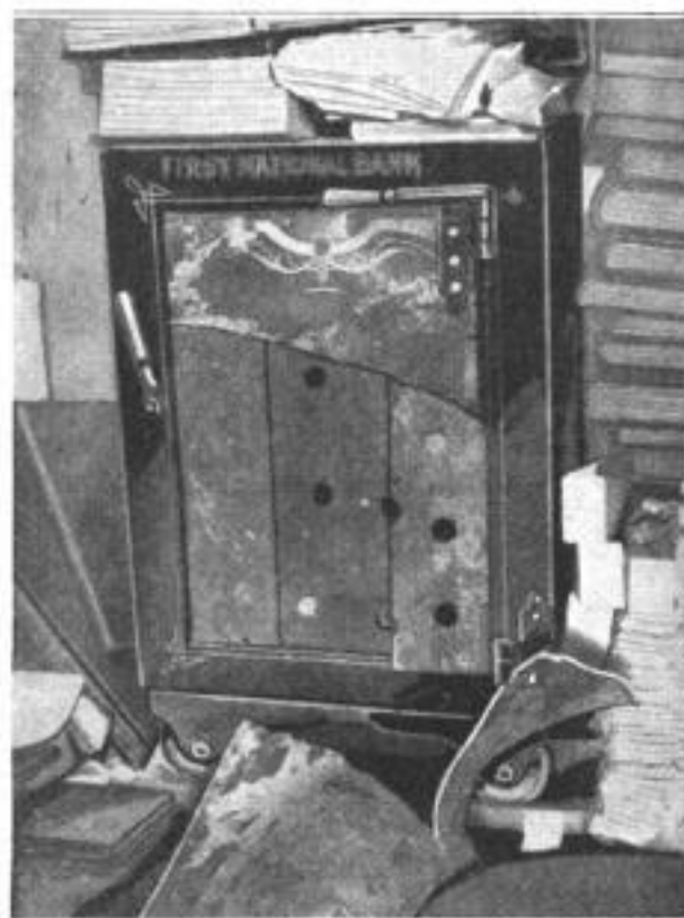
Bank Safe Which, Owing to Its Scientific Construction, Resisted the Efforts of Burglars to Blow the Door off Its Hinges
