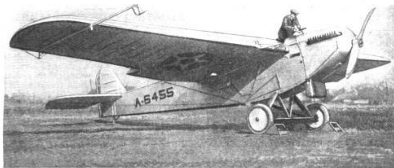
First All-Metal Airplane Which has been Accepted by the United States Navy and Which will be Used for Observation Purposes: This Machine Is of the Monoplane Type and So Constructed That It may be Mounted on, and Catapulted from, the Turret of a Battleship
