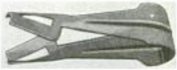
Top: Cleaner Shown Inserted in an Open-End Spark Plug. Bottom: Cleaner, Illustrating Its Simple Construction
