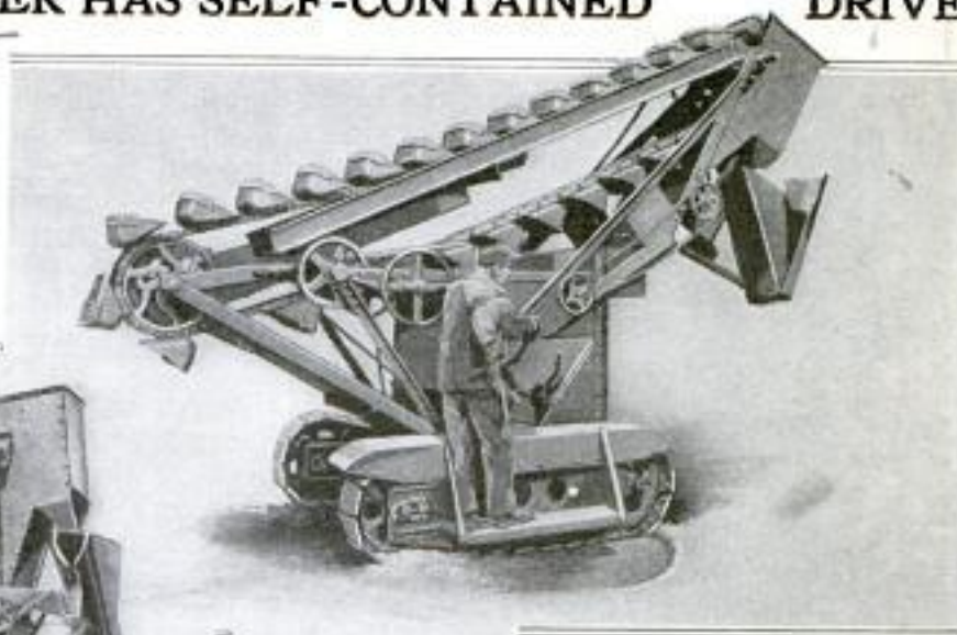
Elevator in Position for Transporting the Self-Propelling Loader, Which is Driven by the Same Motor as the Elevator
