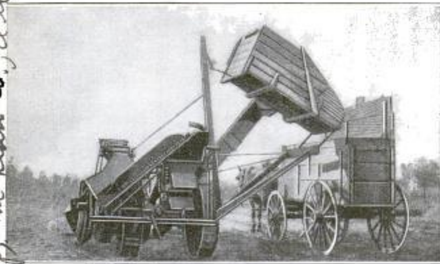
This Homemade Combination Corn Picker and Tractor Harvests and Loads 10 Wagonloads of Corn in 10 Hours, and is Operated by One Man. It is Built from Parts of Automobiles and Various Other Equipment
