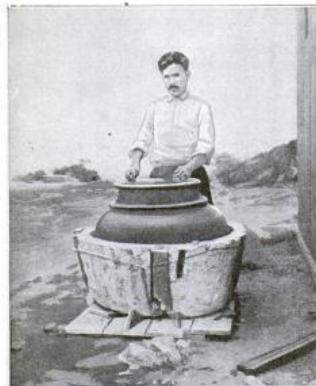
Earthen Vessel in the Process of Manufacture, Showing How the Base is Moldered Inside of a Mortar and the Top Shaped by Hand
