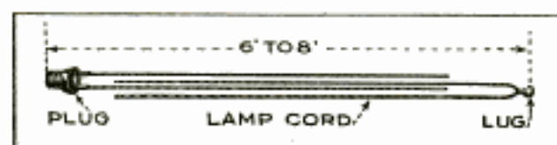
An Inexpensive but Satisfactory Attachment That Enables the Amateur to Use the Lighting Circuit as an Indoor Antenna
