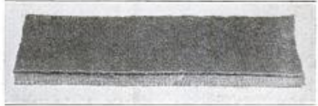
Piece of Six-Ply Material Made from Chemically Treated Cotton Fabric, That Is Suitable for Shoes, Trunks, Belting, and the Like
