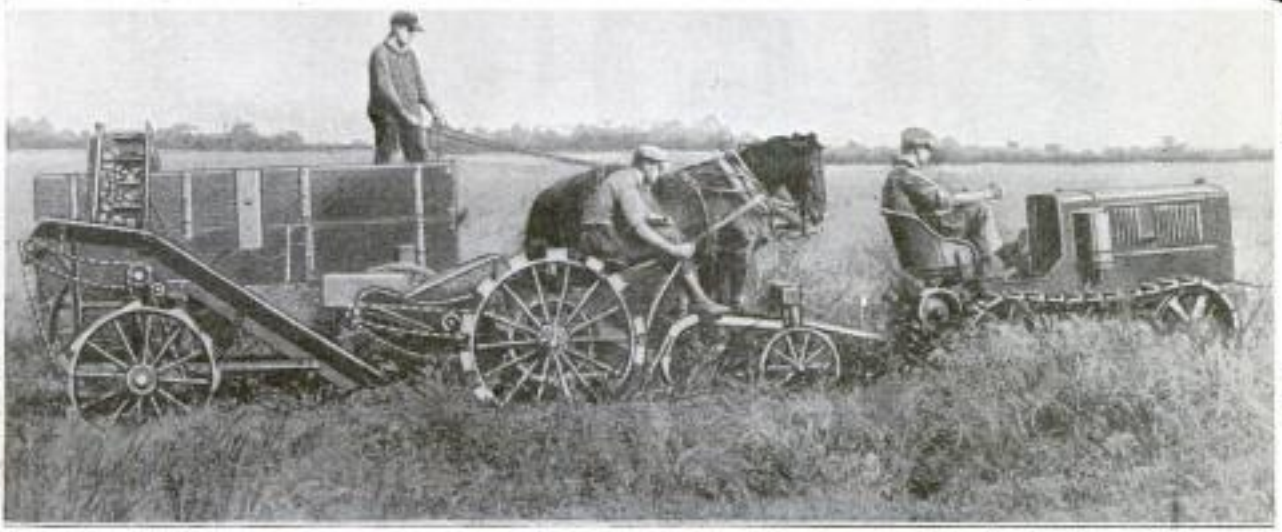
Combined Potato Digger and Loader Drawn by a Tractor and So Arranged That the Potatoes can be Dug and Loaded Simultaneously into an Accompanying Wagon: This Combination, Moving at a Speed of Three Miles an Hour, can Dig and Load Approximately 800 Bushels in a 10-Hour Day
