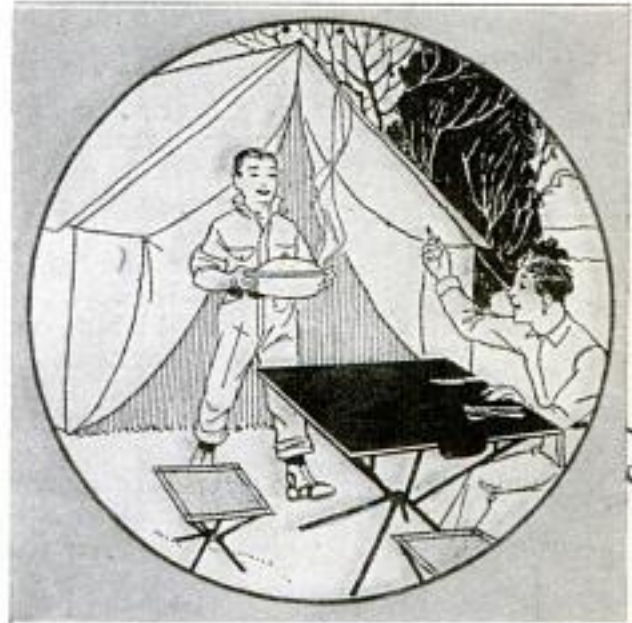
Camp Table That Folds So as to Make a Neat Case, 27 Inches Long, 7 Inches Wide, and 2 Inches Thick: Chairs are Carried Inside
