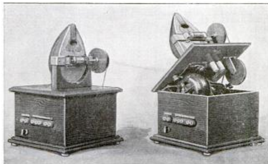
Two Views of an Adaptation of the Attraction Principle, in Which the Sound Box of a Mandolin, with Other Equipment, is Used for the Transmission of Musical Tones
