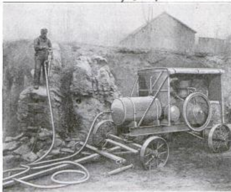
Portable Air-Compressor Unit Driven by a Gasoline Engine, Arranged to Give a Power Impulse to Each Compression Stroke of the Compressor
