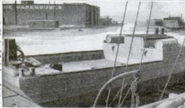
Top: Nonsinkable Barge Made of Balsa Wood Obtained from Life Preservers, Shown High and Dry on Land. Above: A View of the Completed Barge in the Water
