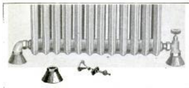
In Connection with the Floor Supports, a Wall Bracket Prevents the Legless Radiator from Tipping. One of the End Supports and the Center Rest are Shown in the Foreground.
