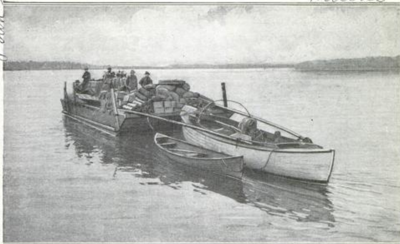
First Steel Scow to be Used on the Lakes of Maine in Connection with the Lumber Industry: This Scow Has a Load Capacity of 30 Tons, and is Pushed through the Water by the Powerful Motorboat at a Speed of Six Miles an Hour in Calm Weather
