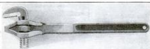
One of the Larger-Sized Wrenches, with Four Sets of Teeth for Using the Wrench in Four Different Ways by Adjustment of the Movable Jaw
