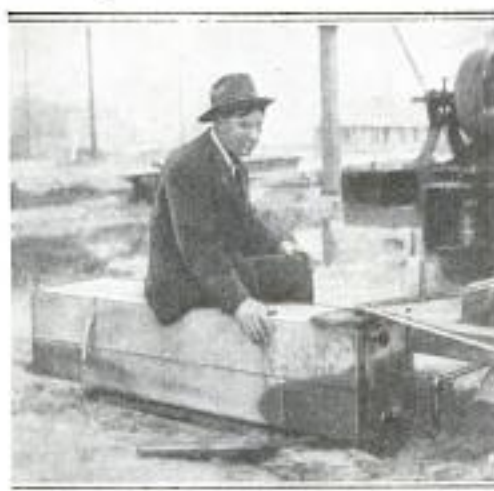
An Old Tank Taken from a Dismantled Launch, Which has been Fitted with a Glass Level-Indicating Tube and is Now Used as the Gasoline Reservoir for the Engines
