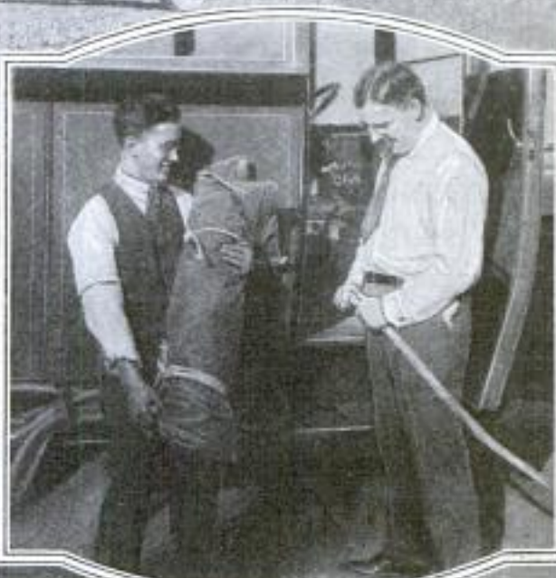
The Man on the Left is Holding the Auxiliary Folding Bed Which is Carried on the Running Board, While Just behind Him may be Seen the Loops of the Long Hose Used for Obtaining Water from Streams or Lakes
