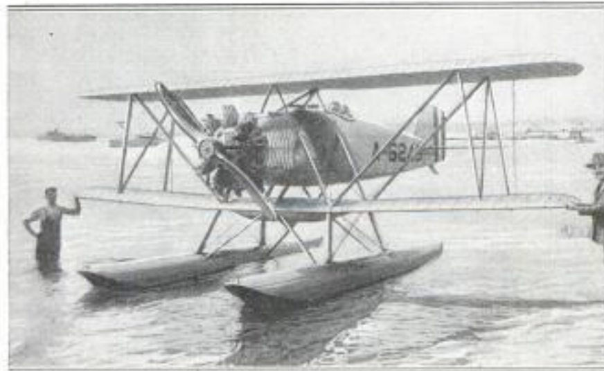
New Shipboard Type of Airplane Equipped with Pontoons for Water Service: Power is Furnished by an American Radial Air-Cooled Motor
