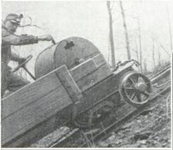
Above: Safety Car near the Top of Incline, Stopped Automatically after Running 25 Feet with the Hoisting Rope Cut. Upper Left: Side View of Car with Hood Open, Showing Details of Safety Device. Right: Car on Grade with Hoisting Rope Disconnected
