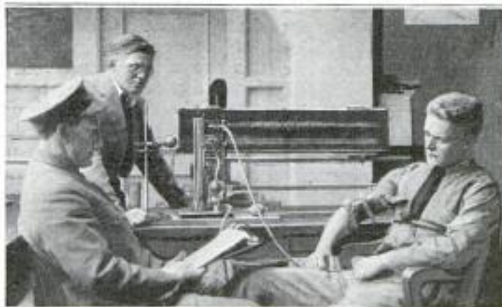
A Prisoner being Tested by the "Lie Detector," Which Records the Variations in Heart Action and Breathing, as the Suspect is Plied with Questions
