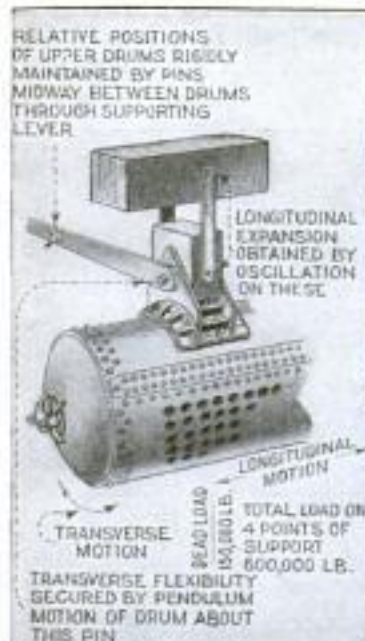
Left: Diagram Illustrating Toggle-Suspension Hangers, Which Permit a Total Play of 1\frac{1}{2} Inches to Take Care of Drum Expansion. Right: Immense Steam-Collecting Drum of Boiler, Rated at 2,650 Horsepower
