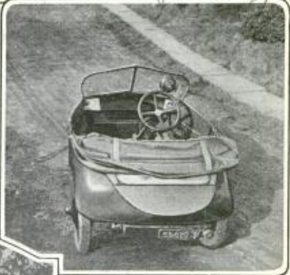
The illustration above and to the left gives a good idea of the mobility of the car. By noting the lines made in the roadway it is seen that the car is able to turn completely around with the third wheel remaining practically in a fixed position. Above: Rear view of the car, showing luggage compartment, collapsible top, and controlling mechanism. Below, left: Removable section taken out, showing the easily accessible motor, a 10-horsepower two-cylinder design
