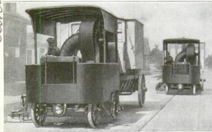
Two of the Huge Vacuum-Cleaning Outfits Which are Used on the Streets of St. Louis, Showing the Large Suction Fan Mounted on the Motor Truck, and the Compartment for Refuse on the Trailer
