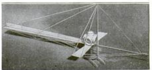
This Landing-Field Indicator can be Seen from Normal Flight Heights, at a Range of Five Miles by Day and 12 Miles at Night
