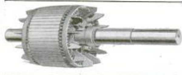
Armature with Projecting Fan Blades at Each End That Act as Blowers, and Expel Dirt or Dust through Openings in the Frame of the Motor
