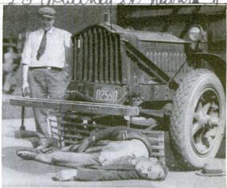
Left: Self-Acting Automobile Bumper Installed on a Motor Truck, Showing How the Lattice Gate Drops When Pressure is Exerted against the Bumper Rod. Right: Another View of the Apparatus, Demonstrating How the Gate Prevents the Body from being Crushed by the Truck Wheels
