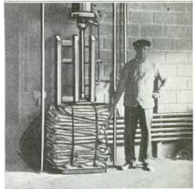
Compressed-Air Ram Used in Cement Plants for Baling Empty Bags: At Least a Hundred Bags can be Baled at One Time in This Machine
