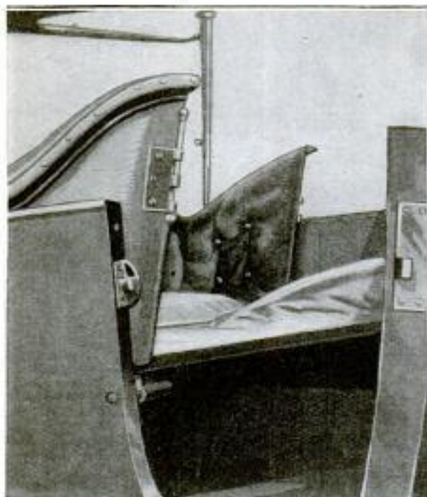
The Back of the Front Seat is Cut at Sides and Bottom So That It can be Lowered When the Occupants Desire to Use the Car for Sleeping
