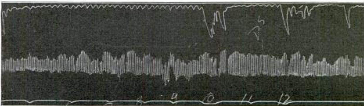
Graphic Record from Lie Detector: Top Line Represents Breathing, Second Line Blood Pressure, and on the Bottom Line is Indicated the Instant of Asking Each Question. Note the Irregularities in the Lines Which Indicate That Questions 10 and 12 have been Untruthfully Answered
