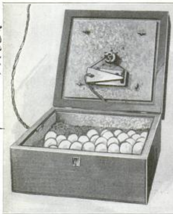
Left: Electrical Incubator with Its Upper Half Closed, Showing the Triangular Contact Breaker That Acts as a Thermostat to Maintain a Uniform Temperature of 103 Degrees. Right: Upper Half with Its Cover Down, Showing the Heating Lamp, and the Bright-Metal Concave Reflector with Cotton-Batting Insulation
