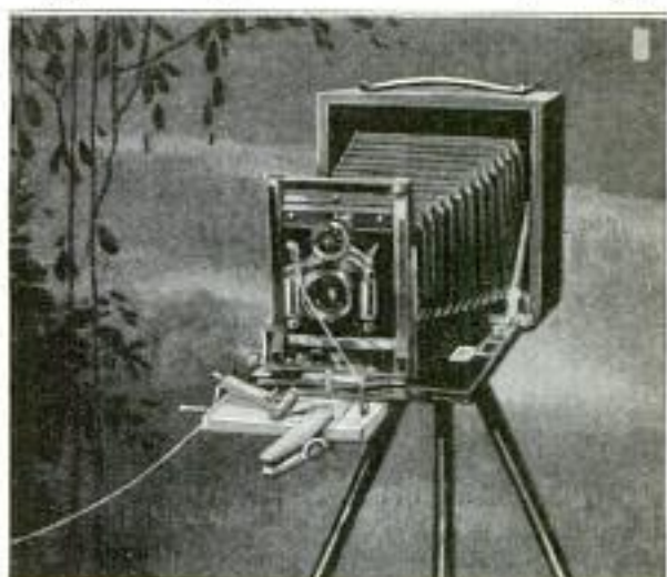
A Common Mousetrap Attached to a Camera may be Used to Trip the Shutter Automatically When Photographing Wild Birds and Animals
