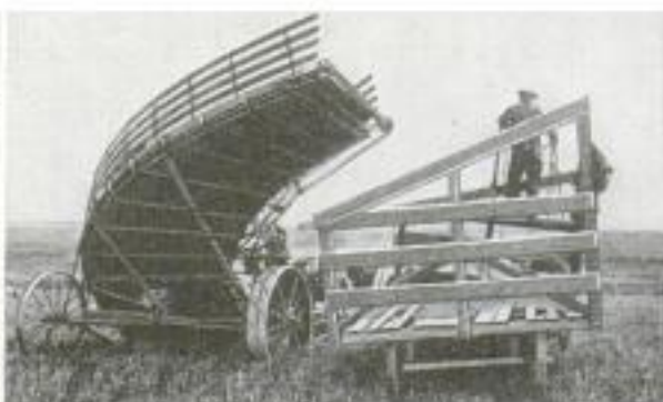
Left: Loading Machine, Showing How the Implement Picks the Shocks of Grain or Hay from the Ground and Carries Them up the Incline for Deposition on the Wagon Which is Driven Alongside. Right: Rear View of the Loading Machine, Clearly Illustrating the 45° Curve in the Carrier
