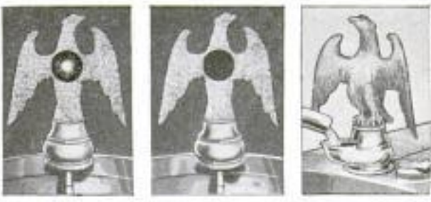
Three Views of Indicator, Showing Appearance from Driver's Seat at Normal Temperature and When Overheating Threatens, and from the Front with Filler Cap Open
