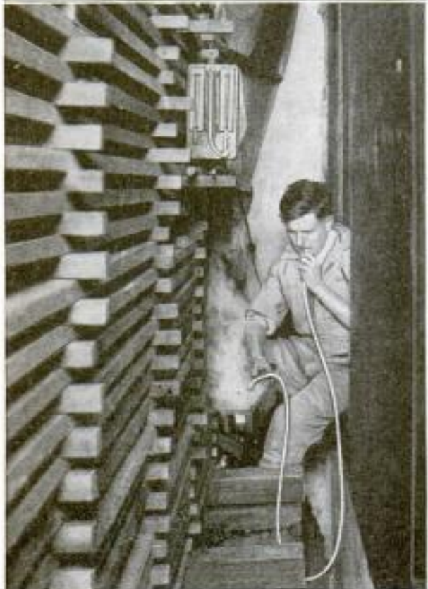
Lumber Dry Kiln, Showing Apparatus for Blowing Hydrochloric Acid across Ammonia to Produce Fumes for Determining Whether the Air is Circulating in a Proper Manner
