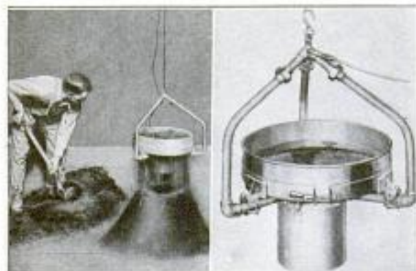
Left: Electric Sifter in Use as a Riddle for Molding Sand. Right: Close-Up of Sifter Which can be Inclosed for Liquids
