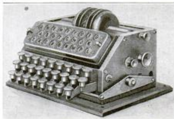
The Coding Machine Complete: The "Key Wheel" is Seen Clamped on Top. Below Is the Receiving Apparatus, Consisting of the Letters of the Alphabet on Opaque Glass, Illuminated from Behind, and at the Bottom the Sending Keys
