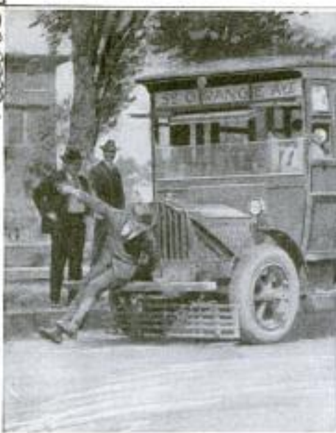
Left: Self-Acting Automobile Bumper Installed on a Motor Truck, Showing How the Lattice Gate Drops When Pressure is Exerted against the Bumper Rod. Right: Another View of the Apparatus, Demonstrating How the Gate Prevents the Body from being Crushed by the Truck Wheels
