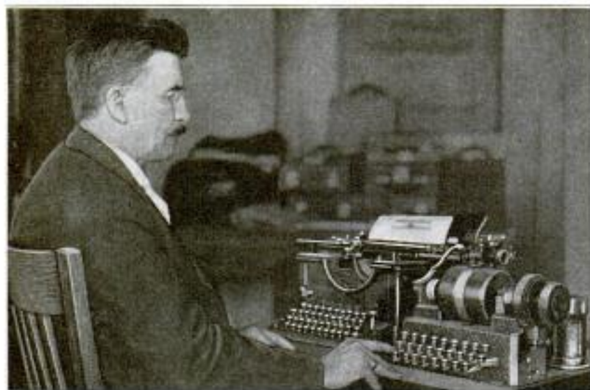
The Inventor is Shown Here with His Code-Sending and Receiving Machine, Which is Equipped to Operate Either by Wire or by Radio. The Machine, with the Proper "Key Wheel" Inserted, Translates the Coded Message from Any Similar Machine Immediately on Receipt. The Typewriter, to the Left, Gives an Idea of the Size of the Coding Machine
