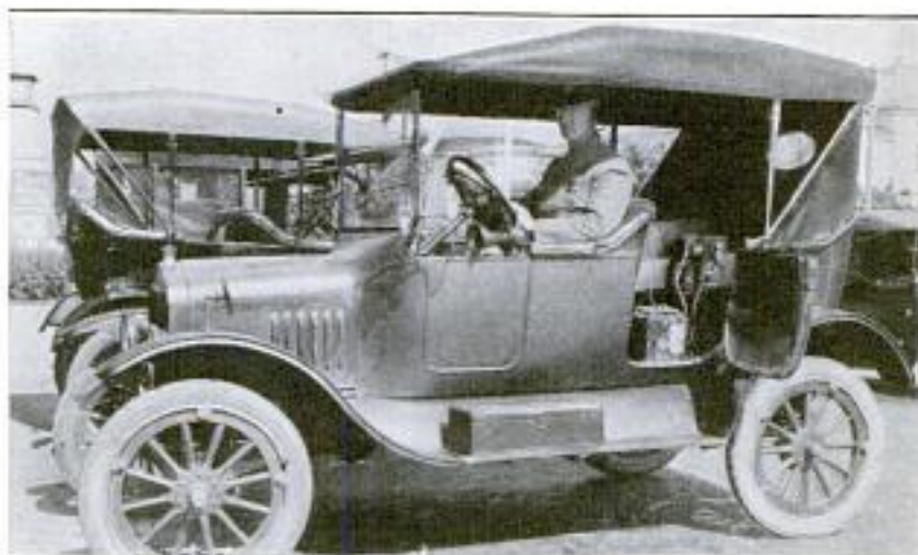
Berkeley Police Car Fitted with a Wireless-Telephone Outfit, with Which It is Expected Each Car will Shortly be Equipped: Note the Receiver on the Head of the Officer. The City of Berkeley is Reported to Have the Only Completely Motorized Police Force in the United States
