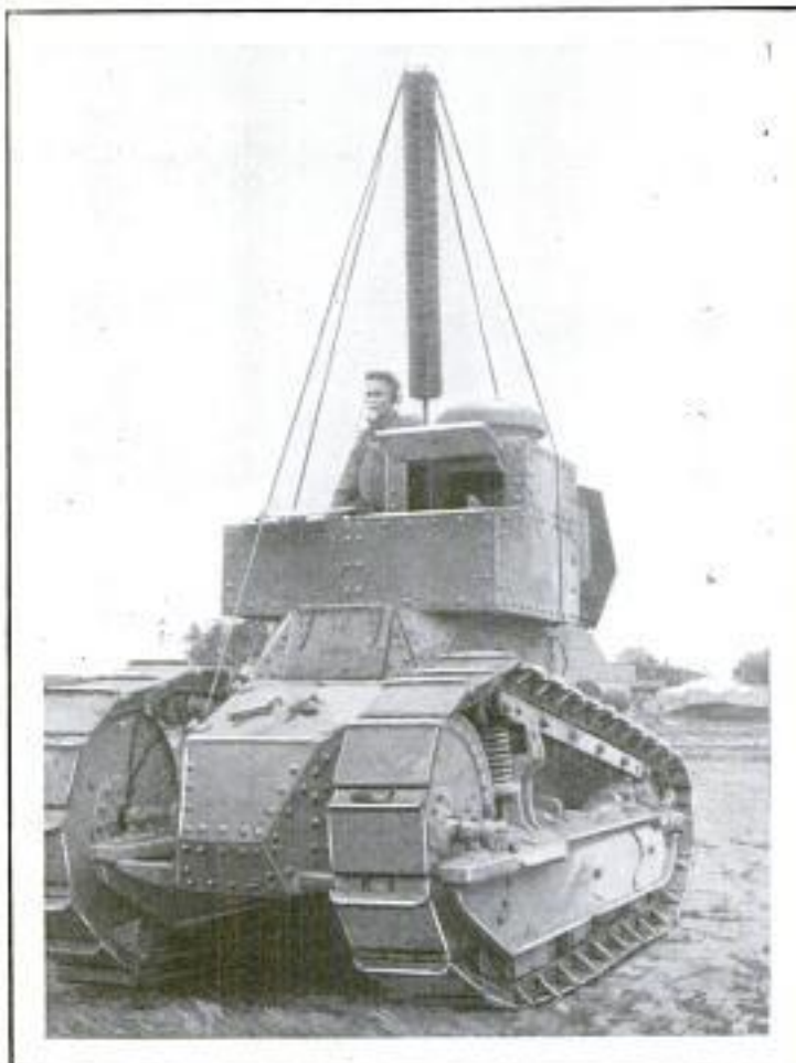
"Baby" Tank Which is Equipped with a Complete Radio Outfit. Having a Sending and Receiving Range of 25 Miles, Showing How the Perpendicular Antenna is Mounted
