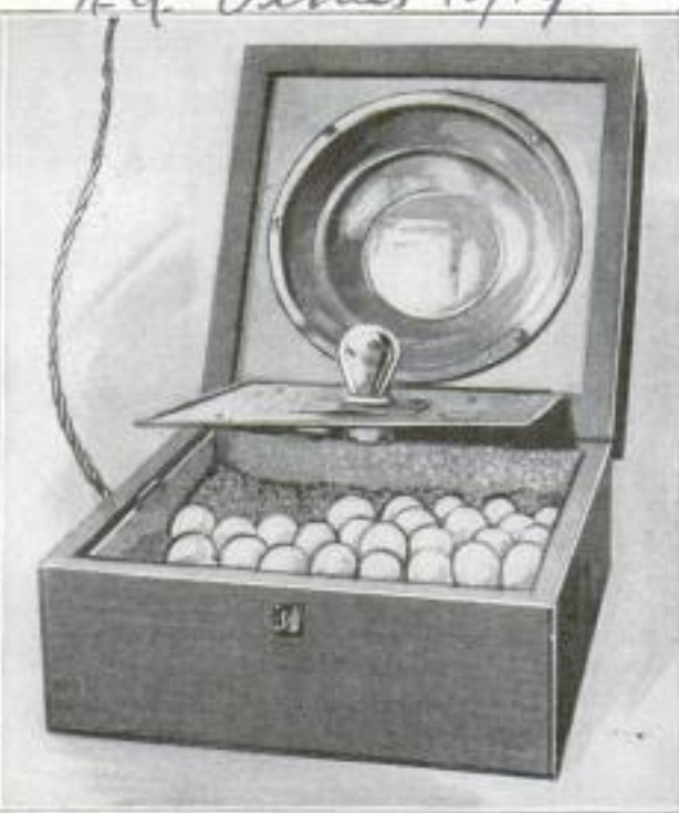
Left: Electrical Incubator with Its Upper Half Closed, Showing the Triangular Contact Breaker That Acts as a Thermostat to Maintain a Uniform Temperature of 103 Degrees. Right: Upper Half with Its Cover Down, Showing the Heating Lamp, and the Bright-Metal Concave Reflector with Cotton-Batting Insulation
