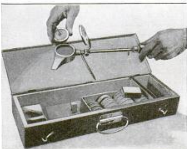
This Soldering Iron is Supplied with Heat from the Reaction of Chemicals
