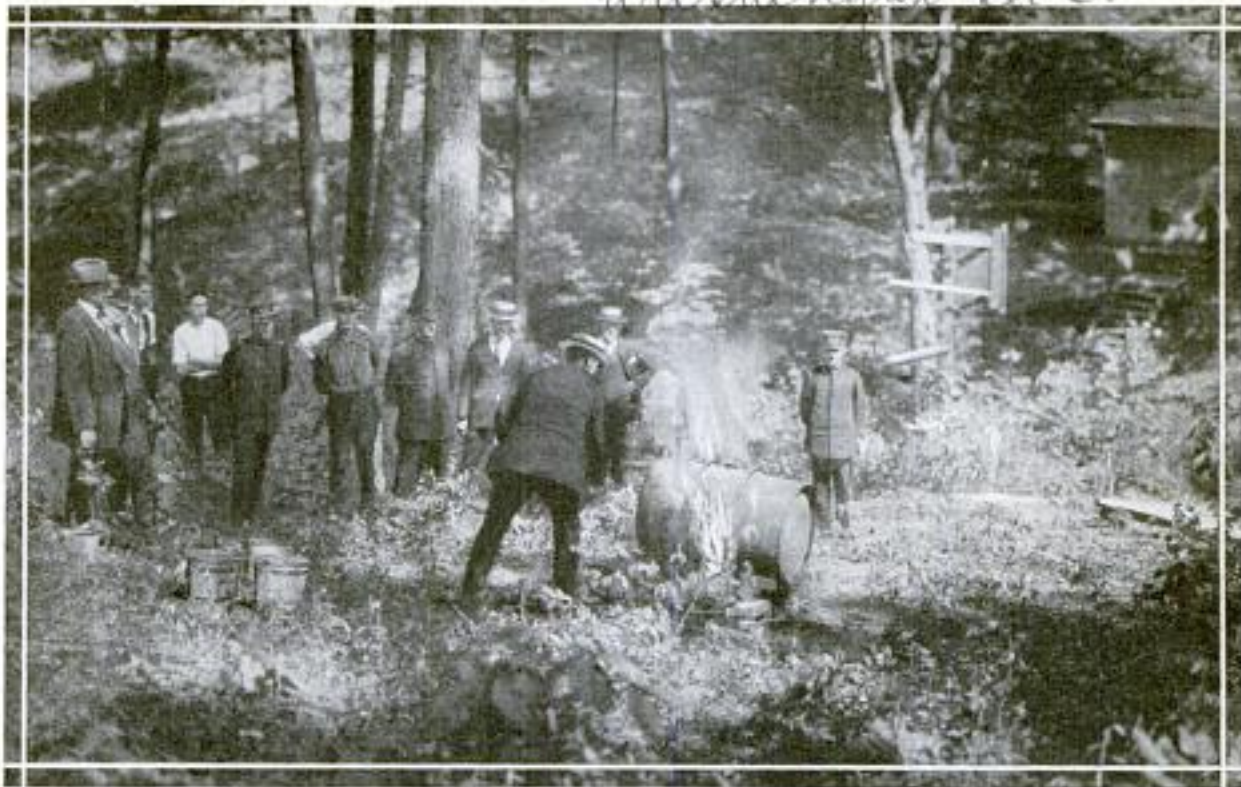
Test of Safety Venting Device on a 50-Gallon Drum, Containing 25 Gallons of Gasoline, before Government Officials: A Brisk Fire under the Drum Caused the Gasoline to Burn without Exploding
