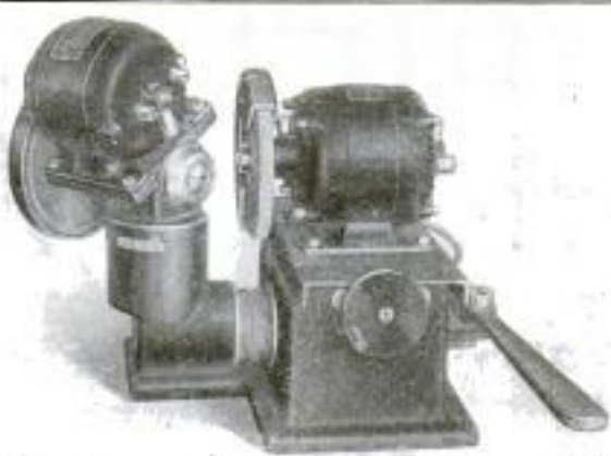
Valve Grinder with an Individual Motor for the Six-Inch Grinding Wheel, and Another for the Work Head, the Whole Occupying a Space of Two Square Feet
