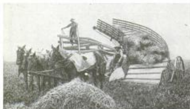
Left: Loading Machine, Showing How the Implement Picks the Shocks of Grain or Hay from the Ground and Carries Them up the Incline for Deposition on the Wagon Which is Driven Alongside. Right: Rear View of the Loading Machine, Clearly Illustrating the 45° Curve in the Carrier
