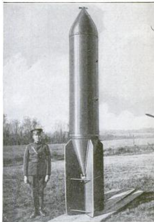
Largest and Most Powerful Demolition Bomb in the World. Made by the Ordnance Department: It Weighs 4,000 Pounds, and Dwarfs the Soldier Who is Standing beside It
