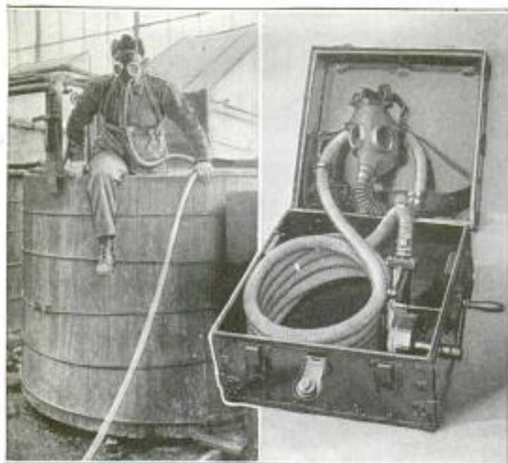
Left: Wearer of the Hose-Connected Gas Mask Climbing Out of a Chemical-Treating Tank after having Cleaned It. Right: Complete Apparatus Packed in Its Trunk, with the Rotary Blower in One Corner
