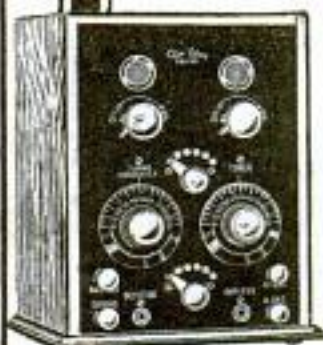
AIR-WAY Model "B" Complete Receiving Set, Long-distance vacuum tube outfit—detector and one-stage amplification.
