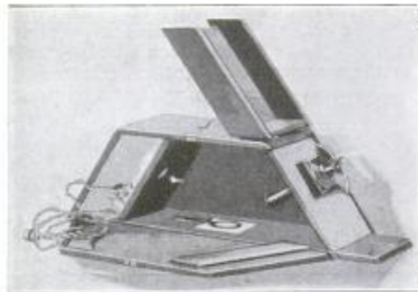
Instrument Used to Determine the Finish on Paper, Furniture, Automobiles, and the Like, by Analyzing the Reflected Light
