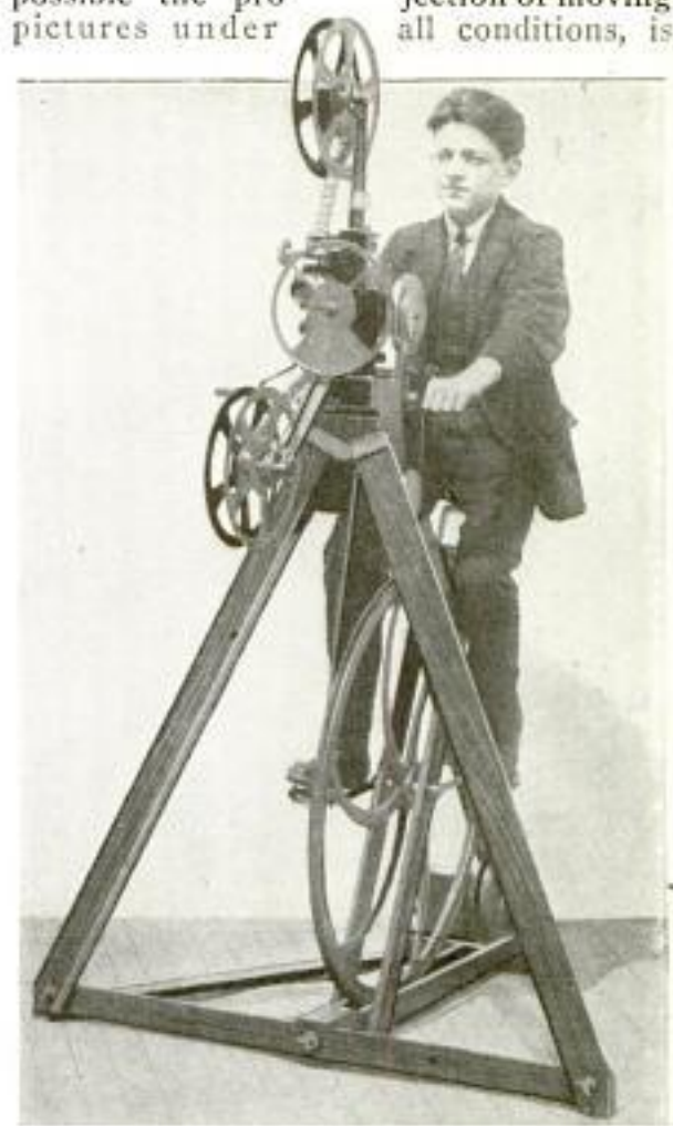
Pedal-Driven Moving-Picture Projector Which Generates Its Own Electricity: The Large Pulley Drives the Dynamo and Film Reel
