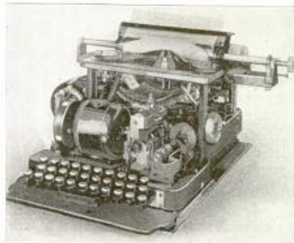
Central-Station Sending Machine of the Printing Telegraph Outfit, on Which the Messages are Typed in Page Form
