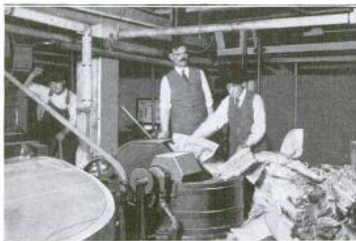
In the Center can be Seen the Large Vat Used in the De-inking Process and in Which Newspapers are Placed and Reduced to a Pulp; Then, to the Washing Solution in the Vat, is Added the Bentonite Which Removes the Ink from the Pulp
