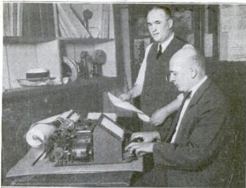
COPYRIGHT, UNDERWOOD & UNDERWOOD Sending Machine of the Printing Telegraph Outfit at Central Headquarters of the Chicago Police Department, with Which Page-Form Type-written Messages are Sent to 40 Outlying Stations
