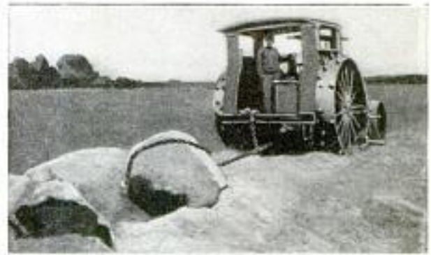
Pulling Heavy Boulders with a Tractor, Illustrating How the Hitch should be Made in Order to Enable the Tractor to Pull the Load Easily
