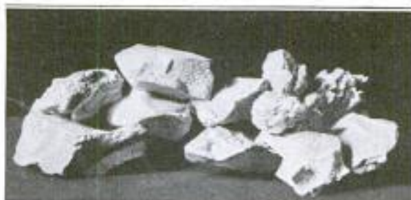
Lumps of Bentonite, Which Swells to Several Times Its Actual Size When Soaked in Water, Becoming a Soft Creamy Mass Like Corn-Meal Mush
