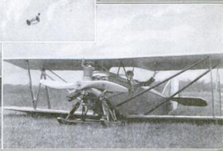
Above: Dropping the Wheel Landing Gear from a Plane in Flight. Left: Airplane Equipped with Combination of Regular Wheel Gear for Leaving the Ground, and Skids for Landing. Right: Making a Landing on Skids, Which can be Done in a Distance of About 50 Feet
