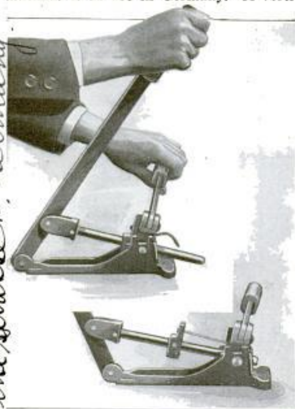
Nail-Straightening Device Shown Above with a Bent Nail in Place Ready to be Straightened by Swinging Back the Vertical Lever, as Shown Below
