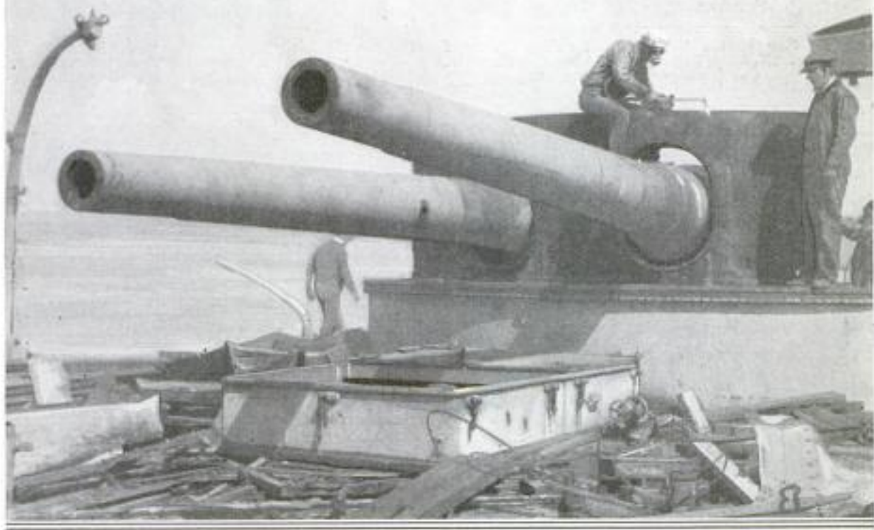
Above: Operator at Work Cutting Up One of the Eight-Inch Guns of the Old Cruiser "Brooklyn," with Torches Using City Gas Instead of Acetylene or Hydrogen. Guns of Scrapped Naval Vessels are Always Disabled before Sale. Below: Cutting Up the Inner Shell of One of the "Brooklyn's" Gun Turrets. Several Pieces of Eight-Inch Armor Plate, Taken from This Turret, can be Seen under the Gun at the Left. The "Brooklyn" Was One of the Ships That Took Part in the Defeat of Admiral Cervera's Fleet off Santiago, Cuba, in the Spanish-American War, and has Long Been Obsolete Like the Other Ships of the Famous American Squadron, Many of Which have Served as Targets for the Guns of Newer Men-of-War
