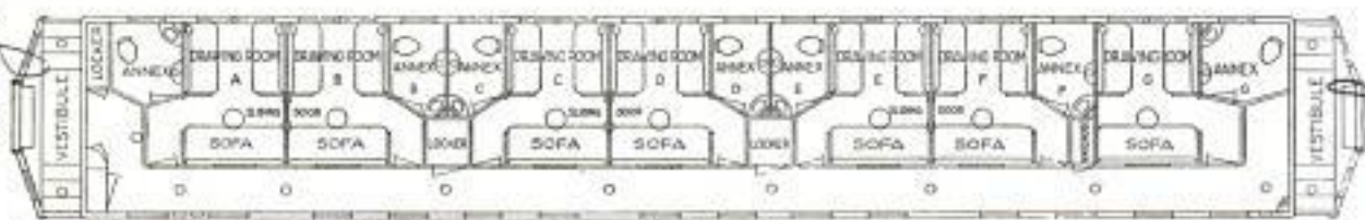
This Diagram of the Steel Sleeping Cars Soon to be Placed in the Transcontinental Service of the Santa Fe Railroad Shows How the Rooms are to be Arranged. Notice the Sliding Doors between the Drawing Rooms
