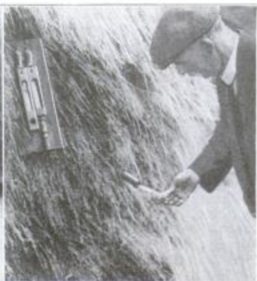
Left: Haystacks being Cured by an Air Blast from a Powerful Blower Fan Driven by an Electric Motor, Right: Taking the Temperature of a Haystack with a Thermometer Fastened to the End of a Stiff Wire
