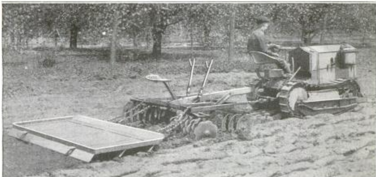
Clod Crusher and Leveler Chained to a Harrow Which is Hauled by the Small Tractor over a Plowed Field: It Crushes the Clods and Leaves the Soil Perfectly Level and Smooth. Three of the Bent Plates Are Sufficient for Most Kinds of Soil, But More can be Added
