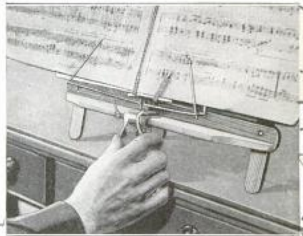
Device for Turning Over the Leaves of Sheet Music on a Piano or Other Music Stand: It is Operated with the Fingers and Thumb in the Manner Shown
