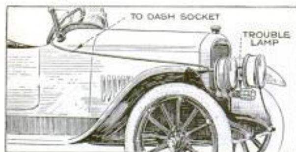
An Extension Trouble Lamp Fastened to the Underside of One of the Headlights Makes Night Driving Safe, and Prevents Arrest for Driving without Lights
