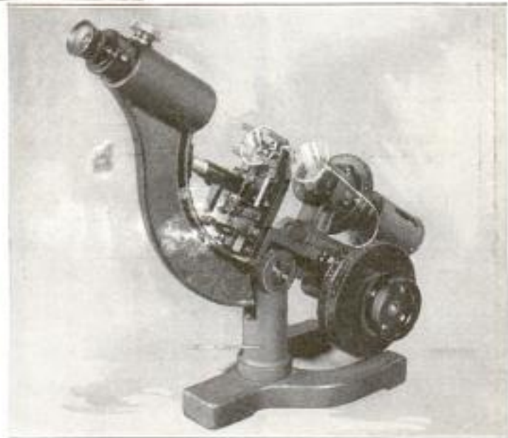
Above: The Inventor of the New Method of Testing the Accuracy of Optical Lenses is Here Seen with the Instrument He has Perfected. Right: Another View of the Instrument, Showing the Means of Holding a Pair of Spectacles
