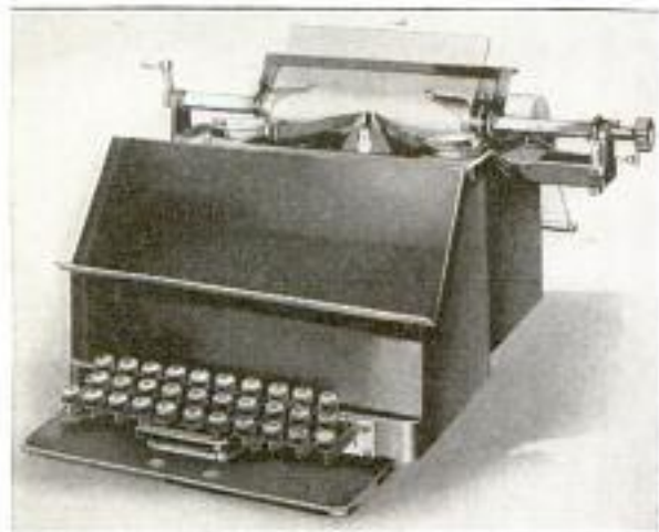
Printing Telegraph Apparatus of the Page-Form Type Which Performs the Double Function of a Sending or a Receiving Machine
