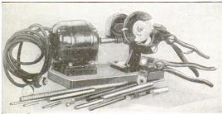
Portable Bench Saw, Weighing 40 Pounds, for Hard or Soft Material, That can be Run from Any Lamp Socket
