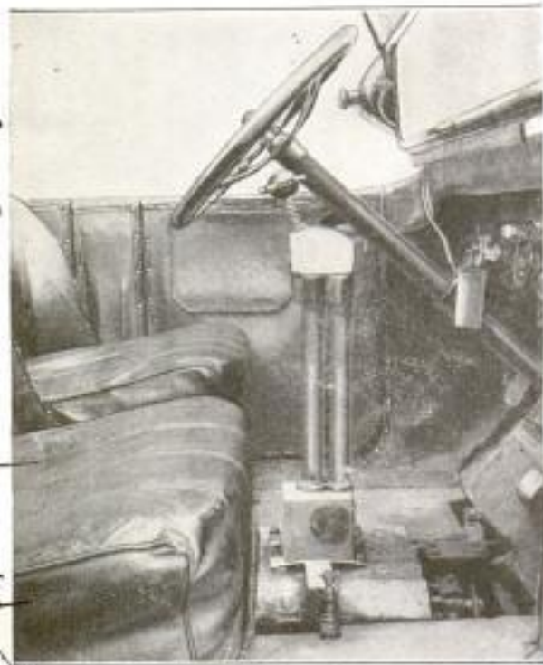
The Motor-Car Control, Mounted on the Transmission Case, is Operated by the Lever with the Spherical Head at the Side of the Steering Wheel
