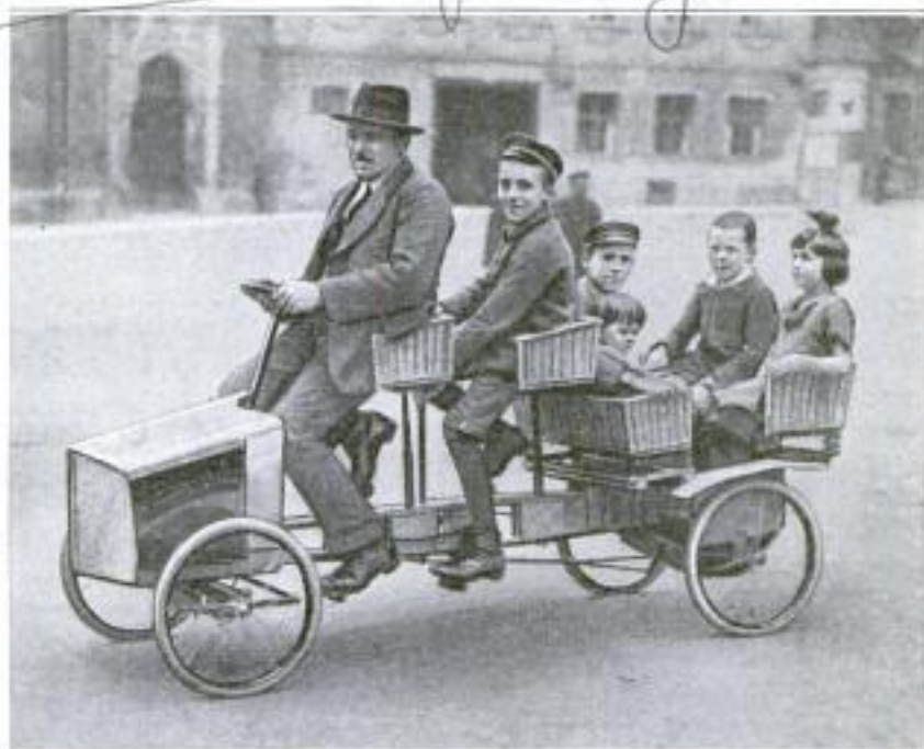
Odd-Appearing Vehicle in Which the Entire Family may be Transported, Showing the Clever Pedal Arrangement and the Wicker Baskets Used for Seats
