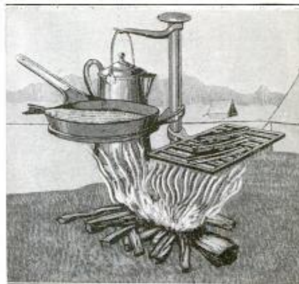
Stake for Cooking over the Camp Fire: The Brackets on the Stake may be Turned, Raised, or Lowered of the racks is intended for roasting, another holds a frying pan, while a coffee-pot may be hung from the third.
