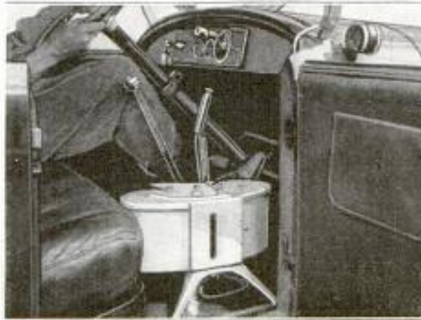
The Flow Meter, Shown in White, Makes a Photographic Record of the Flow of Gasoline to the Carburetor
