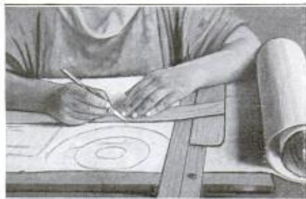
Draftsman Working on a Rolled Drawing and Using a T-Square Guide, Attached to the Board by Thumbtacks
