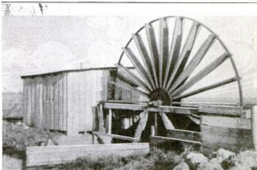
Wheel Pump That Drains 116 Acres of Marshland on a Farm Six Miles West of Sandusky, Ohio: The Wheel Is 16 Feet in Diameter
