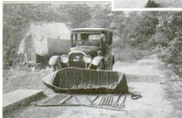
Upper Center: Collapsible Rowboat Shown Packed Ready for Carrying on the Running Board of an Automobile. Lower Left: Boat Shown Partly Assembled, with Oars, Latticed Floorboards, and Ash Strips on Ground in Front of It. Lower Right: Boat Entirely Assembled for Use
