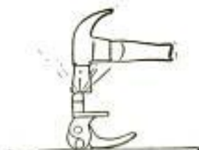
A tap with a hammer sinks the jaws in the wood close to the nail.
