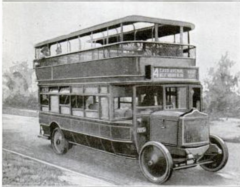
The Top Built over the Seats of the Upper Deck on the Bus Is an Innovation in Motor-Bus Equipment. There Is No Covering over the Aisle; Strips Similar to Auto Curtains Inclose the Sides in Rough Weather
