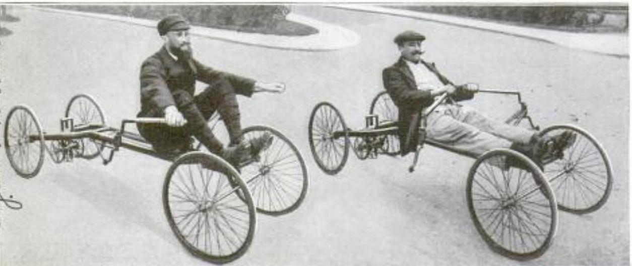
Four-Wheeled Auto Cycle That is Propelled with the Same Movements as in Operating a Pair of Sculls in a Boat with a Sliding Seat: The Left-Hand View Shows the Beginning of the Power Stroke, and the Right-Hand View the End of It
