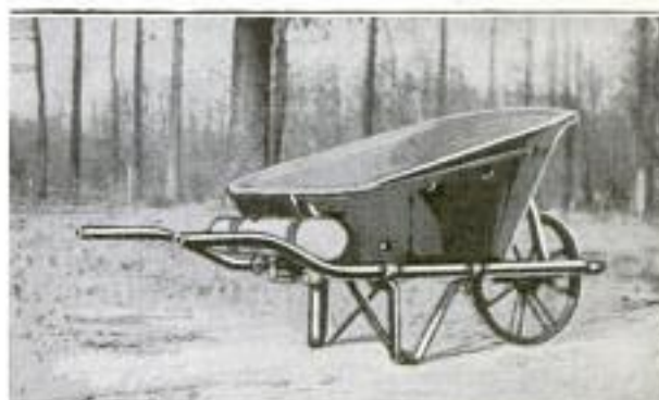
Above: Wheelbarrow Which Has a Gasoline Heater Incorporated in It for Facilitating Road Repairs. Below: Interior, Showing Road Material being Heated. The Fuel Tank is Seen between the Handles
