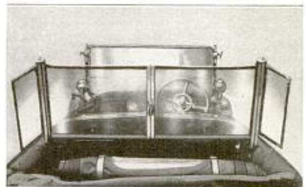
Flexible Windshield in Position, Showing How the Rear Seat is Adequately Protected from the Wind
