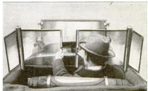
Flexible Windshield for the Rear Seat being Pulled from the Cylinders and Fastened in the Center
