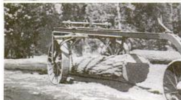
Above: Close-Up of Logging Wheel. Below: Wheel under Pull and Log Raised
