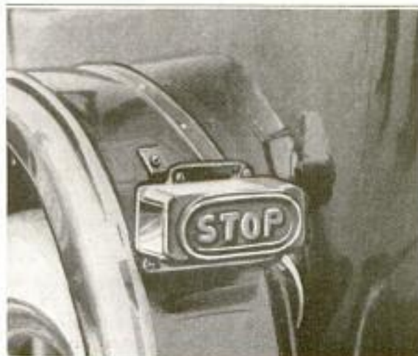
Automobile Stop Signal That Flashes Its Light Automatically and Exclusively by Any Retardation, Great or Small, in the Speed of the Car
