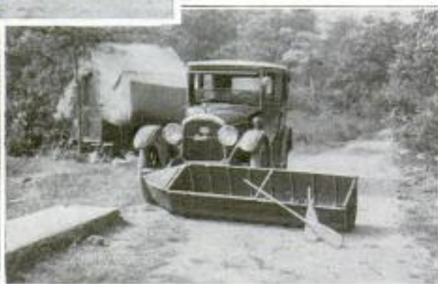
Upper Center: Collapsible Rowboat Shown Packed Ready for Carrying on the Running Board of an Automobile. Lower Left: Boat Shown Partly Assembled, with Oars, Latticed Floorboards, and Ash Strips on Ground in Front of It. Lower Right: Boat Entirely Assembled for Use
