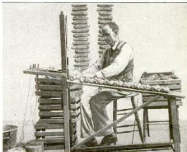
Device for Rapidly Stringing Ears of Corn So That They may be Hung Up for Drying or Storage, as Seen behind the Operator
