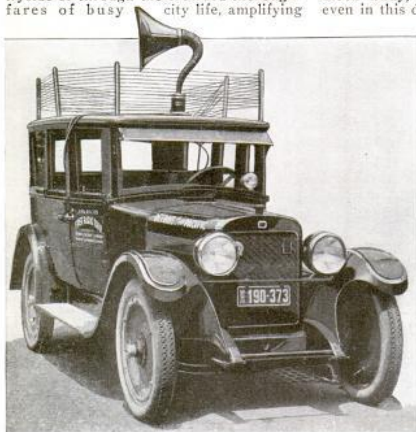
Automobile Equipped with Radio-Receiving and Amplifying Apparatus, Which Recently Completed a Successful Overland Trip, Giving Out News and Concerts along the Way
