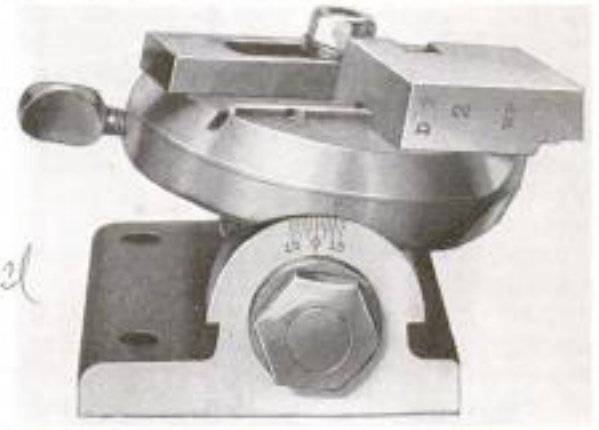
Chamfer-Grinding Fixture with a Thread Chaser in Position Ready for Grinding: When in Use, the Fixture is Bolted to the Grinder Table
