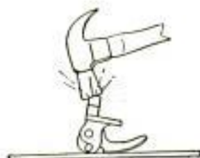
Then rap the bevel to close the jaws on the nail.
