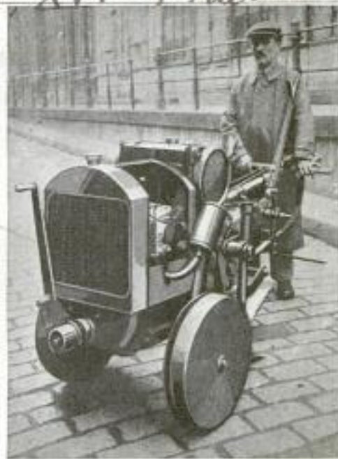
Side and Front Views of an Agricultural Tractor That is Propelled by the Two Feet on Vertical Oscillating Levers. Plainly Seen Above: The Driver Operates the Tractor Either on Foot or in the Small Seat Seen beside Him
