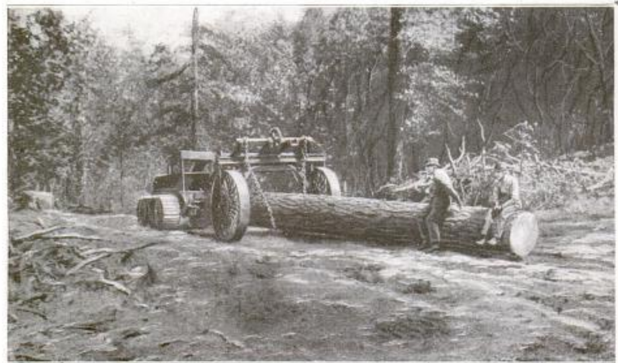
Crawler-Type Tractor and All-Steel Logging Wheel Engaged in Hauling a Large Log through the Forest in California: Note How the End of the Log at the Wheel is Held above the Ground
