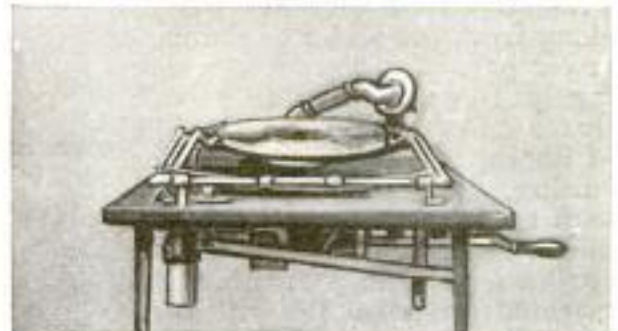
Three Views of Device for Automatically Turning over Phonograph Records: In the Center It is Shown Turning the Record Over
