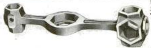
Socket Wrench Having 11 Different Grips Which will Fit Practically Every Nut and Bolt on Well-Known Small Car
