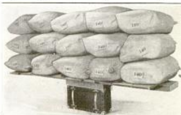
The Combined Weight of the Sacks Shown Above Is 2,100 Pounds. They were Loaded on This New Steel-Bound Suitcase in a Test to Determine Its Strength
