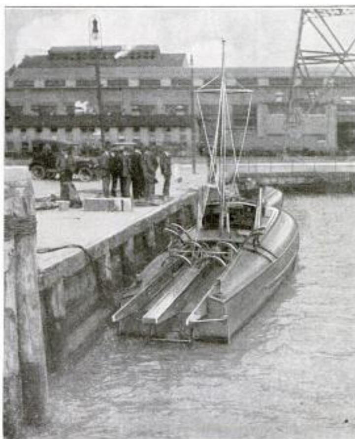
The Two High-Speed Torpedo Boats: The Nearer One Is 55 Feet Long with Two Torpedo Troughs, Seen at the Stern. The Smaller Boat Beyond Is 45 Feet Long
