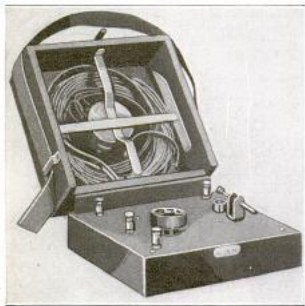
Portable Radio Outfit Opened, with Headpiece, Antenna, and Ground Wire Packed in the Cover, Ready to be Taken Out and Used
