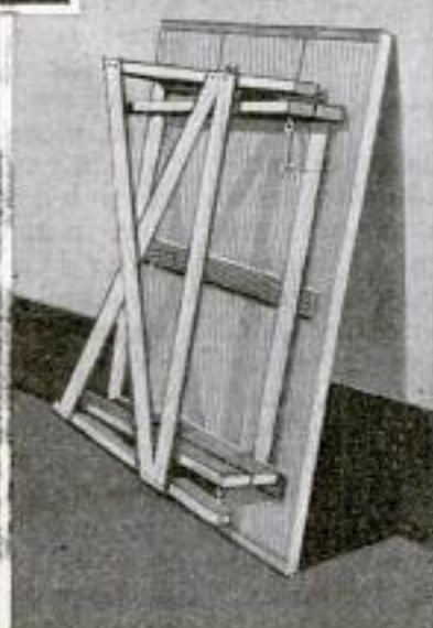
Upper Left: The Complete Table. Upper Right: Constructional Details. Lower Left and Lower Right: The Height of the Table Varied to Conform to the Posture of the User by Lengthening or Shortening the Chains That Hold the Legs Together. Center: Table, Folded
