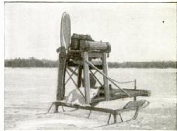
Ice Sled for Passengers and Freight, Showing the Propeller, Engine, and the Iron Steering Runner
