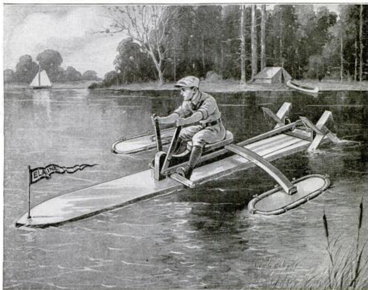
A Hand-Propelled Paddle-Wheel Water Craft of the Catamaran Type: The Back-and-Forth Movement of the Hand Levers Drives the Paddles through Connecting Rods and a Crankshaft. A Curved Out-rigger is Provided with Wooden and Pneumatic Floats on Either Side
