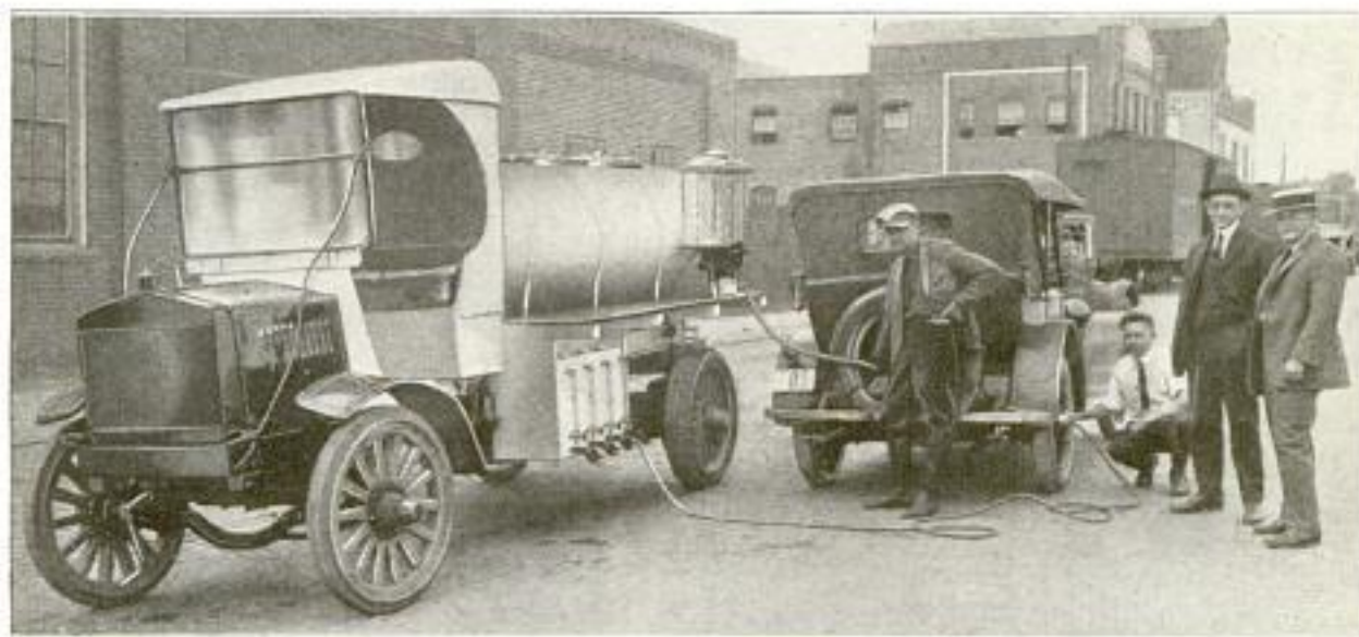
This Traveling Filling Station, Which Delivers Gasoline, Oil, and Air from House to House, or Dispenses Them on the Highways, is Here Shown Inflating the Tires of, and Also Supplying Gasoline to, a Passenger Car Encountered on One of the Streets of the City
