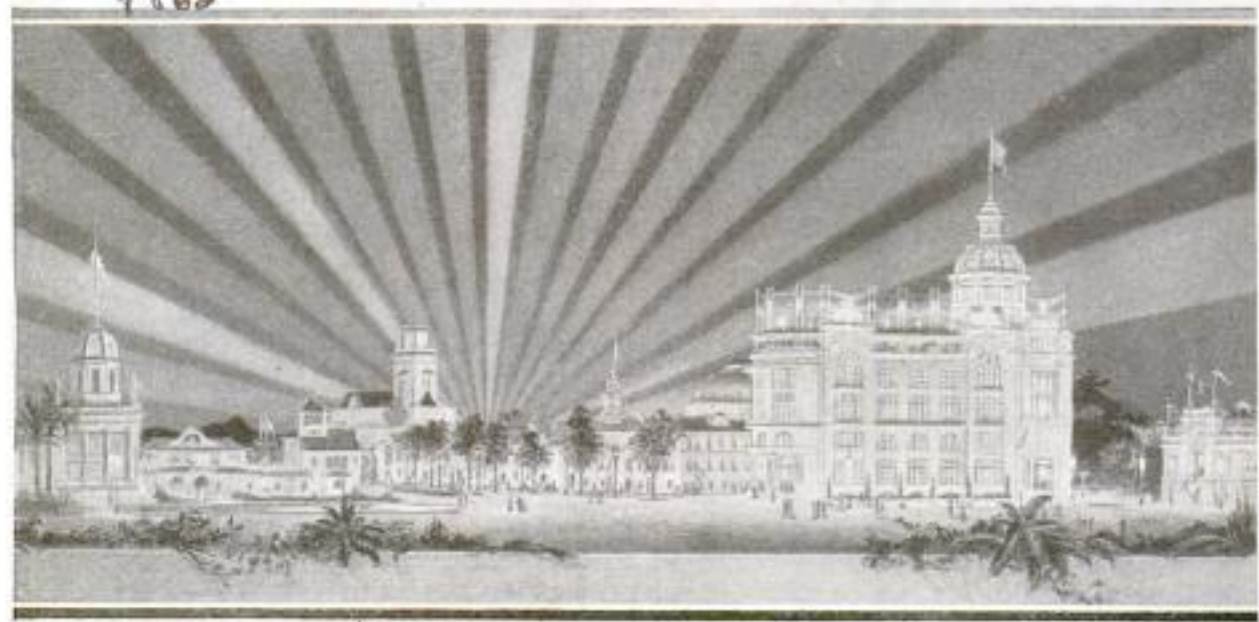
View to be Seen at the Forthcoming International Exposition at Rio de Janeiro, Brazil, Showing Effect of "Scintillator": The Apparatus Consists of a Battery of Sixteen 31-Inch Arc Searchlights Which Throw Their Beams of Light Radially over the Exposition Buildings. The Lights Are of Different and Changeable Colors
