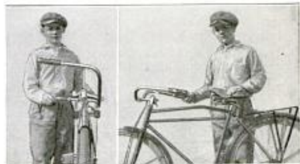
A New Adjustable Handlebar for Bicycles, Which can be Turned, as Shown at the Left, So That the Cycle can be Rested Safely against a Wall
