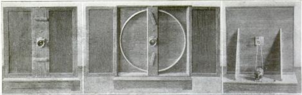
Left: Front View of Camera, Closed. Center: Front of Camera, Opened, Showing the Aluminum Ring for Holding the Film, and the Lens in the Center, behind Which Is the Rotative Prism. Right: Rear of Camera, Showing Small Electric Motor Which Drives the Prism
