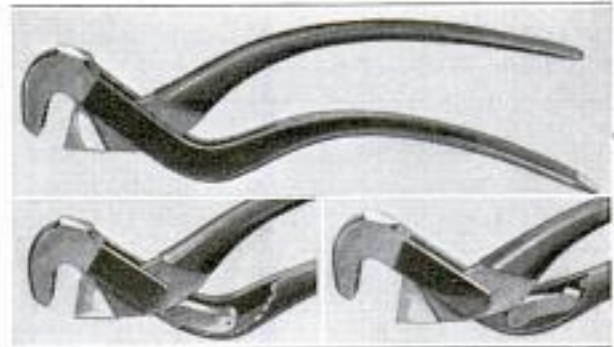
Self-Adjusting Wrench: In Lower Views Where Handle is Cut Away, Movable Fulcrum is Shown in Position, at Left for Small Objects, and at Right for Larger Ones
