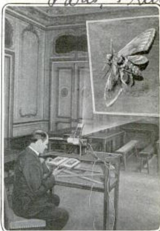
Apparatus in Use at the Art School of the Louvre, in Paris, That Projects the Image of an Object onto a Screen in a Room Sufficiently Lighted to Allow the Writing of Notes by the Students: The Apparatus will Project Greatly Enlarged Reproductions of Insects, as Shown to the Right, Where the Magnified Image of a Moth is Reflected by the Inclined Mirror onto the Screen.
