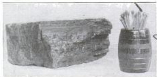
This Ornamental Match Holder was Machined from a Solid Lump of Coal and Buffed to a High Polish
