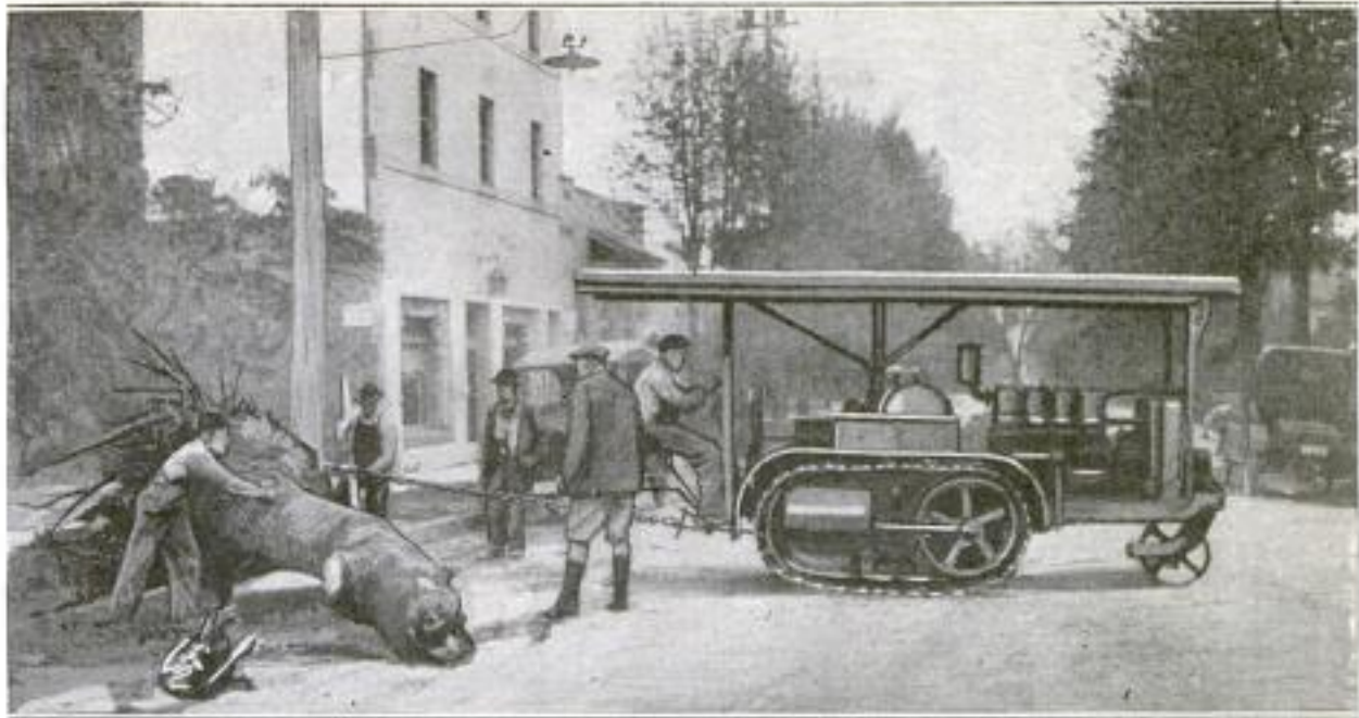
After Pulling the Tree Out by the Roots, the Tractor with a Single Mighty Heave Rolled the Stump and Trunk, Weighing Four Tons, onto a Sledge. It Then Towed the Whole Load to a Local Woodyard, Accomplishing the Entire Task in 20 Minutes
