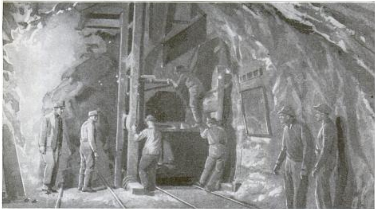
The Broken Salt is Loaded into Small Cars Which are Drawn to the Bottom of the Shaft and are Then Raised in the Cage to the Surface of the Ground
