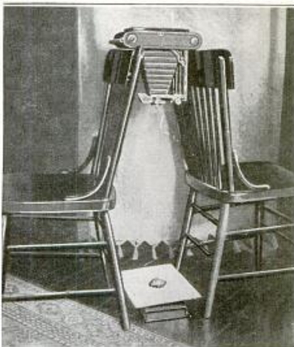
Small Articles can be Photographed More Easily with the Camera Arranged as Shown
