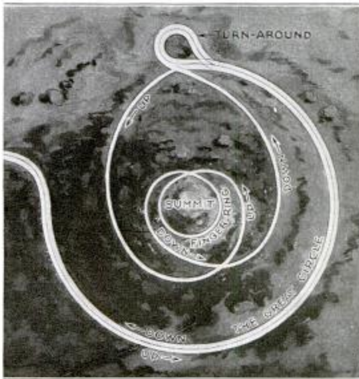
Diagram of the Tenderfoot Spiral Drive: As Far as the Turn-Around, the Road Is Full-Width, and from There On It Is Only Wide Enough for One Car
