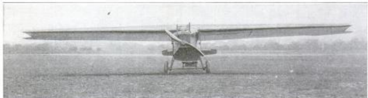
This Fokker Monoplane, Recently Delivered to the Army Air Service at McCook Field, Ohio, Seats 10 Passengers Comfortably and Has a Flying Speed of 41 to 95 Miles an Hour
