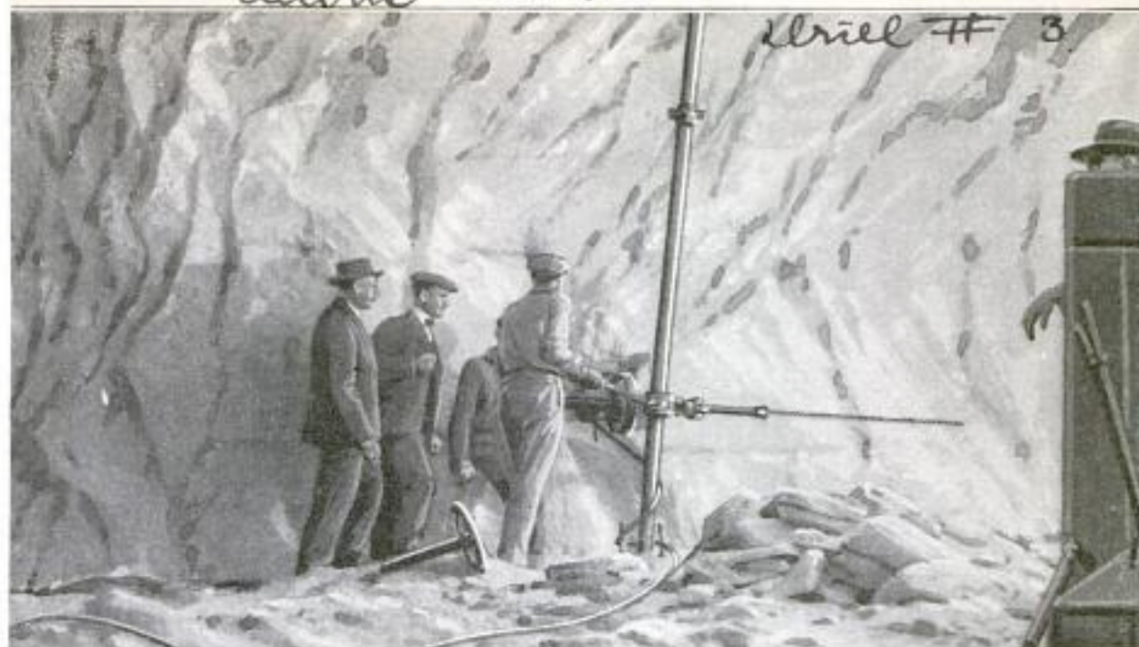
Scene in a Rock-Salt Mine, Showing One of the Electric Drilling Machines Boring a Hole in the Salt: The Machine is Clamped to the Vertical Bar, and the Augerlike Steel is Fed Forward through the Center of the Electric Motor That Drives It
