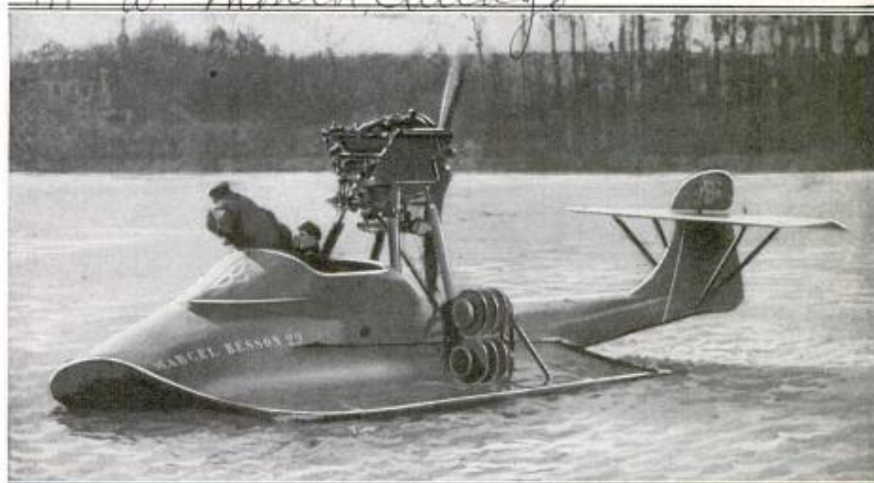
New French Hydroglider That Has a Speed of 63 Miles an Hour: The Motor, Directly Connected to the Air Propeller, Develops 300 Horsepower. In Every Respect It is Built Very Much on the Lines of a Flying Boat
