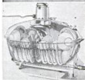
Above: Dishwashing Machine Which Utilizes Atmospheric Pressure in Cleansing the China and Silverware. Left: Interior View of Machine, Showing How Dishes are Packed
