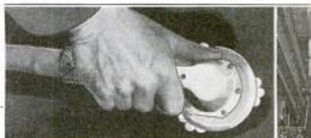
Above: Close-Up of the Electrical Skinning Tool. Showing the Blades of Clover-Leaf Design Which are Revolved at a High Rate of Speed. Below: Skinning a Steer with the Electrically Driven Tool
