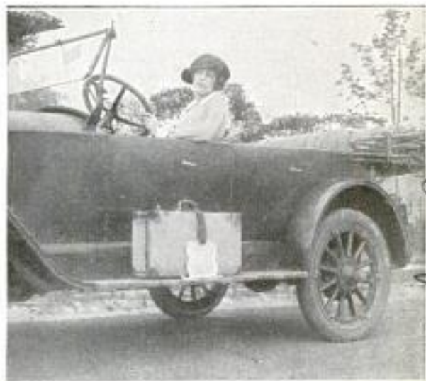
Combined Auto Step and Carrier as It Appears When Mounted on the Running Board of a Machine and Holding a Suitcase
