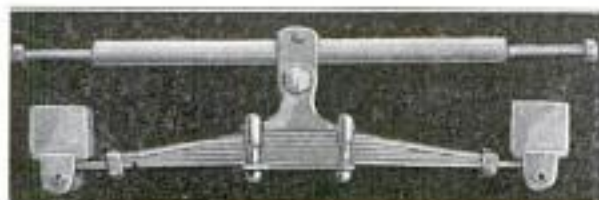
Three-Point Suspension Device: The Shackles on the Ends of the Spring Connect to the Axle, and the Cylindrical Crossbar Above Connects to the Car Body
