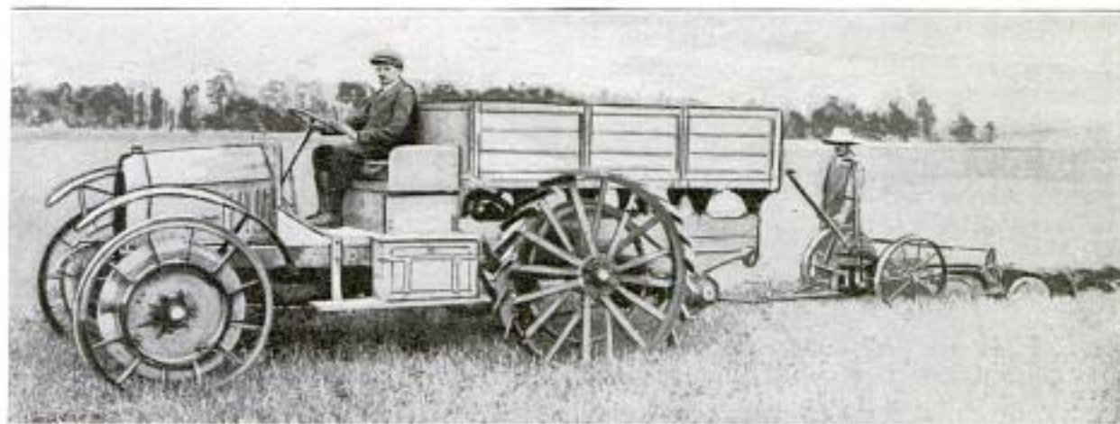
Interchangeable Power Car in Use as a Tractor, Shown Hitched to a Plow Ready to Start to Work on the Stubble: The Rims are Mounted on the Front Wheels. The Rear-Truck Wheels have been Removed, and the Sprocket on Their Axle Is for Driving the Tractor Wheels
