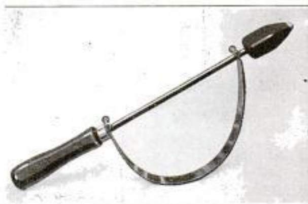
This Attachment for the Soldering Iron Removes the Weight of the Tool from the User's Wrist and Serves to Support the Iron in the Flame
