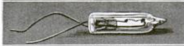
Miniature Lamp (Exact Size) Which Aids in Changing Sound Waves to Light Waves When Voice Variations in the Transmitter Vibrate the Filament
