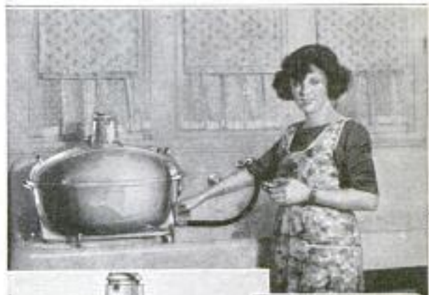
Above: Dishwashing Machine Which Utilizes Atmospheric Pressure in Cleansing the China and Silverware. Left: Interior View of Machine, Showing How Dishes are Packed
