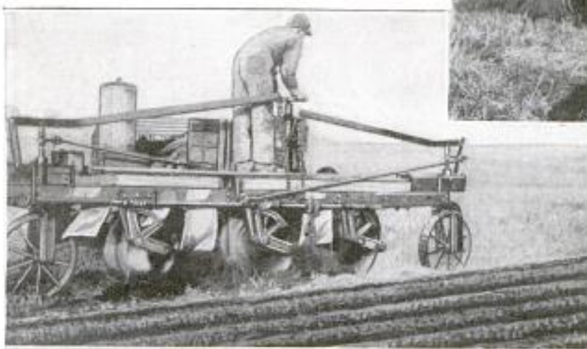
Side View of the Plow in Operation on Stubble, with Three of Its Rotary Shares Visible: With a Single Operator Handling the Machine, as Shown, It will Plow 15 Acres in 10 Hours
