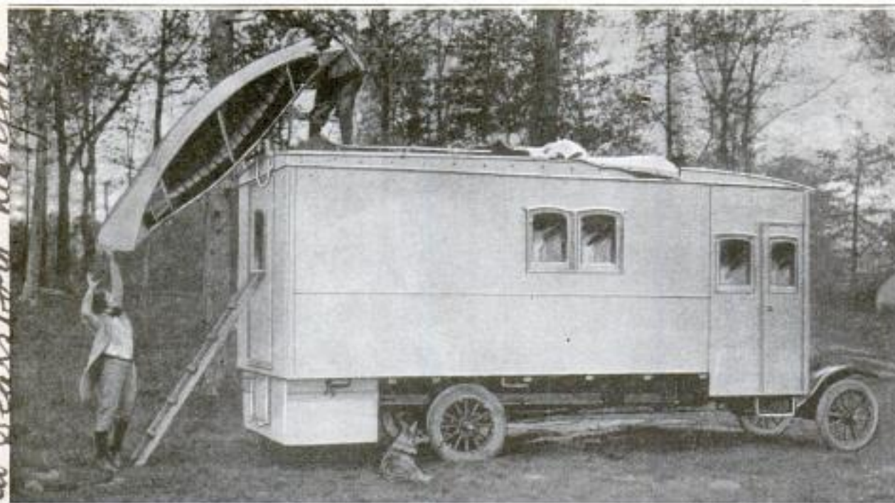
House on Wheels Which is Constructed on the Chassis of a Motor Truck: The Outfit has Come to a Stop for the Night, and the Tourists are Lowering the Canoe, Which is Carried on the Top of the Vehicle While Traveling
