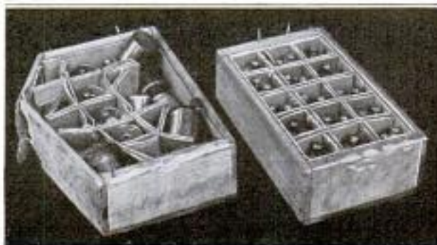
Results of "Tumbling" Test with Two Boxes, One Packed Tightly and the Other Loosely
