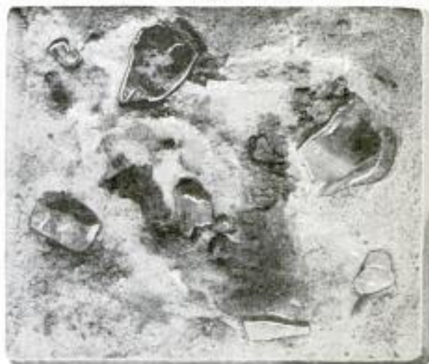
Decorative Tile Made of Neutral-Tinted Concrete, into Which, While Plastic, Fragments of Flint, Agate, or Quartz are Thrust, Leaving the Edges Protruding
