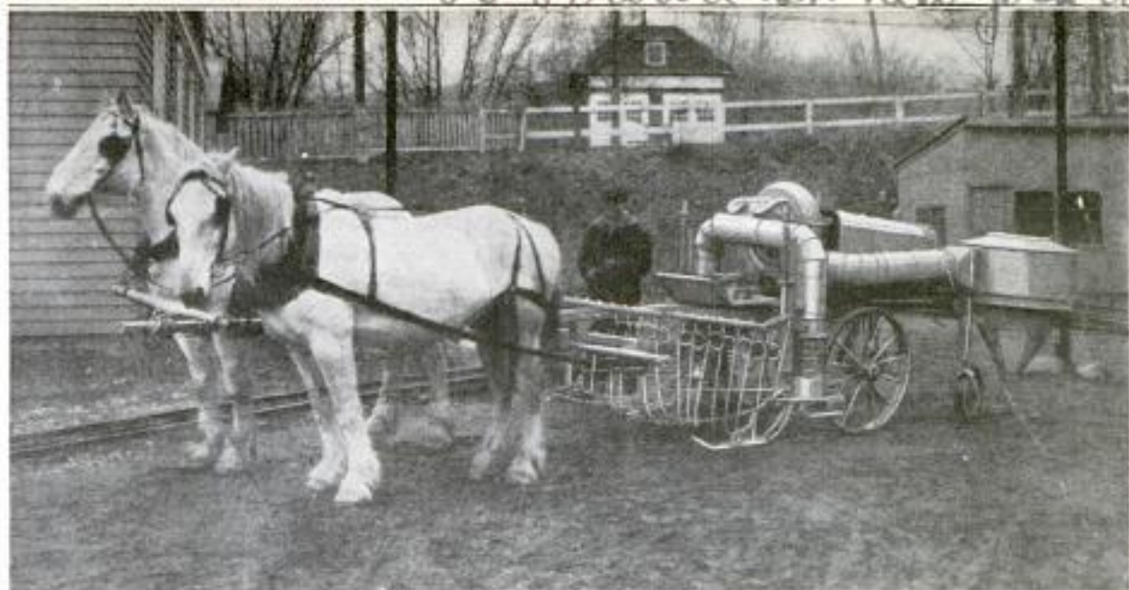
The Suction Machine, with the Flexible Pipes Raised to Clear the Ground When Moving from One Field to Another: In Operation, These Pipes are Lowered Close to the Ground and Pick Up Weevils and Slugs, Dislodged by the Spring-Wire Agitators in Front
