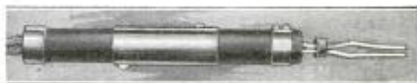
Electrically Heated Tool for Setting Roller-Table and Pallet Jewels in a Watch, Showing the Two Small Jaws and Fiber Ring
