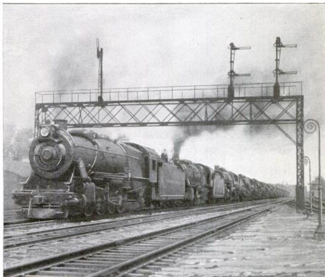
The "Prosperity Special," a Train of Southern Pacific Locomotives, of the "2-10-2" Type, That Traveled from the Baldwin Works, at Philadelphia, to Corsicana, Texas: Each Locomotive with Tender Is Nearly 100 Feet Long, and When Loaded Ready for Service, Its Total Weight Is 310 Tons
