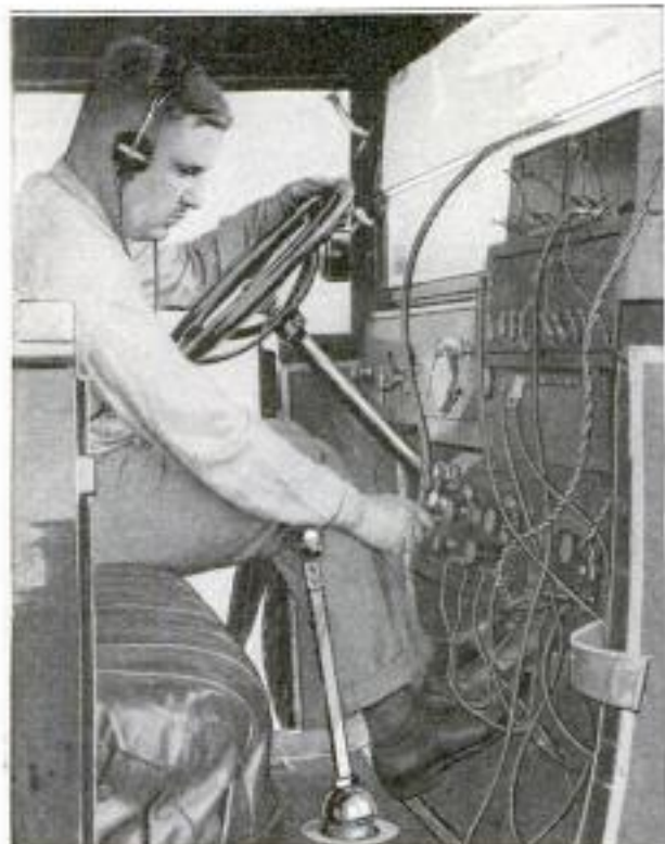
Left: Elaborate Radio-Instrument Installation, Which was Placed on the Dashboard of the Machine So the Driver could Also Do the "Tuning In." Right: Front View of the Motor Bus, Showing the Method of Mounting the Aerial on the Machine
