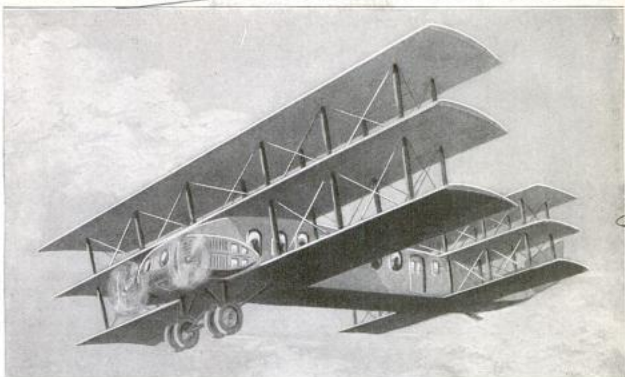
This Passenger and Freight-Carrying Triplane is Now being Constructed in Kansas City, Missouri, and is Designed to Carry 30 Passengers and 1,000 Pounds of Freight. The Fuselage is Built on a True Wing-Shape Section and is Over Eight Feet Wide and Six Feet High
