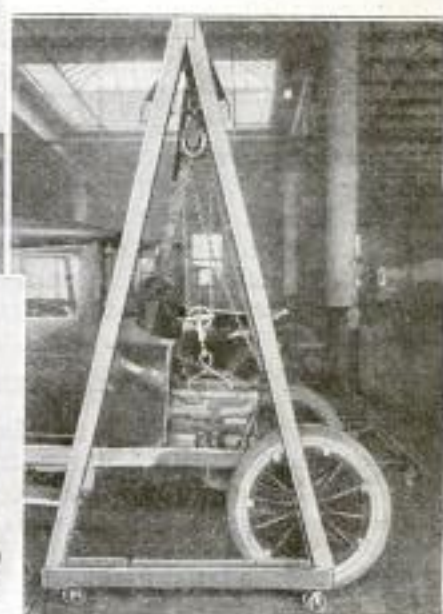
Left: A Portable Hoist, Built from Timbers and Mounted on Ball-Bearing Casters. Center: An Engine Puller Made from Two Spark-Plug Shells and a Piece of Steel Rod. Right: Both Devices Shown in Use for Lifting an Engine from Its Position on the Chassis
