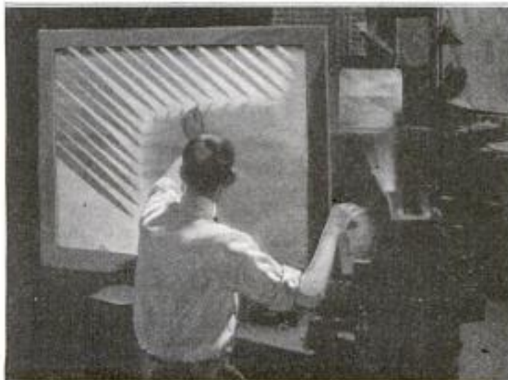
Projection of the Magnified Image of a Gear Tooth onto a Mirror, from Which It is Reflected Back to the Ground-Glass Screen on Which the Operator is Drawing Its Outline
