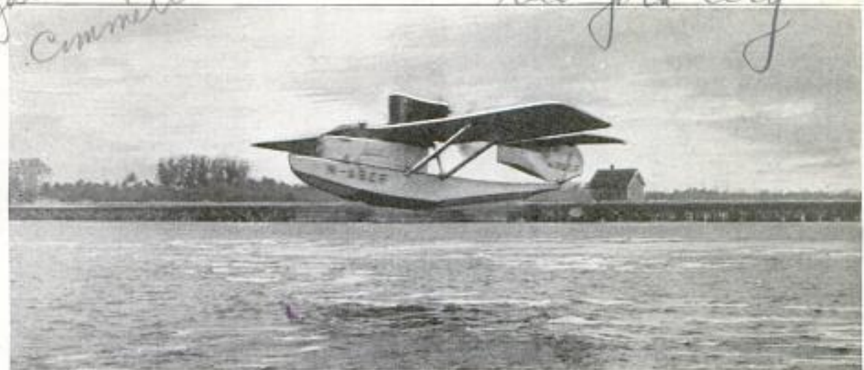
This Loening Air Yacht, of Remarkably Graceful Lines, Seats Four Passengers Besides the Pilot, and is Noted for Its Successful Long-Distance Flights and Rapid Climbing Ability
