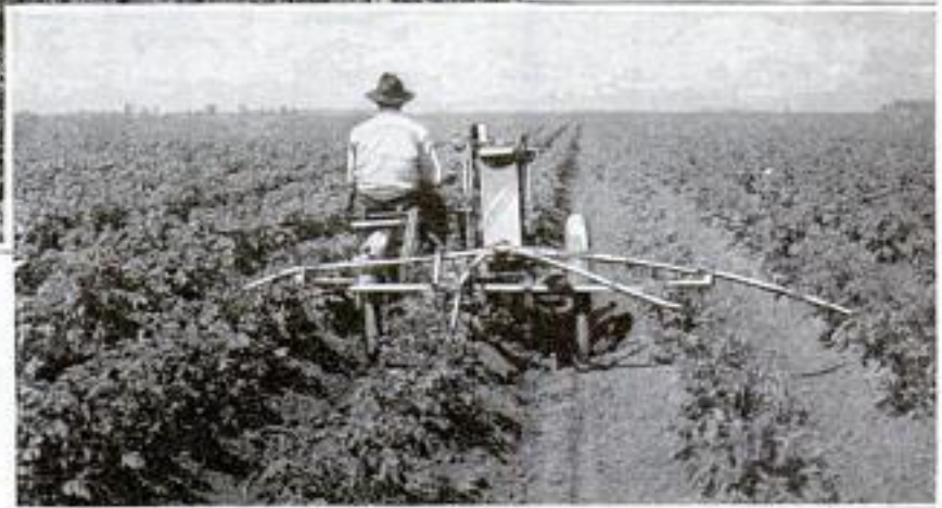
Upper Left: The Motorcycle-Mounted Potato-Plant Sprayer as Seen from the Side. Lower Right: Spraying Outfit Seen from Rear, Showing How the Machine Sprays Four Rows at Once
