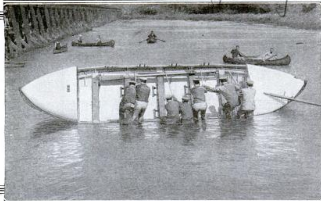
Lifeboats are Made Unsinkable by being Constructed with Water-Tight Air Compartments Fore and Aft, So That, If the Boat is Capsized, Though It may Turn Upside Down, It will Never Sink. Here is Seen a Pacific Coastguard Crew Righting an Unsinkable Lifeboat That has been Upset. They are Doing It as Part of Their Practice Drill. One Oar can be Seen Secured to the Thwarts. Others may Be Afloat in the Water
