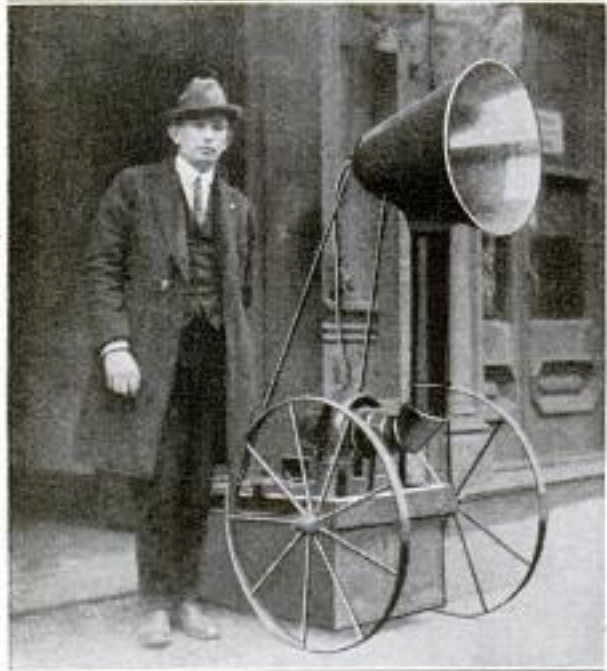
A Bright Light in the Funnel of This Bug Catcher Attracts the Winged Pests, and a Suction Fan Draws Them into a Screened Trap
