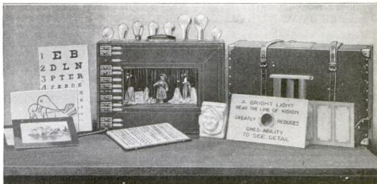
A Suitcase Outfit for Demonstrating Lighting Principles and Advantages of Different-Style Lamps: All the Material Shown can be Packed in the Case When Moving On to the Next Customer
