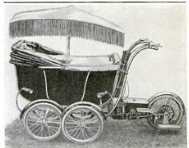
Baby Carriage, Showing Motor, Extra Wheel, and Footrests at the Rear: The Control Mechanism is Shown on the Handle
