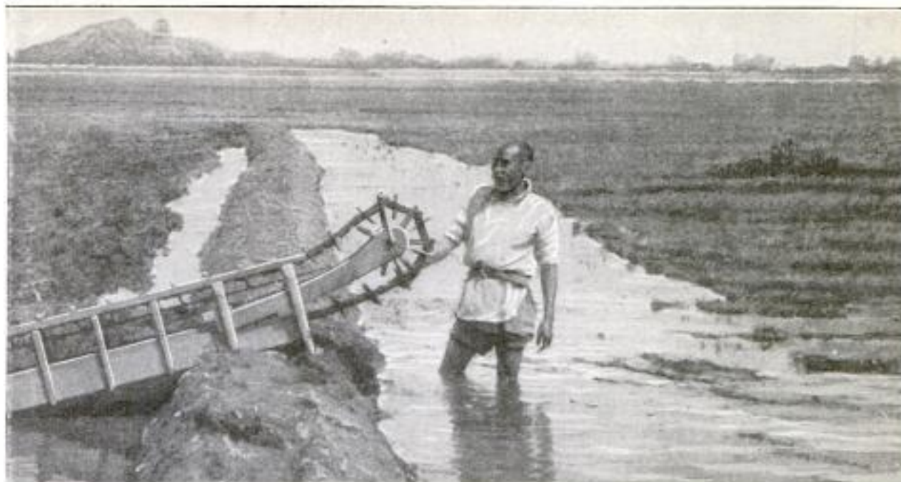
A Form of the Well-Known Chinese Pump Used on the Rice Fields of China for Conveying Water from One Field That is Well Irrigated to Another That Needs More Irrigation: The Hand Crank That Operates This Chinese Pump is Seen near the Right Hand of the Chinaman
