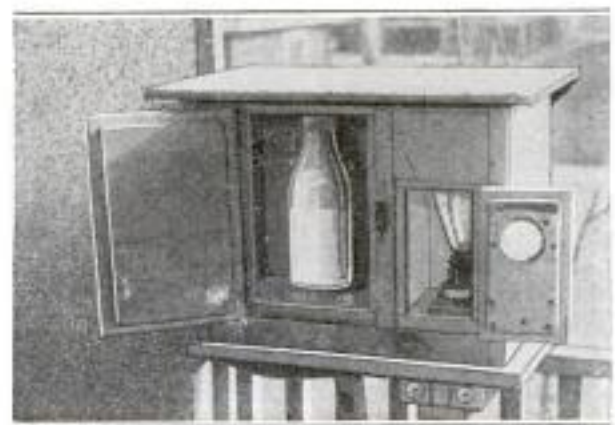
Box Designed to Keep Milk from Freezing: The Bottle can be Seen in One Compartment and the Lamps in the Other
