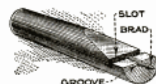
A Simple Clamp for Holding Pistons Securely, and without Danger of Distorting or Scratching Them
