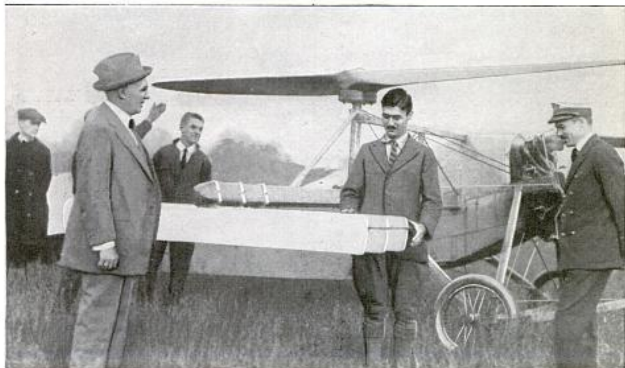
A Closer View of the Machine, Giving a Good Idea of the Size of the Propellers, and the Arrangement of One Set of the Balancing Vanes That Function as Ailerons
