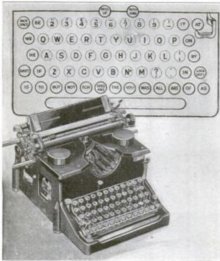
Word-Writing Typewriter: The Enlarged Keyboard Shows the Keys for Writing Words at One Stroke. The Carriage-Shifting Lever Is at the Right of the Keyboard
