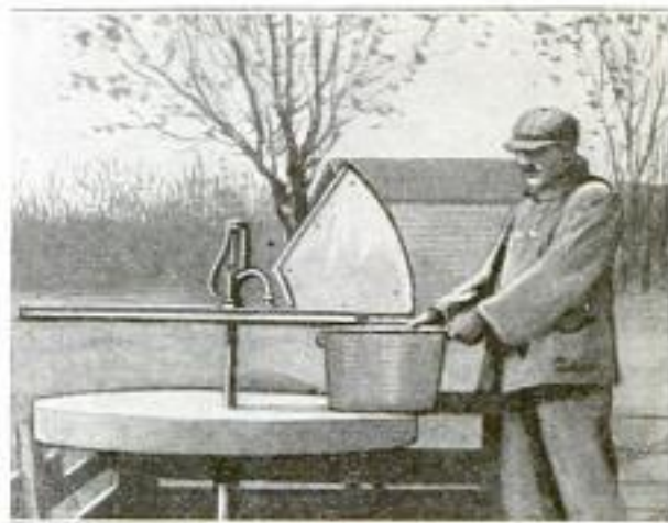
A Device for Soaking Grain Used as Swine Feed: It is Attached to the Yard Pump
