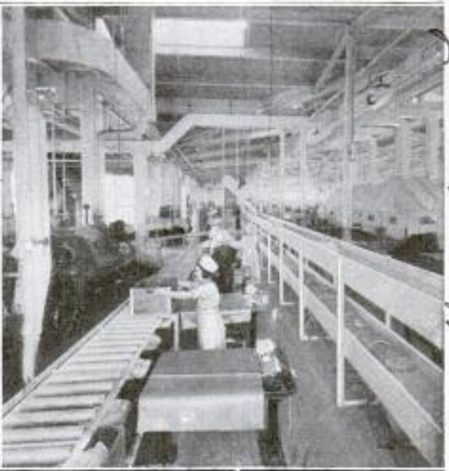
Roller and Belt Conveyors are Used in This Laundry for Transferring the Wet Clothes or Finished Bundles from Point to Point with a Minimum of Labor
