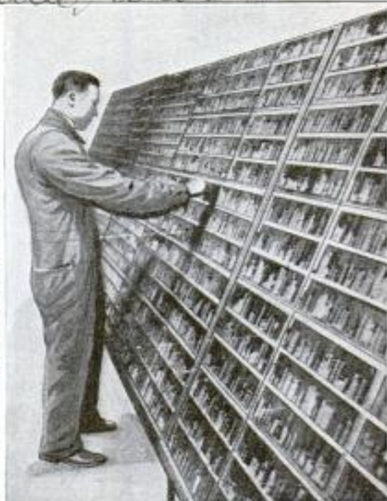
Above: This Is the Press Used for Printing the Chinese Newspaper Published in Seattle, Washington. Ordinary Newsprint is Used, and the Printing is Done in a Glaring Shade of Red Ink. Right: Setting the Type for the Chinese Newspaper. In the Ordinary Typesetter's Font There Are Some 6,000 to 7,000 Characters Used, Each One Denoting a Single Word
