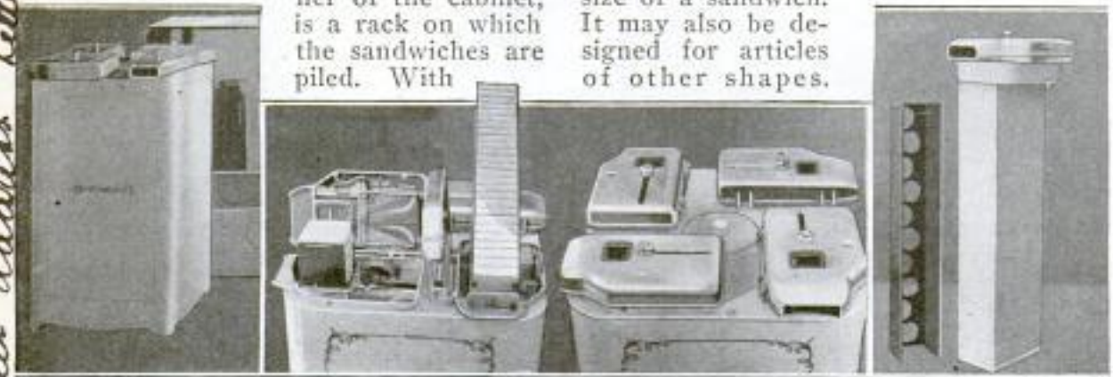
Left: General View of Sandwich-Vending and Refrigerating Machine. Center: Two Top Views, the One at Right Showing Device at Each Corner for Delivering Sandwiches, the Other Showing Two of These Open, with Sandwich Piles Raised. Right: One of the Racks in Which Sandwiches are Piled
