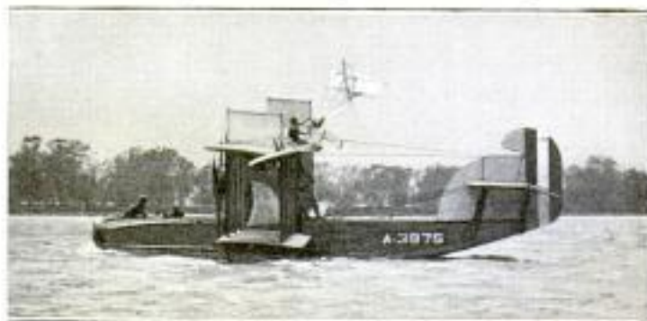
If the Seaplane is Forced Down and Needs Assistance, the Kite Carries Aloft the Wireless Antenna, While the Wind Stream from the Propeller drives the Radio Generator
