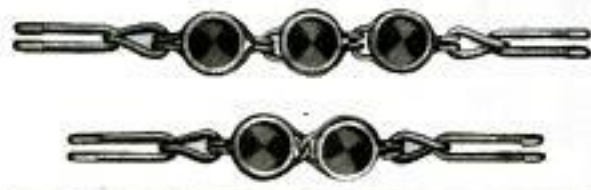
Cross Chains for Automobile Tires: Two or Three Links on the Tire Tread Have Each a Vacuum Cup That Grips Firmly and Resists Wear
