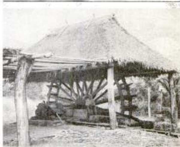
In This Small Sugar-Cane Mill a Small Stream has been Diverted and the Water Wheel is Used for Driving the Rollers of the Mill
