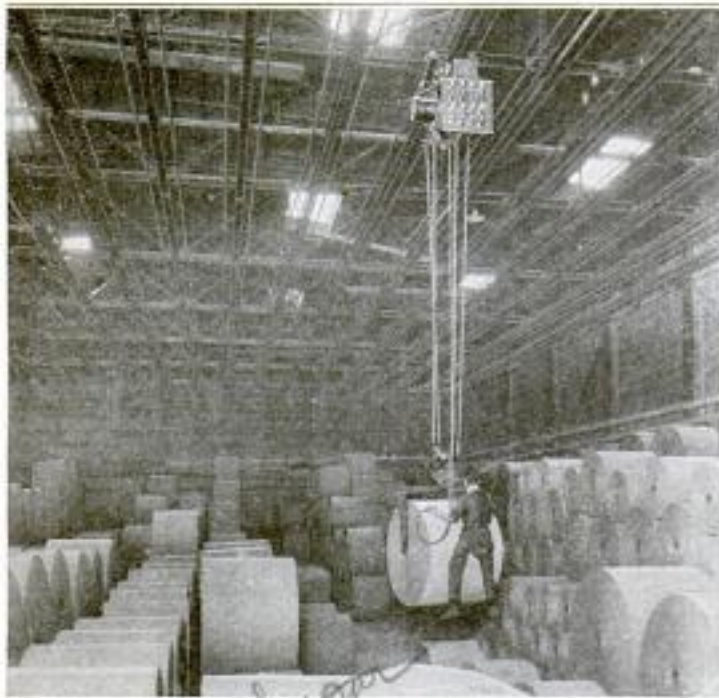
Left: One-Man Electric Crane Handling a Large Roll of Paper in the Warehouse. Overhead can be seen the I-Beam Tracks and the Electric Panel Which is Controlled by the Push-Button Switch in the Hand of the Operator. Right: Close-Up of the Crane, Showing the Saddlelike Seat
