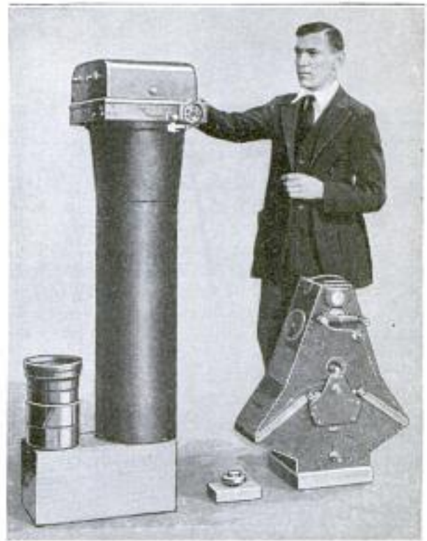
The Huge Camera at the Left, Due to Its Unusual Focal Length, can be Used at Very High Altitudes. At the Right Is the Triple-Lens Camera for Mapping
