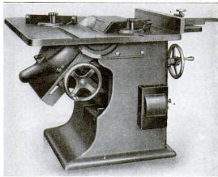
Tilting Arbor Saw Bench with Direct Motor Drive, and Saw at an Angle of 45 Degrees: Motor on Bracket at Left Is Adjustable
