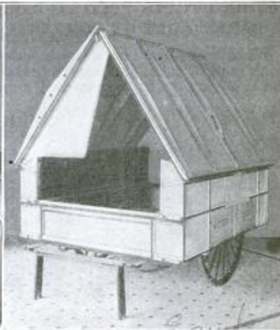
Above is Shown the Baggage Trailer Ready for Attaching to the Rear of an Automobile. The Cylinder in Which is Contained the Coil Spring, can be Seen Just above the Center of the Wheel. The Tanks for Gasoline and Oil Are Also Visible. At the Right is Shown the Manner of Raising the Top of the Trailer When Temporary Sleeping Quarters are Desired
