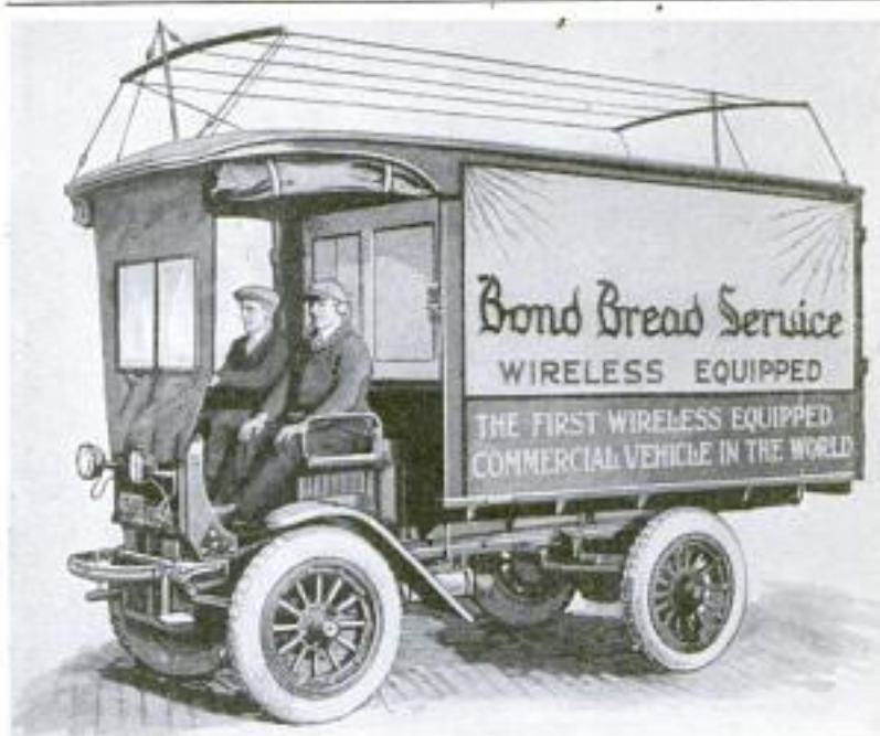
Delivery Truck Showing the Aerial for the Wireless Messages Which Enable the Manager of the Company to Keep in Constant Touch with the Drivers: Note the Receivers on the Man's Ears
