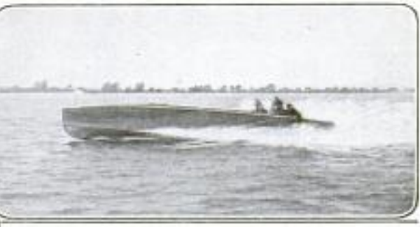
Left: When the Deck is Folded Over, the Two Liberty Motors of 450 Horsepower Each are Entirely Inclosed. Above: The Nonsinkable Motorboat on a Trial Run. During One Trial the Boat Sank, but as Soon as the Momentum had been Overcome the Water-Tight Compartments Exerted Their Buoyancy and Brought the Boat to the Surface
