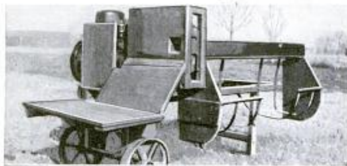
Tobacco-Gathering Machine That Strips the Leaves from the Lath When It is Inserted in the Hole Seen above the Table
