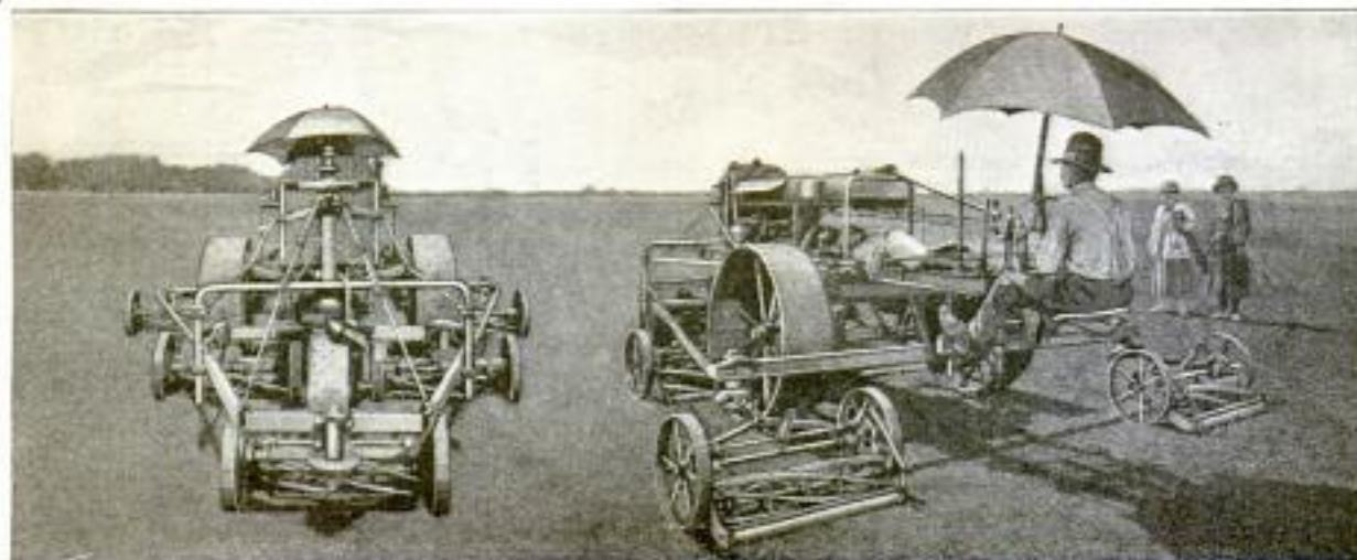
The Front View of the Motor-Driven Mower, at the Left, Shows the Triangular Arrangement of the Five Cutting Units on the Floating Frame. At the Right Is a Rear View Which Reveals the Extreme Length of the Steering and Control Apparatus
