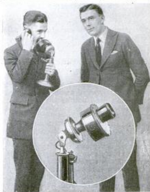
This Mouthpiece Screens the Voice So That a Person Standing Near By Hears Only a Low Murmur
