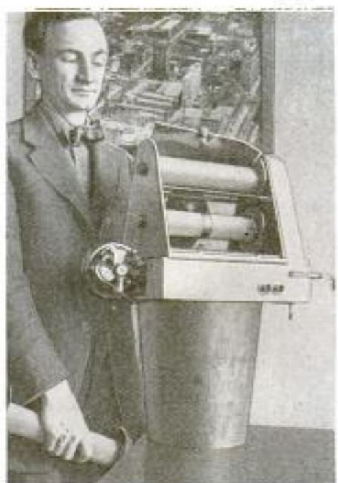
Large High-Speed Aerial Camera, with the Lens End Below, and Above, the Spools on Which the Film is Wound by the Electric Motor Seen on the Left Side
