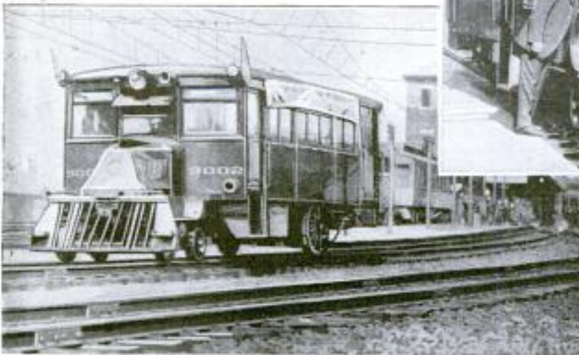
Gasoline-Driven Rail Car Operated by the New York and New Haven Railroad as It Appeared When Leaving the Yards on the Final Test Trip
