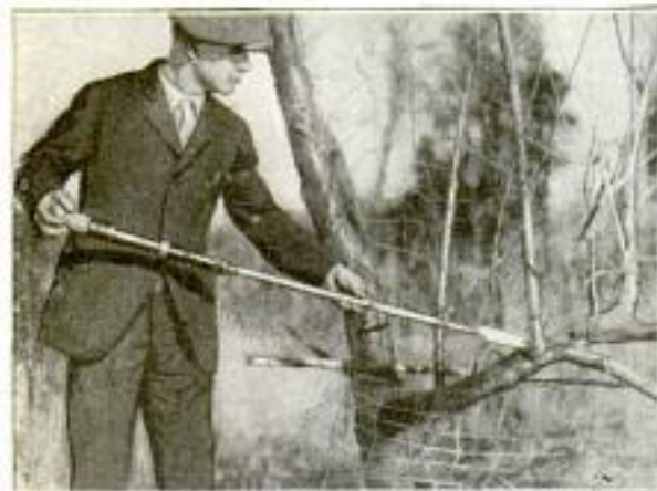
Tree-Pruning Chisel Which can be Fitted with a Long Handle, Thus Enabling the Workman to Trim Small Trees without a Ladder
