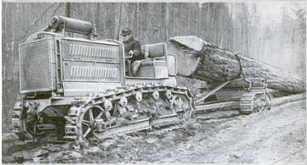
Huge Log being Hauled with Its End Supported on a Dolly, or "Bummer," That Has a Truck Fitted with Continuous-Tread Traction Wheels Similar, on a Smaller Scale, to Those of the Tractor That is Hauling. This System of Traction Allows the Tractor to Haul Heavy Loads over Soft Ground
