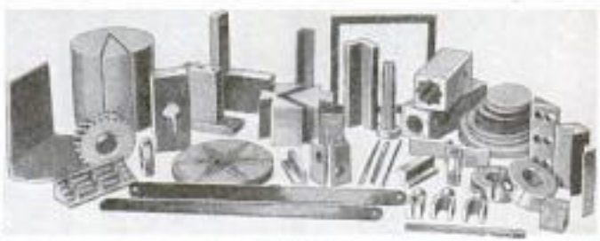
At the Left is Shown the Saw with Which Work Similar to That Done on a Shaper, or a Milling Machine, can be Accomplished. At the Right are Seen Specimens of Numerous Kinds of Work Completed with the Shaping Saw
