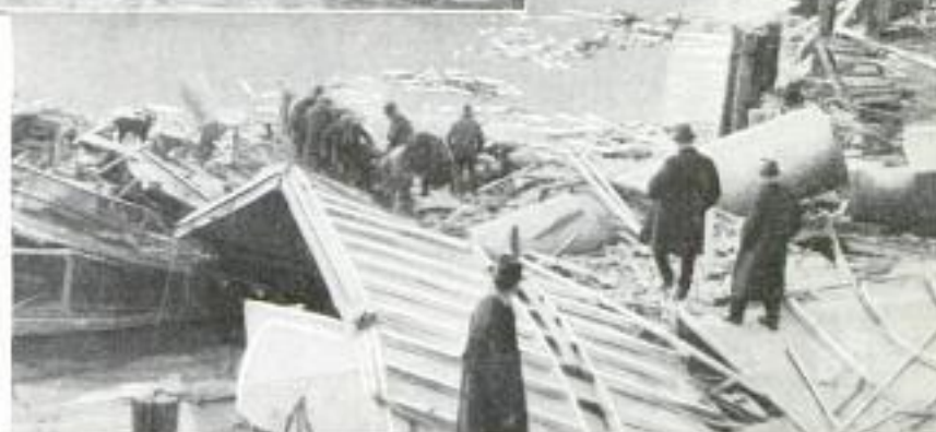
View of the Shattered Hull of the Ferryboat Lying in the Black River, Michigan, Showing How Completely It was Wrecked When Its Boiler Exploded
