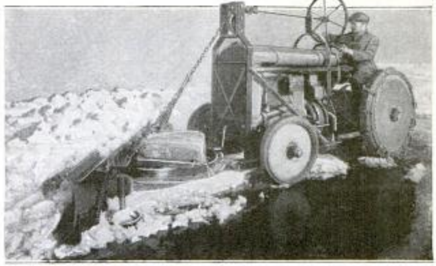
Combined Tractor-Snowplow in Operation, Showing the Method of Attaching the Plow to the Front of the Tractor, and Also How It is Weighted
