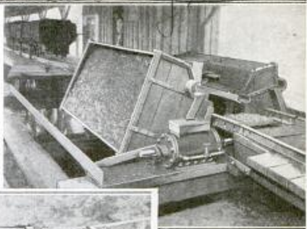
Above: Automatic Car Dump, Illustrating the Manner of Dumping the Cars. The Loaded Car on the Left is being Dumped by Gravity and at the Same Time Elevates the Empty Car on the Right to the Track. Left: The Dumping Mechanism
