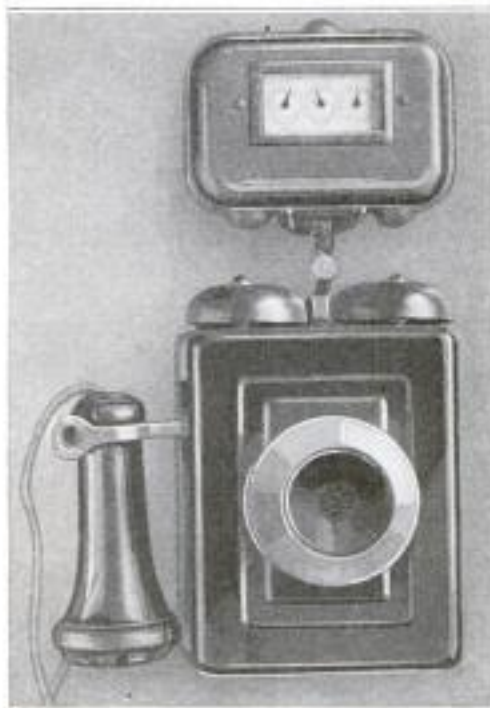
Measured-Service Equipment Which is Installed at the Subscriber's Home or Place of Business, Showing the Recording Meter above the Telephone
