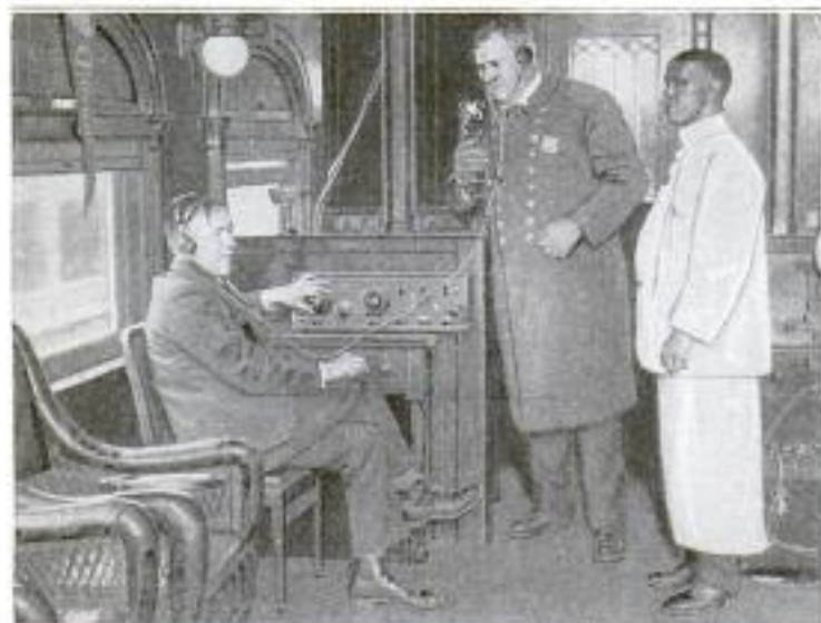
Radiophone Equipment Installed in a Buffet Car on the Lackawanna Railroad being Tested Prior to Its Regular Use on the Trains
