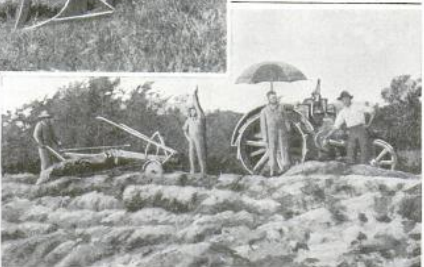
The Tractor-Drawn Brush Plow in Operation: Because of the Extra-Large Clearance in the Throat, the Brush Plow can Turn Under Any Standing Growth That the Tractor Is Able to Override
