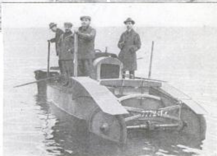
Two Float Tanks Supply Buoyancy for the Car When in the Water, and the Wheels are Drawn Up by a Special Arrangement So the Paddles will Be at the Proper Depth
