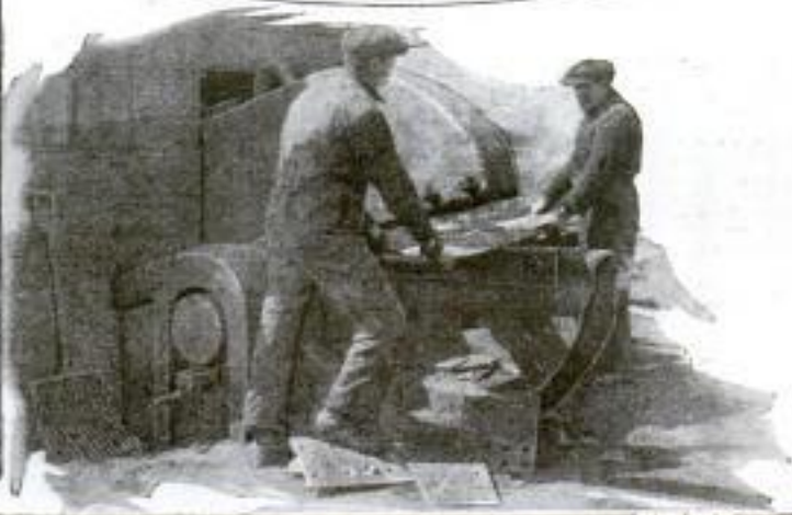
Lower Right: Crocodile Shear Cutting Up a Plate of Protective Deck Chrome-Nickel Steel Armor from a Scrapped Torpedo-Boat Destroyer. This Valuable Alloy is Adapted to Many Peaceful Uses, Particularly in the Automobile Industry
