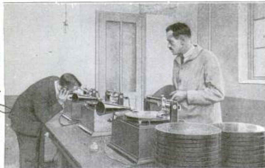
These Phonographs Run at Much Higher Speed than the Regular Machines, and are Used in Receiving High-Speed Radio Messages Which are Recorded and Preserved on the Extra-Heavy Disks
