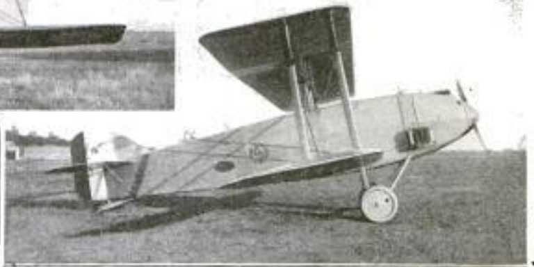
Above: In This French Airplane, of Unusual Appearance, the Lower Wing Has a Span Greater than the Upper Wing, This Design being Adopted to Equalize the Stresses in the Wings. Right: The Wings are Set Much Farther Back on the Fuselage than Is the Case with Airplanes of Conventional Design
