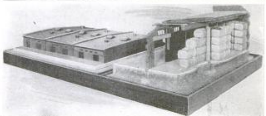
This Model Shows the Proper Construction for a One-Story Warehouse When Brick is Used. It is Built in Sections, with 18-Inch Firewalls between Them, Which Extend 18 Inches above the Roof
