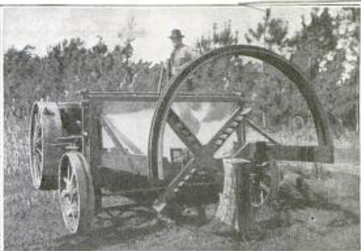
When the Tractor Wheels Force This Machine Ahead, the Rapidly Revolving Cutter Arms Reduce the Stump to Chips in a Short Time, and Leave Only a Moderately Large Hole in the Ground, as Shown at the Left
