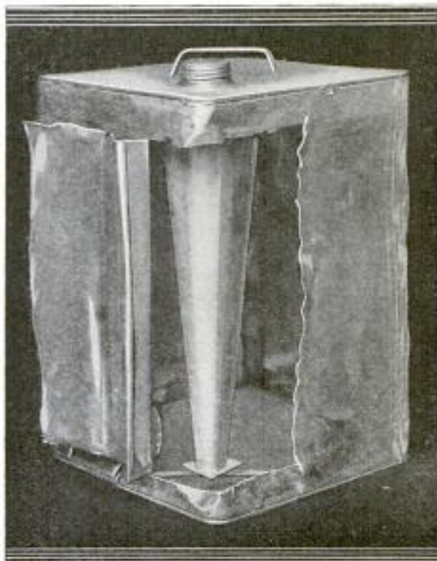
Five-Gallon Can with Sides Cut Away to Show the Arrangement Devised for Swindling Purchasers of Liquor: The Small Cavity Just below the Screw Top was Filled with Whisky, the Remainder of the Can Containing Water
