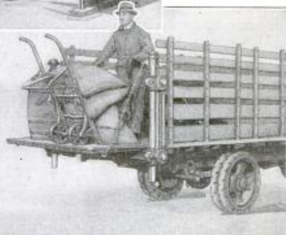
This Elevating End Gate Takes Much of the Labor Out of Truck Loading. The Hand Truck is Run onto Gate When in the Low Position, and by Shifting a Lever, Gears on the Engine Shaft are Thrown In and the Gate and Load Raised
