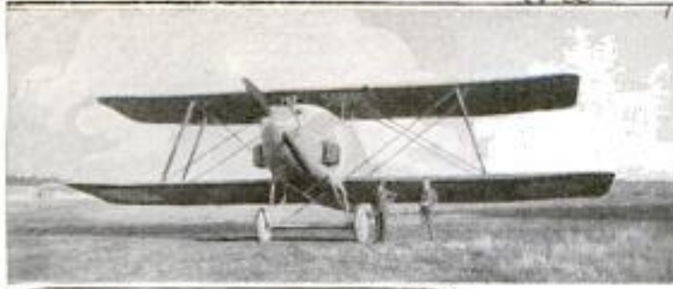
Above: In This French Airplane, of Unusual Appearance, the Lower Wing Has a Span Greater than the Upper Wing, This Design being Adopted to Equalize the Stresses in the Wings. Right: The Wings are Set Much Farther Back on the Fuselage than Is the Case with Airplanes of Conventional Design
