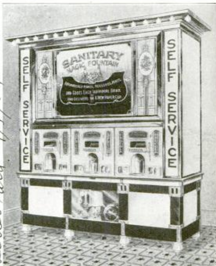
Automatic, Sanitary, Nickel-in-the-Slot Fountain That Mixes Cold Drinks and Serves Them to Three Customers at a Time: Its Own Refrigerating Apparatus can be Seen Below
