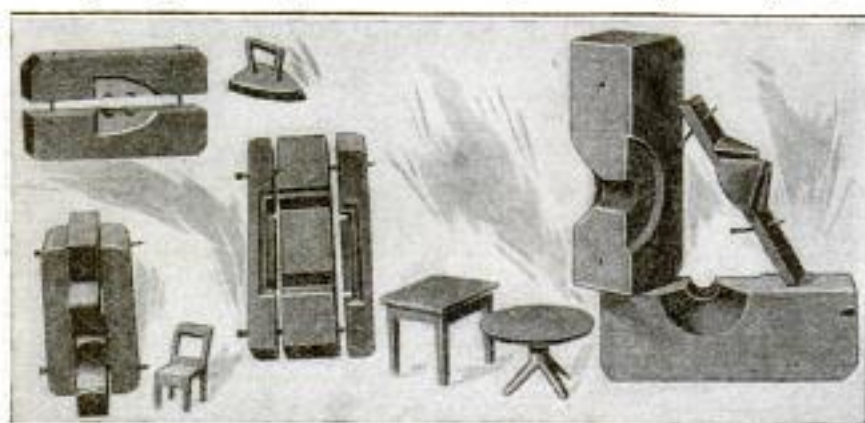
Molds Used for the Flatiron, Kitchen and Dining-Room Tables and Chair, and Samples of the Toys Cast in Them
