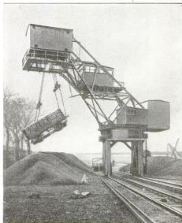
This Revolving Crane Picks Up Loaded Coal Cars and Dumps Them Also, Weighing the Coal as It is Discharged
