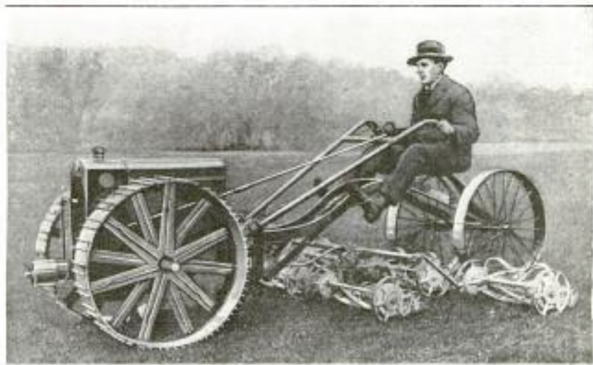
Small Tractor Pulling a Number of Lawn Mowers over the Fairway of a Golf Course: The Plowlike Steering Handles Form an Interesting Feature of the Machine
