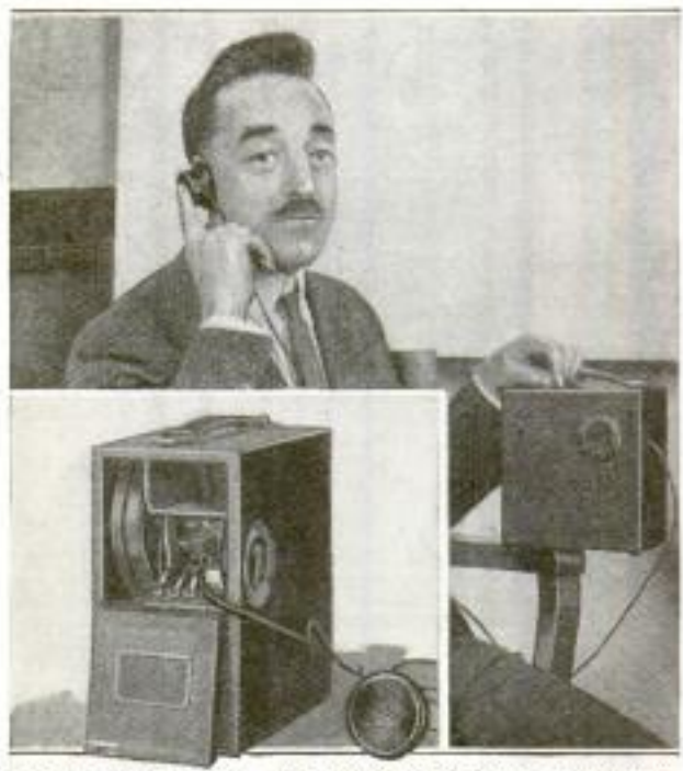
Telephonic Hearing Aid Which Employs a Vacuum-Tube Amplifier: Insert Shows the Instrument with the Case Open at the End
