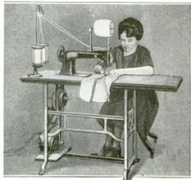
Operator Using Motor-Driven Lace-Sewing Machine Which Equals the Production of 12 Hand Workers
