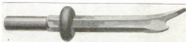
Flue-Beading Tool, Showing the Rubber Retaining Ring Which Prevents the Tool from Going into the Flue
