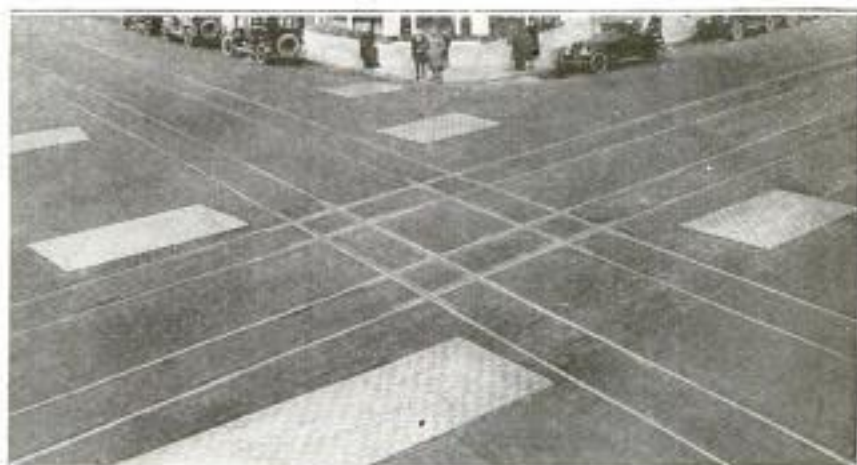
In Order to Show Its Wearing Qualities, Six Pieces of Floor Covering were Placed in the Path of Traffic at the Intersection of Two Busy Streets
