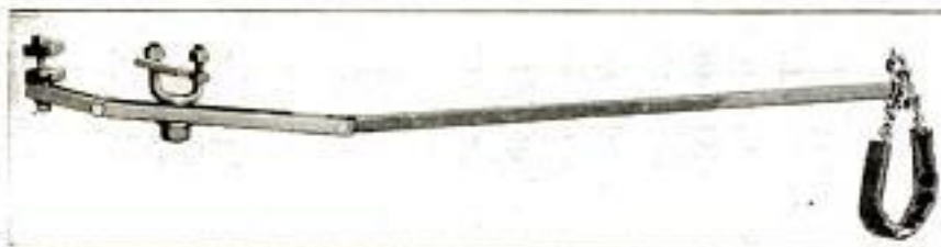
Automobile Towing Tongue Which Automatically Steers as Many Disabled Machines as the Wrecking Car can Pull Back to the Garage
