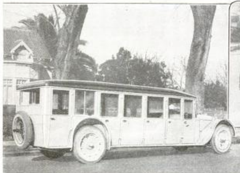
Left: "The Silver Fox" is Specially Designed for Passenger Service and has the Floor and Running Boards Placed Remarkably Low for the Convenience of Travelers. Above: The Extra-Wide Tread Makes for Easy Riding and Reduces Sidesway
