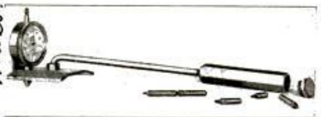
When This Gauge is Inserted in a Cylinder, the Diameter is Measured between the Contact Points, and Irregularities are Registered on the Dial
