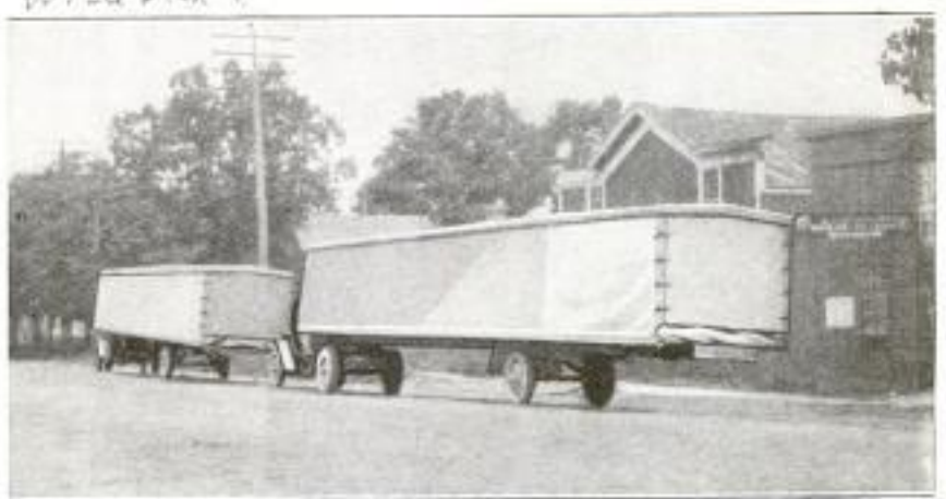
Specially Made Motor Trucks Having Long Canvas Covers, Shown en Route on One of Their Daily Trips from the Factory: Each Truck Contains Five Closed-Car Bodies
