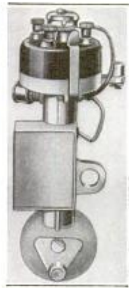
Mechanical Wiper That Enables the Motorman, by Slightly Turning a Handle within His Reach, to Keep the Window in Front of Him Clean in Bad Weather
