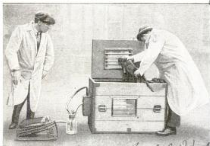
After the Sick Animal is Placed in the Box and the Air-Tight Cover Closed, the Anæsthetic is Forced In by Means of the Bellows
