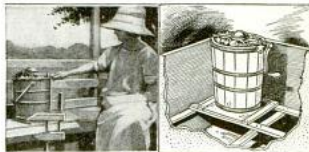
Two Methods of Holding the Ice-Cream Freezer Stationary: At the Left, a Board on the Bottom of the Freezer Allows It to be Clamped to a Solid Support; Right, the Wooden Frame inside a Laundry Tub
