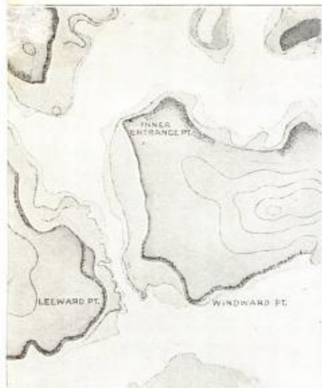
OFFICIAL NAVY PHOTO Left: The Hydrographic Map is Made by Surveying the Land and Making Soundings of the Water Near By. The Areas of Water of Different Depths are Shown by Different Shadings. Right: The Airplane Photograph of the Same Locality in Which the Areas of Shallow Water Appear of Lighter Shade than the Deep Water. The Photograph is Used to Check the Survey Map and to Discover Changes
