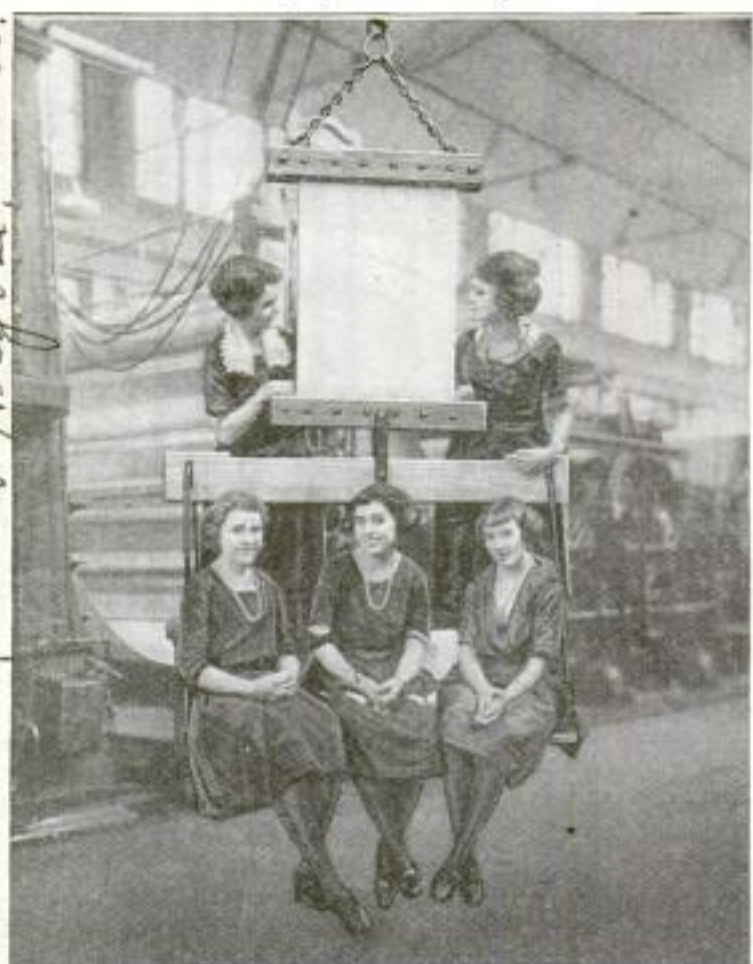
The Single Sheet of Paper is Supporting a Weight of 769 Pounds. The Young Women Seem to Have Perfect Confidence in Its Ability to Hold
