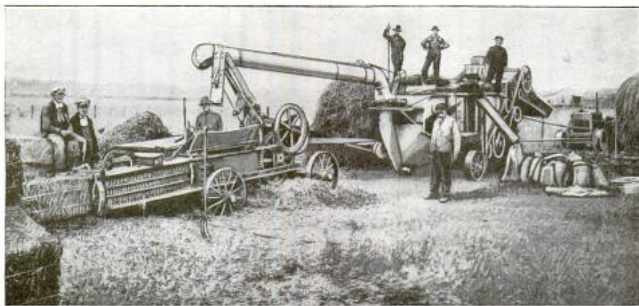
Combined Thresher-Baler, Showing the Manner of Placing the Units to Reduce Labor: At the Extreme Right is Seen the Tractor Belted to the Thresher, While at the Left is Shown the Baler Also Belted to the Thresher
