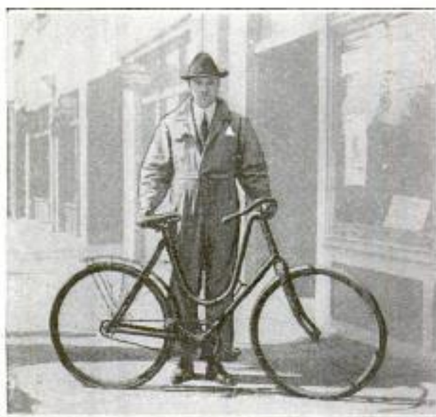
Nine Strips of Hickory Wood were Used in Making This Bicycle Frame, but They are So Skillfully Joined That It Has the Appearance of One Piece
