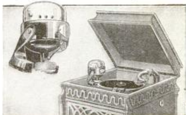
At the Upper Left is Seen the Small Motor with Rubber Pulley, or Wheel, While at the Right It is Shown Mounted on the Phonograph
