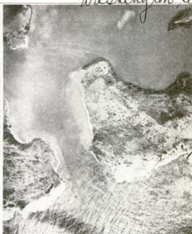
OFFICIAL NAVY PHOTO Left: The Hydrographic Map is Made by Surveying the Land and Making Soundings of the Water Near By. The Areas of Water of Different Depths are Shown by Different Shadings. Right: The Airplane Photograph of the Same Locality in Which the Areas of Shallow Water Appear of Lighter Shade than the Deep Water. The Photograph is Used to Check the Survey Map and to Discover Changes
