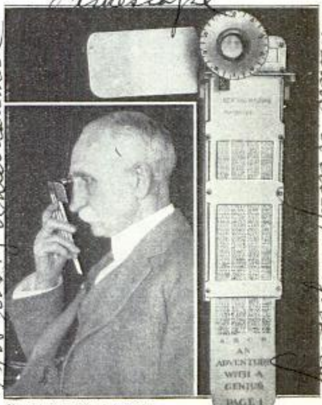
Reading Machine That Uses Reading Matter of Extreme Minuteness, as Seen in the Four Columns on Printed Strip in Its Aluminum Frame. Inset: The Inventor Showing How the Instrument is Used
