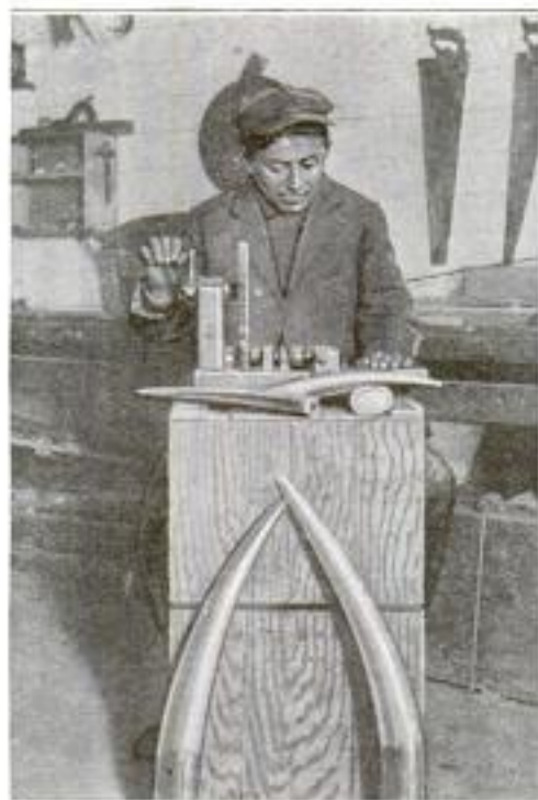
A Native Carver Cutting Beads with a Simple Lathe Which He has Made from Parts Salvaged from an Old Clock
