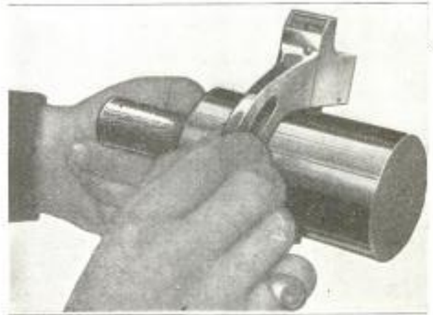
Gauge That Shows, with a Pointer on a Scale Graduated to .0001 Inch, Exactly How Much a Piece of Work Is over or under Size
