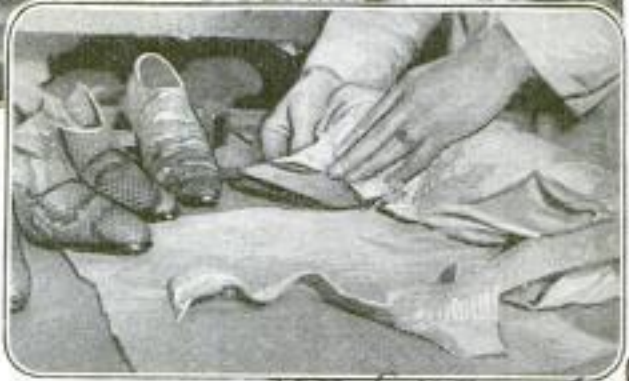
PHOTOS BY RADEL & BERBERT Above: Fish Skins being Cut Up and Fitted as a Substitute for Shoe Leather. Below: Ladies' Footwear being Made from the Skin of the Indian Python
