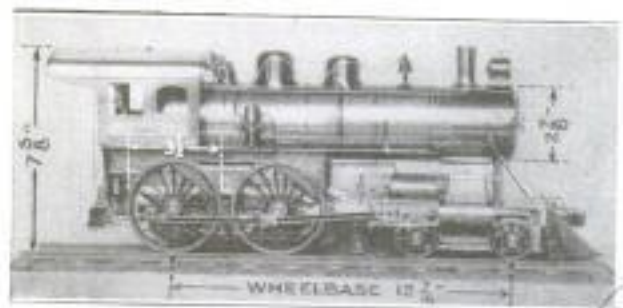
Constructed to Exact Scale, This Model Locomotive Burns Coal and Operates like the Standard-Sized Engine
