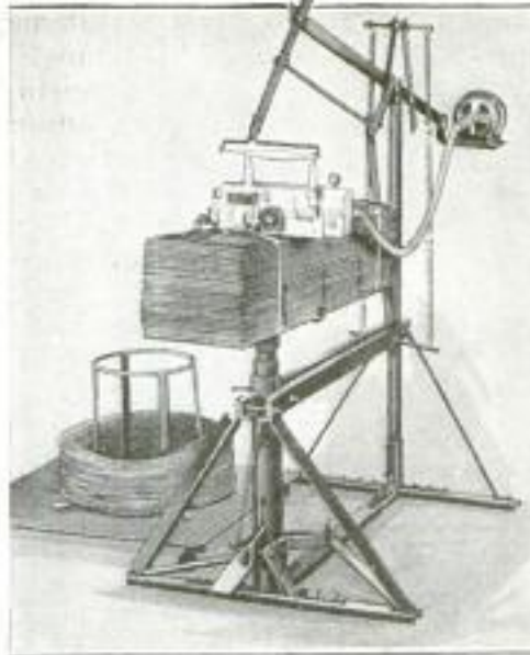
Complete View of the Binding Machine Together with a Coil of the Iron Wire Used: The Pedal Which Applies the Pressure to the Packages can be Plainly Seen
