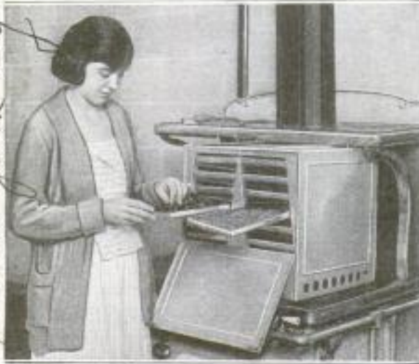
The Dehydrator Used on Top of Ordinary Gas Stove: This Type Has Six Shelves, Accommodating 12 Trays of Different Foods to be Preserved
