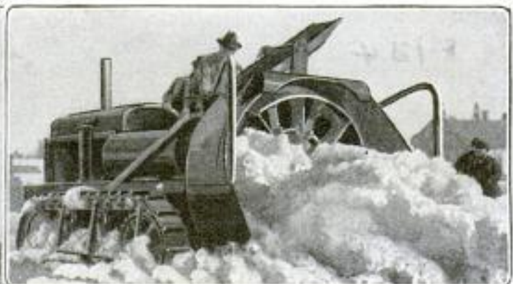
Above: The Rotary Snowplow is Combined into One Unit with the Tractor and is Driven by the Tractor Engine. As It is Forced Ahead, the Wings and Scoop Bank the Snow Up in Front of the Fan. Left: The Fan Cuts into the Snow and Throws It Clear of the Road by Means of the Deflector Mounted above the Fan
