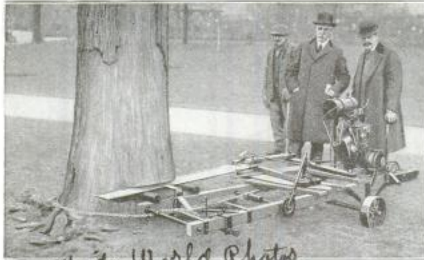
Tree-Felling Machine in Operation, Showing the Driving Motor and Also the Method of Chaining the Apparatus to the Base of the Tree to Provide the Pressure Necessary to Feed the Saw into the Trunk
