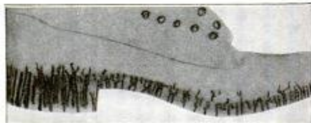
The X-Ray Photo Shows How Nails in the Shoes Form a Metal Path for an Electrical Current to the Ground
