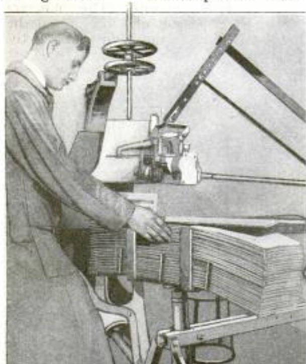
Binding Machine in Action: One End of the Bundle has been Tied and is being Swung Around So That a Wire can be Placed on the Other End
