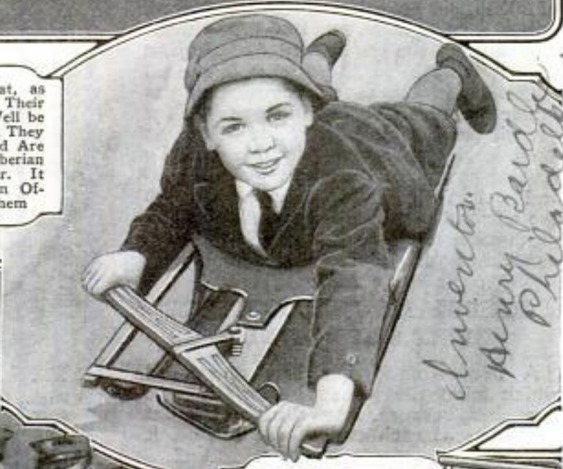
Sled That Has a Fifth Runner Which is Held from the Ground by a Spring on the Post: Pressure on the Handle Pushes It to the Ground into Convenient Position for Steering
