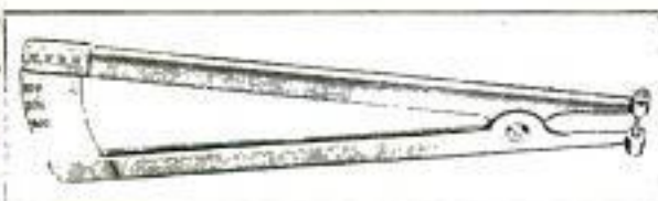
Thickness Caliper, Showing the Scale at the Left, and the Spherical Measuring Points at the Right
