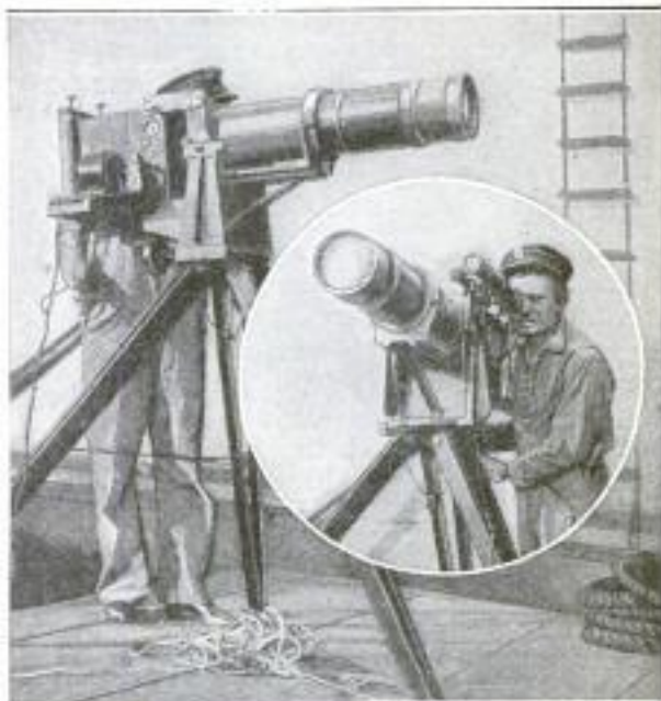
COPYRIGHT, UNDERWOOD & UNDERWOOD Long-Range Camera Set Up for Action on the Deck of a Ship: Insert Shows Photographer Using the Sighting Telescope to Get the Proper Range for the Camera the ordinary camera, unless the operator had exposed himself to the constant danger of being hit by the flying fragments of the high-explosive bombs.
