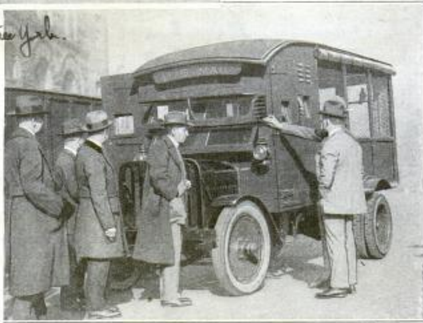
Copyright, Keystone View Co. 91-7th Ave New York. Above: The Truck Body Protected with Steel Plate with Portholes in Sides and End. Right: Truck, in Which Only the Driver's Compartment is Armored. Steel Cover Plates are Provided for the Windshield
