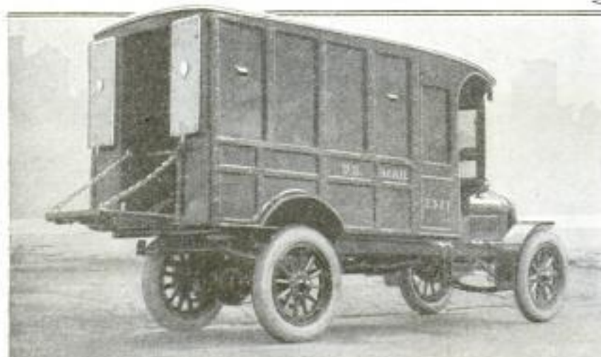
Copyright, Keystone View Co. 91-7th Ave New York. Above: The Truck Body Protected with Steel Plate with Portholes in Sides and End. Right: Truck, in Which Only the Driver's Compartment is Armored. Steel Cover Plates are Provided for the Windshield
