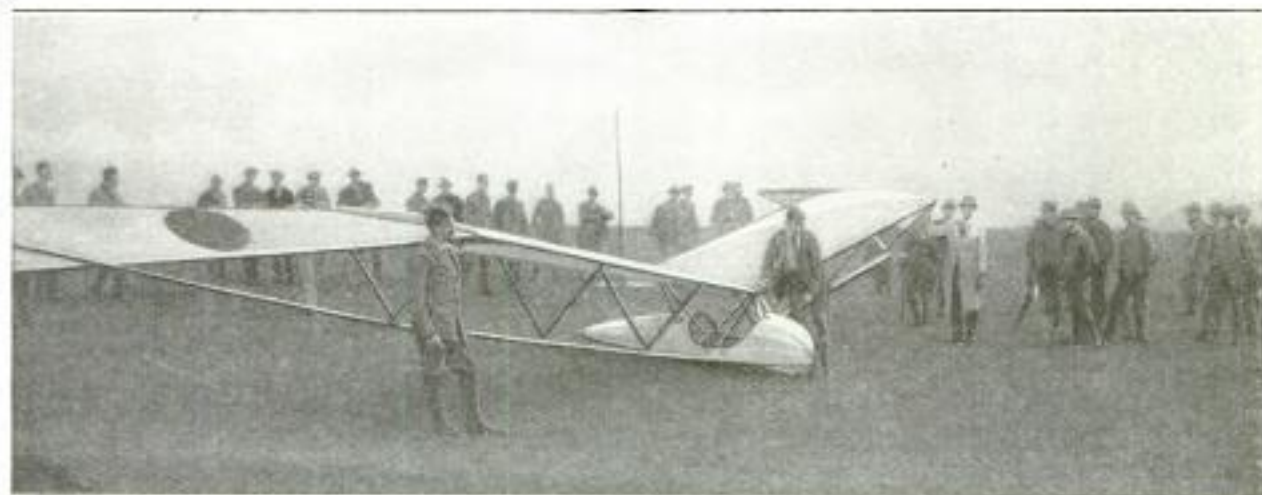
This Glider is of Extremely Light Construction and, Due to the Peculiar Form of the Wings, is Said to Possess a Remarkable Degree of Inherent Stability, in Spite of the Fact That No Tail Surface is Used
