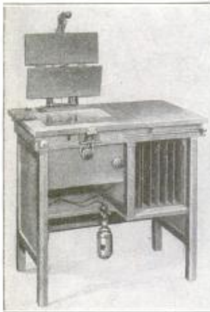
Photograph-Printing Machine, Showing the Two Hinged Sections of the Pressure Back: The Printing Bed is Clamped Down and below It can be Seen the Spotlight, While the Filing Cabinet is Shown at the Right End of the Apparatus. The Insert Shows the Ground-Glass Screen Exposed
