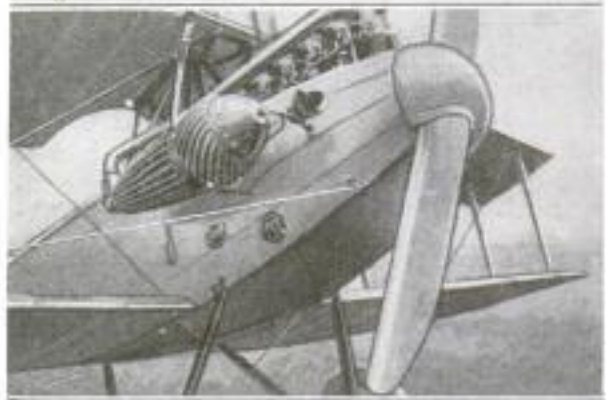
Above: Cross Section of the Silencer, Showing the Path of the Expanding Exhaust Gases. Below: When Running, the Blast from the Propeller Causes the Front Shell of the Silencer to Revolve Rapidly
