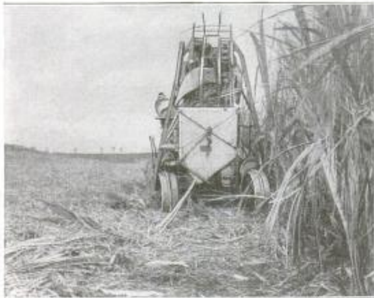
The Harvester, in Passing, Cuts the Cane Stalks at, or below, the Ground Line and Delivers the Cane, Free of Trash, to the Hopper at the Rear or to a Trailer
