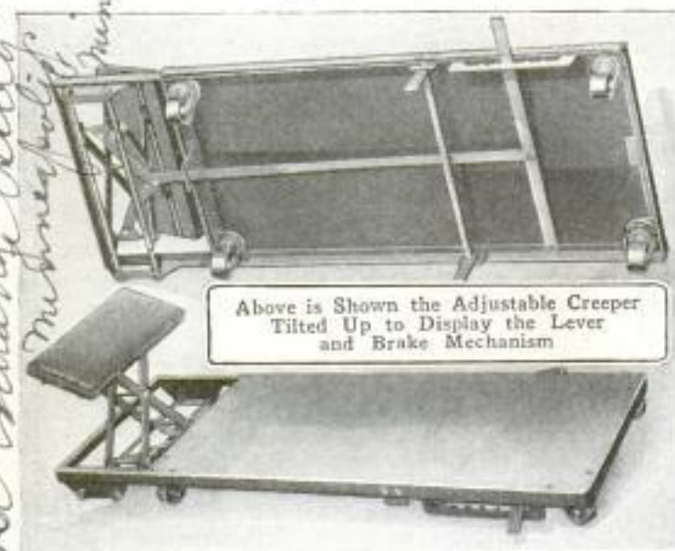
Adjustable Creeper with Headrest Raised, Showing How It Is Possible for the Mechanic to Work in a Comfortable Posture: The Operating Lever is Seen at the Side
