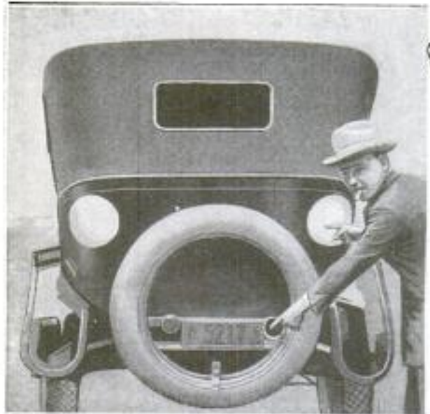
Two Aluminum Disks Placed on the Back of the Ton- neau Identify This Police Auto by Day, While an Extra Taillight of Blue Color Serves at Night
