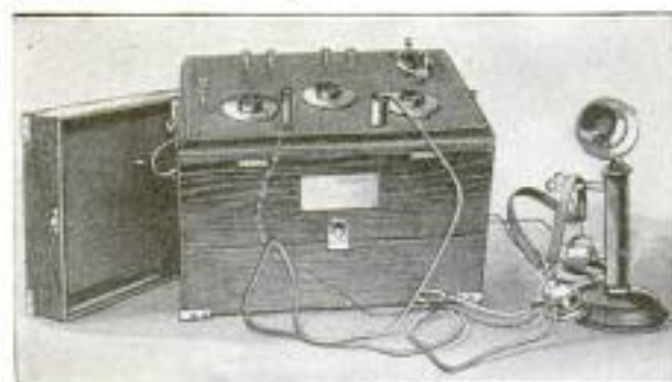
The Superphone Which can be Connected to Telephones in Homes or Offices: By Closing a Switch It is Put into Operation in Place of the Ordinary Phone
