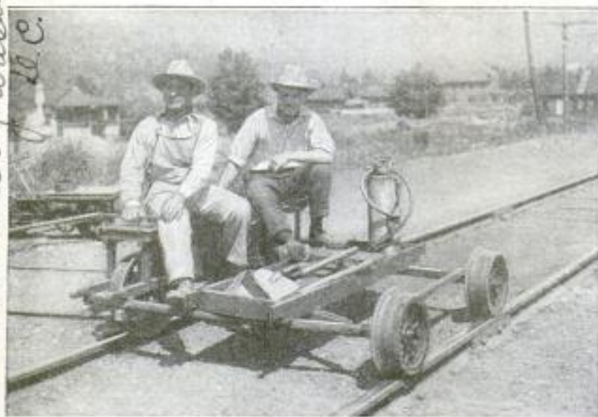
Members of Forest Service on Gasoline Speeder Equipped with Fire Extinguishers and Tools Patrol Railroad Right of Way and Put Out Fires Caused by Falling Sparks
