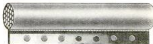
Weather Strip with Core of Cotton Wicking Wrapped with Rubber-Covered Cloth: It is Fastened with Tacks through the Perforated Selvage Which is Covered with Thin Metal
