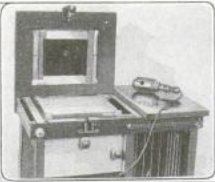
Photograph-Printing Machine, Showing the Two Hinged Sections of the Pressure Back: The Printing Bed is Clamped Down and below It can be Seen the Spotlight, While the Filing Cabinet is Shown at the Right End of the Apparatus. The Insert Shows the Ground-Glass Screen Exposed
