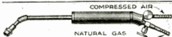
Natural-Gas and Compressed-Air Torch, Designed as Substitute for Other Torches, Where Natural Gas Is Available
