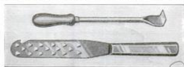
Top: Scraper for Removing Old-Battery Compound. Below: Knife for Separating Battery Elements
