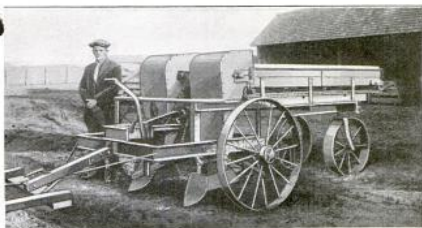
Machine for Planting Peppermint, Showing the Endless Belt Leading into the Hoppers, below Which can be Seen the Tool That Makes the Furrow
