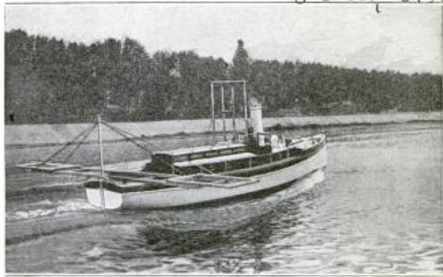
This Boat was Used in Making Experiments on the Seine River in Connection with the Magnetic-Cable Guide. The Receiving Frames are Seen at the Extreme Ends of the Apparatus on the Stern
