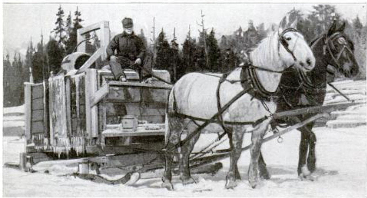
One of the Bobsled Road Sprinklers Used in the Northern Lumber Regions during the Winter Months, to Keep the Surface of Logging Roads Ice-Coated, So That Huge Sled Loads of Logs may be More Easily Hauled
