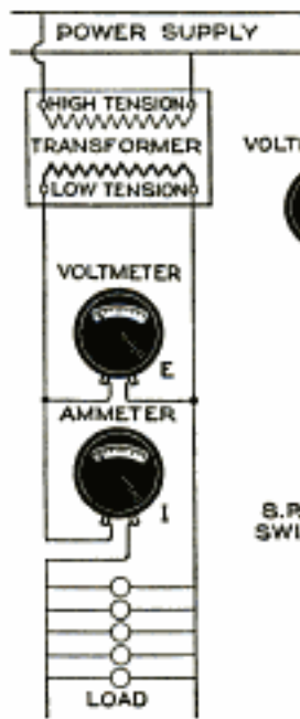
TEST FOR TEMPERATURE RISE
