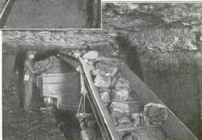
A Storage Hopper with a Conveyor Receives the Broken Coal from the Mining Machine and Loads It into the Mine Cars. By Using the Storage Hopper the Mining Machine may be Operated Continuously
