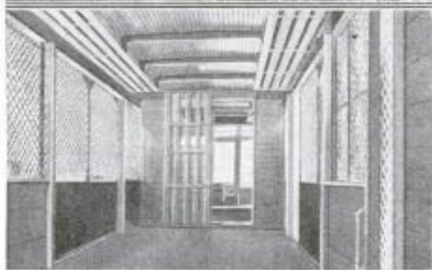
Above: One of the Truck Cars Used for Carrying Mail and Express in the Hetch Hetchy Valley. Left: Interior of the Combination Mail and Express Car. Right: The Dashboard is Raised to Accommodate a Brake Ratchet
