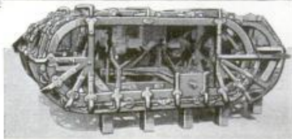
Side View of the Tractor, Which Illustrates How the Machine Has Four "Feet" on Each Side to Rest Upon
