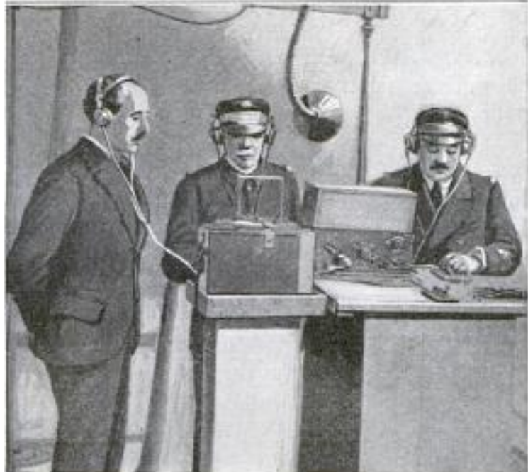
Listening to the Sounds Made by the Impinging of Electrical Waves upon the Receiving Frames of a Large Airplane: The Speaking Tube Shown Terminates at the Pilot's Station
