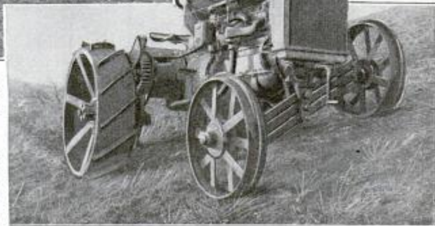
Another View of the Hillside Tractor, Showing the Front Axle Which Works on the Parallelogram Principle in Maintaining the Level of the Machine Constant
