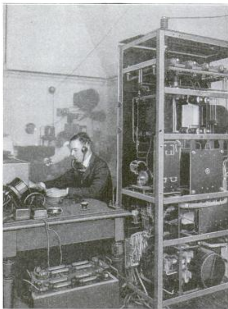
Copyright, Harris & Ering Specially Designed Radiotelephone Transmitting Outfit for Broadcasting Weather and Market Reports, Occupies Small Space, and is Arranged for Either Local or Remote Control
