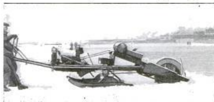
One of the Gas Ice-Cutting Machines, Which have Supplanted Horse-Drawn Machines in the Northern Mississippi Valley: They can be Used on Ice Too Thin to Bear the Weight of Heavy Teams
