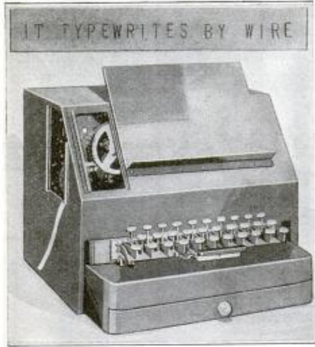
Combined Receiving and Sending Unit: The Receiving Tape Protrudes from the Left Side. A Full-Size Section of Tape is Shown Above
