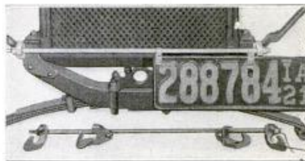
The Radiator-Repair Bolt, and, Above, the Method of Attaching It to a Broken or Leaky Radiator
