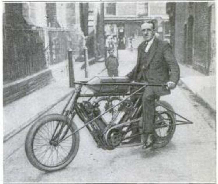
The New 20-Horsepower Motorcycle Built by an English Motorcycle Racer for the Purpose of Breaking the World-Cycle Pacing-Track Record
