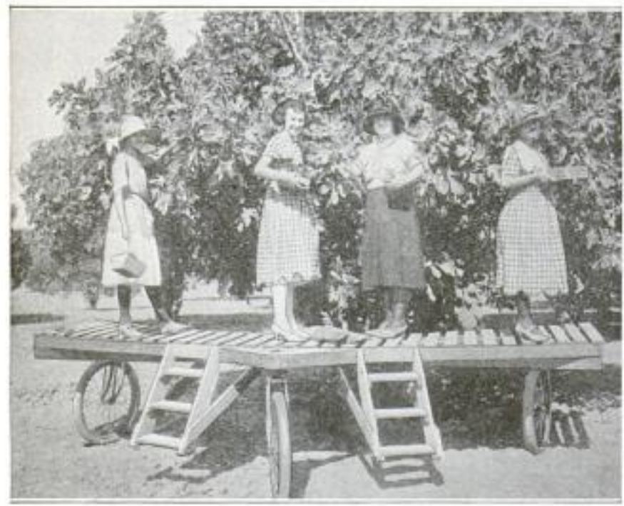
Three-Wheeled Platform, Designed for the Purpose of Picking Figs, and with Which Four Pickers can Strip a Tree of Its Fruit in Much Less Time Than would Be Possible by Using Ladders
