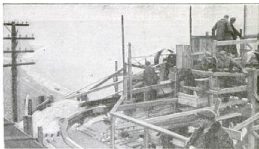
Elevating and Loading Machines for Conveying to Railroad Cars, on the Burlington, Ice Cut on Lake Pepin, in the Northern Mississippi Valley. Which on Account of Its Size, Is a Good Place for Harvesting Ice
