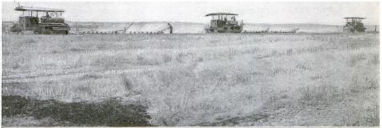
Part of a Battery of Tractors Hauling Rotary-Disk Plows over the Reclaimed Bed of Tulare Lake in the Fall, After the Season's Crop had been Harvested: Deep Plowing Is Not Necessary, and the Disks Turn Over the Top Crust, Providing a Satisfactory Seed Bed
