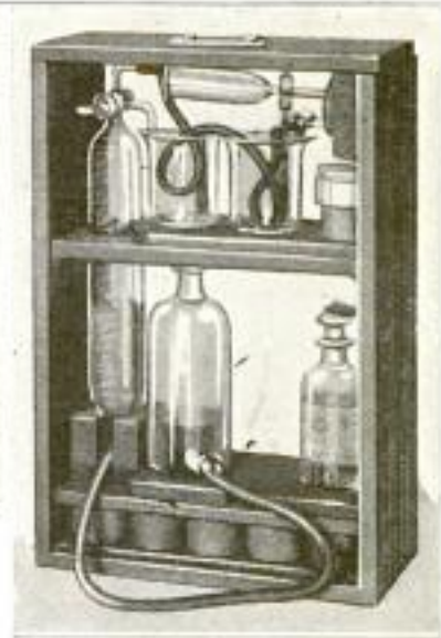
Determining the Weight of Galvanized Coating: The Acid-Resisting Ring Is in Place with the Tubing Connecting It to the Burette in the Cabinet. The Leveling Bottle is being Held at Measuring Level. At the Right, the Apparatus is Shown in Its Cabinet
