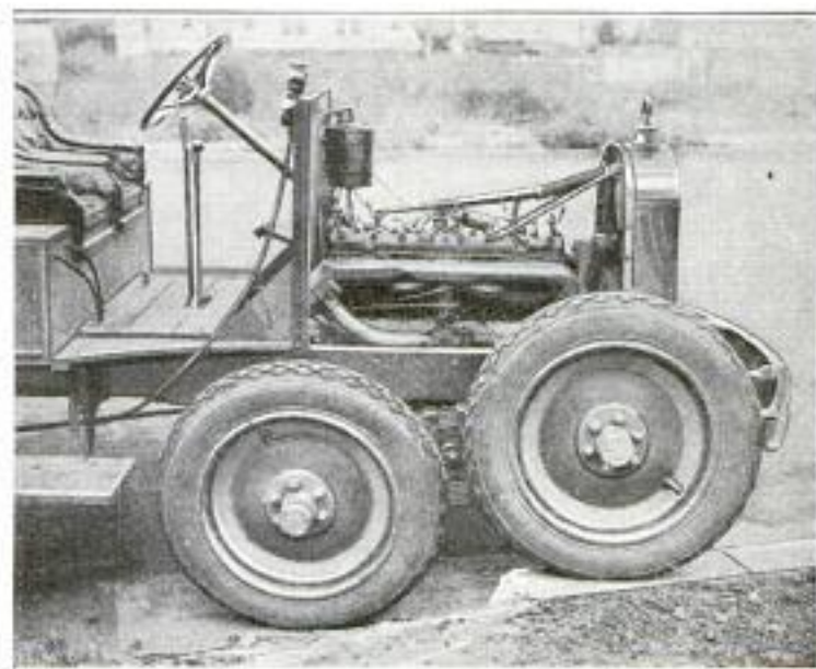
Front Truck of the Eight-Wheeled Motor Bus, with One Wheel Resting upon a Curb, Graphically Illustrating the Remarkable Flexibility of the Axle Arrangement
