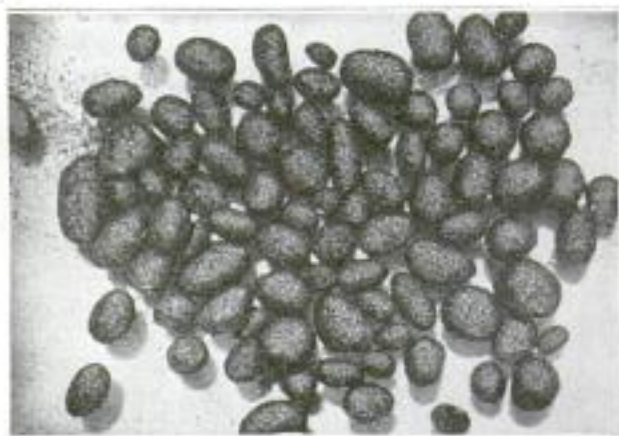
Amalgam Granules, Varying in Size Down to About One-Eighth Inch in Diameter, the Final Product Obtained in Reclaiming Coal
