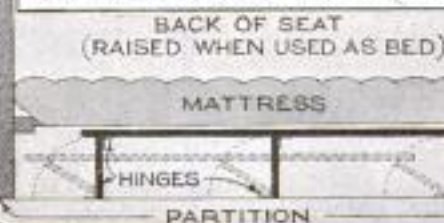
This Diagram Shows the Hinged Support Used under the Seat-Bed Springs, to Control Their Rigidity
