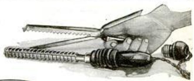
For Marcelling the Hair, the Lower Instrument is Electrically Heated and Thrust into the Hair. The Upper Instrument is Then Tightly Squeezed over the Hair Surrounding the Heated Part
