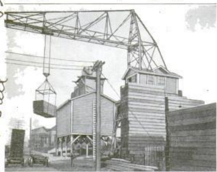
The Outside Crane, Used in Moving Heavier Lumber Which can be Stored Outdoors: The Crane Is Just About to Place Its Load upon the Delivery Truck
