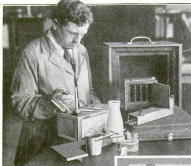
Above: Placing a Drop of Milk, Together with Germ Food, on a Glass Plate. The Small Case with Numerous Shelves for Holding the Plates is Seen in the Background. Below: Amount of Glassware Required by Old Method at Right, and at the Left, the Few Pieces Needed with the New Cabinet
