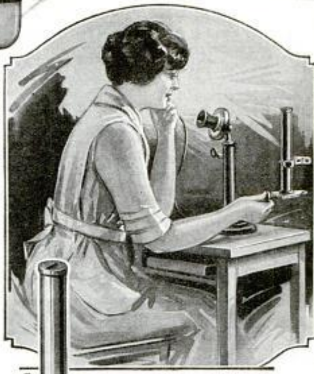
A Telephone-Slug Holder, with Which the Subscriber Always Has the Necessary Means Handy to Operate the Telephone in Case of Emergency Instead of Frantically Searching for a Nickel
