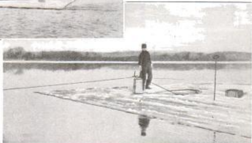
The Block and Pulley, over Which the Cable Runs, are Anchored to the Ice by a Rope and Plank, Dropped through a Hole in the Cake
