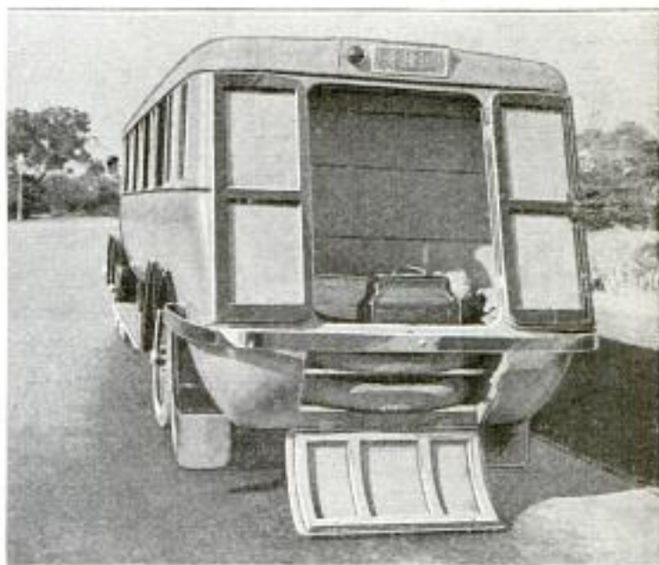
Rear End of the Eight-Wheeled Motor Bus, Showing the Compartment for Accommodating the Baggage of the Passengers and the Spare-Tire Compartment Just Below
