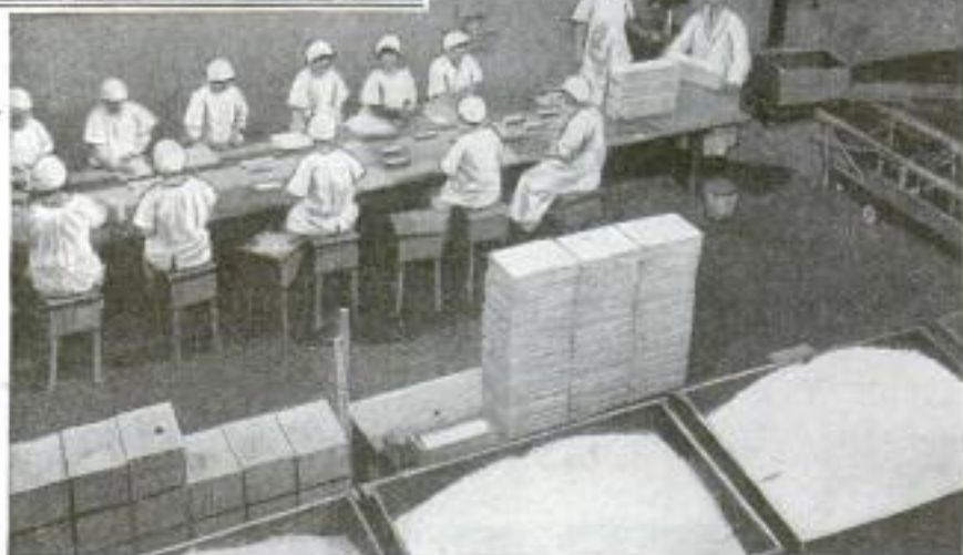
After being Cut into One-Pound Bricks, the Finished "Butter" is Placed on an Endless Belt Which Moves down the Center of a Wrapping Table. Girls, Sitting along the Table, Pick the Bricks from the Belt and Wrap Them
