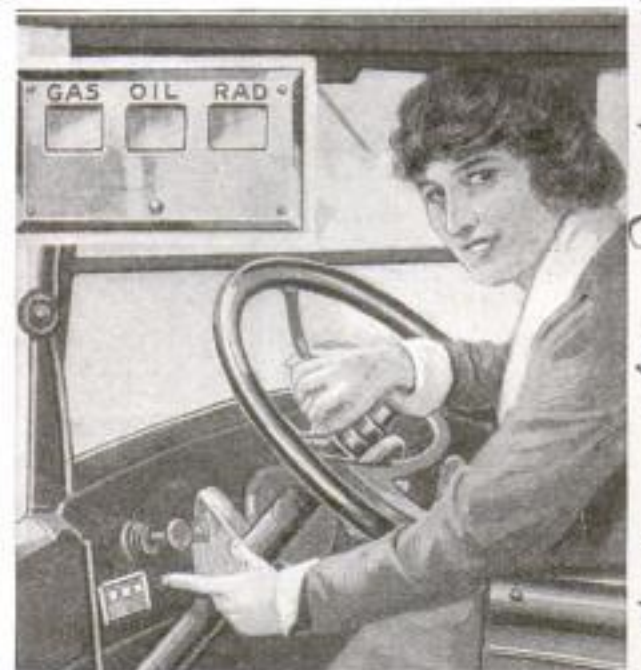
Three Small Windows on Auto Dash, in Each of Which a Red Light Flashes, Warning the Driver of Lack of Oil, Gas Shortage, or Overheating of the Radiator
