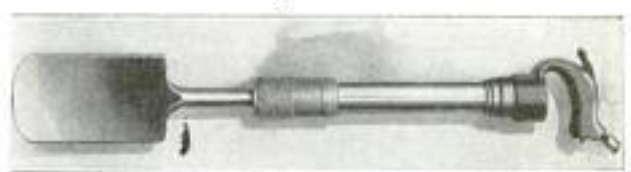
Clay-Digging Tool That Is an Adaptation of a Pneumatic Riveting Hammer, with a Spade in Place of the Hammer: It Strikes 800 Blows a Minute
