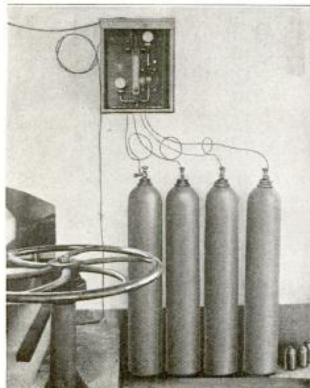
A Chlorinator of the Type Commonly Used for Water Purification, but Modified for the Purpose of "Gassing" Bad Odors
