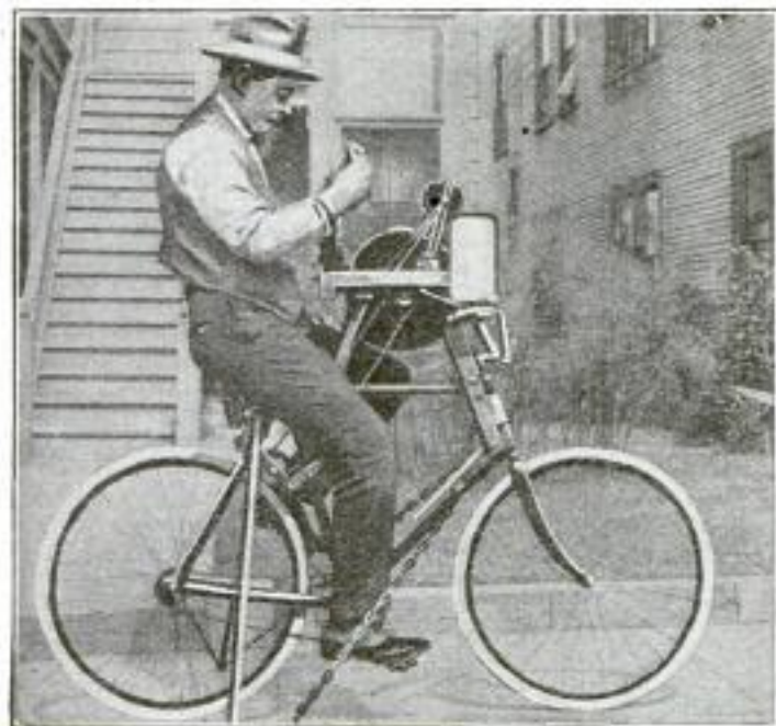
A Tool and Knife-Grinding Outfit Mounted on a Bicycle, the Rear Wheel of Which is Raised by Long Rods: The Upper Photograph Shows the Rods Extended; the Lower Picture Illustrates How the Rods Fold Out of the Way
