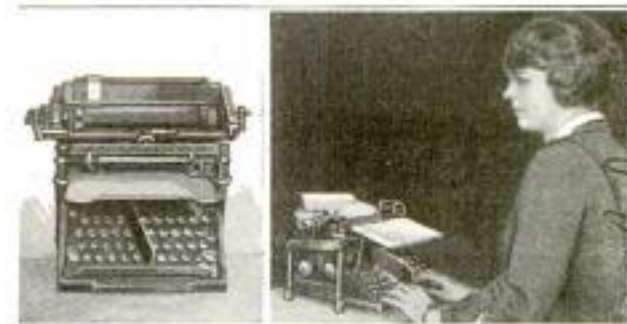
Keyboard Shield and Divider, Attached to a Typewriter, at the Left: The Shield may be Used to Support a Notebook, as Shown at the Right
