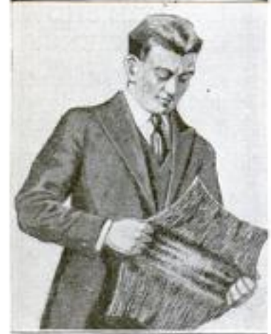
This Type of Paper will Stretch to Shape for Lining Barrels
