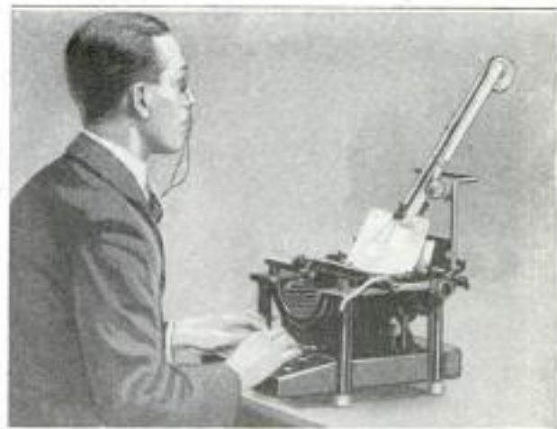
This Device, Attached to the Carriage of an Ordinary Typewriter by Means of the Bracket, Enables a Blind Person to Control the Machine
