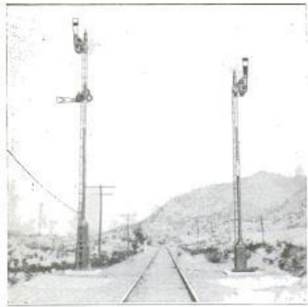
Two Samples—One with Single and the Other with Double Semaphores—of the New Railway Signal That Rises, Instead of Falling to a Horizontal Position, to Indicate Safety
