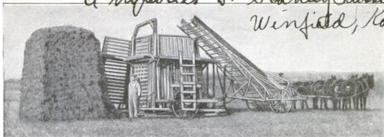
A Stack has just been Completed and Slipped Out of the Bin of the New Hay-Stacking Machine. One of the Rear Gates is Still Open, but the Nearer One has Swung Shut. The Sloping Sides of the Bin Give the Stack the Necessary Pitch to Shed Water When It Rains
