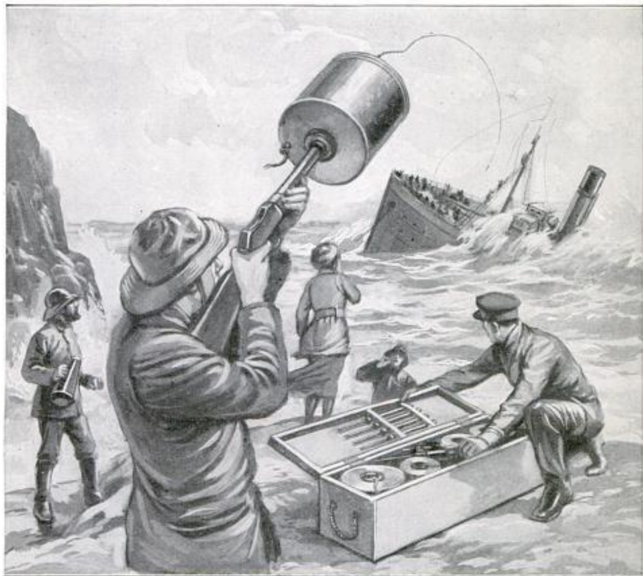
The Portable Line-Throwing Gun in Use: No Matter Where It is Needed, It Quickly Meets the Emergency, For It Requires No Permanent Base or Other Preparation. The Box Contains Extra Cylinders of Line, Projectiles, and Cartridges, Complete Equipment for Every Need
