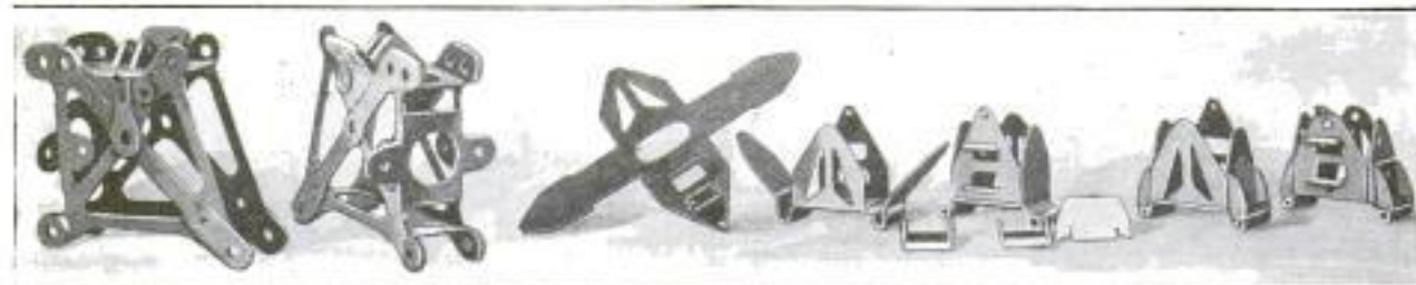
Airplane Wing-Beam Hinges, in Various Stages of Completion, are Shown at the Left. The Smaller Forms at the Right Are Parts of a Box Fitting. After Welding, These Forms are Dip-Brazed and Heat-Treated. They must Have Great Strength and Resiliency, the Box Fitting, for Example, Carrying the Stresses from 10 Timbers
