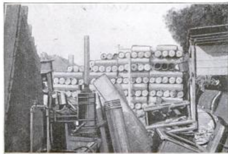
Section of the Plant Where Water Tanks and Heaters are Salvaged: Parts of Stoves and Ranges Which Are Still Good are Saved to Replace Worn-Out Parts in Others
