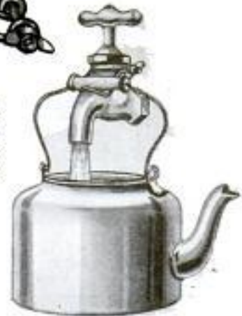
To Hold a Kettle under the Faucet While Filling It, a Small Wire Device Is Convenient. It may be Fitted to Any Faucet by Tightening or Loosening the Wingnut
