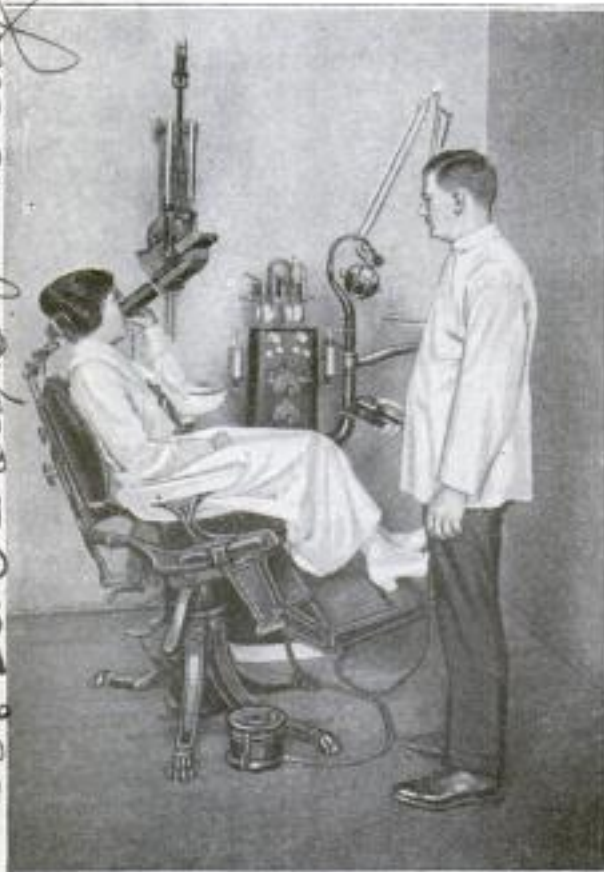
Using the Midget X-Ray Apparatus for Dental Work: The Patient is Seen Holding the Focusing Cone to Her Face to Concentrate the Rays
