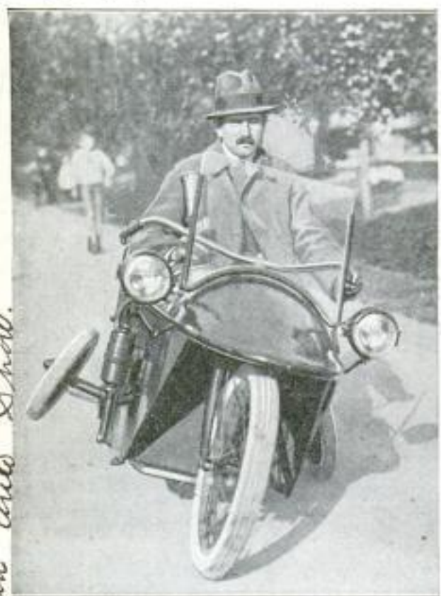
The Antiskid Motorcycle with a Body Built on It, in the Act of Making a Turn: The Small Wheel to the Right is Seen Touching the Pavement, Thus Preventing a Fall or Skidding
