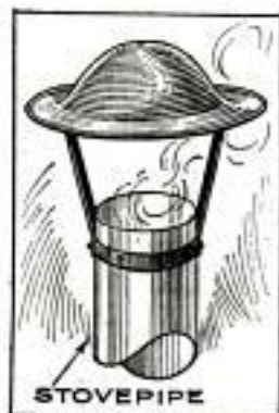
A Helmet Cap on the Stovepipe Prevents Rust and Down Draft
