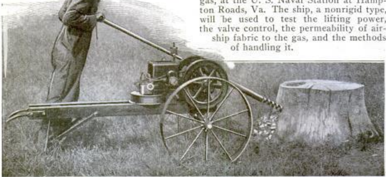
Portable Machine Equipped with a Kerosene Engine for Driving an Auger That Bores a Two-Inch Hole through a Three-Foot Tree Stump in 30 Seconds: The Auger is Started or Stopped at Will by a Lever-Controlled Clutch. The Handle Is Long, So as to Balance the Weight over the Axle
