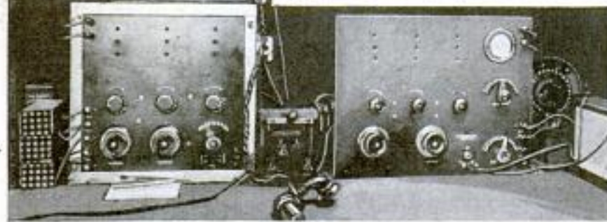
At Department Headquarters, This Radio Set is Used to Keep in Communication with the Chief, through the Set on His Machine, When He Is at a Fire
