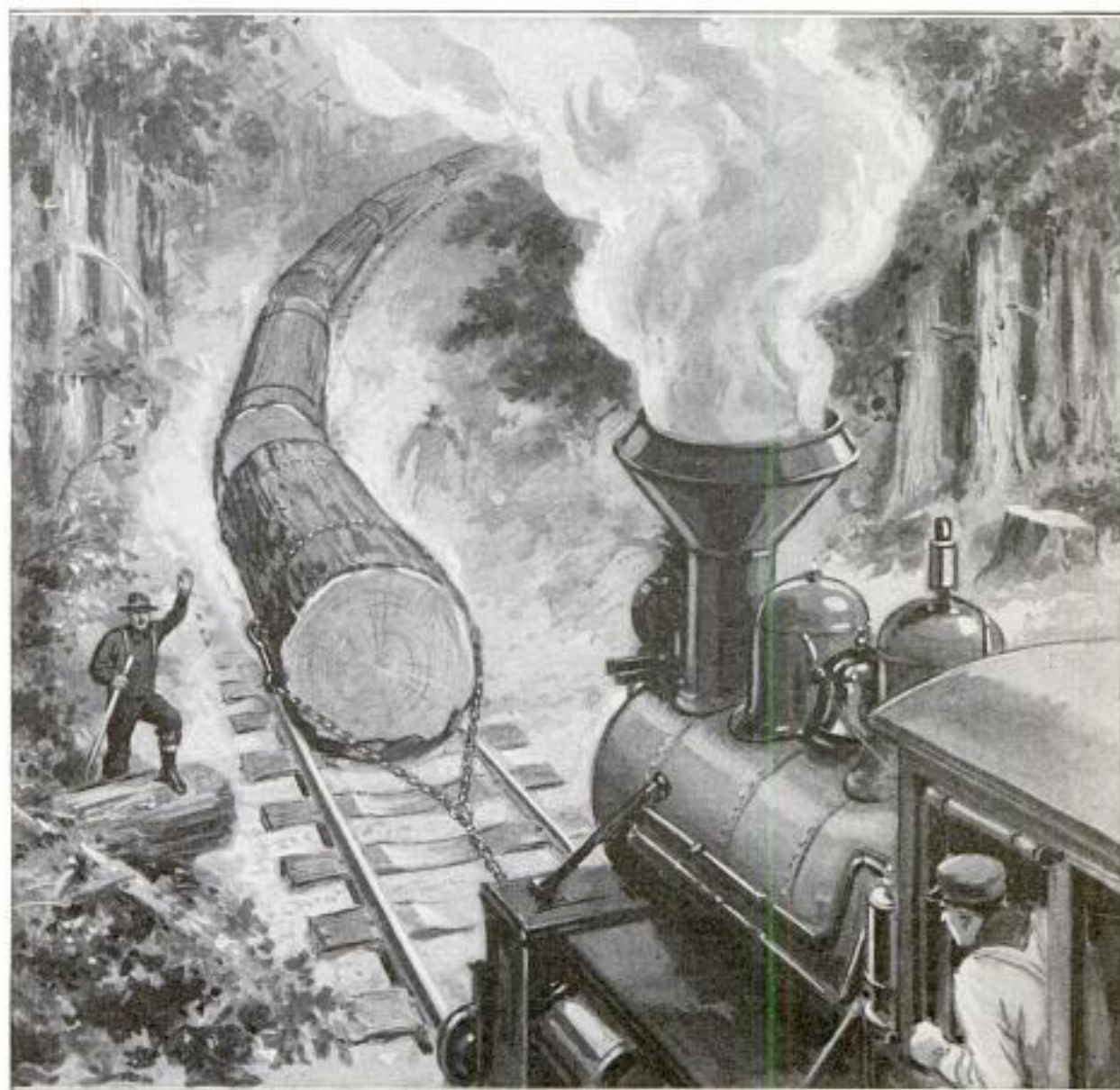
Skidding Logs to the Mill without Loading onto Cars: The Engine Hooks onto a String of 20 Logs and Hauls It along a Skidway between the Tracks. This Method Is Both More Rapid and More Economical Than the Usual Method of Hauling on Flat Cars, Especially in Rough Mountain Country
