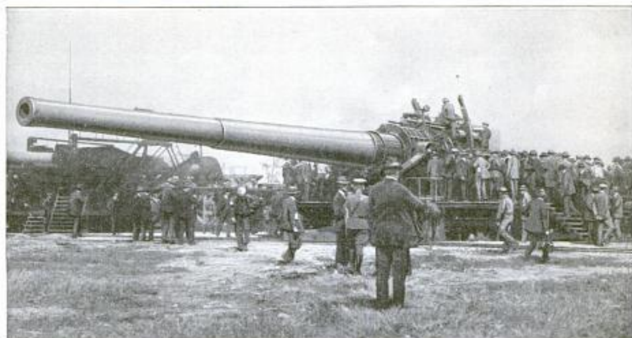
Ordnance Experts Examining the New 50-Caliber 16-Inch Rifle at the Aberdeen, Maryland, Proving Grounds: Tests Demonstrated It to Be the Most Powerful Gun in Existence. It is Mounted on a Barbette Carriage, and is Elevated and Turned Laterally by Electric Appliances. It Has a Calculated Range of 35 Miles
