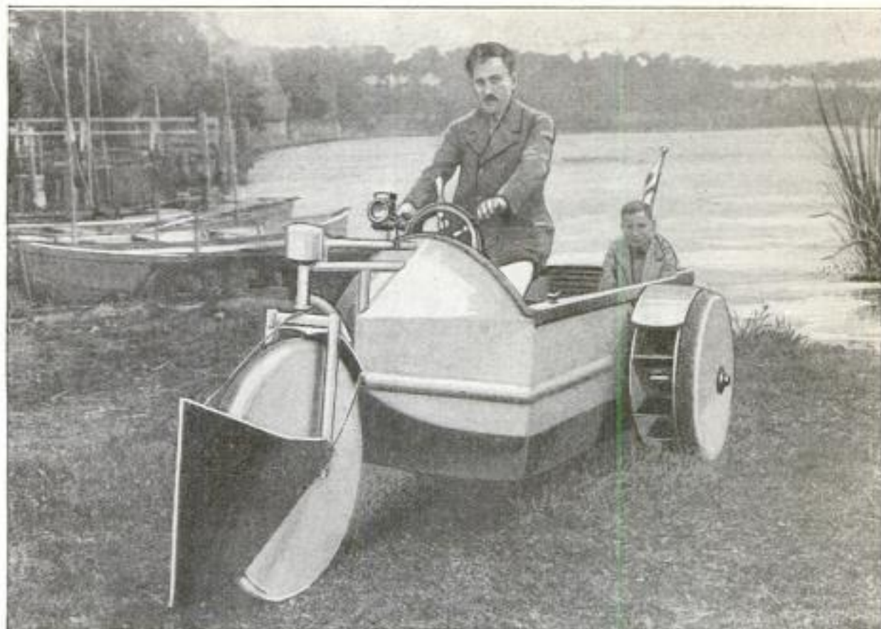
The Automobile-Boat has Just Emerged from the Water. The Method of Mounting the Paddles upon the Rear Wheels can be Seen Clearly Here, as Well as the Mounting of the Front Wheel
