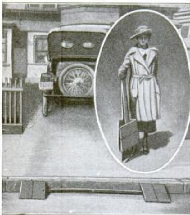
The Manner in Which the Portable Runway is Placed for Use: The Insert Shows Runway Folded in Middle, Which Permits It to be Carried in Car
