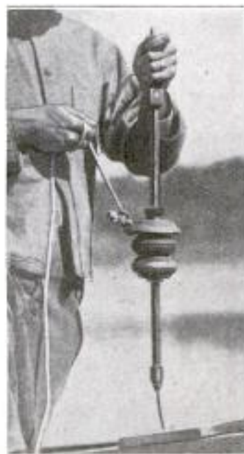
Device for Snagging the Logs: It is Fastened to the End of the Lifting Cable. The Large Nail at the Bottom is Driven into the Log by Letting Fall the Sliding Weight on the Rod
