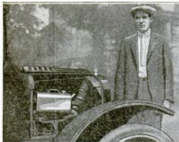
The Hood of the Car is Raised to Show How the Coffee Cooker Fits onto the Exhaust Pipe. This Was the First Utensil Made
