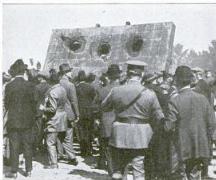
Crowd of Ordnance Experts and Others Viewing the Holes Made in a Heavy Armor Plate by Three Projectiles from the New 16-Inch Naval Gun: On Account of Hazy Weather It could Not be Tested for Its Extreme Range
