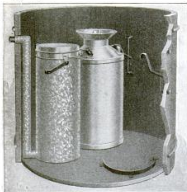
Newly Separated Cream is Cooled in the Closed Can inside the Open Galvanized Tank, and is Then Placed in the Storage Can beside It
