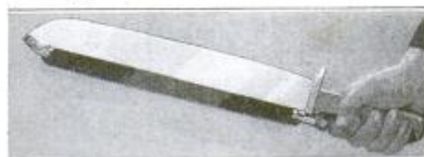
The Saw Blade is Held Tightly against the Back of the Knife by a Thumbscrew, Placed at the Hilt of the Knife
