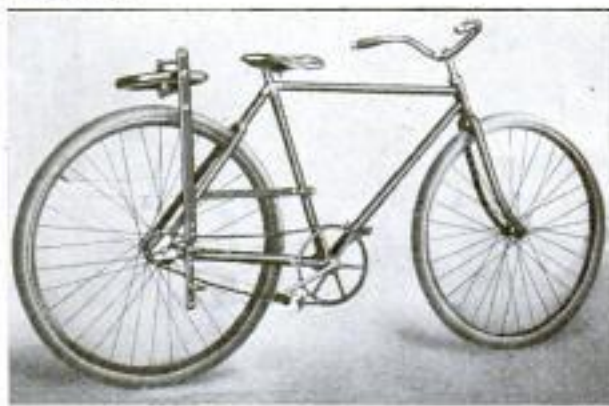
This Bicycle Sidecar Attachment, for Carrying Bundles, can be Folded Out of the Way, as Shown at the Right, When Not in Use
