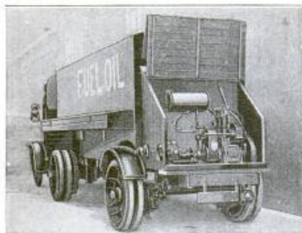
A Two-Cylinder Marine-Type Engine is Placed at the Rear of the Oil Truck to Operate a Gear Pump for Filling the Tank
