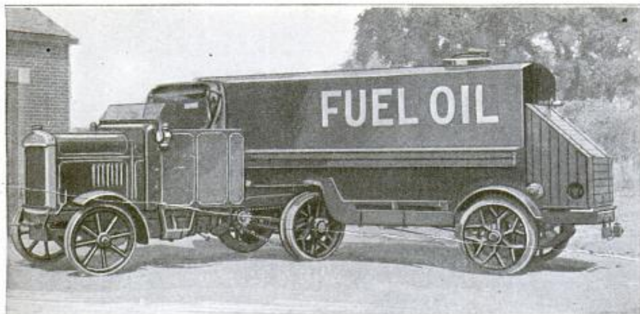
The Oil Tank Mounted on the Trailer Portion of a Six-Wheeled Truck Unit, for Transporting Heavy Oils: The Mounting is So Arranged That the Truck can be Turned in an Even Smaller Radius Than Indicated by This Illustration. The Dropped Frame Gives the Unit Stability
