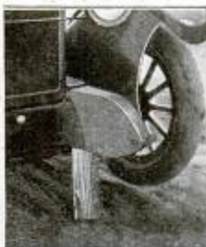
A Simple Method of Raising an Automobile Wheel for Removing a Damaged Tire, When No Jack Is Available
