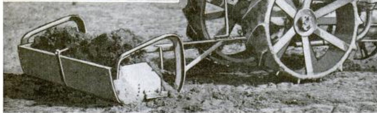
Above Is a Scraper Drawn by a Tractor and Equipped with a Hitch Operated by a Hand Lever. In the Insert the Construction of the Hitch is Shown in Detail
