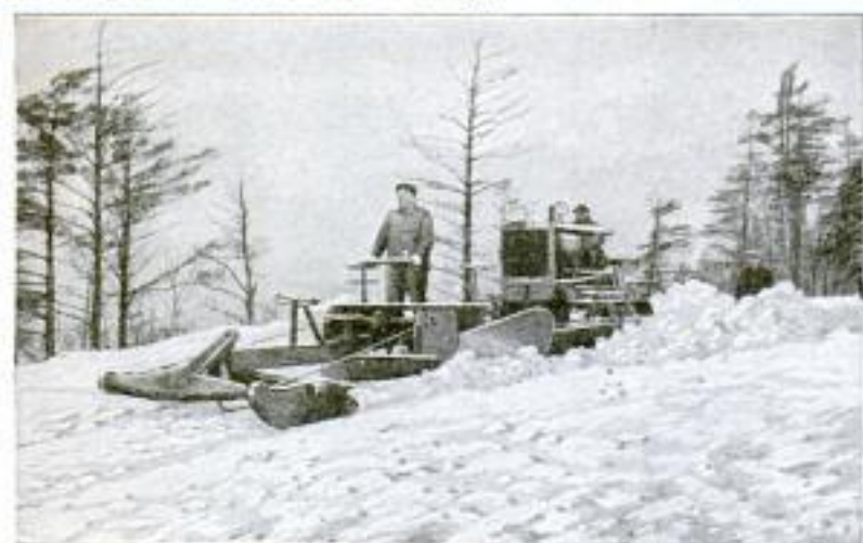
Snowplow in Front being Pushed by the Tractor Behind: The Man on the Plow Sets the Outboard and Another Man Runs the Tractor
