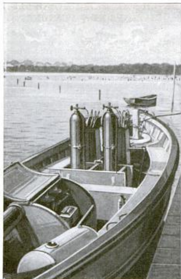
The Launch Equipment, Shown at the Left, Consists of Tanks Containing Chlorine Gas, and Others in Which the Gas is Mixed with Water. The Mixture is Used to Purify the Tidewater of a Bathing Beach at Washington, District of Columbia. At the Right, the Launch is Seen Circling the Beach during the Purifying Process
