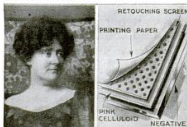
At the Left: A Photograph Showing the Effect of the Retouching Film. At the Right: The Negative, Film, and Paper Arranged for Printing
