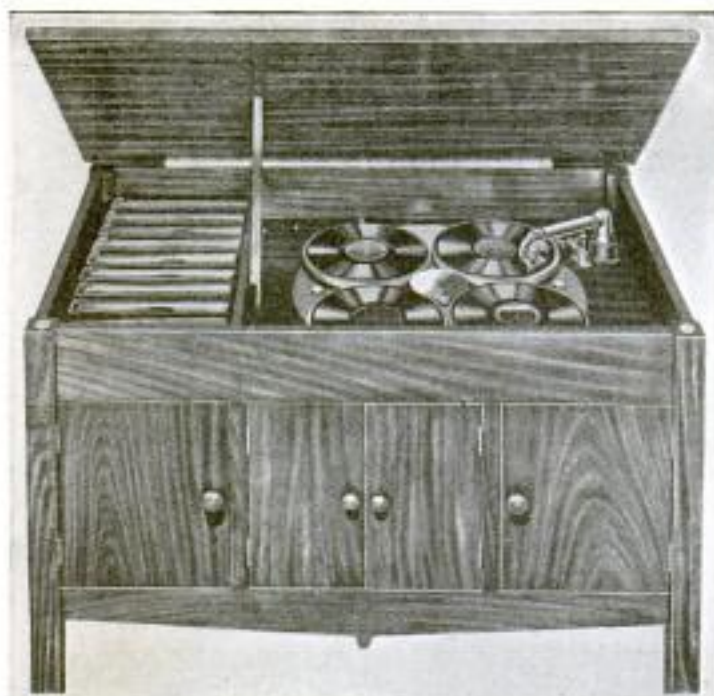
The Larger Disk, Supporting the Four Record Tables, Moves the Latter Slowly While the Record is Playing. When the Piece is Finished, It Rotates Quickly and Sets Another Record for Playing
