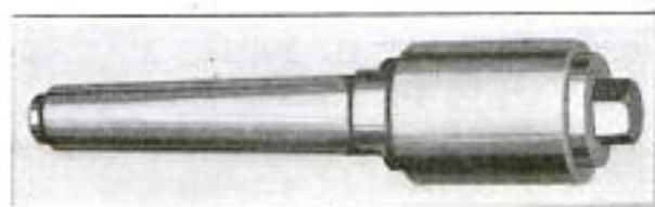
Left: Blank on Its Work Arbor with Tapered Shank and Thrust Collar, Ready for Shaper Which Cuts from It the Gear Shown to the Right
