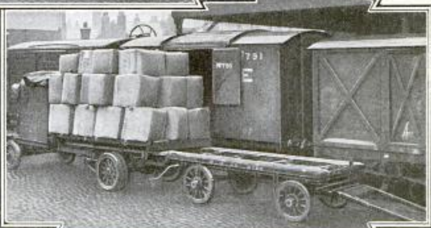
Above: The Loaded Car being Rolled from the Tender onto the Truck. This is Done with a Hand Windlass or with a Windlass Operated by the Truck Motor. It is This Quick Loading, Making Possible Utilization of the Full Time of the Truck, Which Makes the Device Valuable
