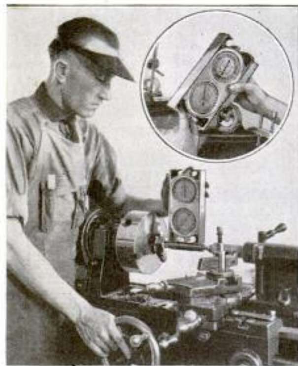
Angle Indicator Which Gives Accurate Readings for Precision Work in Machine Shops, Shown in Setting Up Lathe, and Above, Setting a Machinist's Protractor
