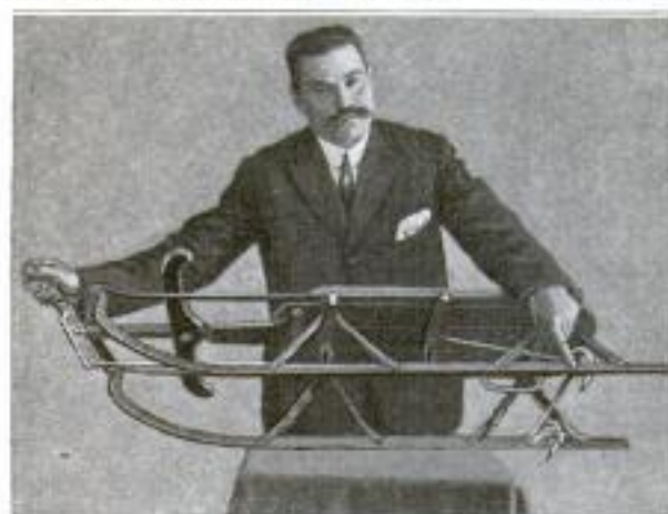
A Sled with the Safety Device Attached: The Sharp Hooks Operated by the Lever at the Front Form a Most Effective Brake
