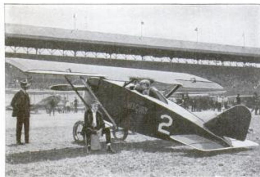
Although Equipped with Only a 90-Horsepower Engine, This Tiny Plane Made 130 Miles an Hour. Its Wing Measures 21 Feet 9 Inches
