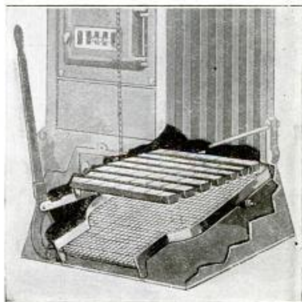
The Unburned Coal Falls to the Cellar Floor or into a Receptacle in Front of the Sifter
