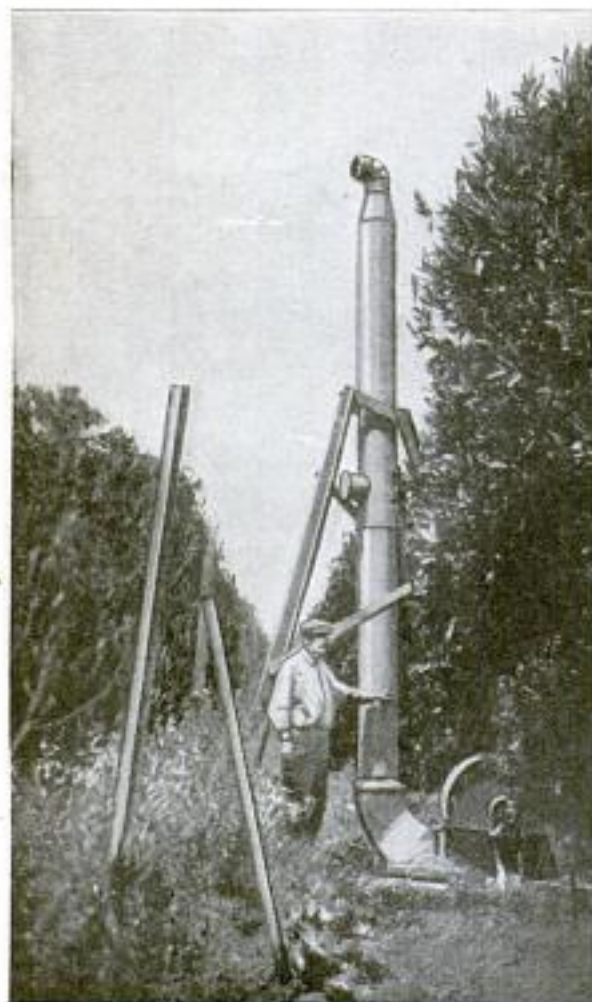
The Apparatus Which Mixes Upper and Surface Air to Protect Citrus Orchards from Frost
