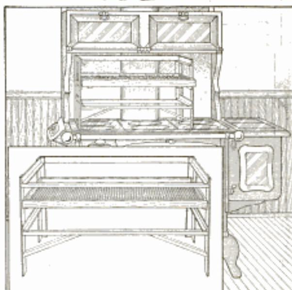
A Homemade Fruit and Vegetable Drier That can be Set on Top of the Kitchen Range or Inserted into the Oven
