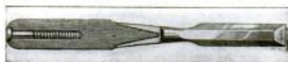
A Nonsplitting Chisel Handle: The Cavity between the Screw and the Bore of the Hole is Filled with Cement, Which Cushions the Driving Blows
