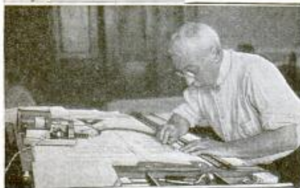
A Motor-Driven Eraser for the Drafting Room Made from the Electric Motor of an Old Dictating Machine with a Flexible Shaft and Holder from a Dentist's "Engine"
