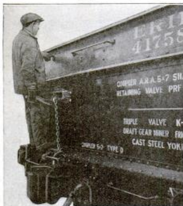
Ratchet Hand Brake for All Types of Freight Cars, That Leaves One of the Operator's Hands Free for Holding Himself onto the Car, and is Operated by Pulling the Lever Upward, So That the Harder He Pulls, the Firmer Is His Footing
