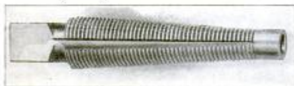
By Tapping on the End of This Tool After Its Threads have Taken a Grip in the Bushing Metal, the Bushing will Come Out Easily
