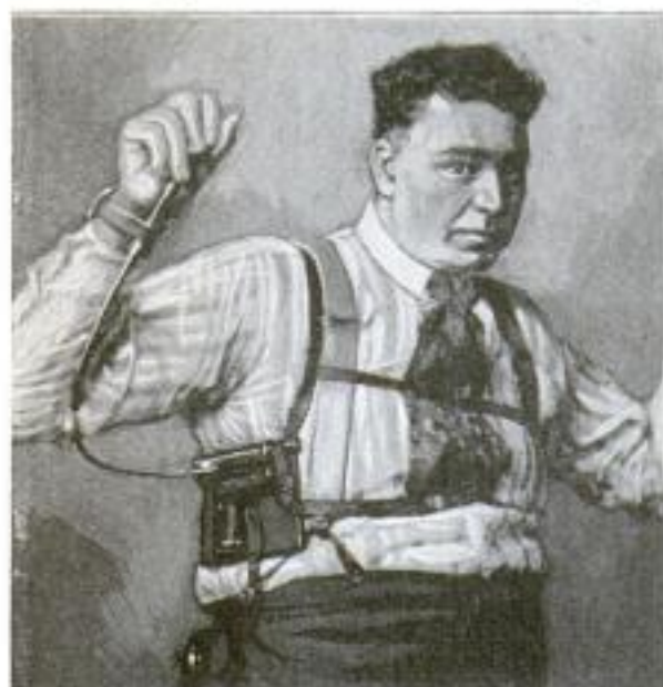
The Gun Strapped to the Teller's Side may be Fired by Operating a Bulb Held in the Hand
