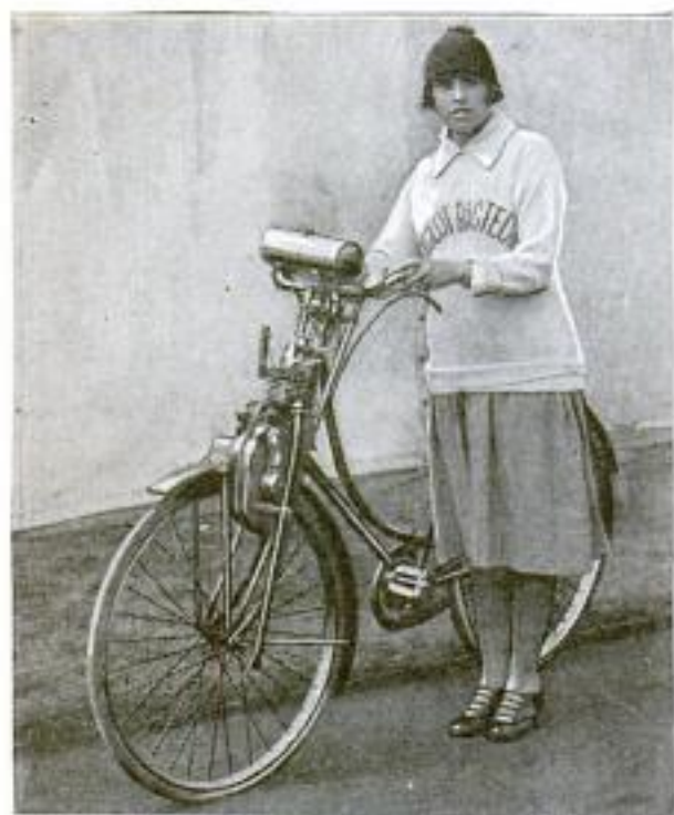
The Smallest Gasoline Motor: It Drives a Bicycle at 20 Miles an Hour and Runs 50 Miles on One-Third Gallon of Gasoline
