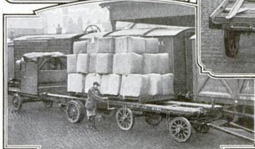
Above: The Tender Coupled to a Truck. The Misalignment can be Overcome to the Extent of 10 Inches by Means of the Chain and Lever on the Rear Part of the Tender
