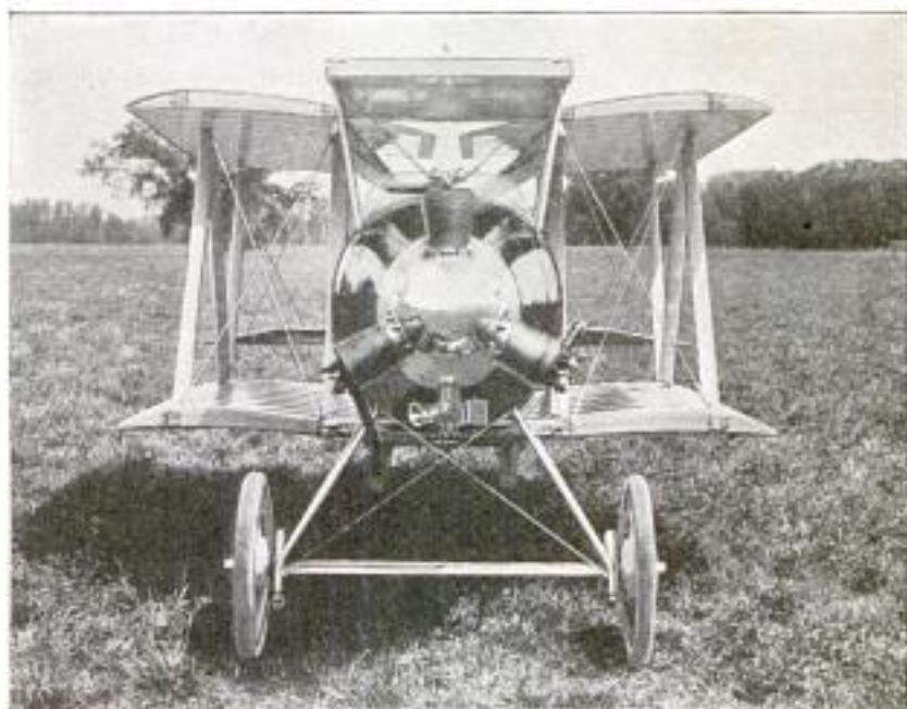
The Plane with the Wings Folded Back Is Only 8 Feet 9 Inches Wide, 7 Feet High, and 19 Feet Long. An Ordinary Automobile Garage Is Large Enough to be Used as Its Hangar. The Extended Wing Span Is 18 Feet
