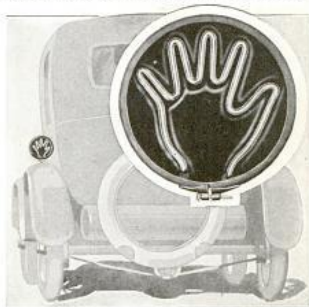
Auto Signal, Attached to Rear of Car, Made of Glass Tubing Filled with a Gas That Becomes Incandescent When an Electric Current is Sent through It, and Shines with a Red Glow
