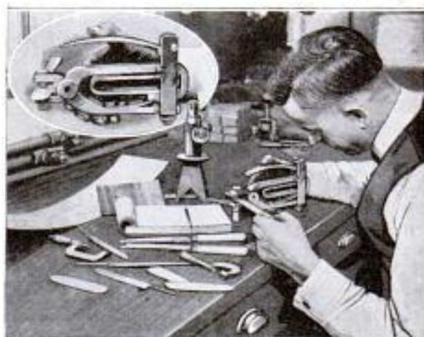
Plierlike Tool for Testing the Hardness of Materials: Any Pressure on the Lever under the Thumb Transmits a Never-Varying Pressure on the Material Tested
