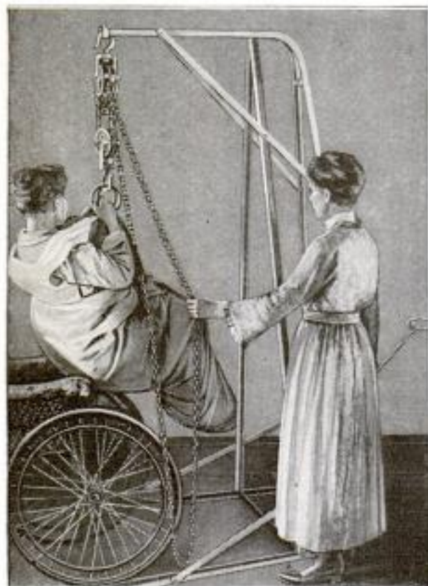
The Inventor Uses This Device to Lift Her Invalid Sister into a Wheelchair. It Is Also Convenient in Changing an Invalid's Bedding
