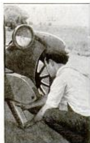
A Simple Method of Raising an Automobile Wheel for Removing a Damaged Tire, When No Jack Is Available
