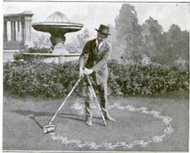
The Tool for Marking Patterns on the Ground in Use: The Circle can be Made Any Desired Size by Merely Adjusting the Arms of the Tool
