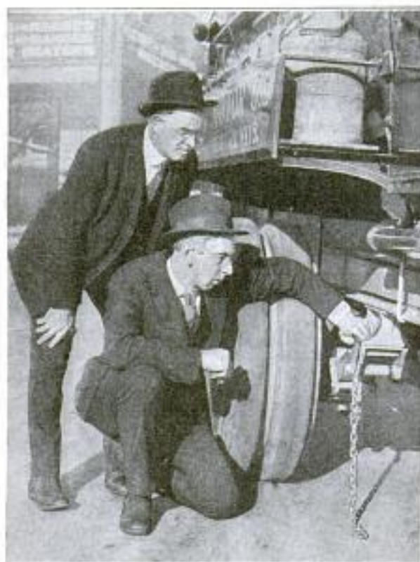
The Chain Dragging on the Ground Eliminates the Static Electricity Generated by the Gasoline When It Flows through the Pipes in the Tank
