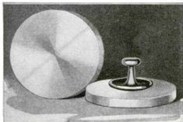
Two Small Samples of the New Metallic Alloy That Resembles Magnesium, Being Lighter Than Aluminum: Its Color and Luster can be Judged by Comparing It with the Collar Stud
