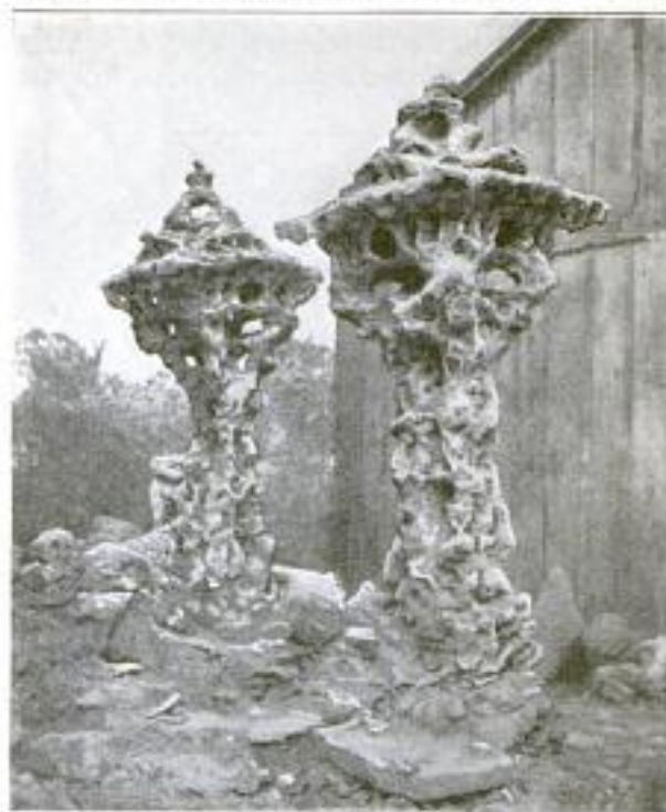
Oddly Shaped Lamp-Posts are Also Cast by Using the Mud Molds. When the Concrete has Thoroughly Set the Mud is Dug and Washed Away
