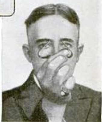
Above: New Range-Finding Gun and Rifle Sight. Lower Right: Sight in Position before the Eyes, with the Result Shown in Upper Right, Where the Sloping Sides Appear to Form an "X"
