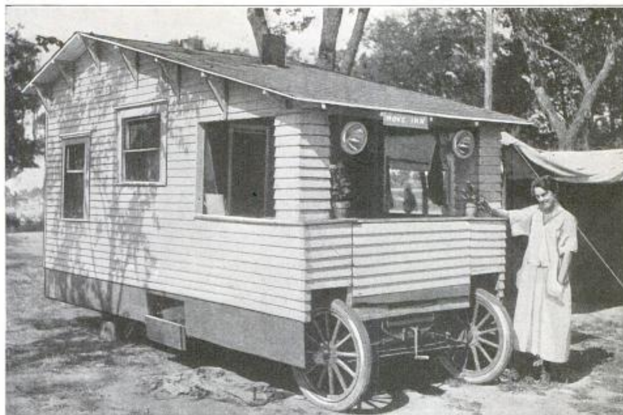
The Front Steps of This Home on Wheels Fold Up into the Porch, Creating a Closed-Porch Effect, and Making the General Resemblance to That of a Two-Room Cottage Very Striking
