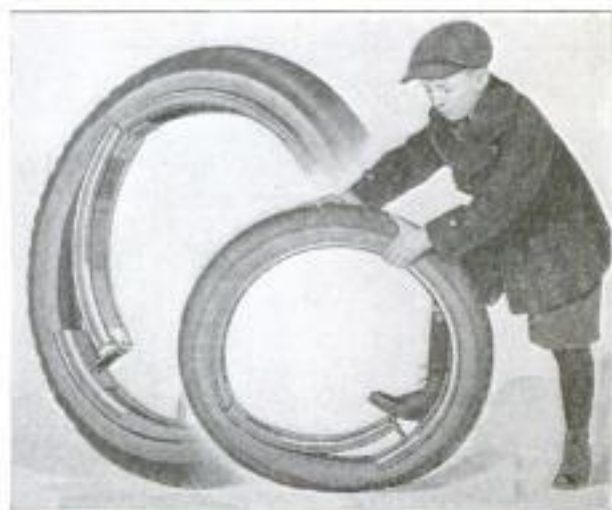
The Hinged Section of This New Tire Rim Is for Ease in Assembling. The Tire is Readily Slipped On and Off When the Rim Is in the Collapsed Condition Shown
