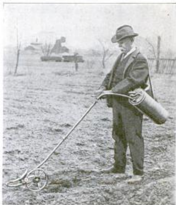
The Implement Sprays Plants from the Ground Upward. The Two Nozzles at the Wheel are Connected by the Pipe to the Tank That Contains Insecticide under Pressure. A Valve in the Pipe Controls the Spray
