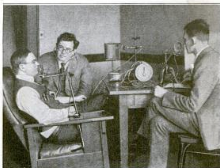
This Picture Shows the Questioner, at the Right, Speaking His Questions into the Little Mouthpiece of the Lie-Detecting Apparatus. The Subject, at the Left, Replies in the Same Manner
