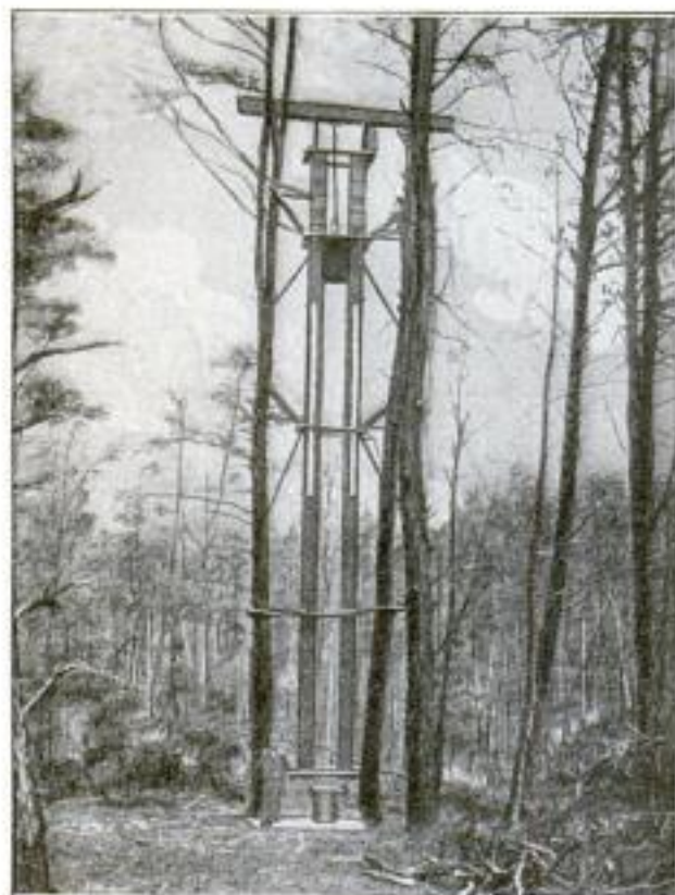
The Testing Device for Depth Bombs, Showing, near the Top of the Guides, the Weight That Falls upon the Bomb, Which is Placed on the Block Below
