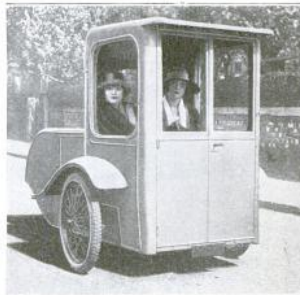
An Electric Sedan for Invalids or Shoppers That Runs on One Rear and Two Side Wheels, Accommodates Two Passengers, and is Entered from the Front
