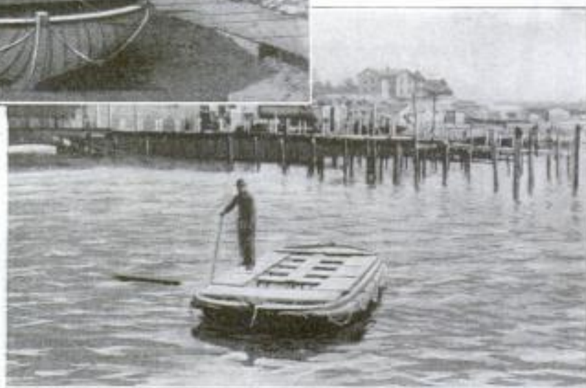
Upper View Shows the Collapsible Boat with the Sides Up. The Seats for the Oarsmen Are Visible. The View to the Right Shows the Boat in the Collapsed Form, Launched to Show How High It Rides in the Water
