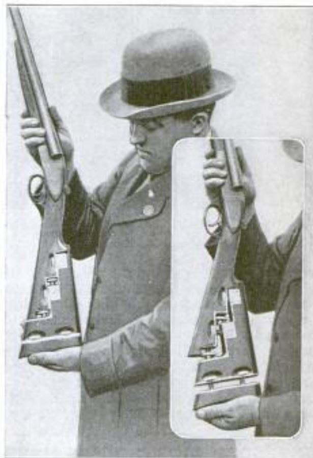
Left: The Gunstock Closed, Showing the Setscrews by Means of Which It can be Extended, as Shown to the Right. Springs, Not Visible, Absorb the Recoil
