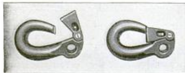
New Logging Hook, in Open and Closed Positions, Used on Steel Cables in Western Logging Operations: A Spring Keeps the Catch in Place
