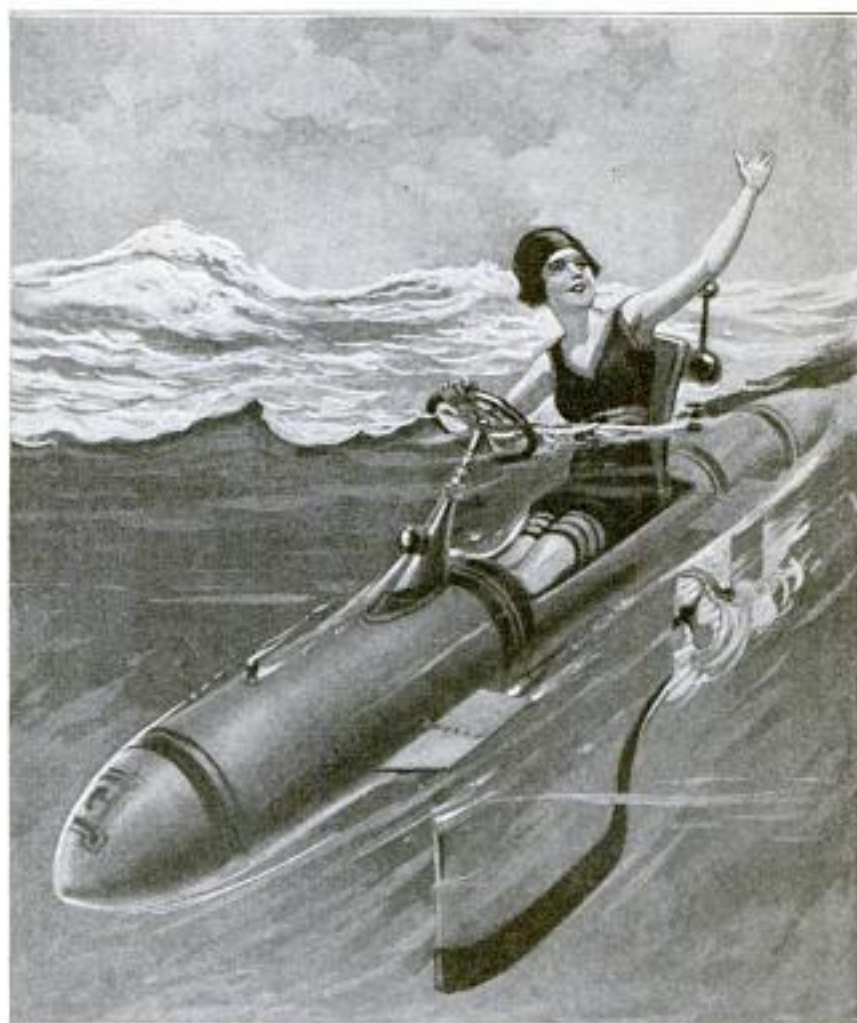
The Submerging Boat That Travels on the Surface, or below the Surface, as Shown, with the Rider's Head and Shoulders above the Water: The Propeller is Electrically Driven by a Motor and Storage Batteries Installed inside the Hollow Keel
