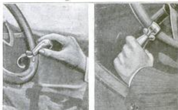
Left: Showing How Handle, for Added Leverage in Steering, is Slipped over Narrow Part of Rim. Right: A Spring inside the Handle Holds the Side Lugs in Tension against the Hook
