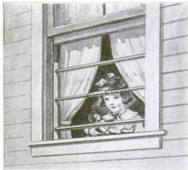
A Bar Arrangement Fastened into Any Window, by Means of the Turnbuckle of the Middle Bar, Prevents Accidents
