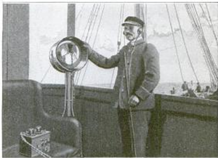
The Operator is Guiding the Parabolic Gilded Mirror with His Right Hand, and with the Telephone Receivers on His Ears He Detects the Approach of an Iceberg
