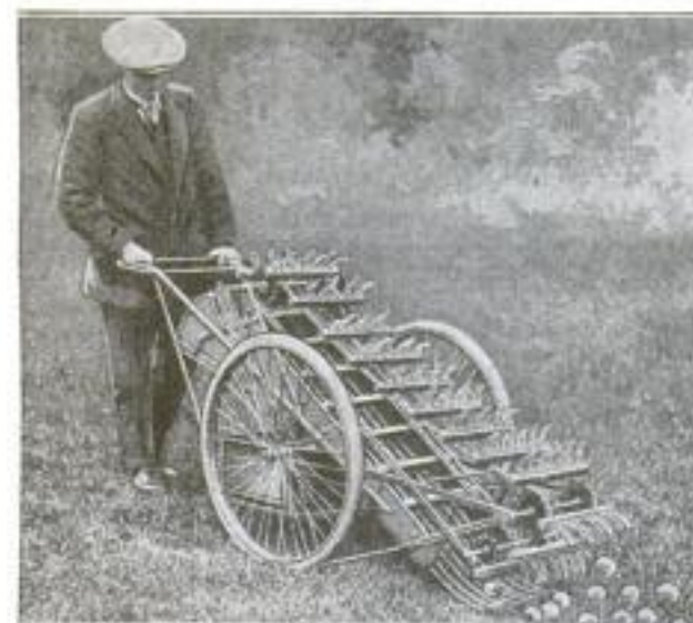
The Rakelike Arms Pick Up Apples from the Ground and Deposit Them in the Basket at the Rear
