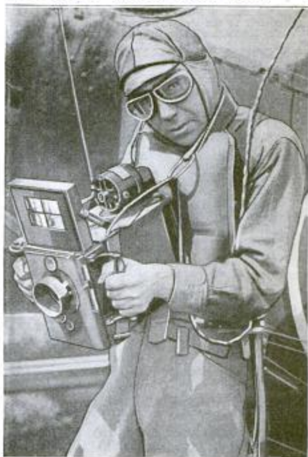
The Airman is Grasping the Movie Camera by the Side Handles. A Small Electric Motor Drives the Camera
