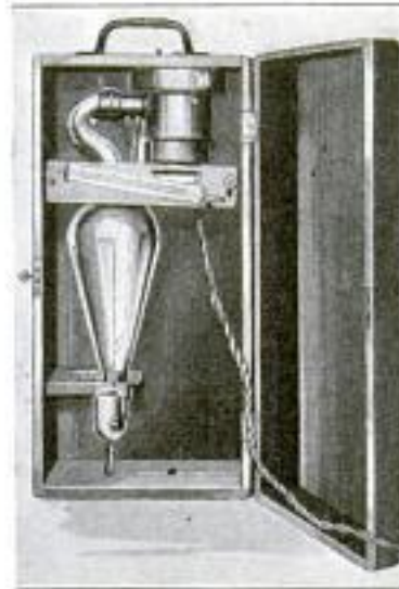
Apparatus Which is Used to Determine the Amount of Solids and Soluble Matter Floating in the Air in the Third Street Tunnel at Los Angeles
