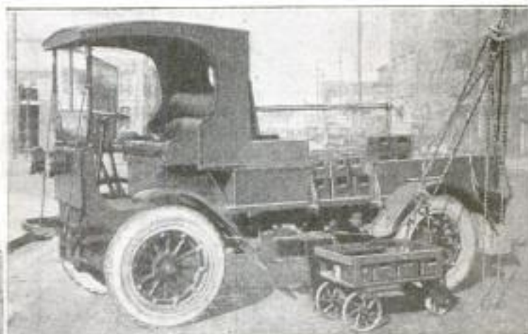
Wagon-Scale Testing Outfit. Large Truck for Testing Ends of Platform, "Dolly" for Testing All Four Corners. Left: Lowering Dolly from Truck
