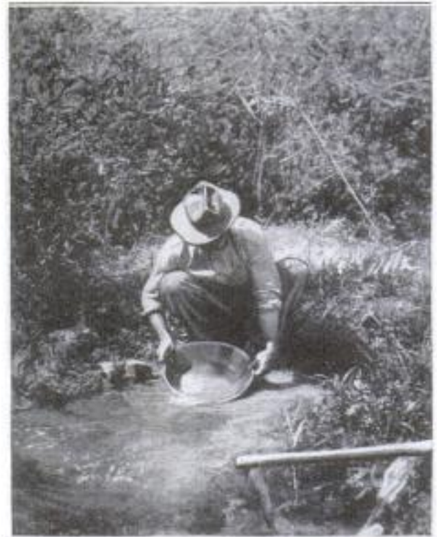
A "Pan," the Same as in Placer Mining, is Used for Washing the Dirt Out of the Mercury and Gold Before Placing It in a Buckskin Bag
