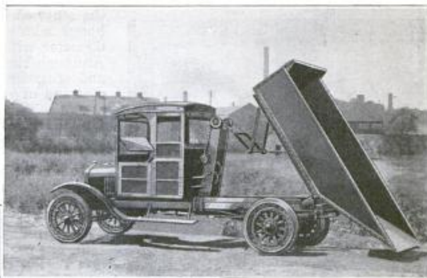
Left: The Truck Is in Position for Loading. The Receptacle for the Garbage Is Low Enough to Allow a Man Standing Beside It to Easily Reach Over It. Above: The Garbage Receptacle has been Raised by the Winch to the Dumping Position with Its End Sloping to the Ground
