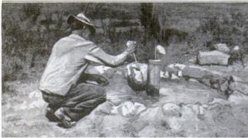
The Miner is Pouring Mercury into the Concrete Basin That is Constructed for Extracting the Gold from the Ore. This Is the Last Operation Necessary before Evaporating the Water
