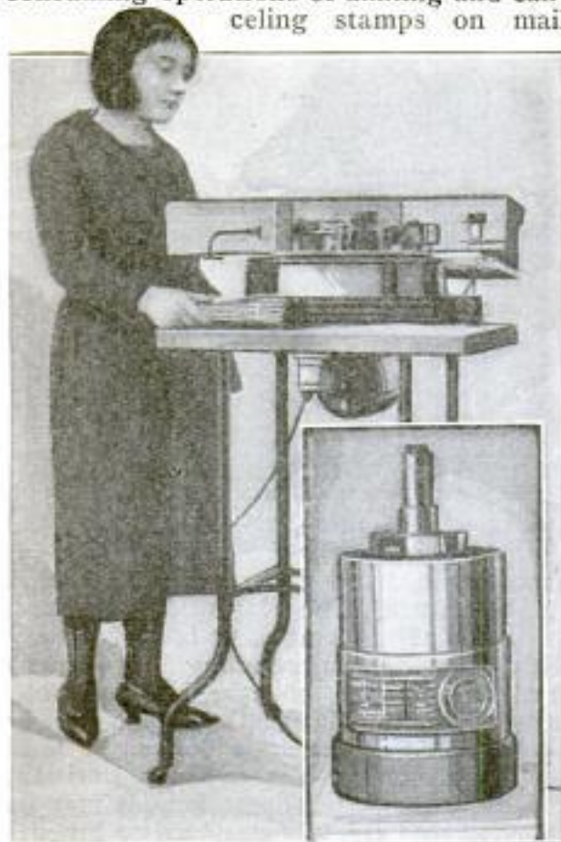
Demonstrating a New Electrically Operated Canceling Machine: A Canceling Mark is Printed on the Envelope by Means of the Cylindrical Die Shown in the Insert
