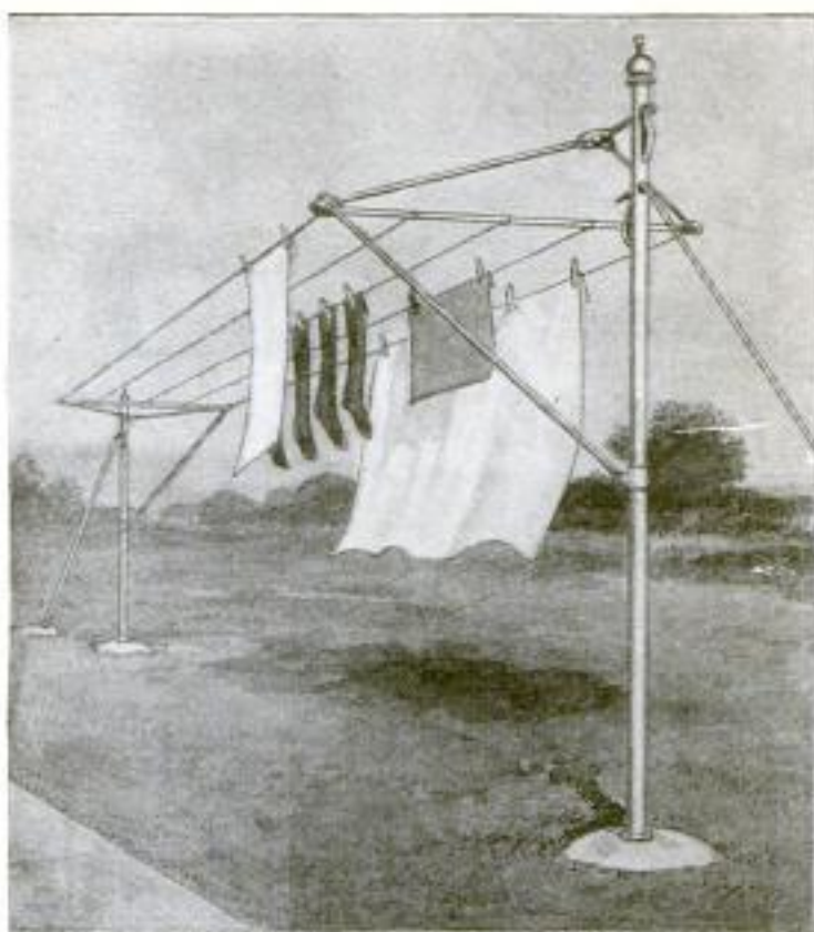
The Multiple Clothesline Support Has a Triangular Upper Frame, One Side of Which Serves as an Anchor for Many Lines. The Lines are Drawn Tight by Turning a Handle on the Upright Support
