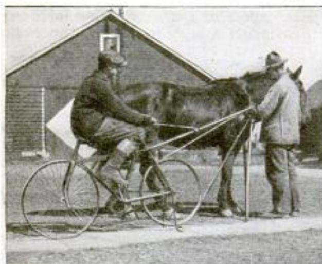
By Connecting a Set of Power Clippers to an Old Bicycle a Farmer and Stock Raiser Is Able to Clip Many Animals Each Spring with a Minimum of Labor
