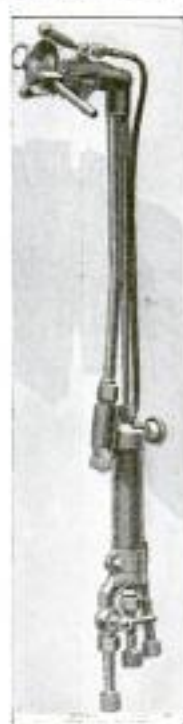
An Oxyacetylene Blowpipe That can be Ignited by a Diver under Water
