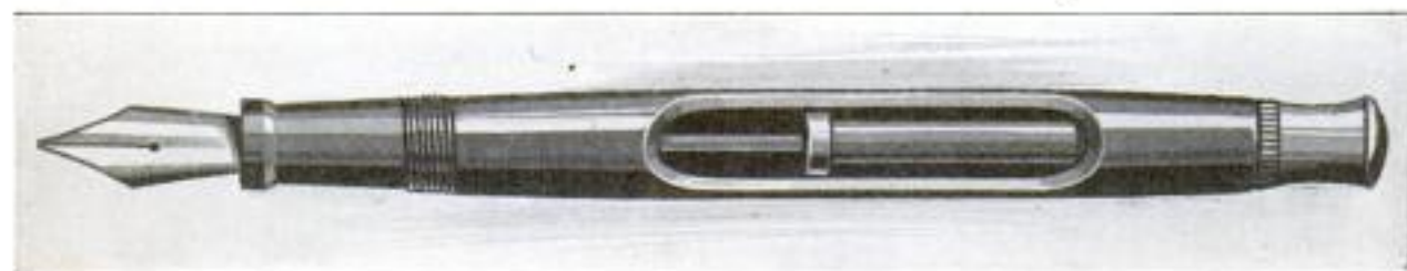
This Fountain Pen Works Like a Pump in Filling. The User Grasps the Knurled Cap at the End and Pumps It Back and Forth, Drawing the Ink Up into the Pen Barrel
