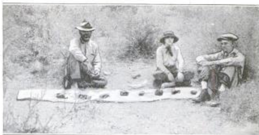
On the Cloth Are Pieces of the Ore Showing the Size to Which It is Broken in Preparation for Putting It through the Crushing Process That Takes Place in the Concrete Basin
