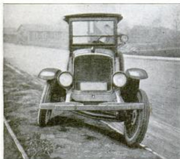
The Pivoted Front-Axle Spring Suspension of This Light Speed Truck Allows the Front Axle to Rock Transversely through a Limited Arc, Preventing Frame Distortion
