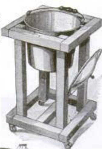
Refuse Receiver Provided with Casters for Rolling It along the Floor
