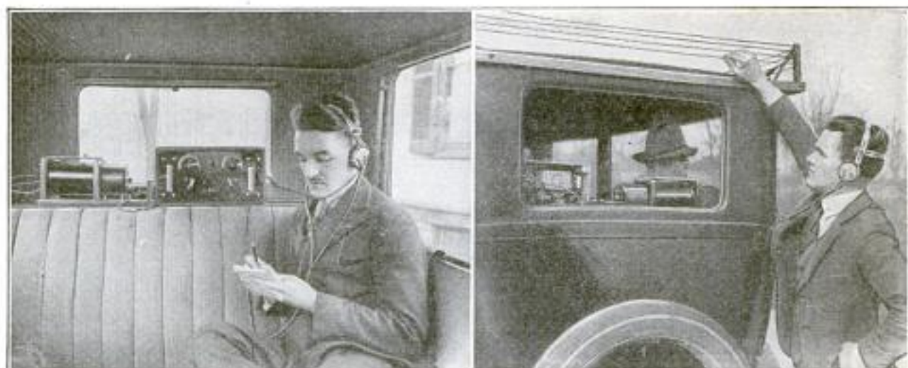
These Two Views Demonstrate a New Wireless Receiving Set Designed More Especially for Physicians. The Picture on the Left Shows the Convenient Disposal of the Small and Compact Instruments inside the Rear of the Tonneau. The Placement of the Antennæ around the Top Edge of the Car Body is Shown on the Right
