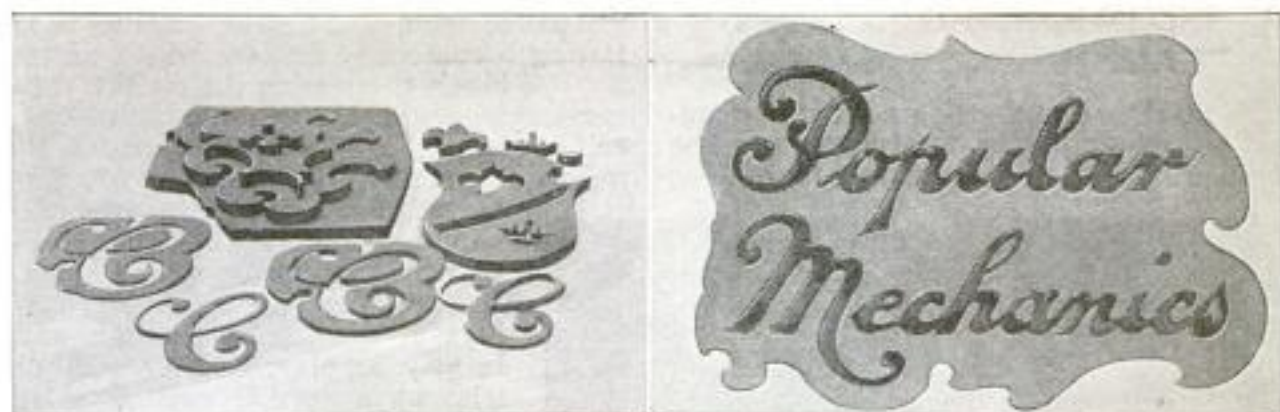
Patterns Cut in Rubber: In One of the Pieces Above, the Pattern is Raised above the Surface. The Four Pieces Below are All Cut at the Same Time
