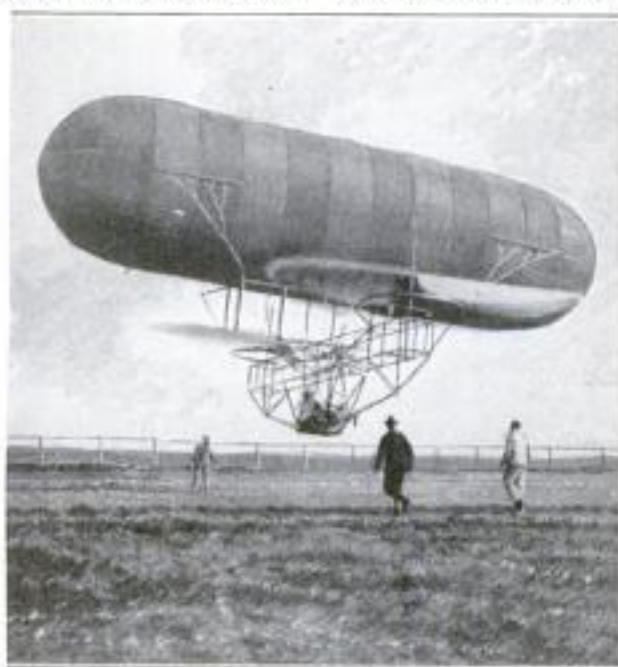
The Inventor did Not Risk an Altitude of More than Six Feet in the Preliminary Trials. Since the Propellers were Built for Lifting Only, and Not for Driving Horizontally, the Machine would Drift with the Wind
