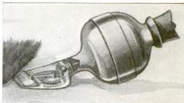
This Motor-Driven Skinning Knife Separates the Hide from the Animal by Driving a Reciprocating Blade between the Hide and the Flesh
