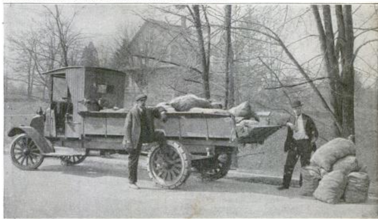
Road Crews Patrol the State of Maryland, Equipped with Portable Loadmeters or Jacks. Trucks That are Overloaded are Forced to Reduce Their Freight to the Legal Requirements on the Spot
