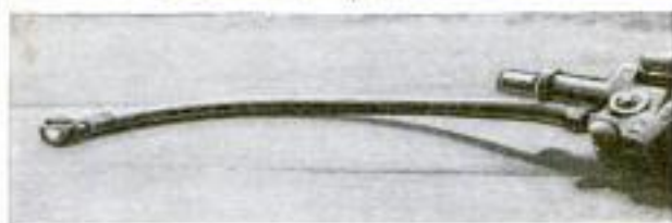
The Upper of the Two Views Shows the Motorist Testing the Tire Pressure with the New Gauge. Below Is a Close-Up of the Pistol-Shaped Valve Casting with the Extension Hose and Cap
