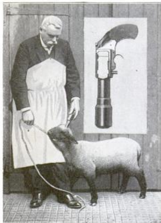
Killing a Sheep by Placing the Nozzle of the Slaughtering Gun Against Its Head and Then Pulling the Trigger. Inset: A Detailed View of the Pistol
