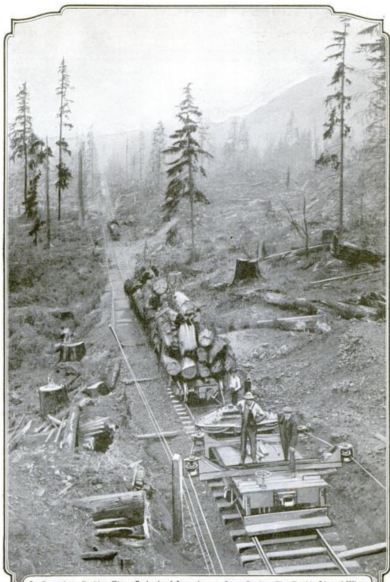
In Operation—Braking Three Carloads of Logs down a Steep Grade: The Double Line of Wires to the Left of the Road is the Electric-Signal System. When the Bottom of the Mountain, a Mile Distant, is Reached, the Loaded Cars are Unhooked and Empty Cars Picked Up and Taken Back to the Place Where the Logs are Yarded. The Two Men in Shirtsleeves on the Snubber Truck Are All That are Required to Operate the Train
