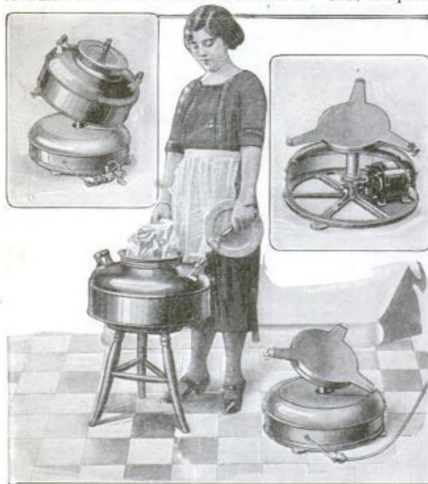
In the Upper Left-Hand Picture is Shown the New Portable Washing Machine Assembled. The Upper Right Insert Shows the Rotating Stand Driven by an Electric Motor. The Lower View Shows the Machine Disassembled
