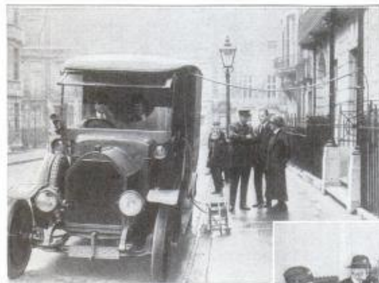
The Ambulance is Standing in Front of the Patient's Residence with the Wire Arranged to Transmit the Power from the Ambulance to the X-Ray Apparatus in the Sick Room
