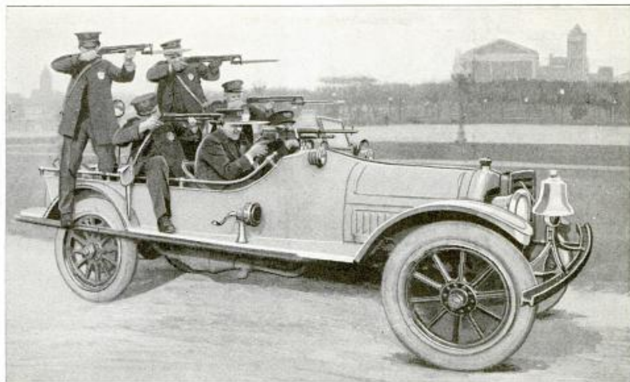
This Bandit-Chasing Automobile Has a Heavy Protective Screen for the Radiator, and the Bumper Consists of a Special Rolled-Steel Rail Section. The Windshield Is Bullet-Proof. Riot Guns, Searchlights, and a Swivel Machine Gun Are Part of the Bandit Chaser's Equipment
