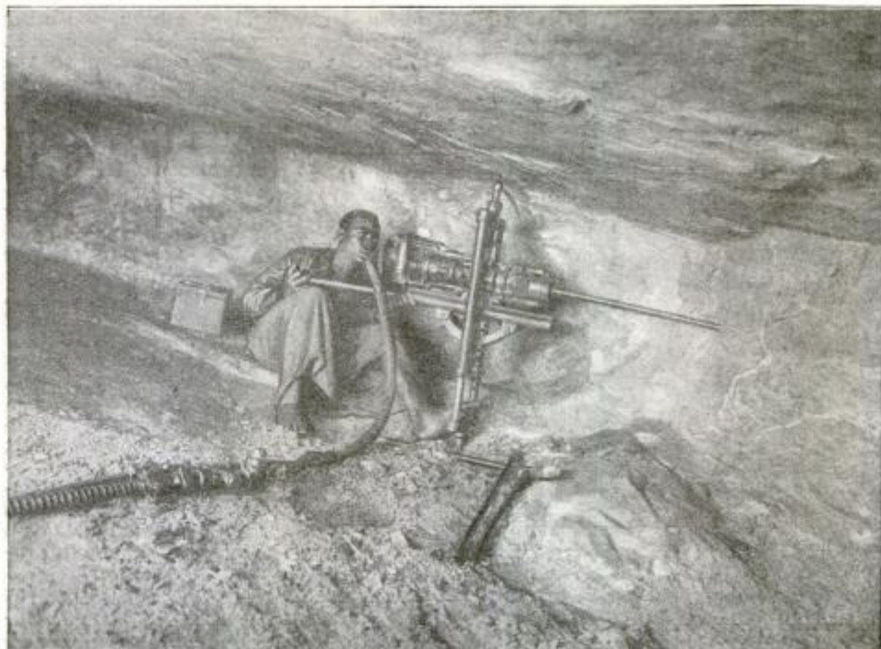
The Rock Drill is Shown Supported between the Roof and the Floor of a Drift with Its Automatic Feed Device in Operation. Under the Drill is Seen the Guide as Well as One of the Holding-Up Springs Connected to It. It will be Seen That Vertical as Well as Horizontal Adjustment is Provided For
