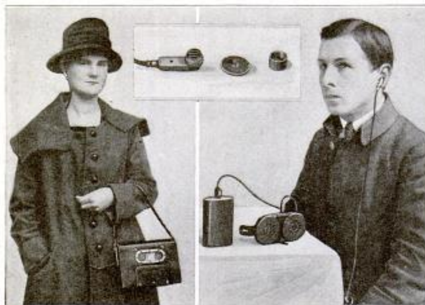
The Transmitter and Battery of the Little Telephone can be Fitted into a Handbag or Placed on a Table. Insert: The Receiver; Note the Size as Compared with the Coin in the Center
