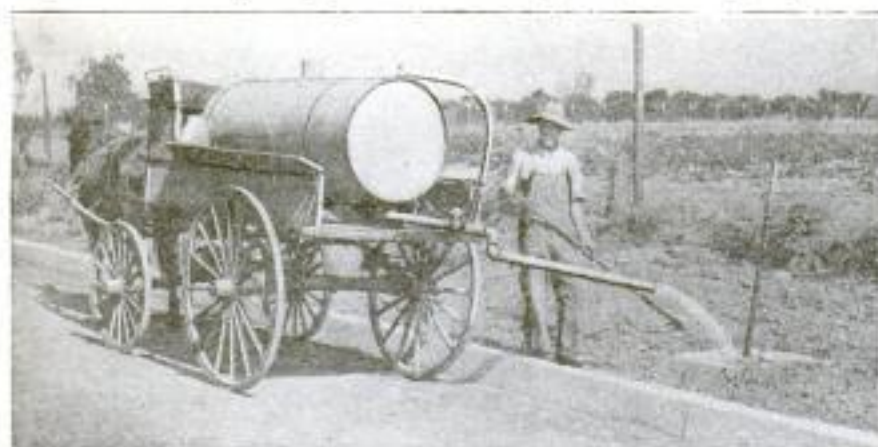
Tank Cart, with Swinging Spout, Used to Water an Eight-Mile Row of Evergreen Oaks along a California Road
