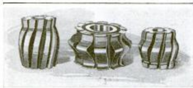
The Formed Milling Cutters Make a Shaped Groove in the Metal Stock. The Teeth are Helically Cut
