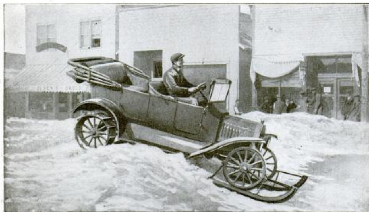
The Light Car Climbs the Deep Drifts Easily, for the Front Wheels have been Replaced by Runners. Two Extra Rims have been Fitted to Each Rear Wheel Which Gives Increased Traction. The Rims are Held Together by Crossbars Made of Angle Strips
