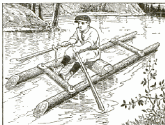
A Useful Boat, Built of Logs as a Catamaran Raft, Takes the Place of a Regulation Rowboat When the Latter is Not Easily Obtained
