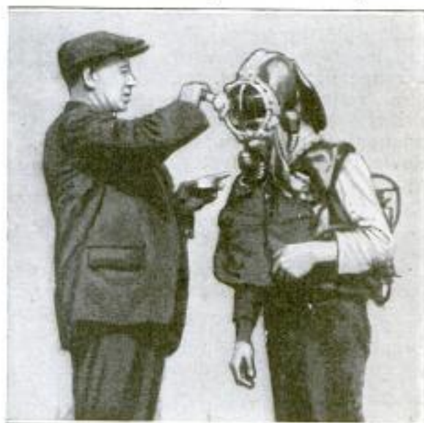
Daubing One of the Gas Masks Used by the San Francisco Firemen with Soap Lather, to Indicate Leaks. A Bubble will Appear Where a Leak Is Present
