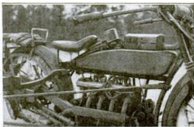
The Views on the Left Show the Motorcycle Passing through the Soggy Wagon Ruts, by the Aid of the Outrigger Wheel. Right: How the Outrigger is Attached to the Cycle Frame; the Fitting was Made of a Buggy Wheel and Axle, and Blacksmith-Shop Scraps.
