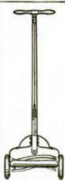
A Swivel Arrangement in the Handle Fitting of the Terrace Lawn Mower Allows the Operator to Walk on the Ground and Mow the Incline
