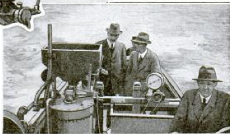
The First Trials were Made in This 35-Foot Launch, Equipped with the Gas Producer to Furnish Fuel to Its 75-Horsepower Motor
