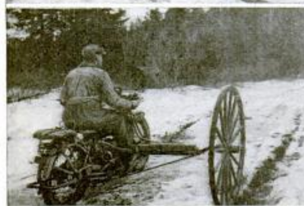
The Views on the Left Show the Motorcycle Passing through the Soggy Wagon Ruts, by the Aid of the Outrigger Wheel. Right: How the Outrigger is Attached to the Cycle Frame; the Fitting was Made of a Buggy Wheel and Axle, and Blacksmith-Shop Scraps.
