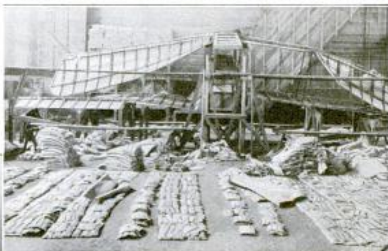
In the Destruction Tests Hundreds of the Sandbags, Shown in the Foreground, are Used. Each is Marked with Its Weight. The Airplane in the Background Is Upside Down
