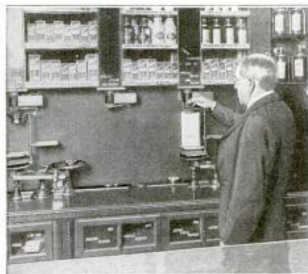
Weighing Groceries Electrically: The Scales, Upright Fitting, and Bin Outlets Are Part of a Circuit. When the Scales Balance the Outlets Close
