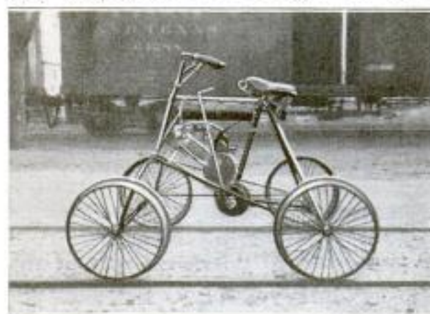
This Railway Motorcycle Has a 2½-Horsepower Engine, and Scurries Along at a Rate of 30 Miles an Hour. The Wire Wheels Make It Very Light and Easily Controlled
