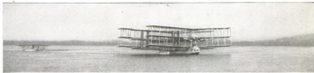
This Illustration Conveys a Good Idea of the Gigantic Size of the Craft in Comparison with a Seaplane of the Conventional Type. Within a Few Moments After This Photograph was Taken the 15-Ton Machine had Demonstrated Its Ability to Overcome Gravity by Making a 400-Yard "Hop"
