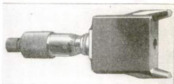
The Adjustable Plug Gauge is Built like a Micrometer and Takes the Place of Many of the Standard Gauges
