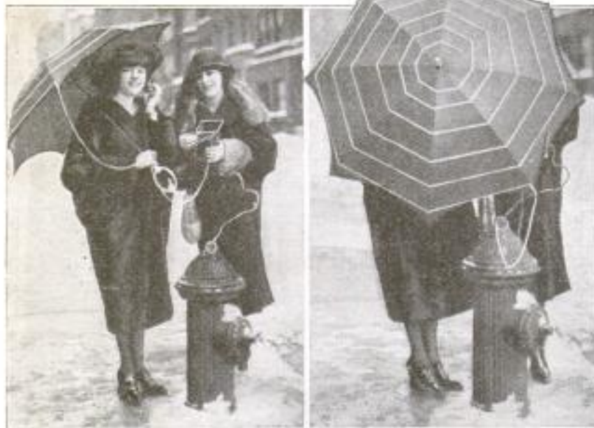
At the Left: The Parasol-Vanity Case Wireless-Receiving Set in Use, Grounded to a Convenient Water Plug by a Flexible Cord. At the Right: The Parasol "Aerial," with Its 110 Feet of Antenna Wire Decoratively Arranged
