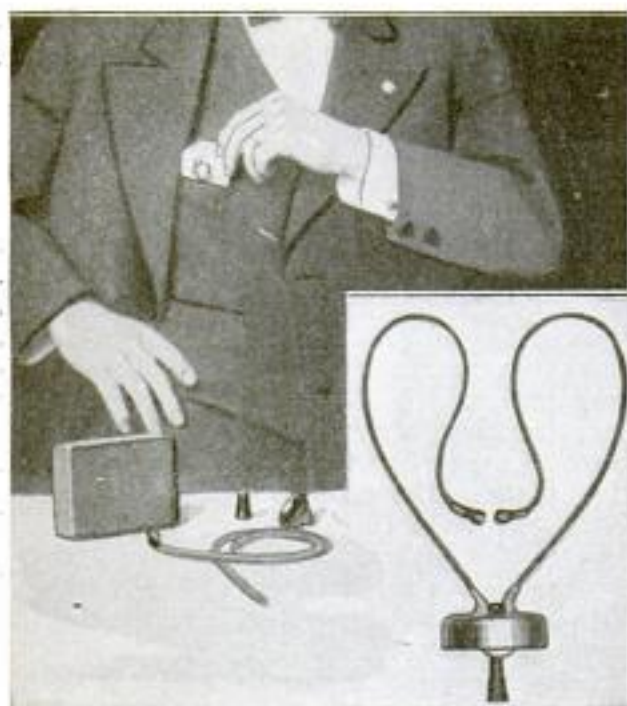
Left: The Parts of the New Light Stethoscope, Showing Its Easy Portability, the Transmitter Section being Carried in the Vest Pocket. Right: The Instrument Assembled for Use
