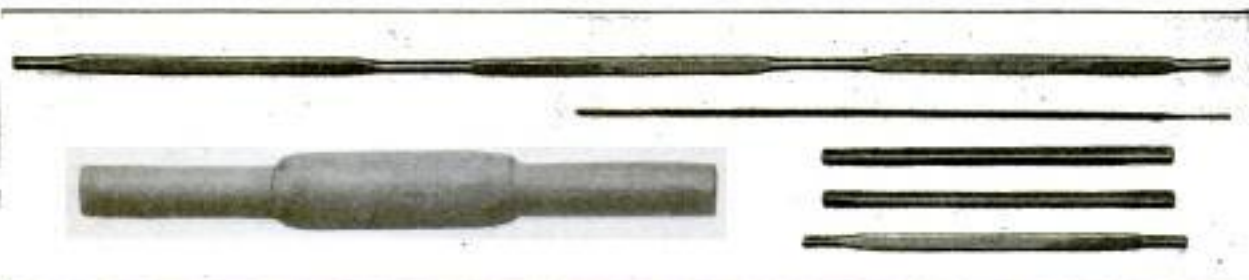
The Rolls for Making These Irregular-Shaped Rods are Built Up Segmentally. Such Construction Effects Economy, For It Is Not Necessary to Discard an Entire Roll with Good Passes Left in It, When the Segments Forming the Defective Pass may be Removed
