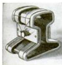
Left: Inner Test Coils for Rails. Right: For Wires and Cables
