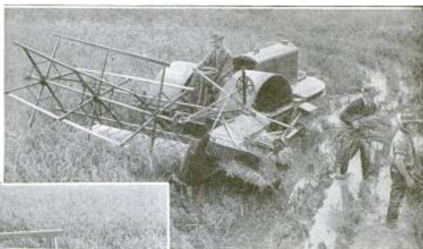
The New Rice-Harvesting Tractor Working in a Field Covered with Deep Mud and Water. Buoyed Up by the Huge, Air-Tight Drums That Compose Its Drivewheels: It Crossed Ditches and Levees with Ease
