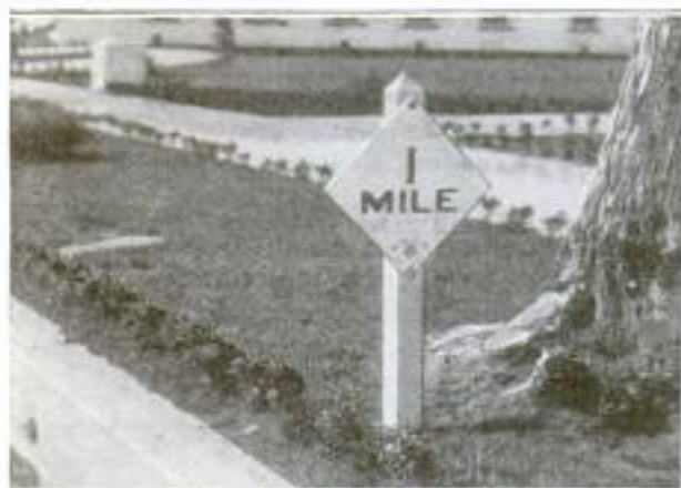
A Milepost on the Speedometer-Testing Speedway: Speed Calculations Based on the Time Required to Cover a Mile, and the Speedometer Indication should Agree
