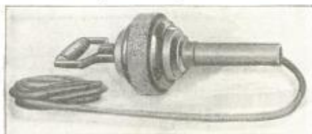
The Emery Wheel, for Dressing Castings, is Mounted on the External Rotor of the Small Motor. The Dresser is Used for Working in Tight Places
