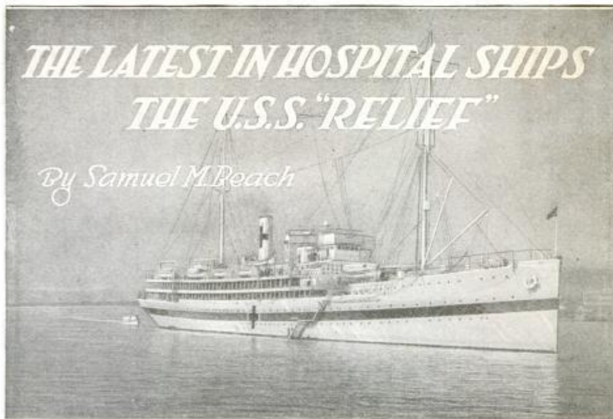
The New United States Hospital Ship "Relief," the First American Naval Craft to be Designed, from the Keel Up, Exclusively for Military-Hospital Use: It Is 483 Feet Long, with a Displacement of 10,000 Tons
