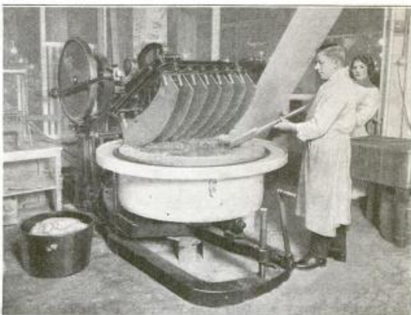
Sausage Meat Prepared with This Machine is Chopped. The Knife Moves Like a Hand Chopper, and the Table Turns Slightly at Each Stroke
