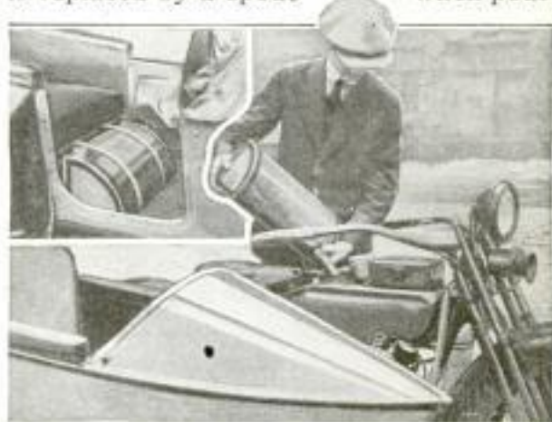
The Sidecar Tank Carries an Additional Supply of Gasoline for Long Trips. Below: Emptying Tank into Cycle Reservoir
