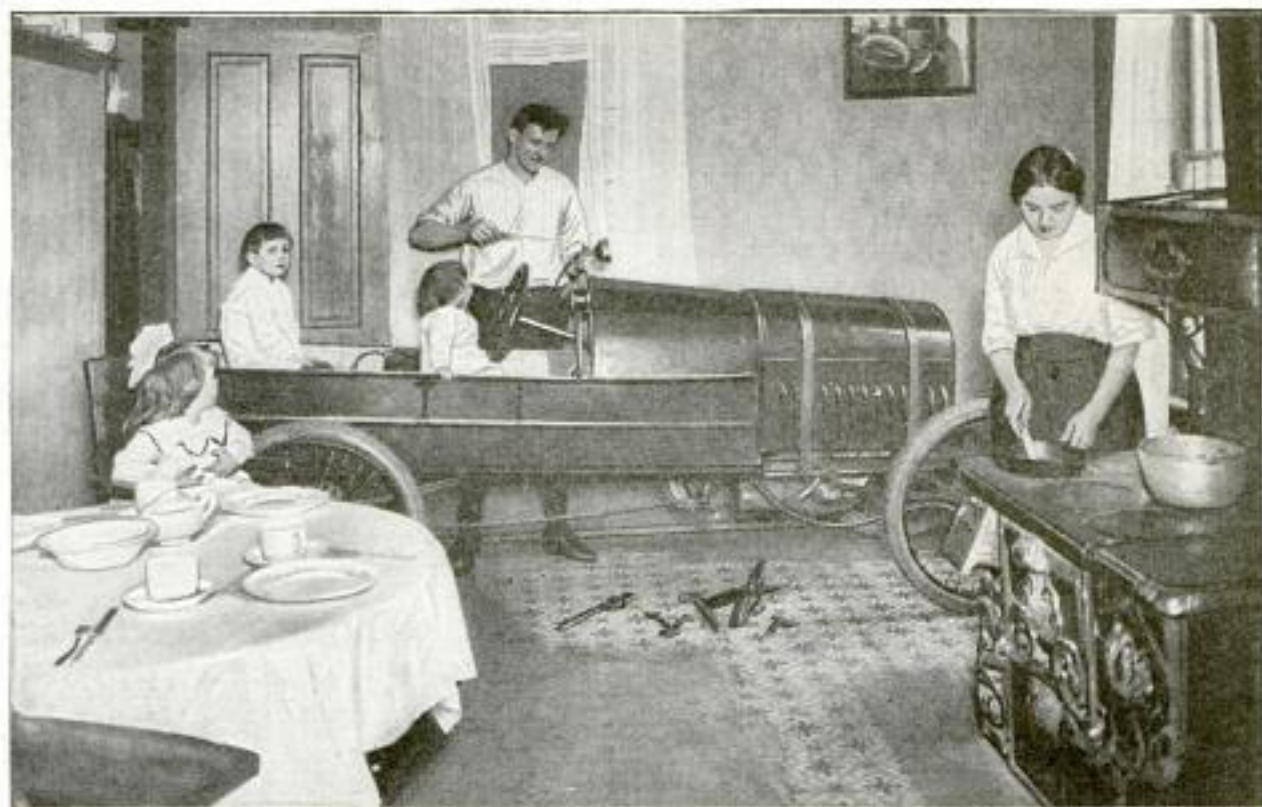
An Amateur Job of Automobile Building, in the Kitchen of an Upper Flat: The Car Has a Motorcycle Engine and Wheels, and, the Body Being Only 20 Inches Wide, It was Readily Lowered through the Window When Finished
