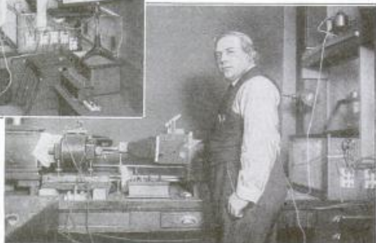
The Laboratory Equipment for Demonstrating, with Photographic Charts, That the Action of Light on the Eye Generates Electric Current
