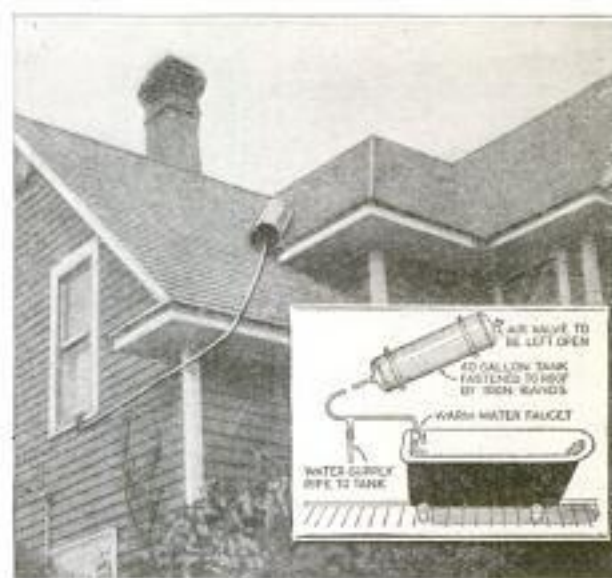
Water Tank on Roof Absorbs Heat from the Sun and Provides Warm Water for Bathing at No Expense for Fuel
