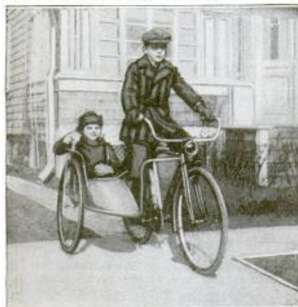
A Comfortable, Easy-Running Sidecar, Easily Attached to an Ordinary Bicycle for Carrying Children
