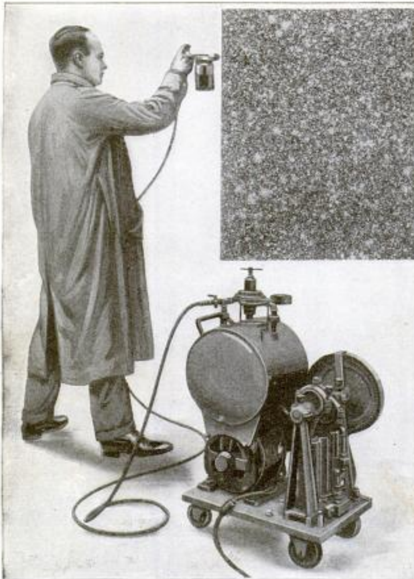
The Operator Decorates the Wall with the Spraying Instrument, While the Machine, in Any Convenient Location on the Floor, is Run by Means of the Electric Motor to Which is Attached a Cable and Plug for Connection to Any Standard Electric-Light Socket
