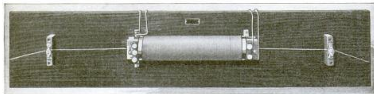
The Stationary Testing Coil Used for Steel Wires; It Is Similar to the Equipment Used for Bars, Except That the Wire may be Drawn through the Coil in Its Process of Manufacture, if Desired
