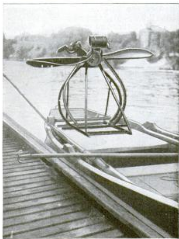
The 1\frac{1}{2} -Horsepower French Rowboat Motor and Air Screw That Pulled Five Boats, with 24 Passengers
