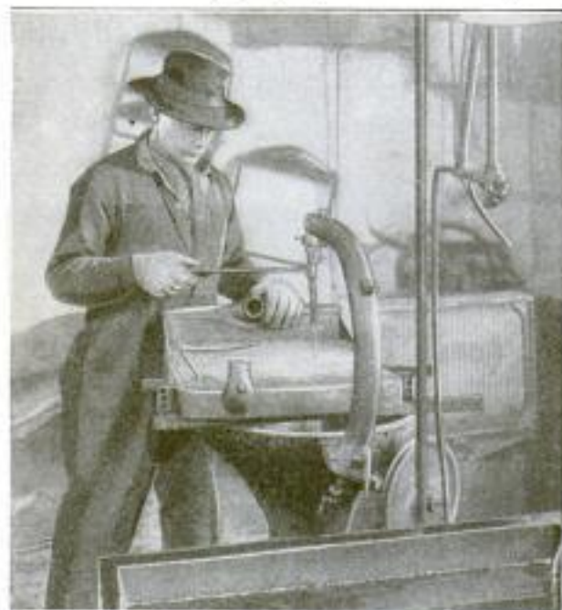
Repairing a Leaky Auto Radiator with a Jet of Melted Solder: The Hot Stream Quickly Stops All Leaks and Carries the Surplus Solder Back into the Melting Pot Below
