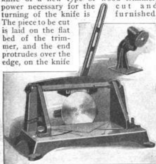
By Pushing the Hand Lever to the Opposite Side, the Cutting Knife is Rotated and Moved. Upper Right: Sharpener
