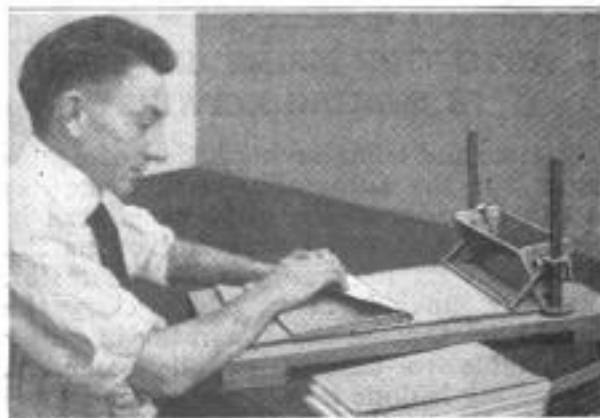
Paste-Applicator for Magazine Wrappers: Each Wrapper in the Stack beneath the Hopper Has a Film of Paste across One End When Drawn Out
