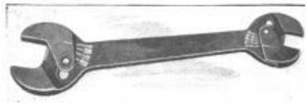
Double-Ended Wrench Adjustable for Ten Sizes, between \frac{1}{4} and \frac{7}{8} Inch, by Sliding the Jaws
