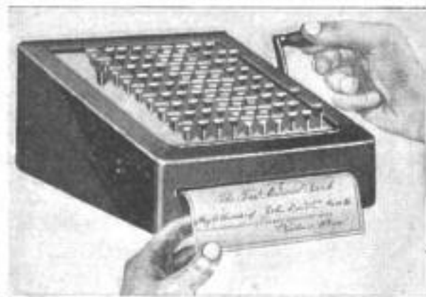
The Check Writer Discharging a Filled-In Check: The Figures are Set with a Motion of the Keys, and Printed with a Pull of the Lever
