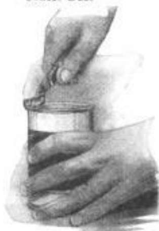
The Ragged Edge of the Can is Turned Up and Smoothed by a New Can Opener That Cuts like Scissors
