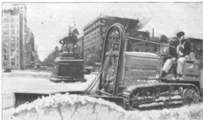
One of a Fleet of Endless-Tread Five-Ton Tractors Used to Remove Snow from the Streets of New York City
