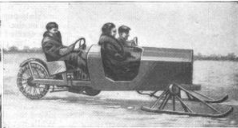
A Three-Passenger Auto Sled Which Attains Speeds of 45 to 50 Miles an Hour: The Runners Are of Standard Tread and are Mounted on Regulation Steering Knuckles. Sections of Chain around the Rear Wheel Insure Traction. Left: The Power Plant, Fuel and Oil Tanks, Gear-Shift Lever, and Steering Wheel. Note That the Throttle and Spark-Control Levers are Placed Directly under the Wheel
