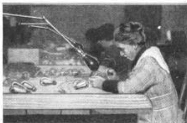
Lacing New Tungsten Wire into the Old Lamps: Using a Special Tool, the Wire is Clamped to One of the Terminals, Laced around the Hooks, and Made Fast
