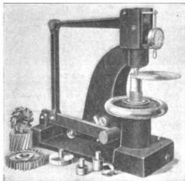
New Direct-Reading Hardness-Testing Machine, with Several Interchangeable Anvils for Work of Different Shapes, and a Number of Samples for Testing
