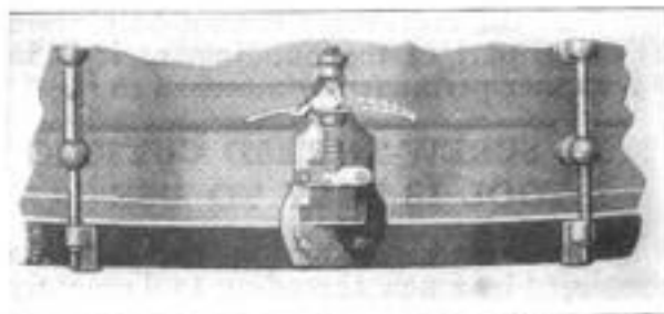
Muffer Attachment on the Lower Hoop of the Drum: Dotted Lines Show Different Lever Positions
