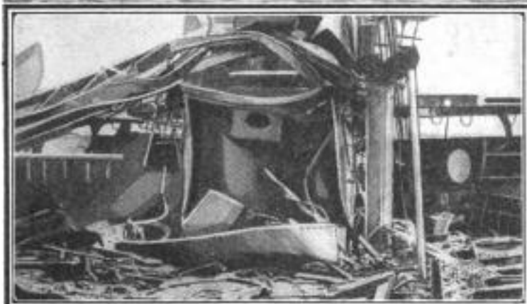
Looking Aft along the Main Deck of the "Indiana" Just after a Bomb Test: The Extensive Damage Indicated was Caused by a Single Bomb. Such a Hit with a Bomb Dropped from a Plane would Be Practically a Matter of Pure Luck, as a Ship's Anti-Aircraft Guns would Prevent the Approach of a Bombing Plane to a Position Close Enough for Accuracy
