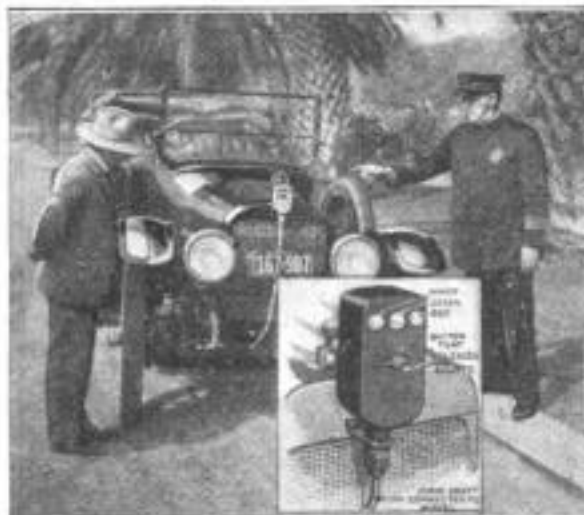
The Speeder "Telltale" Installed on a Car. Insert: A Close View of the Instrument, Showing the Three Lights and the Control Switch
