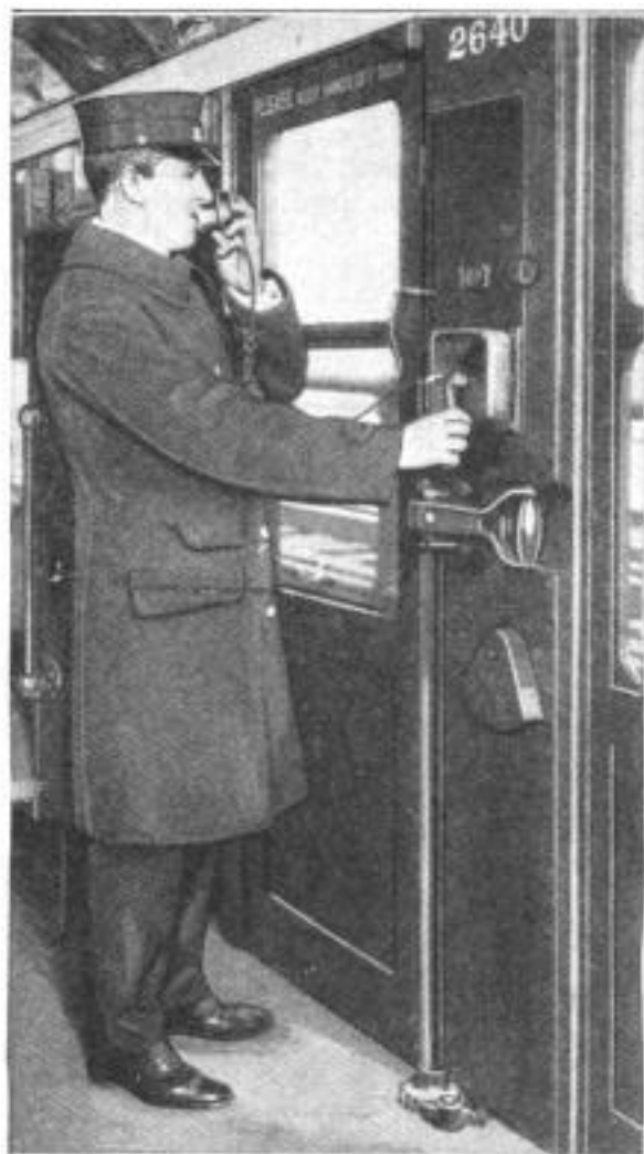
At the Left: A Guard Using the New Door-Control and Announcing Equipment on a Six-Car Elevated Train. All the Doors of the Six Cars are Opened and Closed Electrically by Operating the Hand Lever on the Wall, and the Telephone Transmitter is Connected to Loud-Speaking Receivers in the Cars, Which Repeat the Lone Guard's Announcement of Station Names, and His Admonitions to "Watch Your Step." Above: The Flexible Cord on Which the Telephone is Hung Permits the Guard to Step Out onto the Station Platform, Before He Signals the Motor Man to Go Ahead
