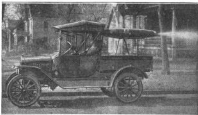
The Big Sheet-Metal Cigar in the Back of the Auto is Connected to the Engine-Exhaust Pipe, and the Driver Makes It Smoke at Will
