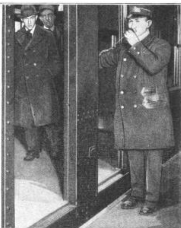
At the Left: A Guard Using the New Door-Control and Announcing Equipment on a Six-Car Elevated Train. All the Doors of the Six Cars are Opened and Closed Electrically by Operating the Hand Lever on the Wall, and the Telephone Transmitter is Connected to Loud-Speaking Receivers in the Cars, Which Repeat the Lone Guard's Announcement of Station Names, and His Admonitions to "Watch Your Step." Above: The Flexible Cord on Which the Telephone is Hung Permits the Guard to Step Out onto the Station Platform, Before He Signals the Motor Man to Go Ahead
