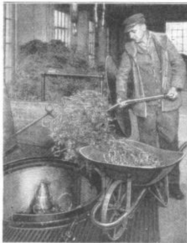
Loading a Centrifugal Extractor Basket with Oil-Soaked Metal Turnings: The Oil is Torn from the Mass by Centrifugal Force and Thrown through the Basket Perforations
