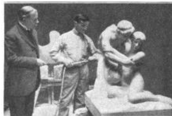
An Assistant of Lorado Taft's, Using a Pneumatic Chisel with Interchangeable Points for Chipping Out a Large Marble Statue
