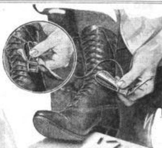
New Ties are Put on Shoe Laces by a Folding Combination Tool That Acts Also as a Buttonhook and a Shoehorn
