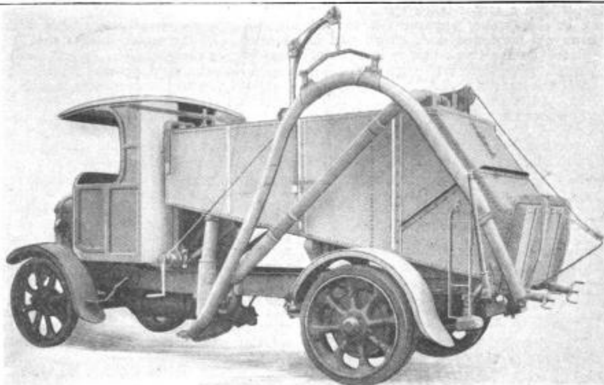
Auto Vacuum Cleaner for City Gutters: The Odd-Shaped Body Has a Capacity of 1,200 Gallons. Hand Winches are Used to Manipulate the Flexible-Steel Suction Tube and Open the Heavy Discharge Door
