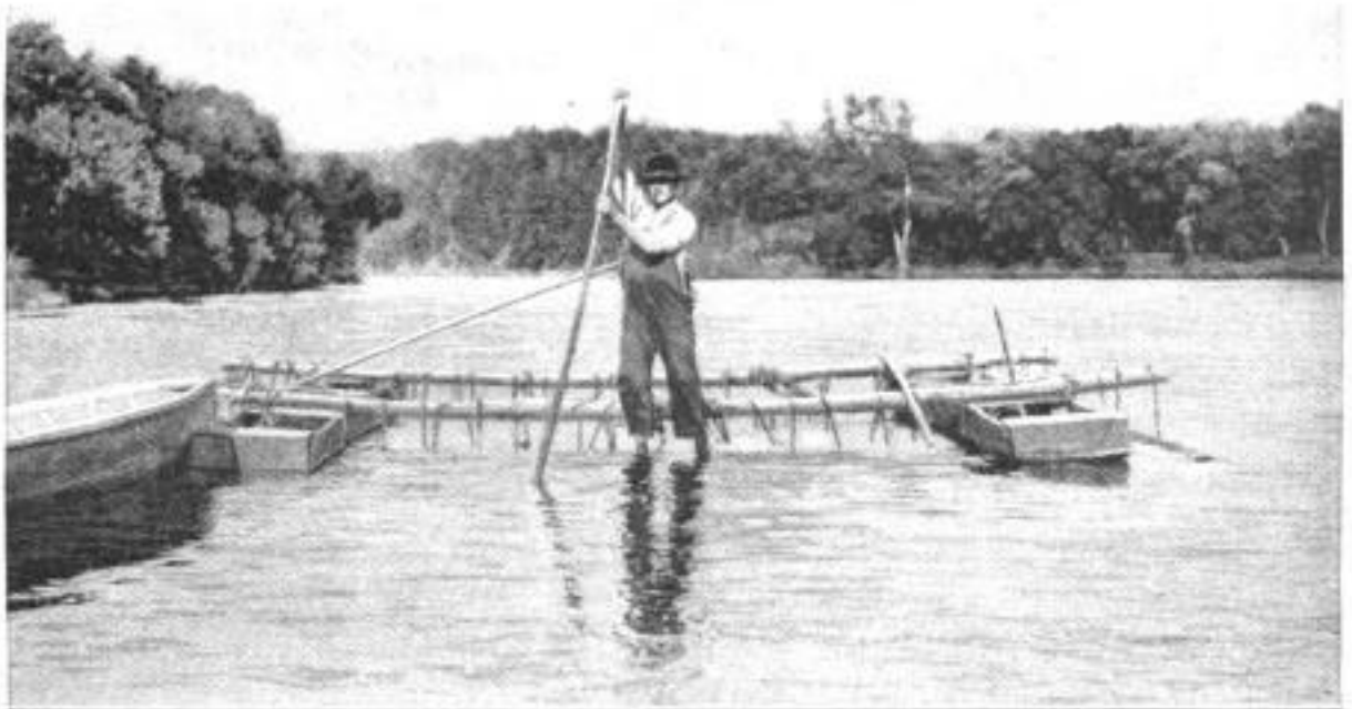
The Deadhead Hunter at Work: The Long Cross Poles That Connect the Two Square-End Boats Carry Chain Slings for the Recovered Logs, and the "Pick Pole" in the Hunter's Hand is Shod with a Steel Screw
