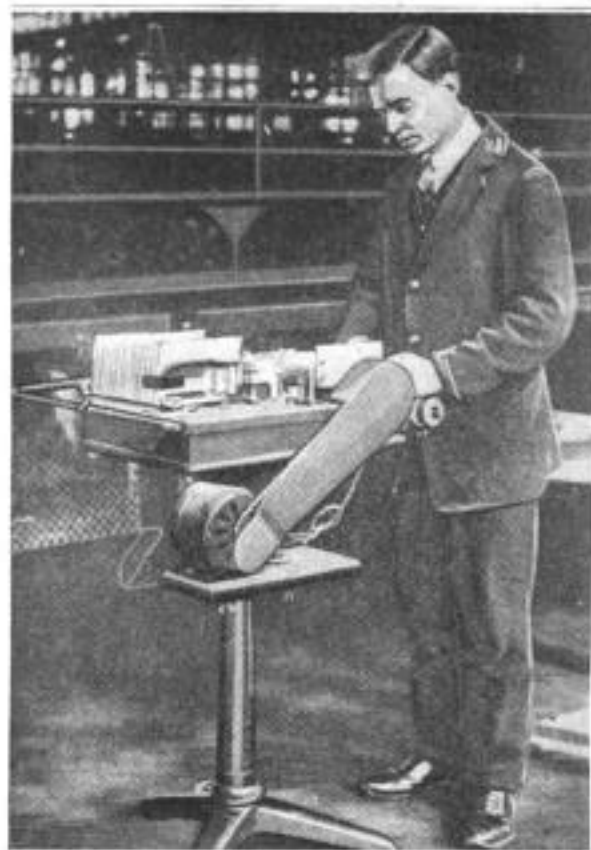
Stamp-Canceling Machine That Prints a Clear Postmark, Now being Tested in British Post Offices
