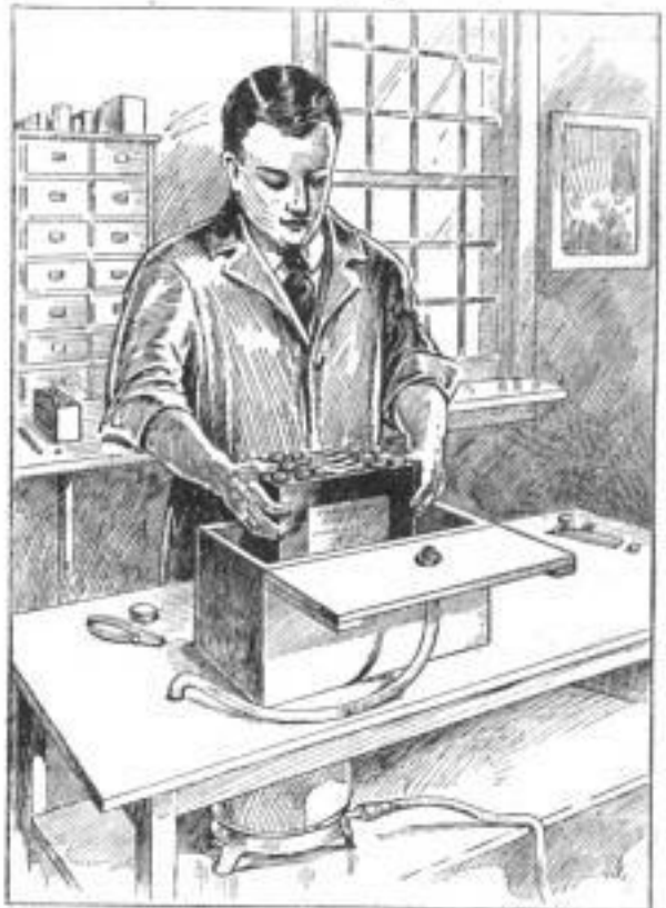
For Garages and Battery Service Stations a Storage-Battery Steamer will Greatly Facilitate the Removal of the Bituminous Sealing Compound When the Battery Elements or Jars are to be Removed
