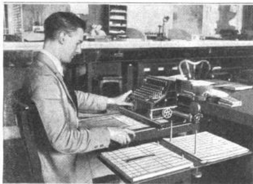
A Bookkeeping Typewriter of the Kind Now in Use in Washington Post Offices for Writing Money Orders and Their File Duplicates: Sheets of 10 Blanks, with Carbon and Second Sheet, are Used with the Aid of a Special Holder
