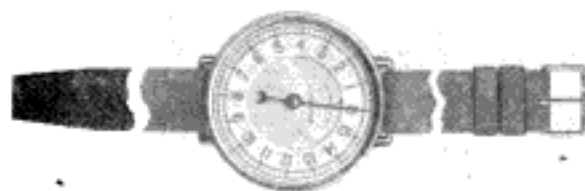
The Wristlet Altimeter, Worn Like a Wrist Watch, Accurately Shows the Height at Which the Wearer is Flying
