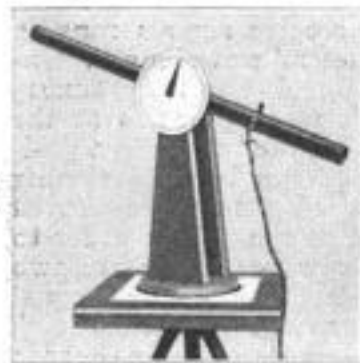
A Close-Up of the Mounted Coil, Showing Its Compass-Card Base, Inclinator Dial, and Sliding Connection Ring
