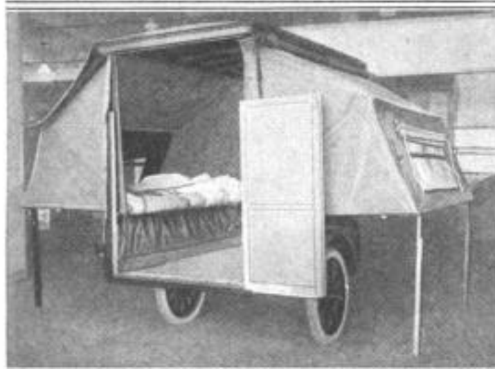
Two Views of a Well-Designed Touring Trailer: The Canvas Extensions Fold Inward, and the Telescoping Sides Permit the Top to be Lowered
