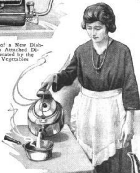
A Teakettle Bail with a Broad Metal Shield Protects the User's Hand from Scalding Steam When the Kettle is Tipped, as Above; and is Easily Attached, as at the Right
