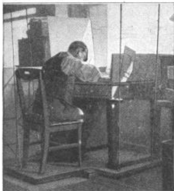
The Platform on Which the Engraver and His Table Rest is Hung Clear of the Floor by Wires from the Ceiling, Preventing Vibration
