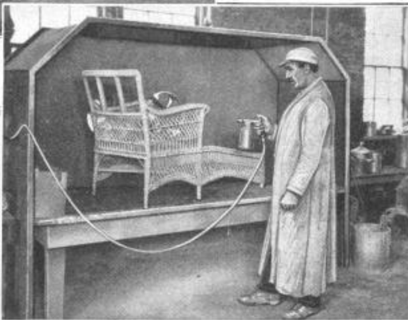
Left: The Type of Paint-Spraying Gun That Screws to the Top of a Mason Jar or Metal Paint Container. Right: Painting a Piece of Reed Furniture with This Type of Gun, in Less than Three Minutes
