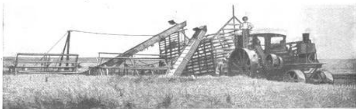
Grain Harvester and Stacker: By Carrying the Grain Along in the Rack Until Enough is Accumulated to Make a Good Stack, This Outfit, with a Crew of Five, Cuts and Stacks 40 to 60 Acres of Grain a Day
