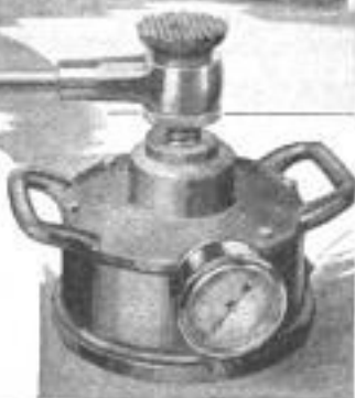
Above: Checking a Heavy Truck for Overloading by Placing a Metering Jack under Each Side of the Rear Axle, and Lifting the Wheels Clear of the Road. Right: A Close-Up of the Oil-Filled Hydraulic Jack with the Metering Dial on Its Base
