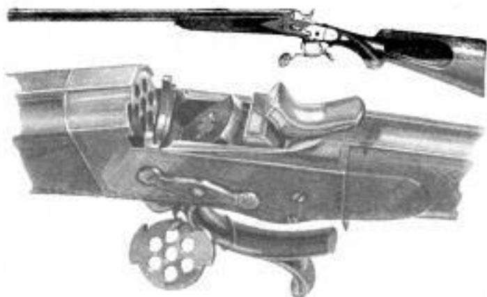
At the Top: The Curious Firearm in Its Entirety. Bottom: A Close-Up of the Seven-Barrel Breech and Lock Mechanism, with the Ejector Tied to the Guard
