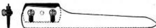
Right: View of a Safety-Razor Blade Fitted into the Handle of a Paper Knife. Left: The Blade Sinks into the Recess When Not in Use
