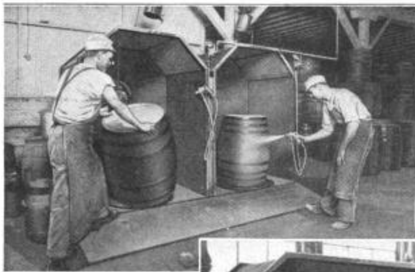
Using the Spraying Gun to Paint a Barrel, Which is Placed on a Revolving Base, Sprayed, and Removed in Less than One Minute
