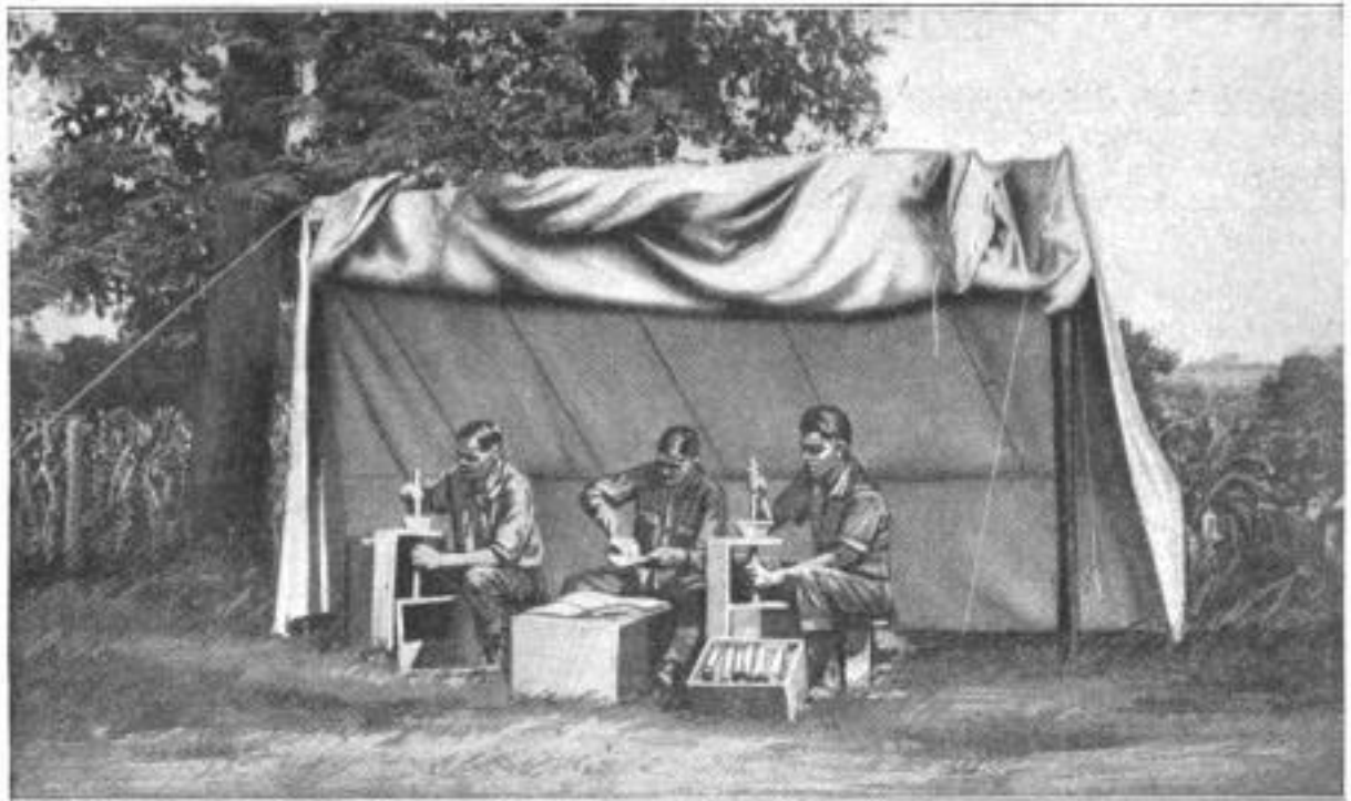
Workers on a Wisconsin Farm Packing Trinitrotoluene, the War Explosive, into Cartridges, like Dynamite, for Use in Blasting Stumps: Cartridges of the Usual Size, 1\frac{1}{4} by 8 Inches, Weigh 5\frac{1}{2} Ounces, as Compared with Eight Ounces for Dynamite
