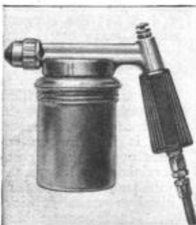
Left: The Type of Paint-Spraying Gun That Screws to the Top of a Mason Jar or Metal Paint Container. Right: Painting a Piece of Reed Furniture with This Type of Gun, in Less than Three Minutes
