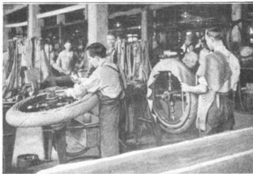
Building Tires by Hand: This Is the Older, Slower Method, but Many Manufacturers are Still Using It. The Workman to the Right has Thrown the Strip of Fabric Which He is Applying over His Shoulder to Keep it Clean
