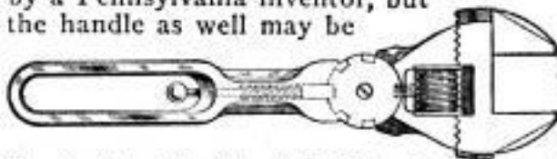
The Handle of the Wrench Is Adjustable at Several Angles to the Head by Means of the Plunger Bolt
