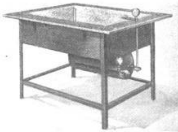
A Completely Self-Contained Automobile-Radiator Test Unit Has a Storage Tank Which Holds Air Enough to Make Several Tests
