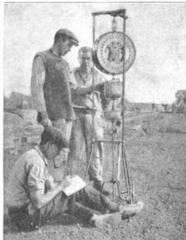
The Reverse Reading of the Subsoil Compactness Scale Shows That 18 Pounds of Shot have Passed from the Scale Bucket into the Lower One. The Small Dials Show the Penetration of the Vertical Rod into the Soil
