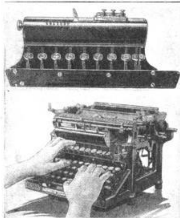
Top: The Adding-Machine Typewriter Attachment Alone. Below: As It Appears Installed on a Typewriter
