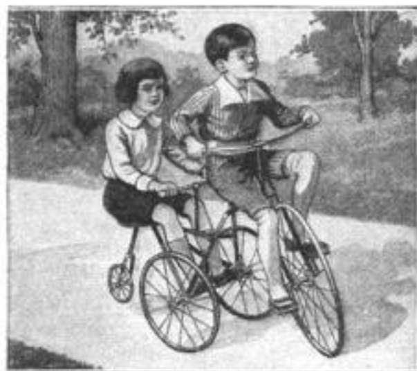
An Auxiliary Tandem Seat Attached to the Boy's Velocipede Makes It a Two-Passenger Vehicle
