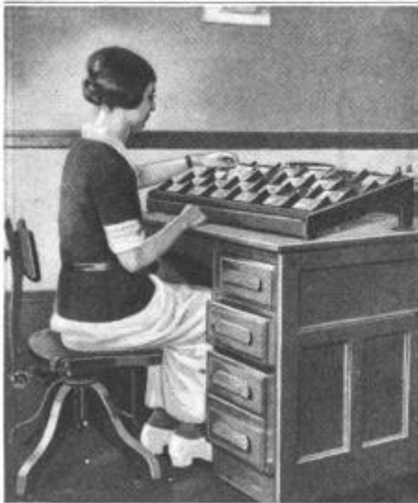
The Card Compartments, Raised by Turning the Button, Shaking the Cards into Their Proper Positions
