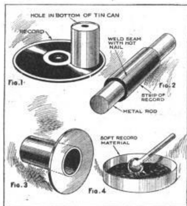
By Applying Heat and Working the Material While Hot, Old Phonograph Records Provide a Cheap and Satisfactory Insulating Material for the Amateur Electrician
