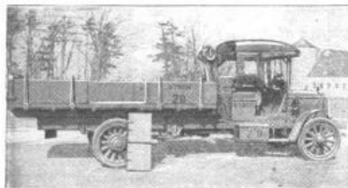
Above: The Multi-Purpose Truck Body with One of the Side Panels Removed. Right: Arrangement of the End-Gate Chute through Which the Load of Sand, Gravel, or Other Loose Material is Dumped at the Roadside, Out of the Beaten Track
