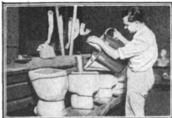
The Heated Wax is Poured into the Molds, Allowed to Harden into a Wall About Two-Thirds of an Inch Thick, and the Remainder Poured Off Again
