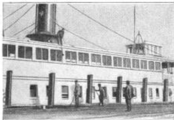
Washing the Outside of a Big Ferryboat with Soap Solution Applied with Long-Handled Swabs, and Washed Off Again with a Hose
