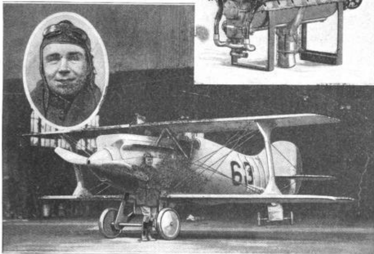
Lieutenant C. C. Moseley. Winner of the Pulitzer Trophy, and His Winning Mount, The Verville-Packard Plane: This Plane, Driven by the 600-Horsepower Engine, Shown Above, is Thought to Be Capable of a Speed of Three Miles per Minute
