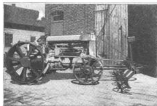
Left: Side View of a Tractor with the New Cultivator Attached to Its Front End, Keeping It Constantly under the Eye of the Driver, and Allowing It to be Steered with the Wheels. Right: Front View of the Machine
