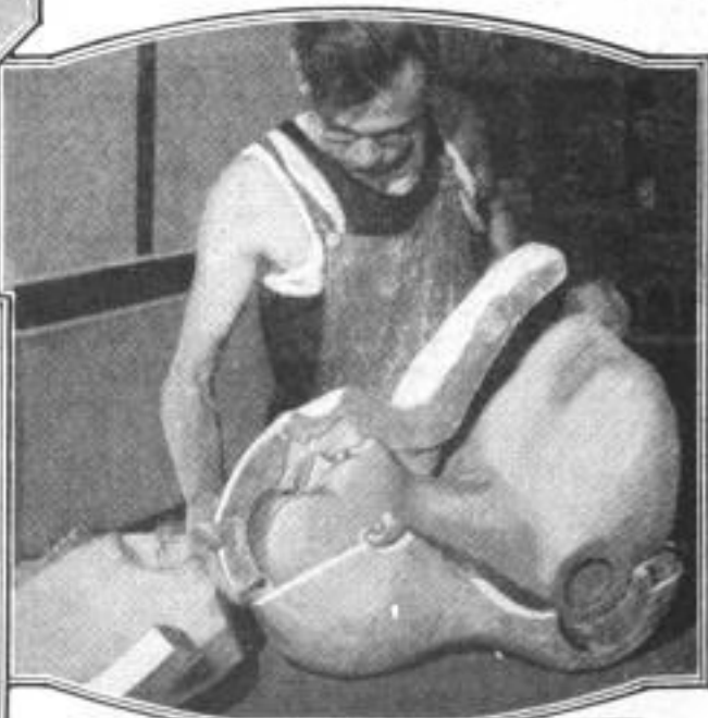
In Casting a Bust, the Mold of Clay or Plaster is Cooled with Water, and the Wax Figure Is Hollow, as Explained in the First Picture. When the Wax Walls have become Thoroughly Hardened, the Cast is Removed by Separating the Sections of the Mold, Which are Tied Together during the Pouring Operation
