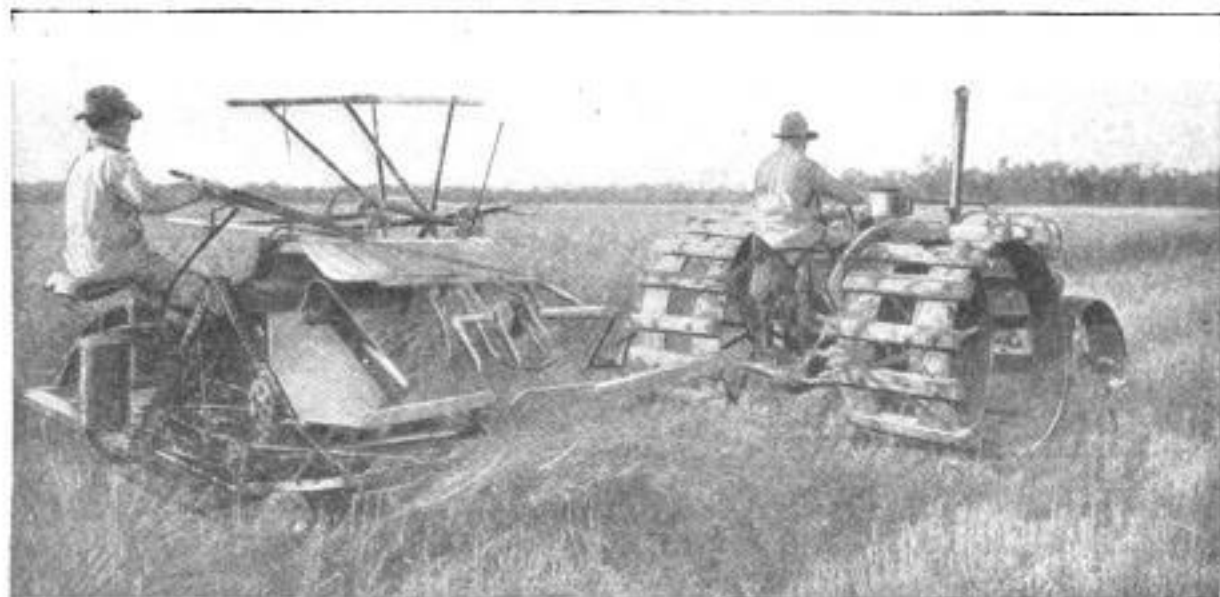
Tractors Used in the Wet Rice Fields are Prevented from Miring by Extension Strakes Attached to the Drive-wheels. Not Only do These Serve Perfectly to Support the Heavy Machines, They Also Assure Adequate Traction
