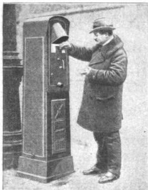
Depositing a Coin in the Slot of the Taxi-Call Machine Brings a Cab Promptly. Provided One is to be Had
