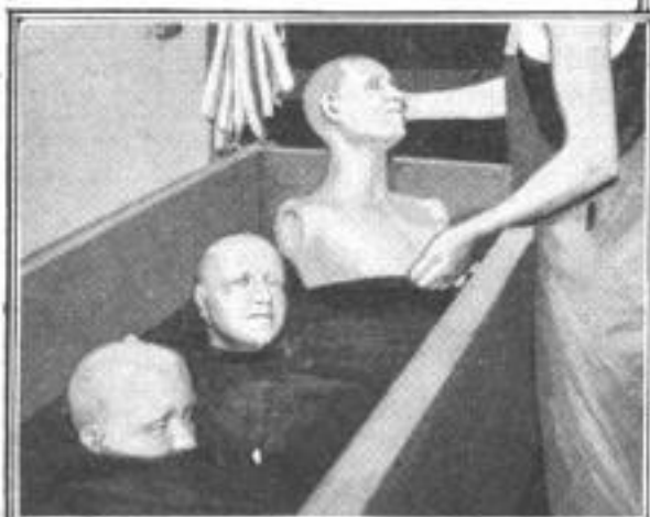
After the Wax Busts are Cast, They must be Thoroughly Washed and Dried Before the Faces are Retouched, Preparatory to the Final Tinting, and the Hair Selected and Fastened in Place
