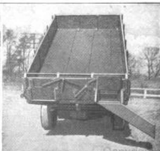
Above: The Multi-Purpose Truck Body with One of the Side Panels Removed. Right: Arrangement of the End-Gate Chute through Which the Load of Sand, Gravel, or Other Loose Material is Dumped at the Roadside, Out of the Beaten Track
