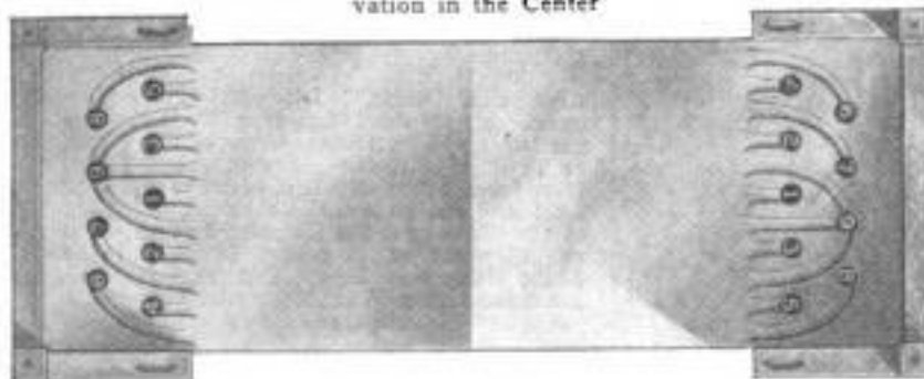
A Plan View of the Putting Green, Indicating the Numbers of the End Holes, the Channels Running to Them, and the Double Slope
