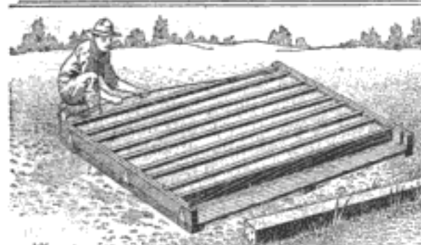
GANG MOLD FOR CONCRETE FENCE POSTS, TAPERED ON TWO SIDES
