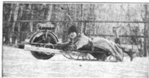
A Light and Easily Constructed Auto Sled Which Consists of Nothing More Complicated than a Motor Wheel Attached to an Ordinary Coaster
