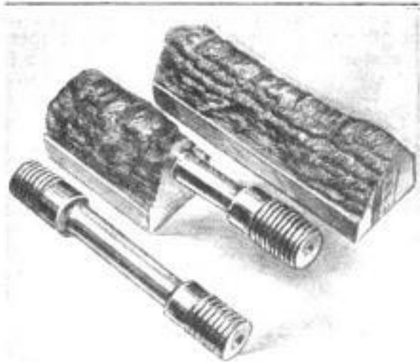
Pieces Cut from Blocks Built Up by the Welding Process, to be Used for Tests of Tensile Strength
