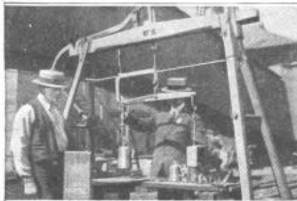
Testing the Accuracy of Customhouse Weights by Means of a Portable Scale Beam and Standard Weights
