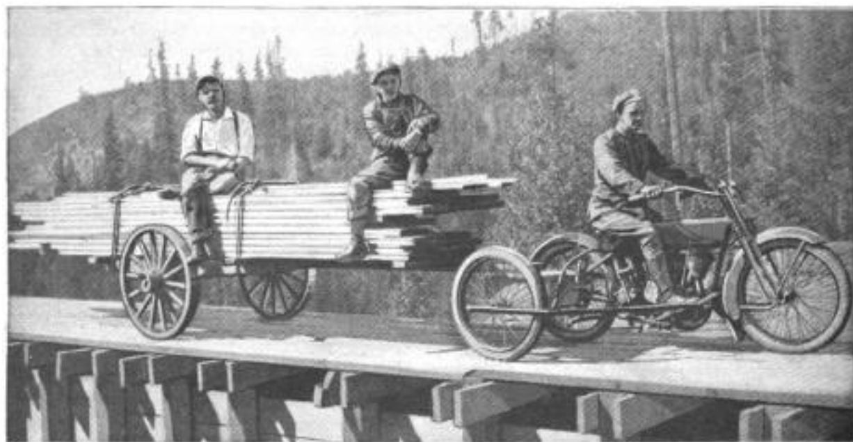
A Standard Stock Motorcycle Fitted with an Extra Rear Wheel Furnishes the Motive Power for a High-Speed Lumber-Carting Outfit. The Roadway Is the Top of a Flume in Which the Lumber is Used
