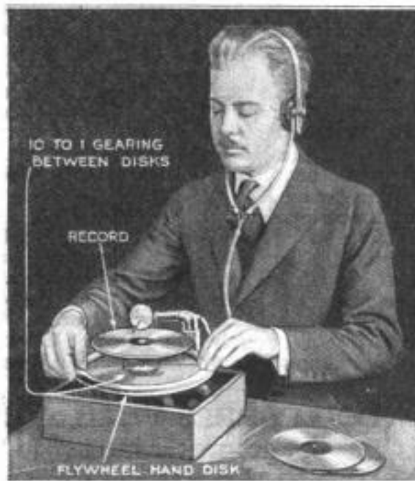
The Hand-Operated Phonograph, the Slowly Revolving Records of Which Carry Combinations of Four Dots Representing the Letters of the Alphabet: Blind Persons Soon Learn to Read These with Ease and Rapidity
