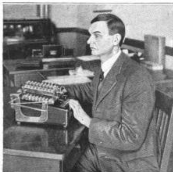
An Adding Machine with an Auxiliary Keyboard and Braille Totaling Figures, for a Blind Operator
