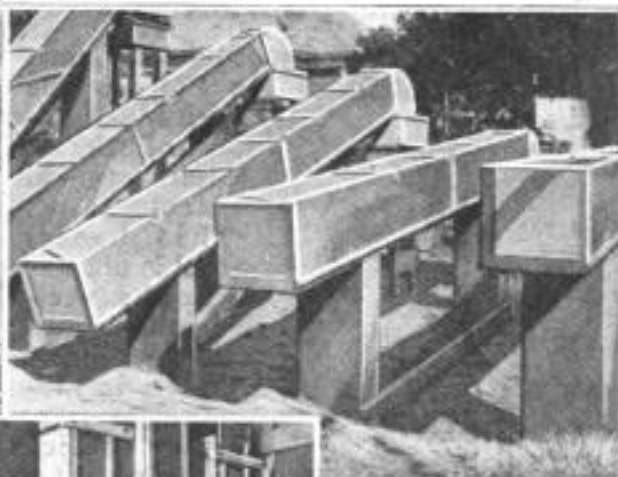
Shorter Test Units Arranged at Various Angles Decreasing to the Horizontal: The Seepage Was Slowest through the Latter
