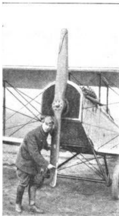
The Heavy Propeller of a Rice-Patrol Airplane, Known to the Airmen as "The Duck Slaughterer": A Lighter Blade would be Shattered When Tearing through the Flocks of Wild Fowl
