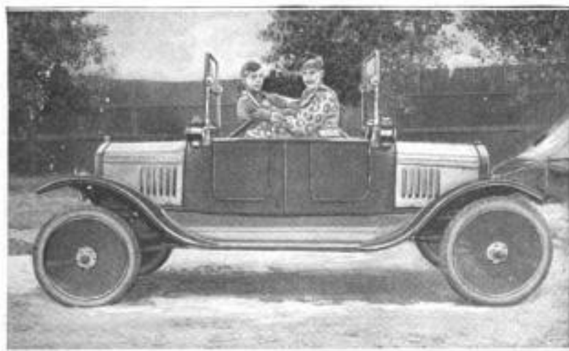
COPYRIGHT, INTERNATIONAL The Siamese-Clown Car Has All Important Units in Duplicate. This Permits Travel in Either Direction at Equal Speeds
