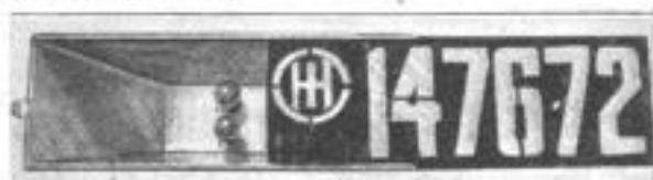
The Number Plate Partly Removed, Revealing the Red and Green Signal Lamps in the Metal Box
