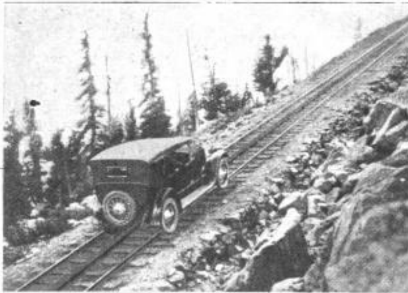
This Rough Road was Safely Traveled by a Motor Car Which Recently Made the Climb to the Summit of Pikes Peak over the Ties of the Cog-Railway Line. The Grade Shown Here Is between 25 and 28 Per Cent. The Average Rise Is 900 Feet to the Mile
