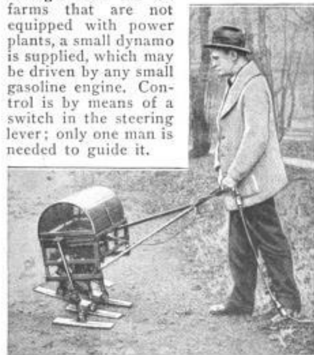
A Power-Tamping Machine Designed to Pack Silage Simulates the Stamping Action Usually Performed by the Feet of the Packer. Being Tilted at a Forward Angle, the Apparatus Walks and Requires Only to be Steered
