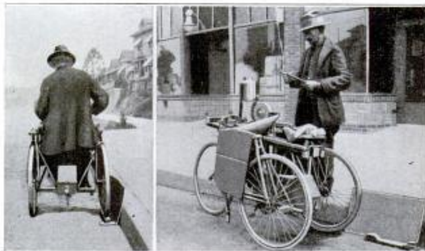
Two Views of a Homemade Grinding Outfit Constructed from Bicycle Parts: Pedals are Used to Drive the Grindstone but are Not Employed to Propel the Conveyance
