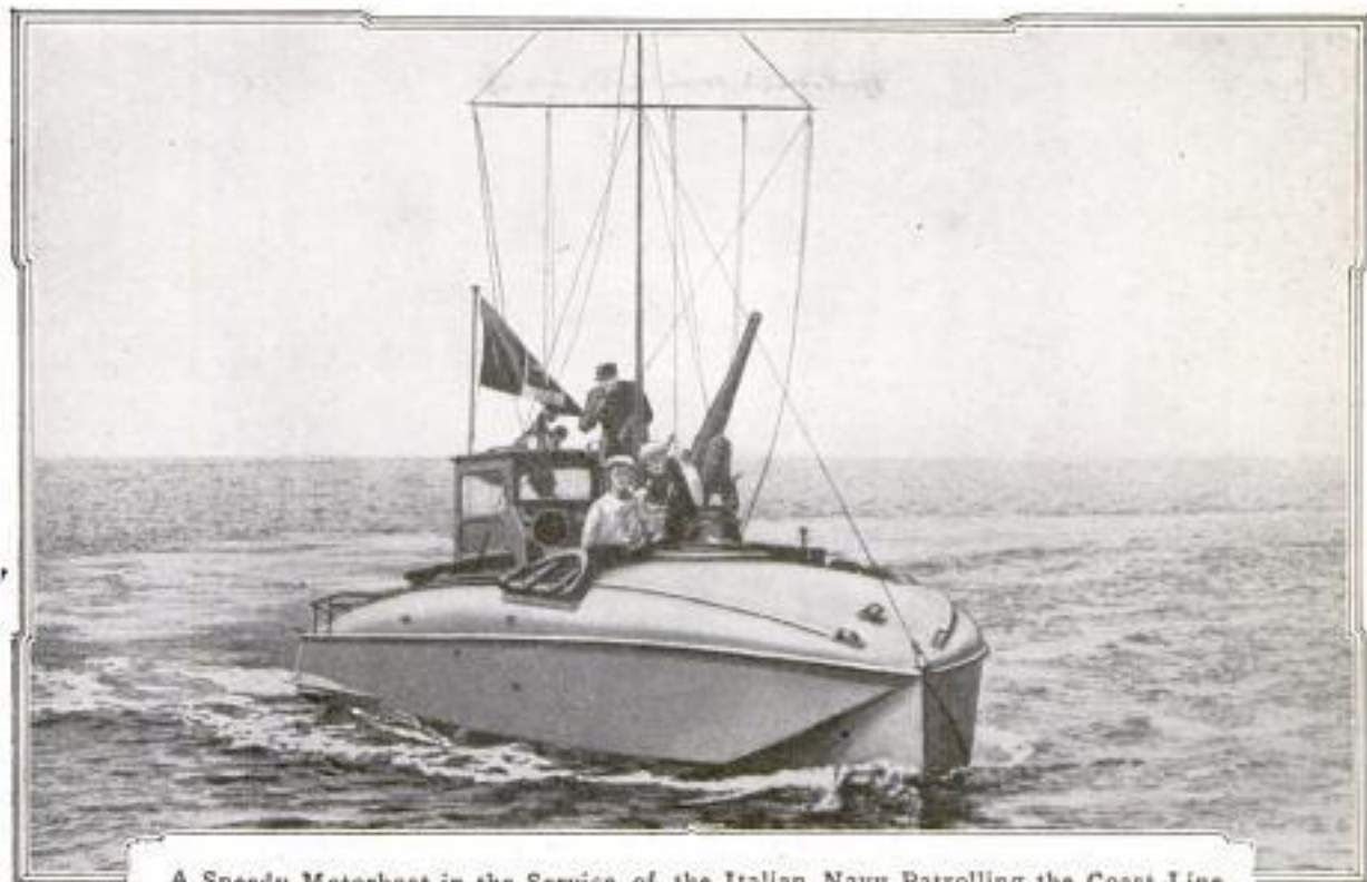
A Speedy Motorboat in the Service of the Italian Navy Patrolling the Coast Line and Maintaining a Constant Vigil for Enemy Fliers: The Craft Mounts a High-Angle Quick-Fire Gun at the Forward End of the Cockpit and Also Supports a Radio Mast. Such Vessels as This One have Proved Valuable throughout the War, and Many of Similar Character are Now Guarding Our Own Waters
