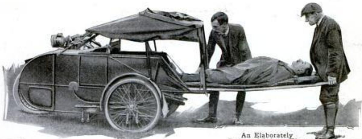
An Elaborately Equipped Sidecar That is Well Suited for Ambulance Service, as Shown Above and at the Left; In the Latter View a Patient can be Seen Lying Full Length in the Car. The Stretcher, Which is of the Folding Type with Wheel Supports, is a Part of the Outfit
