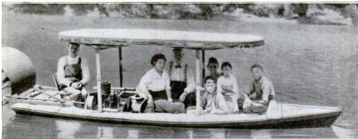
A 22-Foot Gasoline Launch Constructed by a Carpenter during His Spare Hours and Driven by an Engine Made from Parts Purchased from Junk Dealers and in Secondhand Machinery Shops
