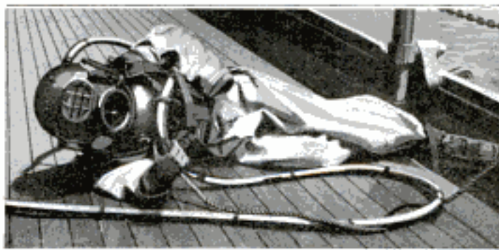
A Modernly Equipped Diver Ready for the Descent: His Suit Proper Is of Rubber and in One Piece. For the Sake of Freedom of Movement His Hands Are Bare
