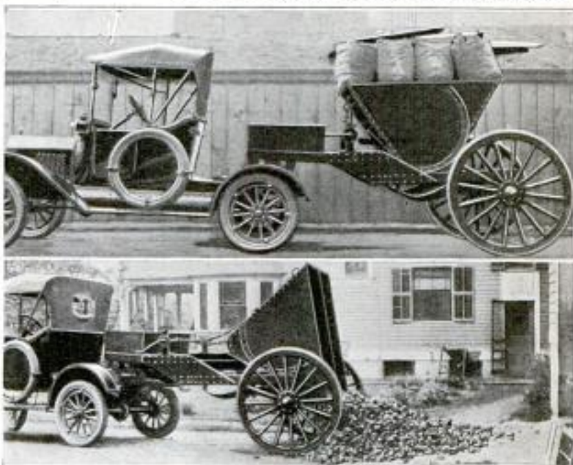
A One-Ton Coal-Carrying Truck That can be Quickly Attached to a Runabout: The Illustrations Show How It Dumps and Also How Coal in Sacks can be Carried
