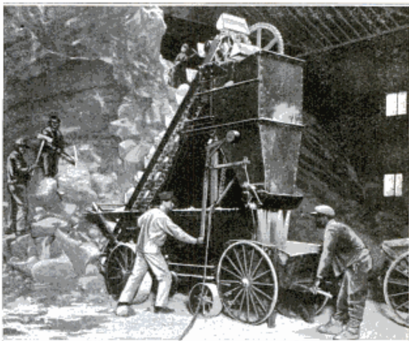
Machine for Loading Acid Phosphate: The Fertilizer Is So Hard That Drills are Used to Break It Up. The Loader's Capacity Is a Ton a Minute
