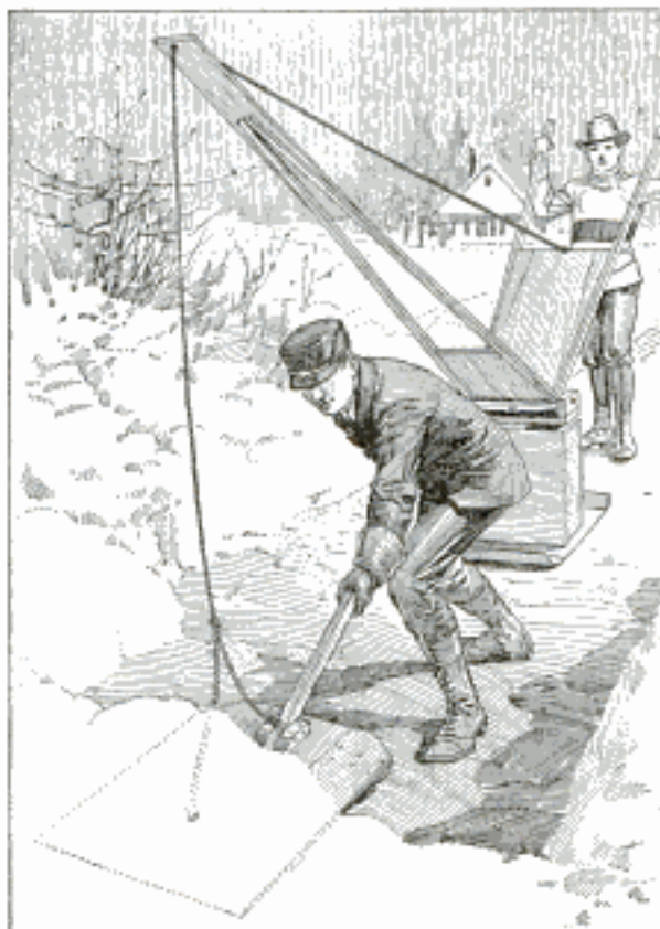
In a Very Heavy Snowfall, When Ordinary Snow Shovels Proved Inadequate, This Novel Two-Man Outfit was Built to Handle Large Loads Quickly
