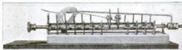
The Instrument Is of Compact Size, and Proportions Powder for a Druggist More Quickly Than Does a Spatula
