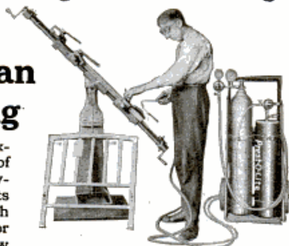
One of the oxy-acetylene welding operations employed in metal bed manufacture by The Simmons Company factories at Kenosha, Wisconsin
