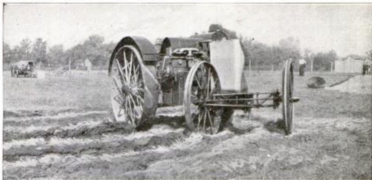
Tractor at a Country Fair with Front Wheels Cramped by Means of a Wire so That It could Run in a Circular Path without a Driver
