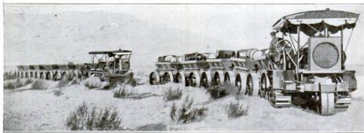
The New Way Which has Made Possible the Development of Many Desert Mining Fields: A Tractor and Its Trailers can Carry 25 Tons 20 Miles per Day
