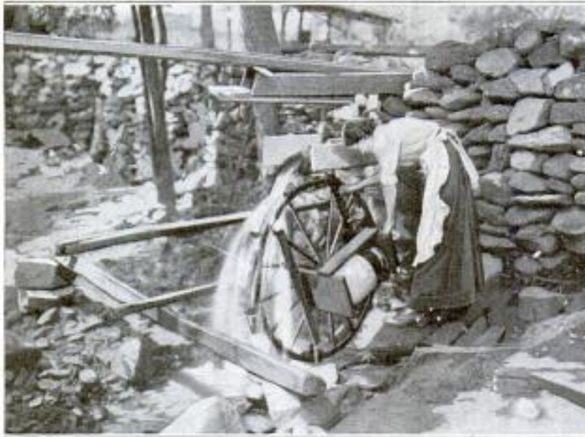
Water Wheel Made by a Farmer's Wife from a Few Articles Found Close at Hand: It Revolves the Churn 60 to 90 Times a Minute
