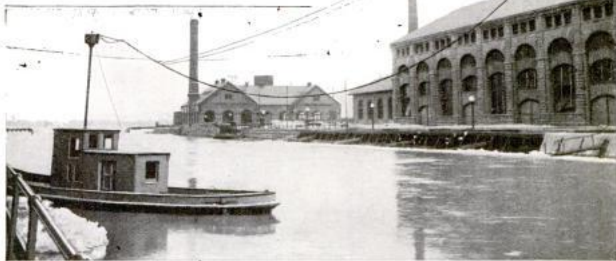
The Little Steel Boat, Driven by an Electric Motor, Breaks into the Ice Packs and Keeps the Intake Canals Open during Winter Months
