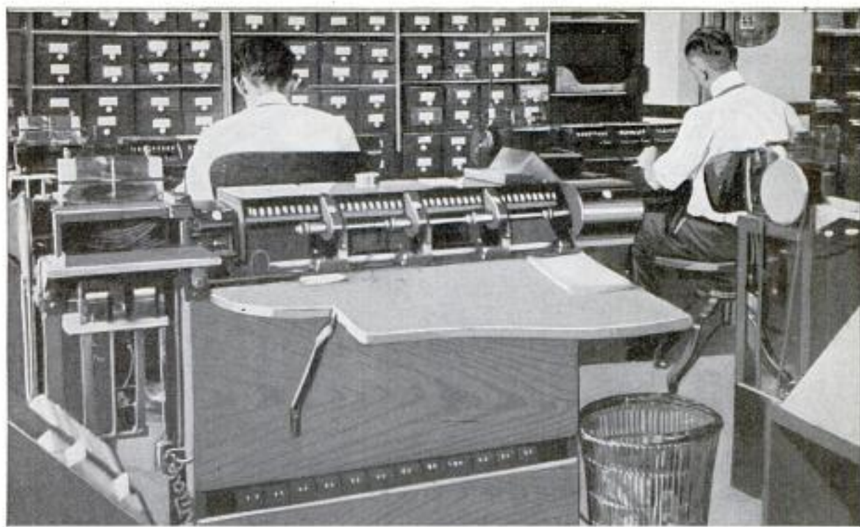
A Battery of Adding Machines Which Automatically Handle a Railroad's Record Cards, Making It Possible to Ascertain in Very Brief Time Such Items as the Total Weight of Certain Commodities Shipped between Two Given Points
