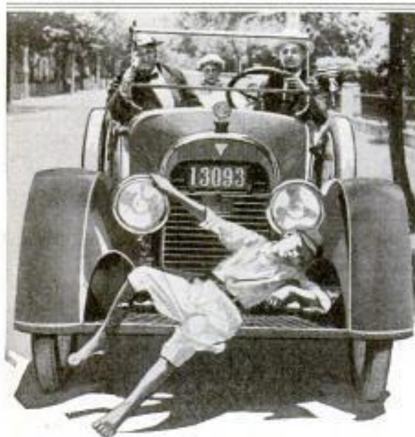
Automobile with Fender Designed to Pick Up a Person Who has been Accidentally Struck, Thereby Preventing His being Run Over
