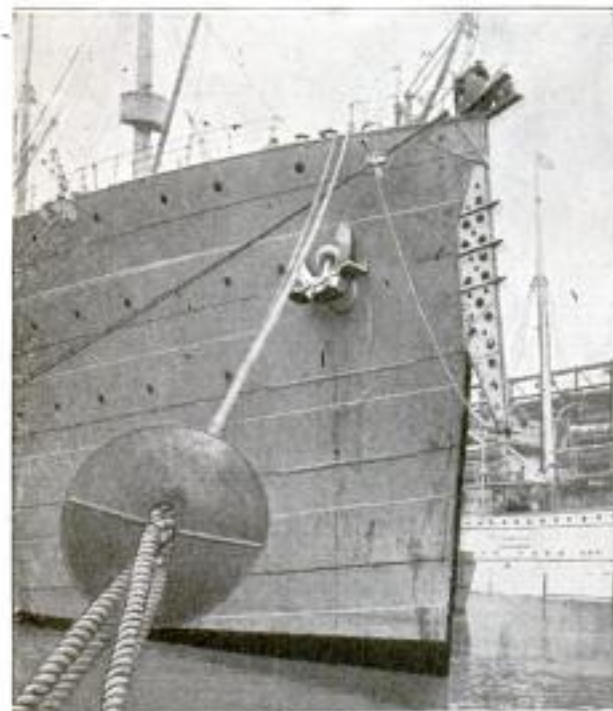
Bow of Steamship "Lapland" Showing at Least Part of the Mounting for One of the Mine Protectors: The Large Net That is Supposed to Extend Ahead of the Stem has been Removed
