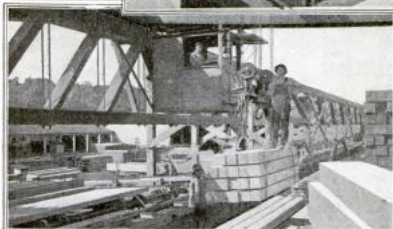
A Loading Crane in the Mill's Lumber Yard, Operated by Electricity: Where Power cannot be Delivered over a Wire, as in the Case of Trucks, Storage Batteries are Employed
