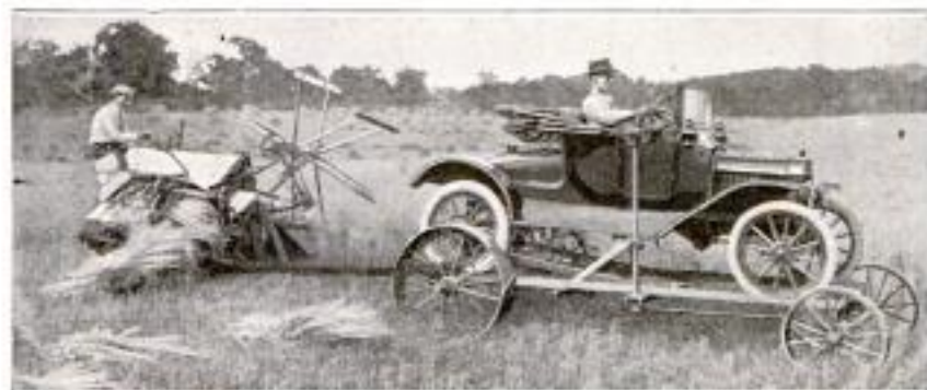
Steel Truck on Which Any Automobile can be Quickly Mounted and Used as a Farm Tractor: The Machine's Speed Is from Three to Five Miles per Hour
