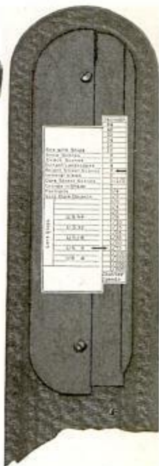
Slide Rule on the Side of the Camera Which Aids in Determining the Right Length for an Exposure
