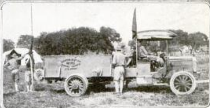
Instead of the Anchor being Raised and Lowered from the Ship, in Ballooning the "Ship" is Raised and Lowered from the "Anchor," Which, in This Case, is a Truck with a Powered Windlass on Which the Steel Cable is Wound
