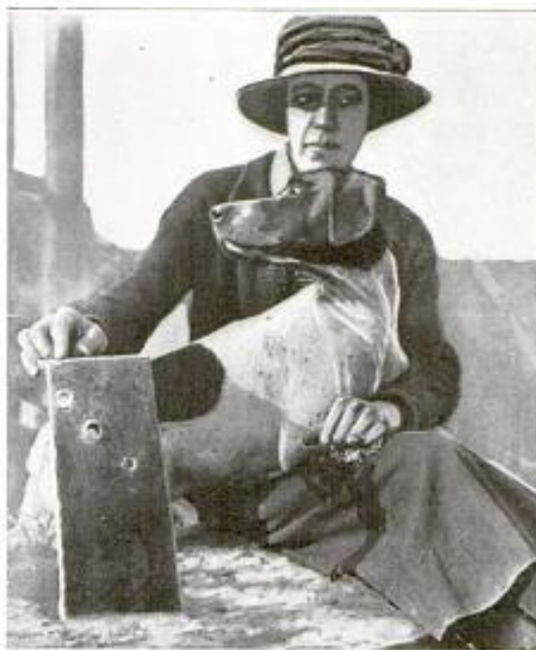
Plate of Half-Inch Steel Punctured at 300 Yards with the New Bullet: The Topmost Mark, a Dent, was Made with a Service Bullet at the Same Distance
