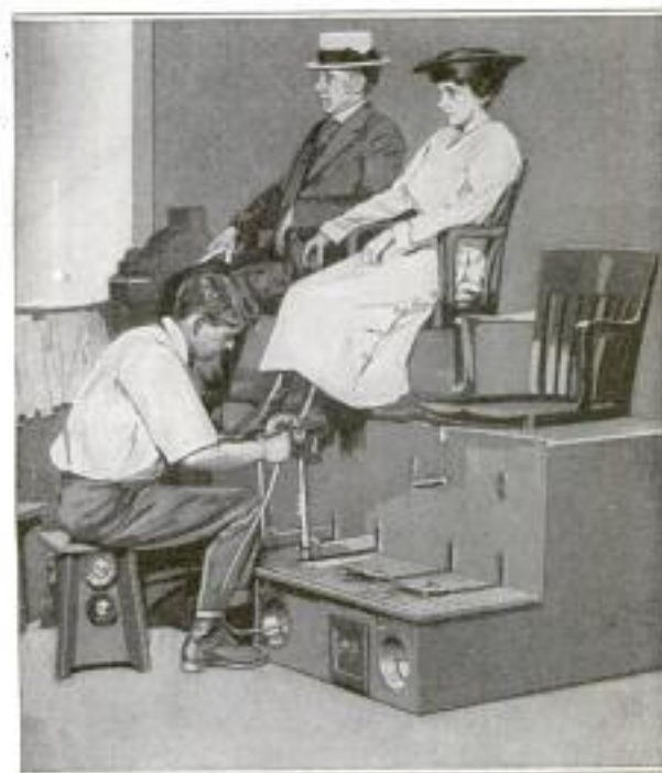
Adjustable Chairs, Disappearing Foot Rests, and Electric-Driven Brushes Are Outstanding Features of This Shoe-Shining Outfit
