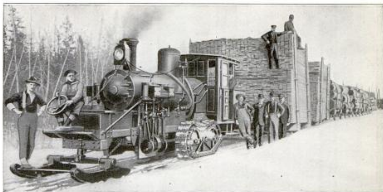
With Creeper Treads and Forward Runners, This Steam Locomotive Makes Six or Seven Miles an Hour While Pulling 15 Heavily Loaded Sleds over Snow-Packed Roads
