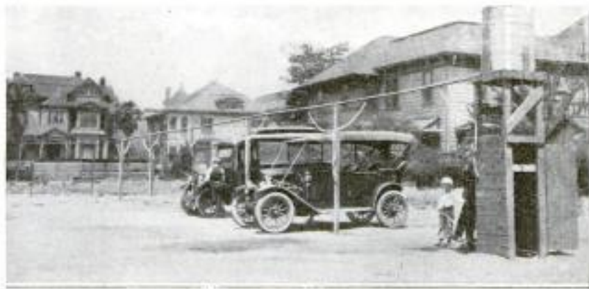
At This Outdoor Automobile Station, One Attendant Is Able to Remove Carbon from the Cylinders of a Dozen Cars Simultaneously
