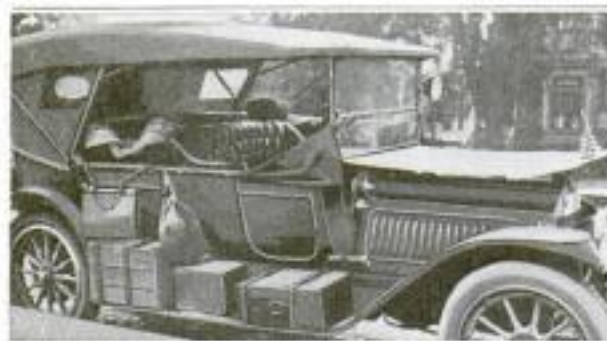
Prepared to Cross the Desert: An Awning Stretched above the Engine Hood to Shield the Radiator from the Direct Rays of the Sun and so Lessen Evaporation
