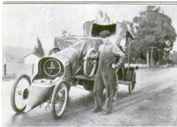
By Tying the Front Wheels of the Racing Car on the End Gate of the Loaded Truck This Motorist Was Able, Single-Handed, to Transport Both Machines a Distance of 40 Miles
