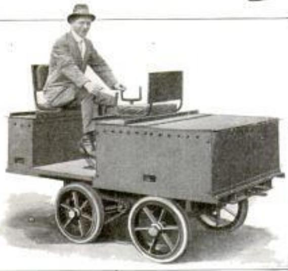
Two Pedals and Handles Control the Machine and may be Manipulated from Either Seat. The Arrangement Eliminates Much Needless Turning
