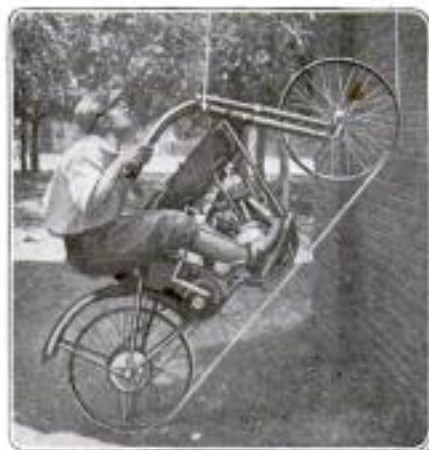
The Beginning of the Climb is Shown in the Left-Hand Picture. One End of the Wire is Fastened to the Rear Rim While the Other is Attached to the Steering Head.
