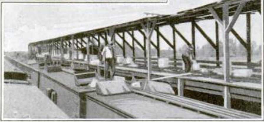
As the Conveyor Shoots the Big Cakes of Ice Along, Men with Long Spears Shove Them onto Runways Leading to the Icing Holes at Opposite Ends of the Cars through Which They are Dropped to the Bunkers. During a Normal Melon Season about 20,000 Tons of Ice are Used at This One Station
