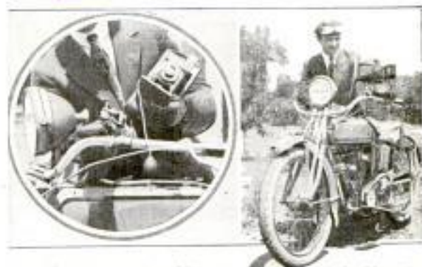
Two Views Showing Motor cycle Handlebars Fitted with Tripod Head to Support a Camera
