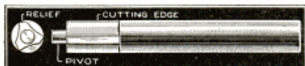
A Counterbore of This Type can be Ground Quickly from a Piece of Tool Steel, Which is Then Properly Tempered
