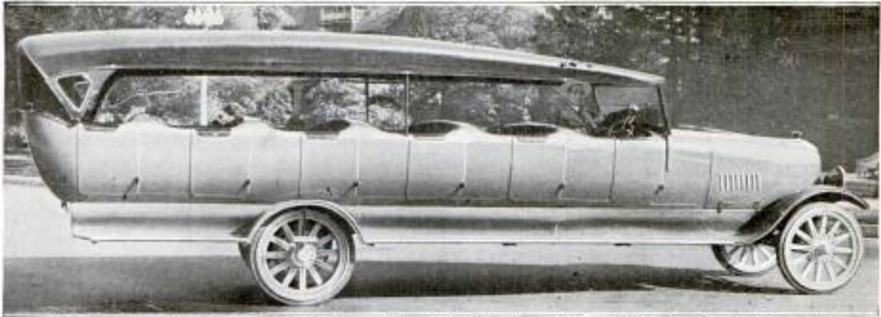
This Car with Six Cross Seats Conforms More Nearly to the Ordinary Touring-Car Design. The "One-Man Top" is Not Misnamed, for One Person can Open and Fold It
