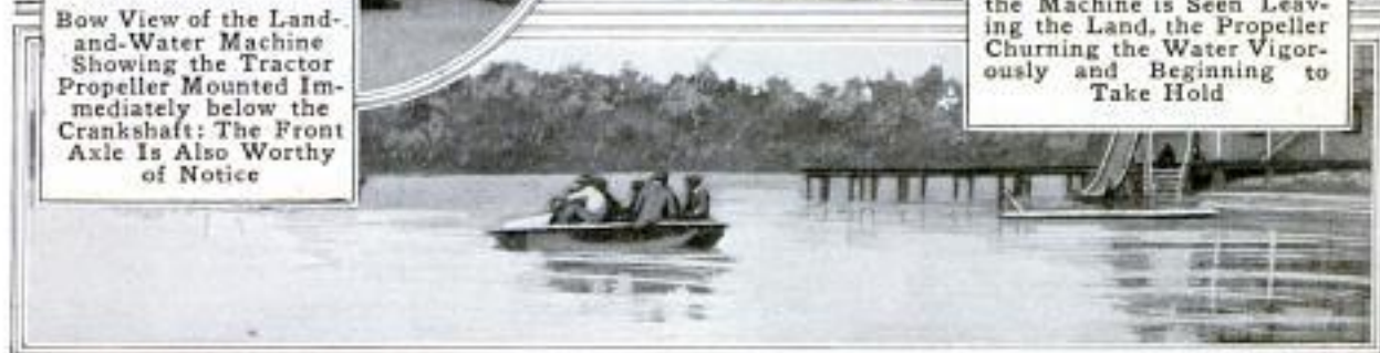
The Front of the Engine Compartment is Sealed by a Steel Bulkhead so That Water can Not Enter through the Radiator. As may be Seen Above, the Car Serves Efficiently as a Motorboat When a Deep, Bridgeless Stream has to be Negotiated
