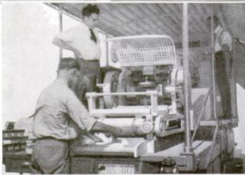
One of the Machines at Work: With Five Men Attending to Its Operation, It Produces 6,000 Loaves of Bread an Hour
