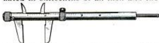
A Caliper for Making Any Inside, Outside, or Depth Measurement up to Four and One-Half Inches or 11 3/4 Centimeters
