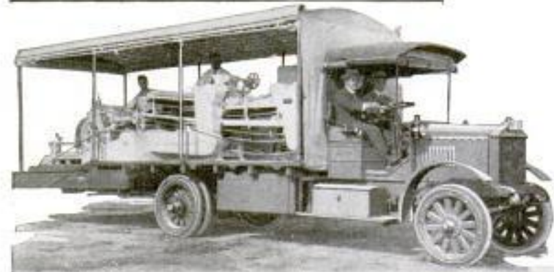
General Appearance of the Bread-Making Apparatus, Which Is as Portable as the Ordinary Field-Kitchen Outfit
