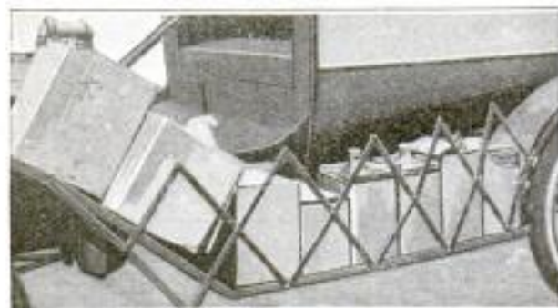
Lazy-Tong Type of Holder for a Running Board: It is Light and Durable and can be Folded Back against the Rear Fender When Not in Use
