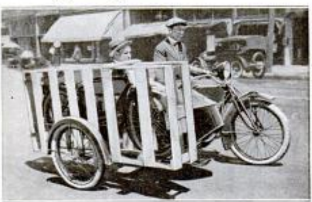
The Adjustable Axle Provides Space between the Sidecar and the Outer Wheel for a Small Platform on Which to Carry a Crated Motorcycle
