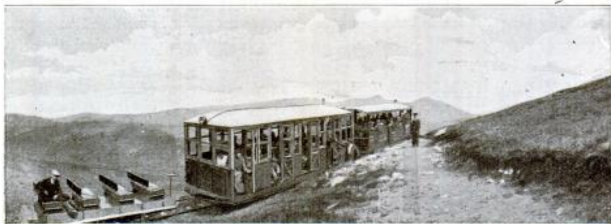
The Gasoline Railroad Motor Cars and Trailer at the Summit of Mount McClellan
