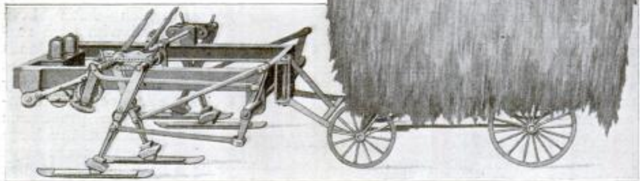
Not a Comic Cartoon, but a Drawing Showing a Four-Legged Farm Tractor Hitched to a Hayrack, is Presented Above. The Machine, Seriously Designed for Real Work, Is Literally a Motor-Driven Steel Horse
