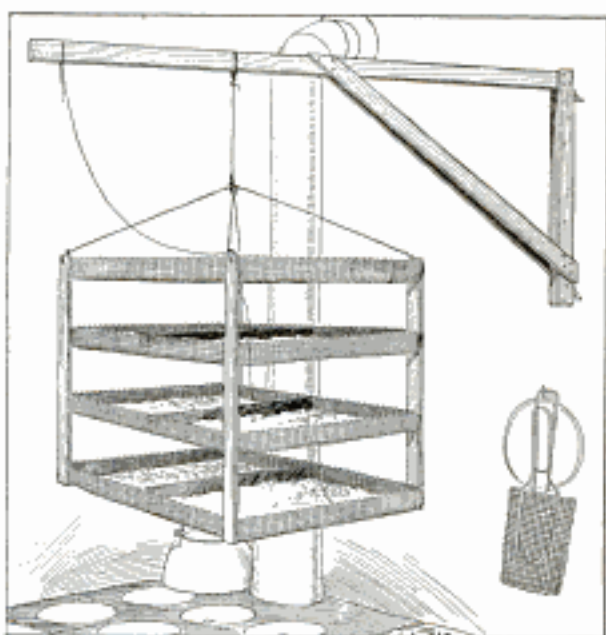
Fig. 2—This Multiple-Deck Tray Arrangement Utilizes the Waste Heat from the Stove, and can be Swung Aside When in the Way for Cooking
