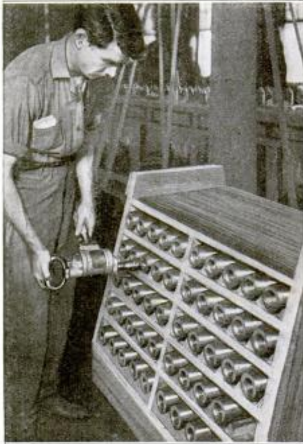
COURTESY OF MACHINERY Cleaning the Threads of Shells with the Aid of the Motor-Driven Wire Brush
