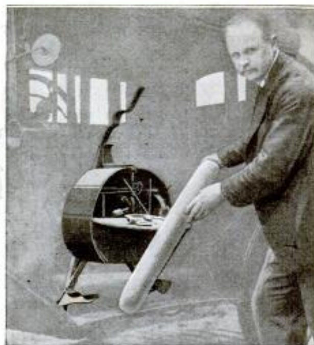
Showing Interior of Upper Compartment Provided in Tire Rack for Storage of Tools
