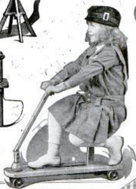
This Coaster Has a Fine New Feature. The Seat and Post can be Held Down Out of the Way with One Foot, While Getting Up Speed. When Ready to Coast, Move the Foot, and Up Springs the Seat into Place, as Shown
