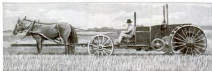
With the Fore Truck of a Wagon in Place, It Was an Easy Matter to Steer the Broken Tractor and Keep It at Work
