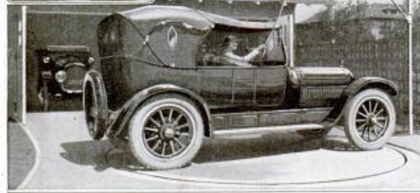
The Push Button Hangs within Easy Reach, Enabling the Driver to Start and Stop the Turntable without Leaving the Car
