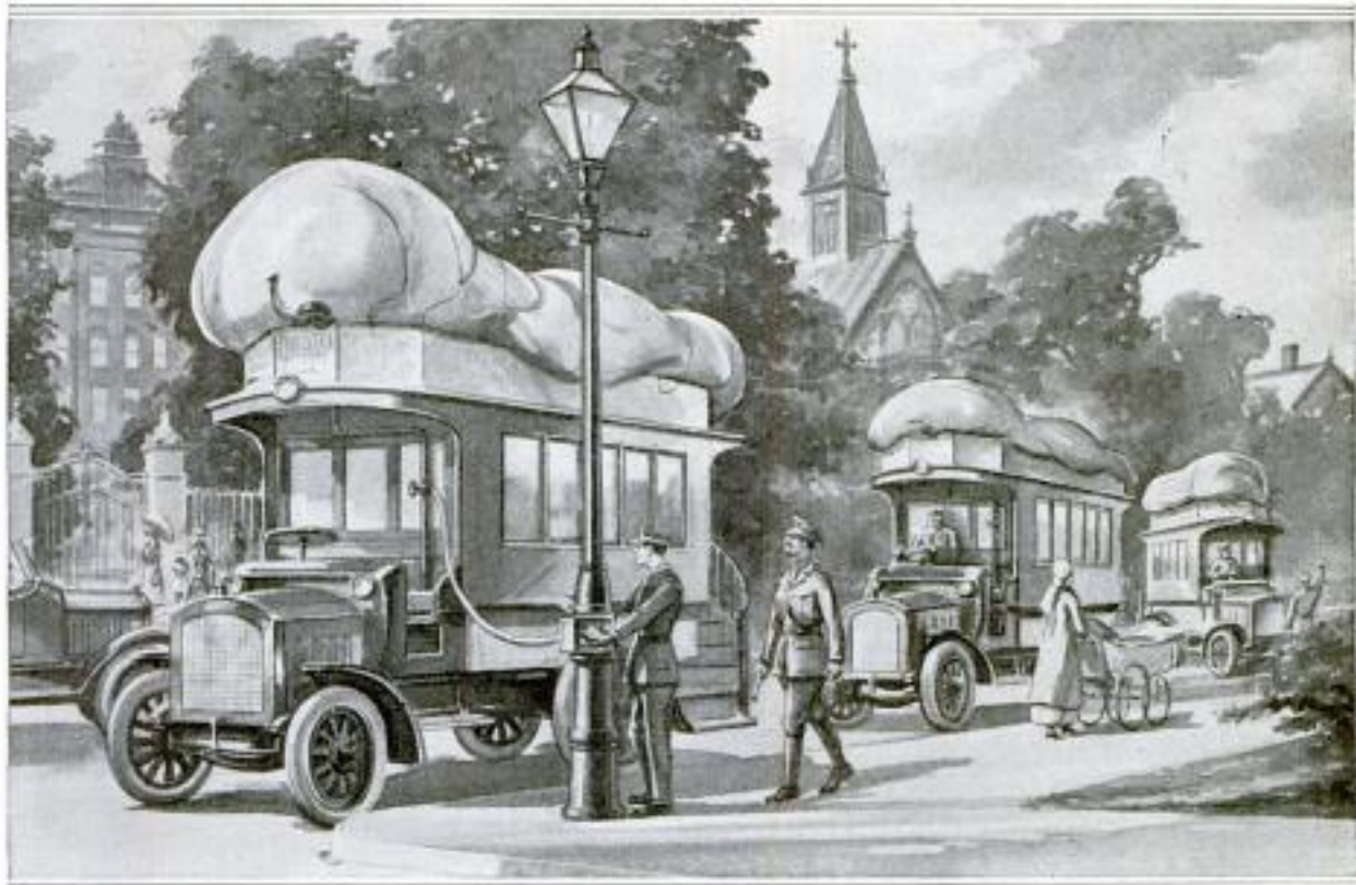
Inflating the Gas Bag at a Filling Station: London Motor Busses Operating between the City and Its Suburbs are Said to Use Illuminating Gas Instead of Gasoline for Fuel
