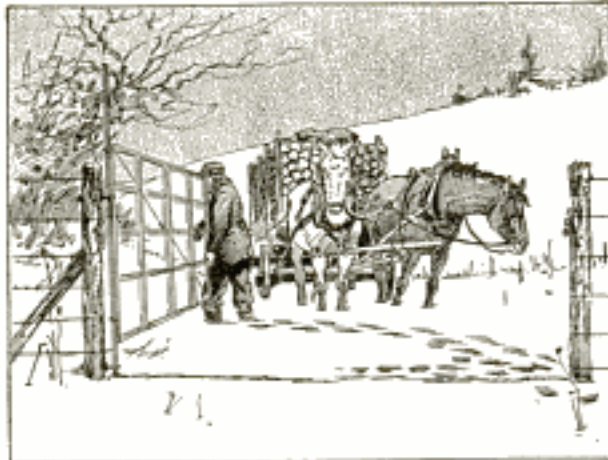
Instead of Shoveling a Path for the Gate at Its Usual Level, It is Raised and Supported on Pins Set in the Long Pipe
