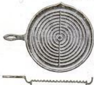
Broiler and Frying Pan Combined: Grease Runs from Corrugations into the Outer Ring Where It is Not Apt to Burn
