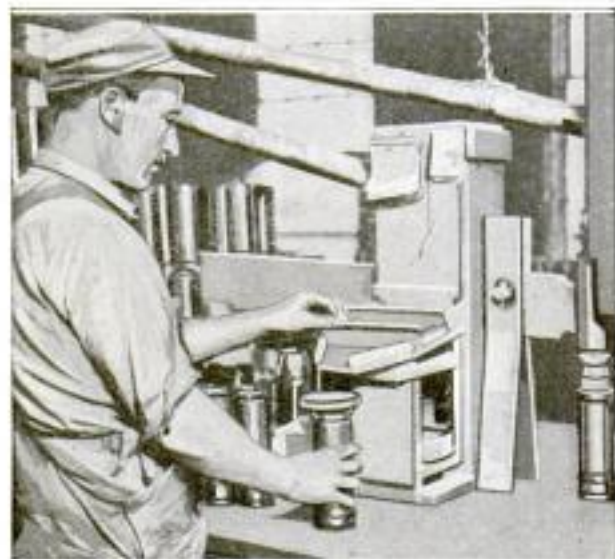
Filling Shrapnel in a Modern Munitions Plant: An Ingenious Arrangement Releases the Correct Number of Balls at Each Operation
