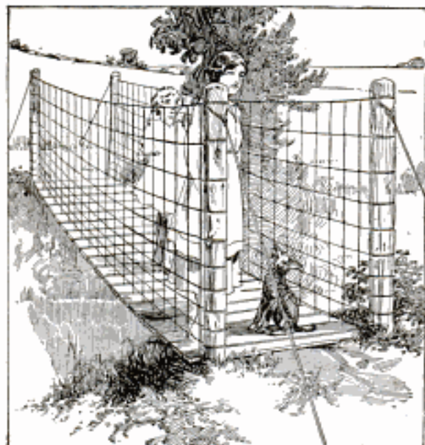
A Practical Bridge for a Small Stream on a Farm was Made by Supporting the Footboards on Woven-Wire Fencing
