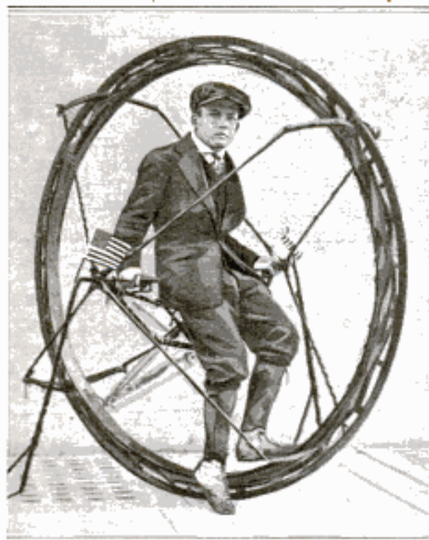
Unicycle Built 35 Years Ago and, after a Generation of Disuse, Ridden in a Recent Parade: The Rider Paddles with His Feet and can Make Good Time on a Level Road
