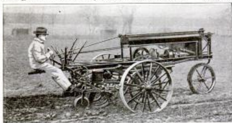
Side View of the Machine, Showing It in Use as a Corn Planter
