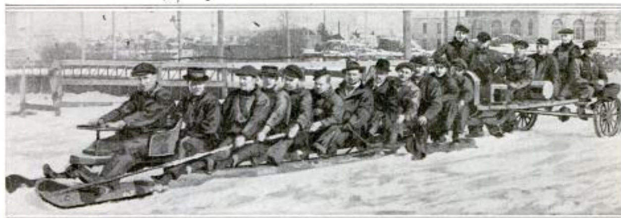
Hybrid Conveyance Employed in the Northwest, Consisting of a Long Bobsled Driven by an Automobile Stripped of Its Body and Front Wheels
