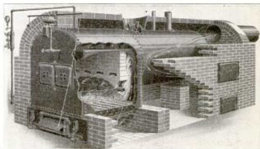
Diagrammatic View of Fire Box Showing Brick Partition Dividing It into Two Parts: Heated Air and Gases Pass through the Openings Down into the Burning Fuel and So Promote Combustion. The Perforated Plates are Not Shown
