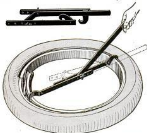
Contracting a Rim with a New Tool for Tire Removal: The Tool Is Adjustable to Any Size of Rim
