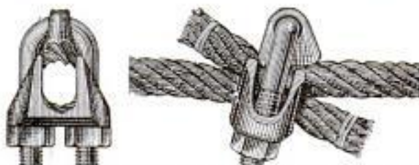
As the Pull upon the Spliced Cable is Increased the Clamp Tightens Its Grip
