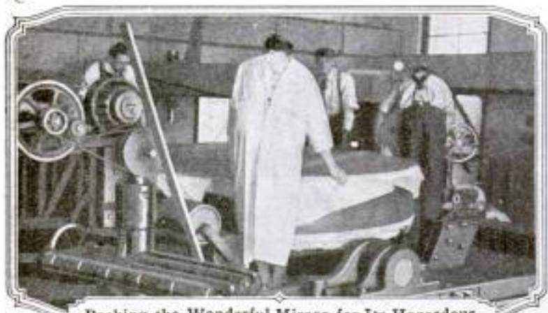
Packing the Wonderful Mirror for Its Hazardous Trip: Its Surface was Protected by Thick Layers of Cotton, on Top of Which Heavy Paper was Placed Before a Wooden Covering was Fitted. The Mirror Is 101 Inches in Diameter and was Cast at St. Gobain, France, in 1906.
