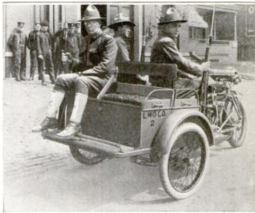
Showing a New Cart Attachment for Military or Police Motorcycles That Allows Four Men to be Carried: Under the Seats Is Storage Space for Arms and Ammunition
