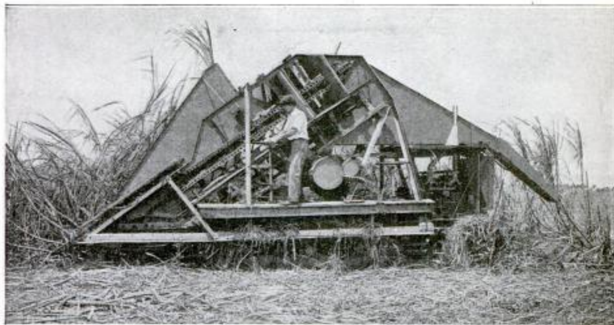
The Heavy Cane Harvester is Carried on Creepers so That Soft Ground Has No Terrors. It Delivers the Stalks Ready for Grinding
