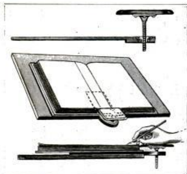
With the Arm Rest in Place, It Is Easy to Make Entries at the Bottom of a Ledger
