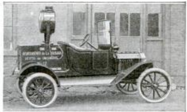
Mobile Searchlight Equipment of the Havana, Cuba, Fire Department: The Box below the Light Contains Electric Batteries and Other Equipment
