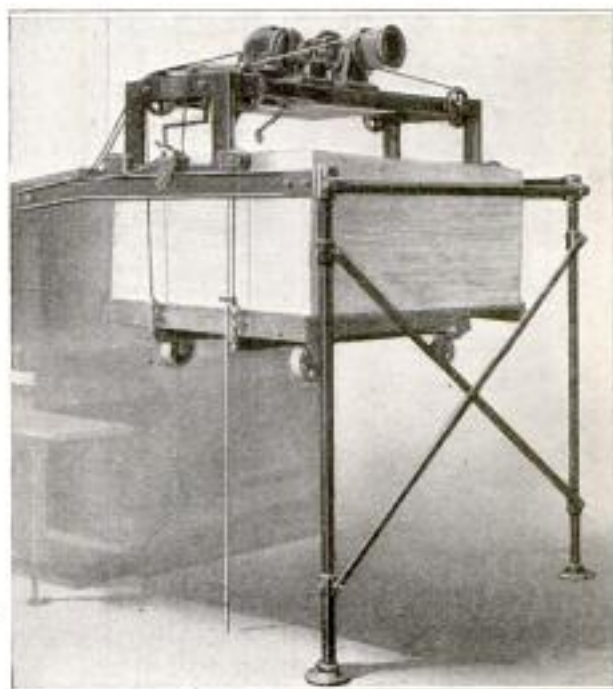
Showing One of the Paper Elevators, Attached to a Flat Press, in Actual Use
