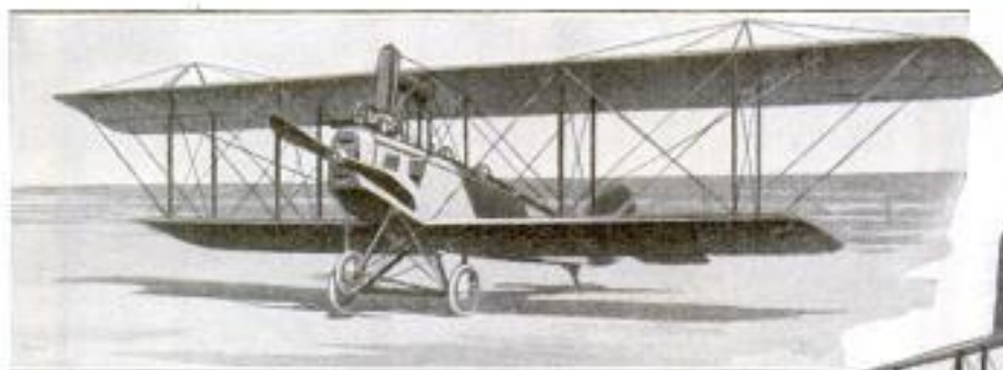
The Three-Wheel Landing Gear Is a Noticeable Feature of This New Biplane, Which is Now being Supplied to the Govern-
