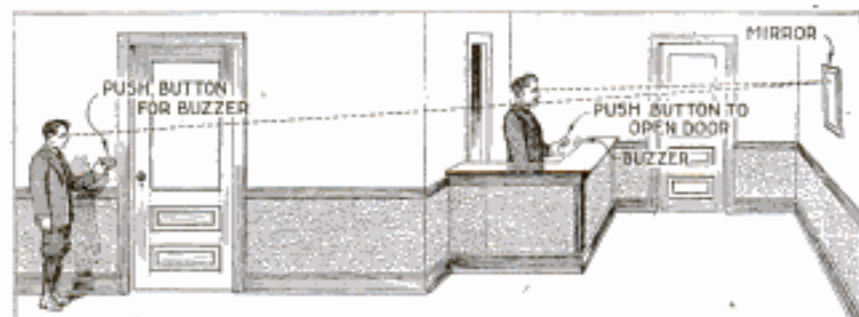
The Attendant Identifies Those Who are Admitted, and Releases the Door by Means of the Push Button
