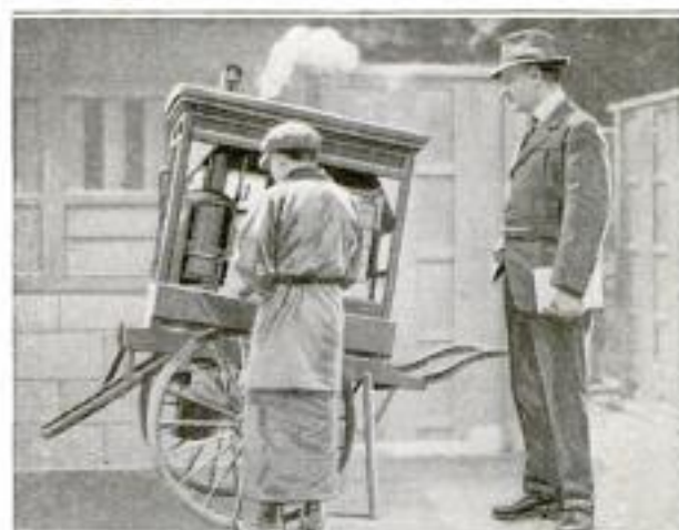
Japanese Itinerant Worker Cleaning a Smoker's Pipe: His Portable Outfit Includes a Little Copper Boiler from Which a Jet of Steam is Forced into the Pipe After It has been Swabbed Out
