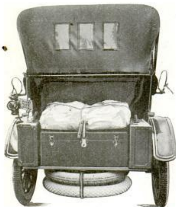
Steel Rack Which can be Easily Attached to the Rear of an Automobile: It can be Used to Hold Tires Only or to Carry Sacked Grain, Baggage, or Other Articles in Addition to the Tires
