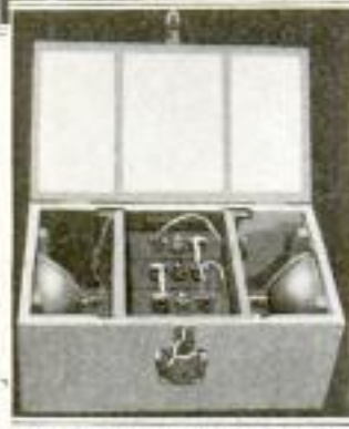
The Portable Lights, Showing the Storage Batteries in the Center and the Lamps Installed at Either End
