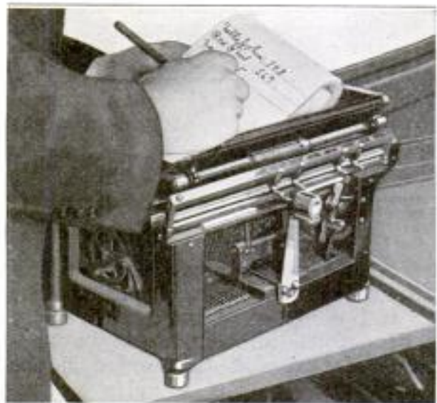
The Cyclometer Attached to This Machine, Engaging the Escapement Wheel, Records the Number of the Typist's Strokes, Thereby Furnishing an Accurate Measure of the Work Done
