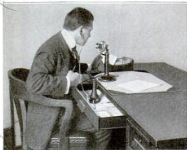
In Addition to Magnifying the Sound Vibrations, the Device Excludes Foreign Noises from the Telephone User's Ears.
