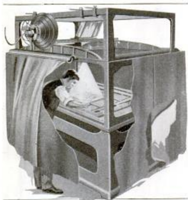
Registering a Printer's Form for the Press by the Aid of a New Projector, Which Throws an Image of the Copy Downward from Above: The Man Works inside a Curtained Inclosure While Adjusting the Plates
