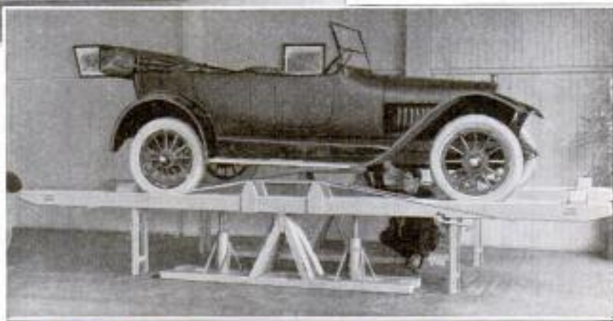
The Runways Take a Horizontal Position When Car Passes Center; Oil-Cushioned Plungers Bring This About without Shock
