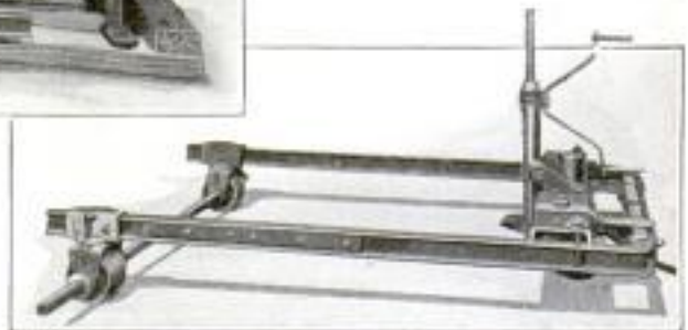
The Jack by Which the Load is Tilted is Shown at the Right-Hand End
