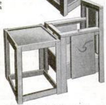
Above Are Two Views of a High Chair That can be Changed into a Low Chair and Table. Under the Seat Is a Place for Baby's Things
