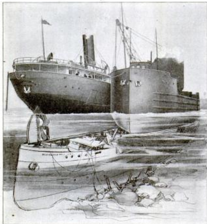
Showing the "Wissahickon" atop the Submerged Coal Boat, and the "Rescue" Alongside, Taking Over Its Cargo
