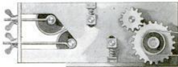
The Arrangement of the Rollers, Which Hold the Two Belts in Close Contact, is Illustrated at the Top. The Second Drawing Shows How the Tension is Maintained and Illustrates the Gearing That Causes the Belts to Travel at Different Speeds
