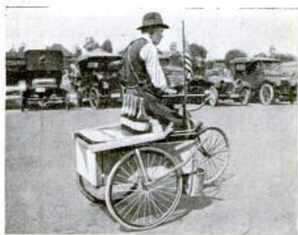
Portable Soft-Drink Stand: The Box is Divided into Two Compartments, One Containing Ice and the Other Various Utensils. Holders are Provided on Top for Bottles and Glasses
