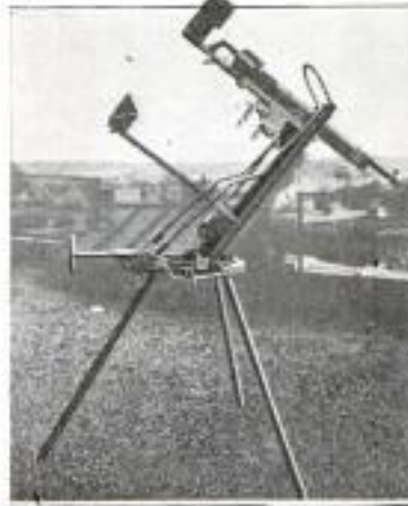
New Machine-Gun Mount with the Gun at 45-Degrees Muzzle Depression, Commanding Streets from a Roof
