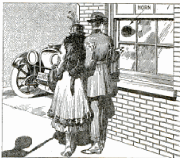
The Warning Horn Set in the Metal Window Pane Is Effective in Safeguarding Pedestrians
