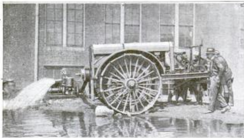
This Farm-Tractor Engine is Driving a Pump for Drawing Water from a Flooded Cellar in Norfolk, Nebraska
