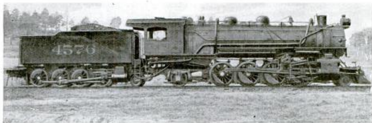
One of the "Duplex" Locomotives of the Southern Railway, Made by Mounting the Tender on the Running Gear of an Old Light Locomotive, Thus Making an Auxiliary Tractor Which is Supplied with Steam from the Engine Boiler
