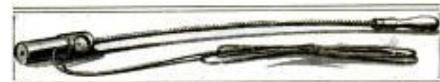
The Little Lamp at the End of This 18-Inch Handle Is Convenient in Examining a Motor. The Magnet Enables One to Pick Up Small Metal Parts Easily
