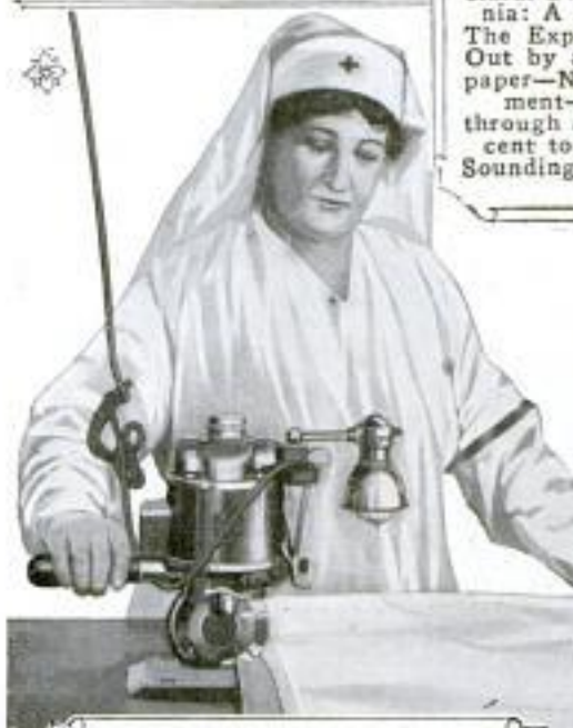
Red Cross Worker Employing an Electric Machine That Cuts Gauze into Bandages of Various Widths: Many Thicknesses of the Flimsy Material are Cut Smoothly and Quickly in a Single Operation by This Machine Driven from an Ordinary Lighting Circuit
