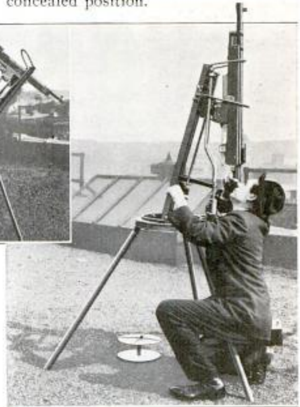
This Shows the New Mount Carrying a Machine Gun Operating at 90-Degrees Perpendicular Fire, against Air-Craft Attack. It will Carry Any Machine Gun Used in the Army
