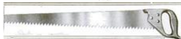
Saw Designed Especially for Pruning Trees: It Is 26 Inches Long and Has Three Teeth to the Inch
