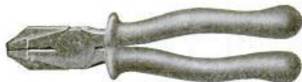
Metal Pliers for Electrical Workers, with Rubber-Covered Handles Insulated for 10,000 Volts
