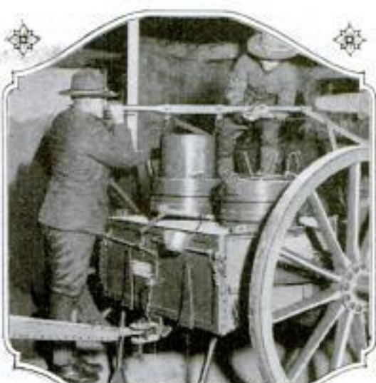
Placing Food in a Heat-Retaining Compartment of One of the New Kitchen Outfits: In This Way Victuals can be Prepared While an Army is Marching. General Efficiency is an Outstanding Feature of the Equipment
