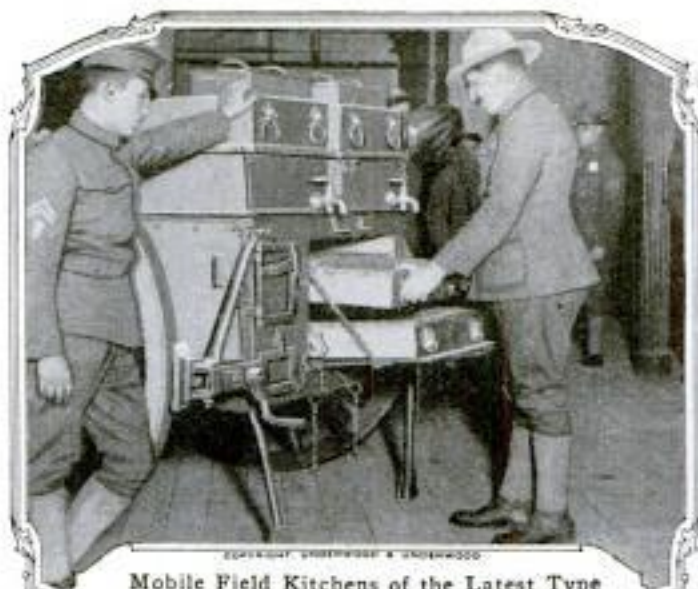
Mobile Field Kitchens of the Latest Type are Supplied with Insulated Heat-Retaining Compartments That Keep Food Piping Hot for Hours at a Time. A Unit Such as is Pictured Above is Adequate to Serve the Needs of 250 Hungry Soldiers
