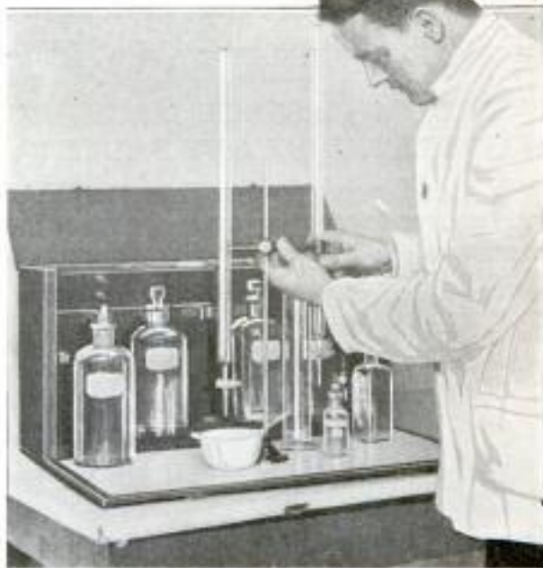
Compact Chemical Testing Outfit Designed Especially for Laundrymen, with Which They can Make Tests of Their Cleaning Materials, Thus Avoiding the Cost of Analyses by Chemists
