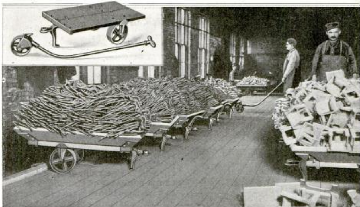
Labor-Saving Trucks, All of Which, Save One, Have Tongues and Front Wheels Detached: As the Material in the Trucks is Needed the Detachable Unit, Which is Clearly Shown in the Insert, is Hooked onto One of the Loads and It is Drawn Away
