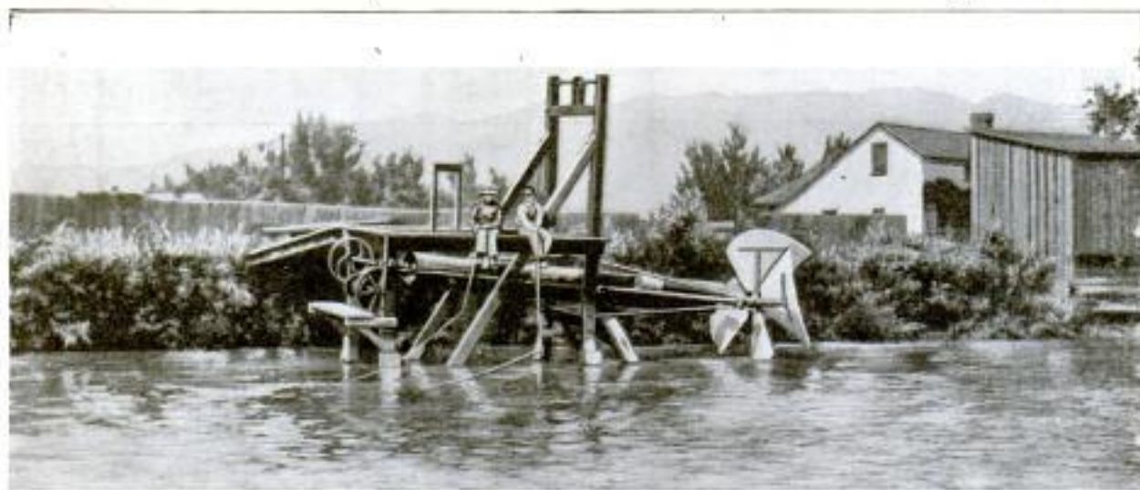
By Means of a Cable and the Drum, Shown at the Left of the Framework, This Novel Water Wheel is Lowered into the Current. As It Turns, a Screw in the Hollow Shaft Elevates the Water to a Trough That Leads to the Near-By Garden
