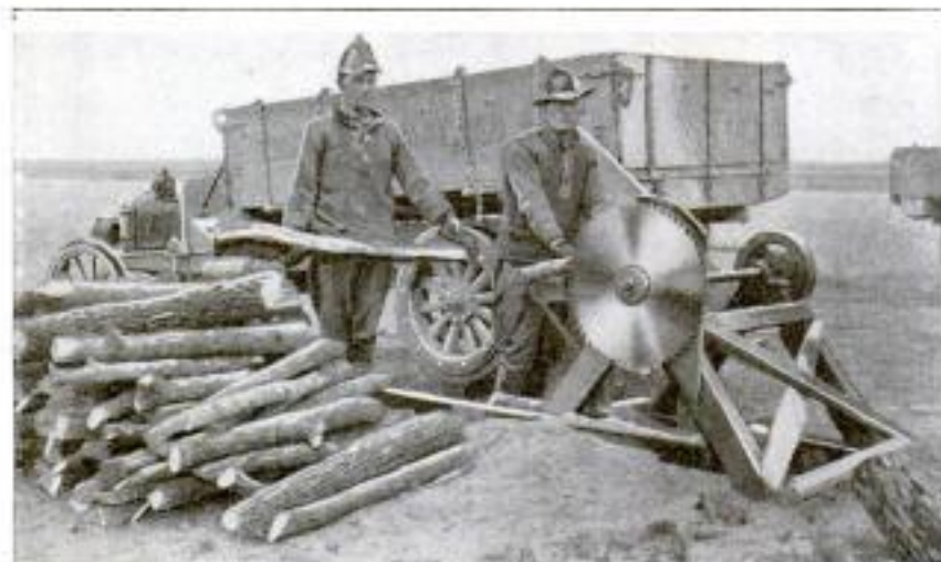
Sawing Wood with an Army Truck: Labor-Saving Arrangement Devised by One of the Soldiers on the Front Which Utilizes One of the Big Cars When It would Otherwise Be Idle
