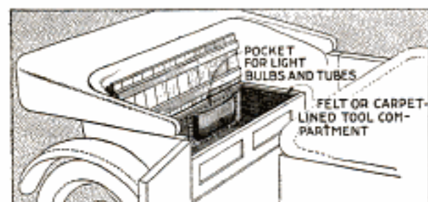
A Lining in the Tool Compartment Protects the Contents and Overcomes the Annoyance of Rattling
