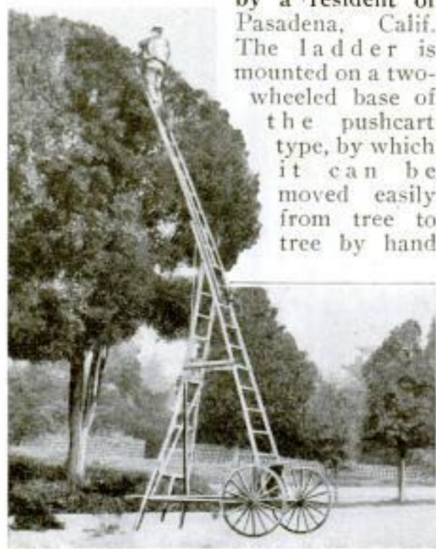
Trimming Trees with the Aid of an Extension Ladder, Wheeled About on Its Cart
