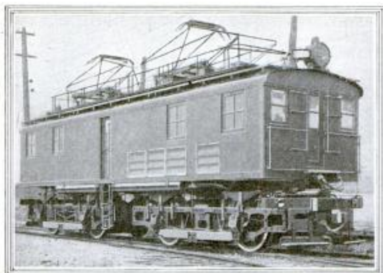
One of Three 120-Ton Electric Locomotives Recently "Knocked Down" at Erie, Pennsylvania, and Packed in Boxes for Export to Chile, Where They will be Used in Transporting Iron Ore from the Mines, 2,200 Feet above Sea Level, to the Shipping Port of Cruz Grande
