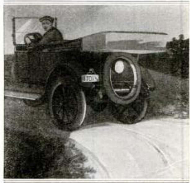
Backing a Car with the Aid of a Rear Searchlight Device, Operated Automatically by the Gear Shift in Reverse
