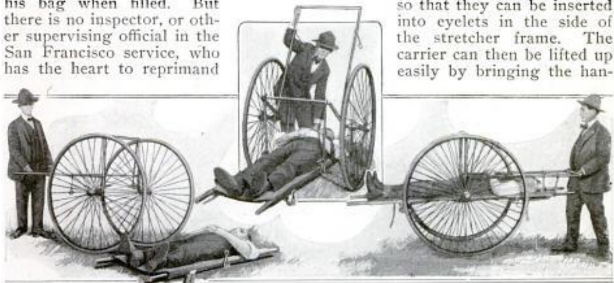
Stretcher Requiring the Services of But One Man Instead of Two: The Axle and Handles Serve as a Lever by Which the Laden Litter can be Lifted from the Ground. Because the Wheels Are Large, the Outfit can be Drawn over Rough Ground or up and down Stairs
