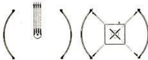
Diagram of Improved Revolving Doors, Showing How They Collapse Outward under Pressure
