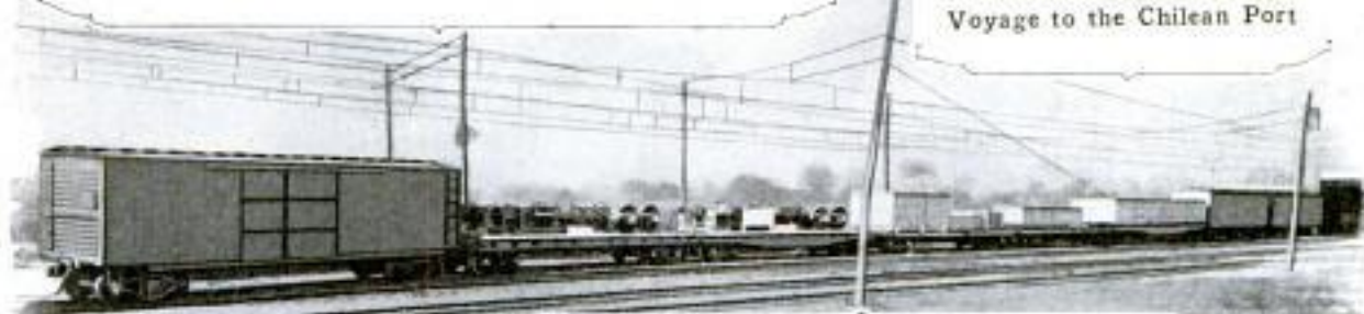
Each Locomotive When Taken Apart was Made Up into 62 Separate Packages Which Completely Filled Eight Box and Flat Cars, as Shown. The Largest and Heaviest Parcel Weighed 23 Tons and Measured More than 45 Feet Long; the Smallest could be Lifted by One Man
