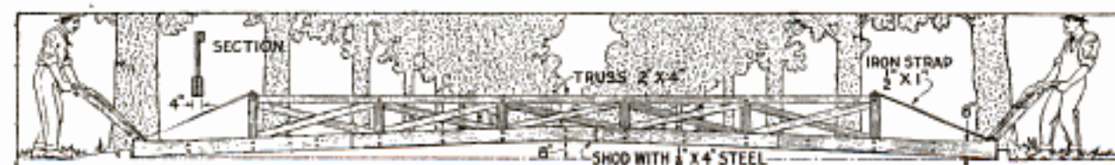
The Concrete was Tamped and the Pavement Crowned in One Operation by the Use of This Strike Board
