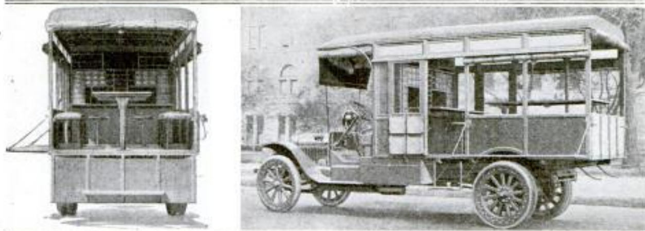
A National-Guard Headquarters on Wheels: This Motor Truck was Designed for the Use of Staff Officers of New York Troops Serving on the Mexican Border, and Makes a Wonderfully Compact Office. Interior View at the Left
