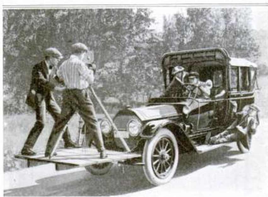
Motion-Picture Photographer Obtaining a Close-Up View of Speeding Motorists: The Camera is Securely Anchored to the Platform
