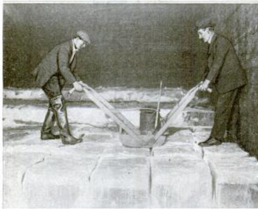
The Motor-Driven Cutter is Held in a Vertical Position so That It Is Possible to Cut along the Irregular Seams between Cakes of Ice That are Frozen Together
