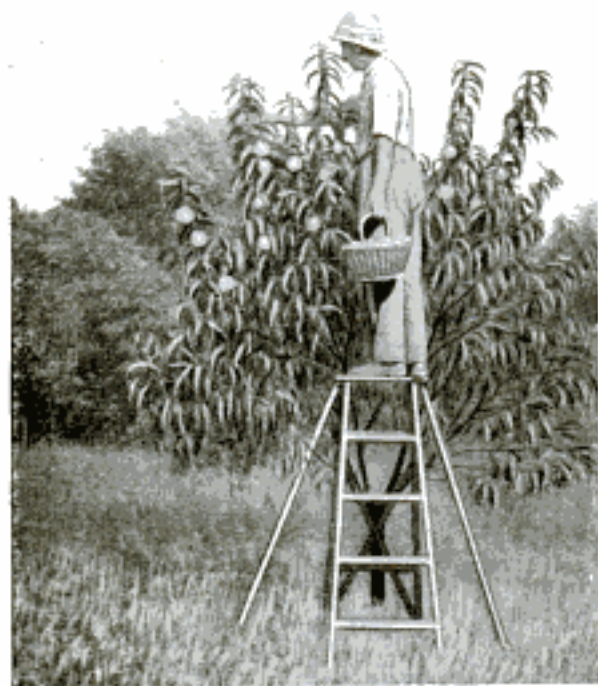
Stepladder Especially Suited for Use in an Orchard Because of the Two Supplementary Legs Which Serve as Braces at Either Side
