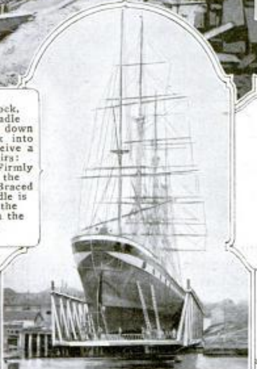
Full-Rigged Clipper Ship Safely Ashore in a Railway Dock, having been Hauled Out in the Cradle in Which it Rests: Vessels up to 4,000 Tons' Burden have been Handled Recently in This Way
