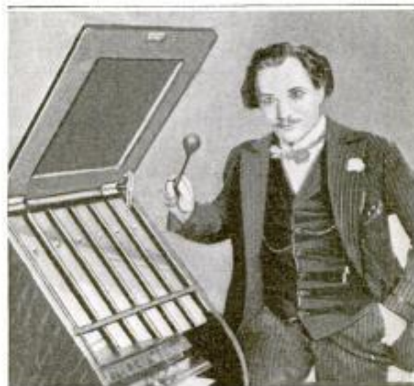
Testing the Pitch of Instruments in an Orchestra with a New Tuning Device: By Striking the Metal Bars Differences from Standard Pitch are Detected
