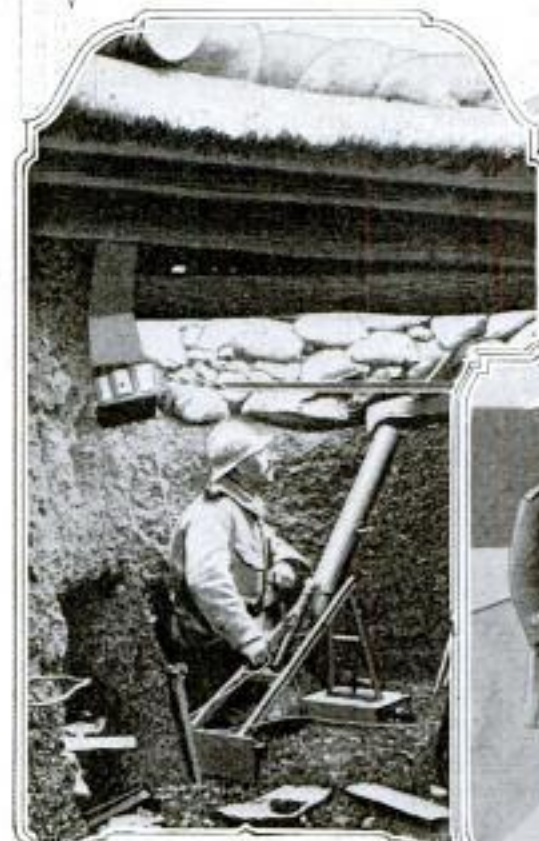
One of the Effective Weapons Used in Trench Warfare by the French is the Bomb Thrower Pictured in Use Herewith. The Instrument is Light, Easily Portable, and Electrically Operated. For Short-Range Work It is Very Valuable
