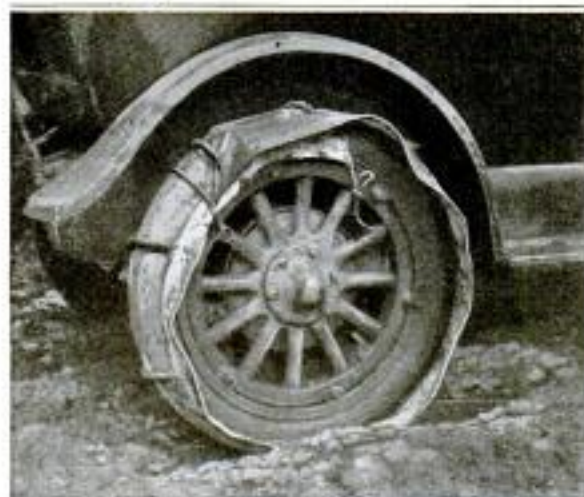
Right: Putting the Container, with Partly Unfolded Cloth Tread, in Position, Preparatory to Getting the Car Out of the Mud. Left: The Canvas Tread with Its Rope Grips in Place
