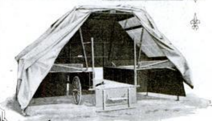
Designed Primarily for Campers and Overland Tourists, This Motor-Car Trailer is Successfully Used by the American Ambulance in France. It is Standard Equipment Manufactured in This Country and Folds Compactly When Not in Use. Opened, as Shown Above, Its Beds Accommodate Four Persons
