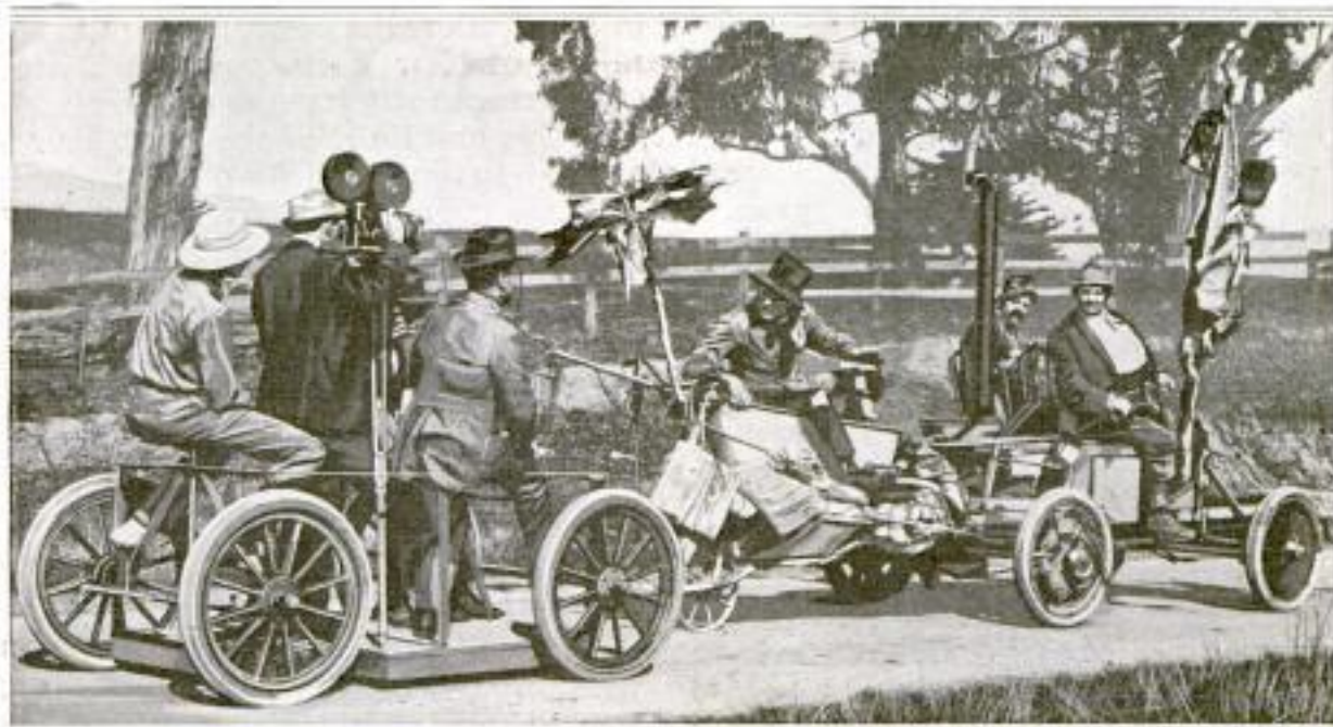
Efficient Type of Camera Truck Attached to the Rear of a Vehicle Used in a Comic "Movie" Scene, Showing How Continuous Close-Up Views are Obtained of a Moving Conveyance
