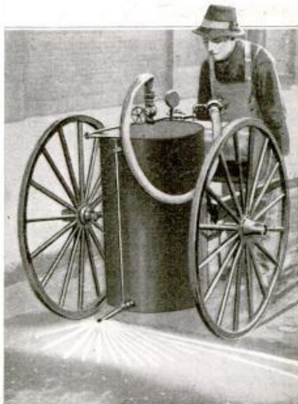
This Hand Sprinkler Carries a Small Tank of Compressed Air behind the Water Tank and Throws a Spray Clear across a Wide Pavement
