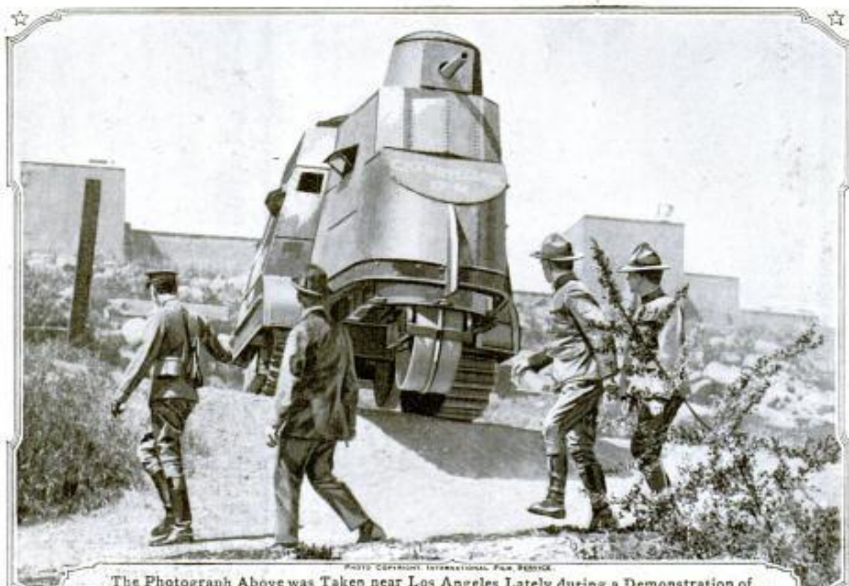
PHOTO COPYRIGHT INTERNATIONAL FILM SERVICE. The Photograph Above was Taken near Los Angeles Lately during a Demonstration of an American-Built "Tank" Car, Similar to Those Used by the British on the Western Battle Front. The Machine was Put through a Series of Severe Tests before Officers of the United States Army. As It was Climbing Out of a River and Ascending a Steep Embankment, the Soft Earth Gave Way and Caused the Heavy Machine to Turn Turtle
