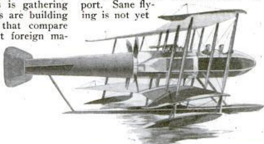
The Novel Mounting of the Propeller Makes the New Gallaudet Seaplane Especially Interesting. The Arrangement Permits the Use of a Streamline Fuselage and Affords Pilot and Observer Unobstructed Vision
