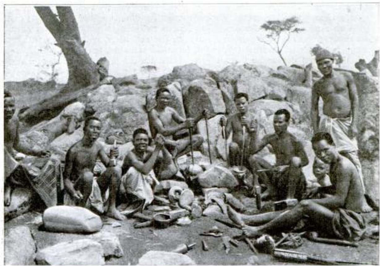
African Smiths and Their "Workshop": The Two Men at the Rear are Holding the Slender Handles of the Crude Bellows. Stones are Used for Anvils
