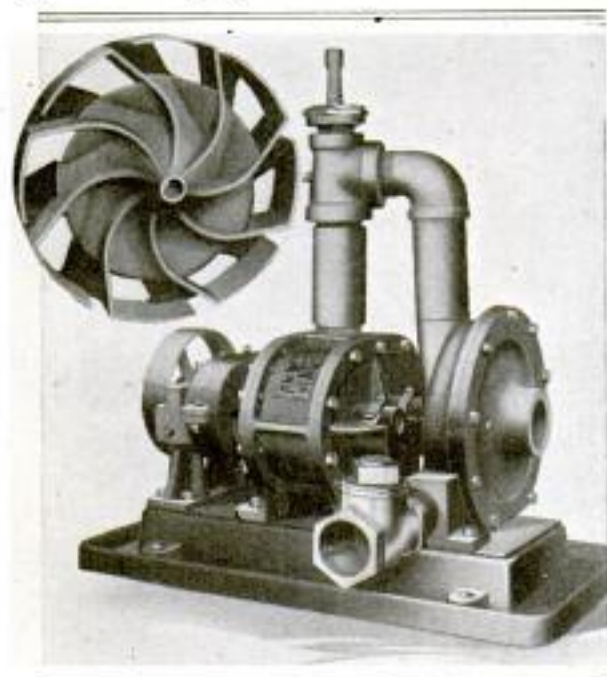
Stationary Vacuum Cleaner Which Washes the Dust from the Air as It Passes through the Rotary Separator Seen Above at the Left
