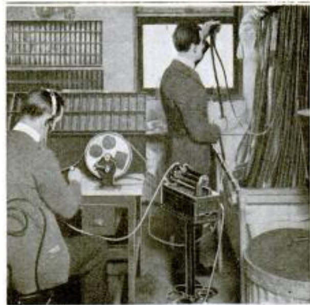
Cutting and Assembling Room, Showing the Film Cutter Following the Director's Orders, Which are being Reproduced from a Dictaphone Record
