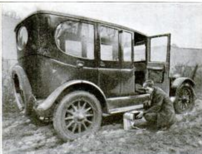
Right: Putting the Container, with Partly Unfolded Cloth Tread, in Position, Preparatory to Getting the Car Out of the Mud. Left: The Canvas Tread with Its Rope Grips in Place
