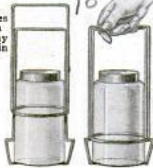
Fruit Jars can be Removed from Boiling Water, in Which Their Content has been Cooked, by Means of the Device Illustrated Above. Pictures Explain Its Operation
